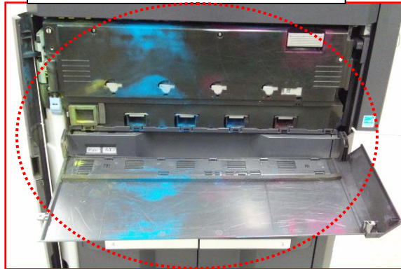
Toner stain on the conveying guide.
