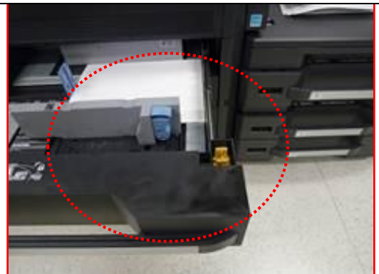
Toner stain on the conveying unit
