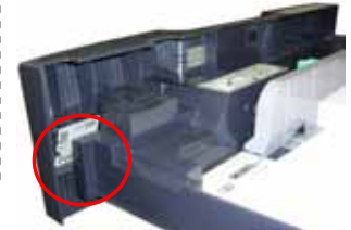
<Plate to confirm the gap>
