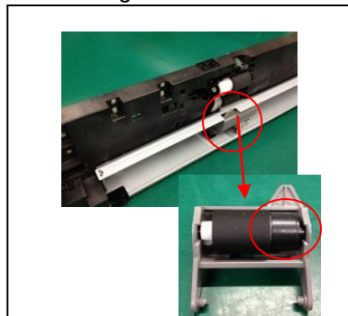
Fig.4 Check the installing direction of Pulley Retard
