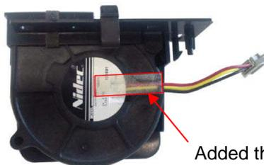
Added the sheet for pressing down the wire
