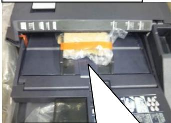
Packing material holding the feed tray lift plate only
