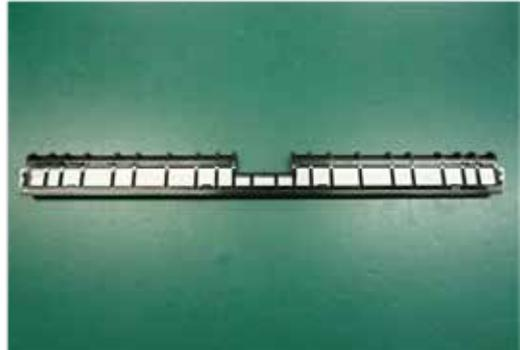
(2) Remove the conveying guide.
