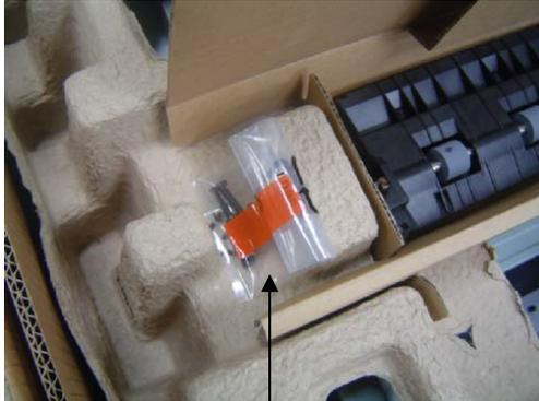
Fixing it on the topside of the upper left pad (at the side of the accessory box bundling the intermediate paper conveying unit) with the filament tape.
