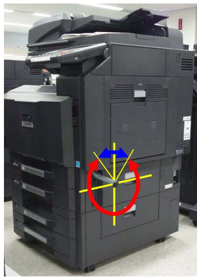
Use the front right side handle only for lifting up with the angle of 30° or less to the front or rear. Do not tilt the machine or move it laterally by using the handle.
