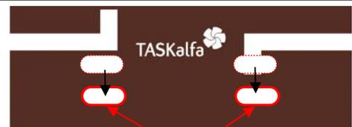
The holes for inserting hands are relocated downward.
