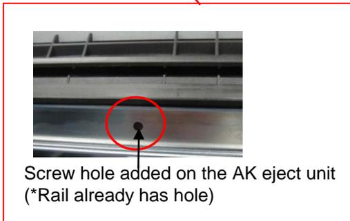
Screw hole added on the AK eject unit
