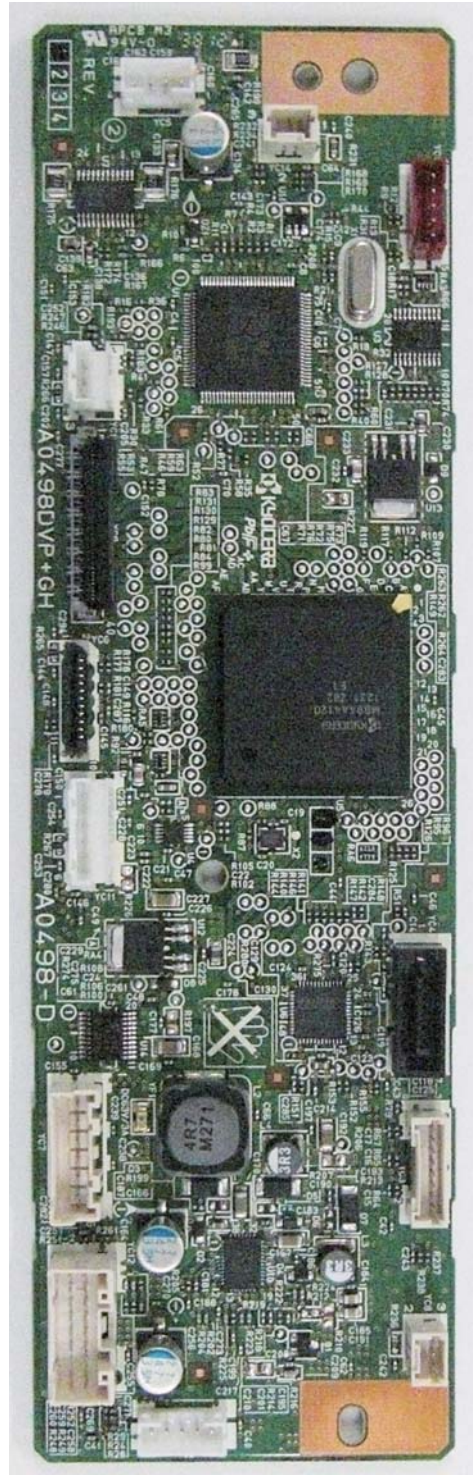
Figure 2-3-4 ISC PWB silk-screen diagram
