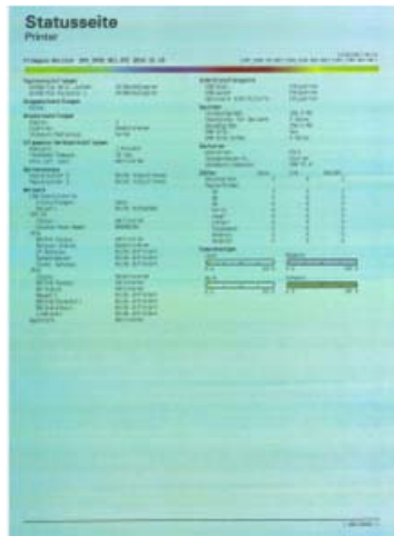
Cyan high voltage contact failure
