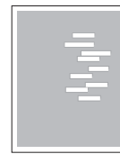
(1-15)Unevenly repeating horizontal streaks in the printed objects Colored spots in the printed objects
