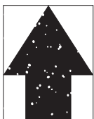
(2-14) Image is partly missing (Outlines objects and white dots)
