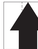
(2-17) Image center does not align with the original center
