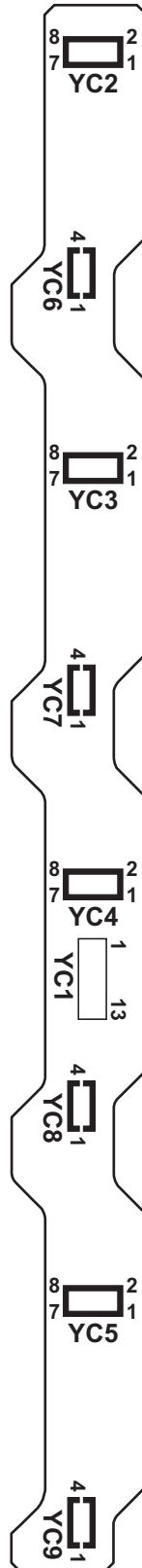
Figure 2-3-4 Drum relay PWB silk-screen diagram
