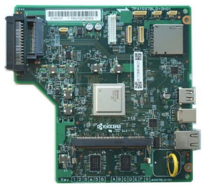
Controls the software such as the print data processing and provides the interface with computers.
