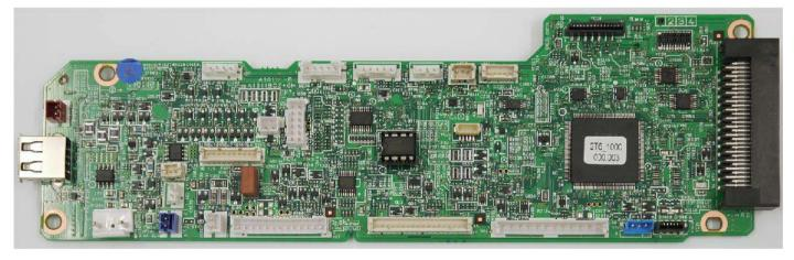
Controls printer hardware such as high voltage/bias output control, paper conveying system control, and fuser temperature control, etc.
