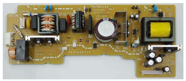
After full-wave rectification of AC power source input, switching for converting to 24 V DC for output. Controls the fuser heater.
