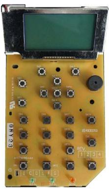
Consists the LCD, LED indicators and key switches.
