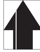
(3-4) White streaks are printed vertically
