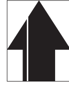
(1-5)White streaks are printed vertically
