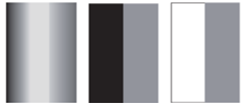
(2-8) Uneven density vertically
