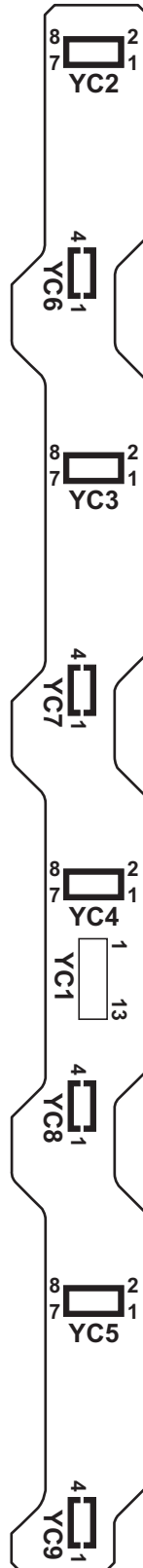
Figure 2-3-4 Drum relay PWB silk-screen diagram
