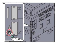
3 Insert the cord into the groove.
