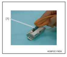
Using the soft cloth dampened with alcohol, wipe the Tray 1 Paper Separation Roller [5].
