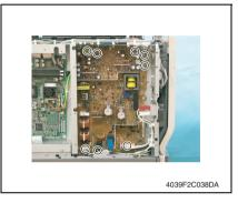
Remove all the Connectors on the DC Power Supply.
