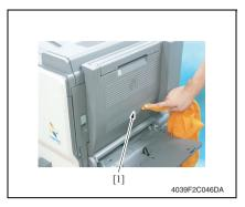
Using a soft cloth dampened with alcohol, wipe the outside of the Ventilation Section [1] clean of dirt.
