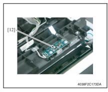
Repeat the step 6 and 7, and remove the IDC/Registration Sensor/2 (rear side) [12].
