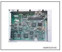
3. Remove all the Connectors and Flat Cables on the Controller Board.
