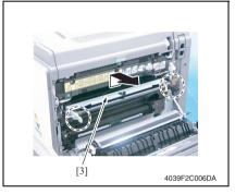
3. Hold the both sides and lift it to take out the Transfer Belt [3] a little.
