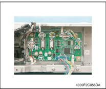
3. Remove all the Connectors on the Control Board.
