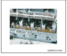
Remove all the Connectors and the Flat Cables on the PH Interface Board.
