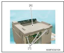
7. Remove three Screws [7], and remove the Exit Tray [8].
