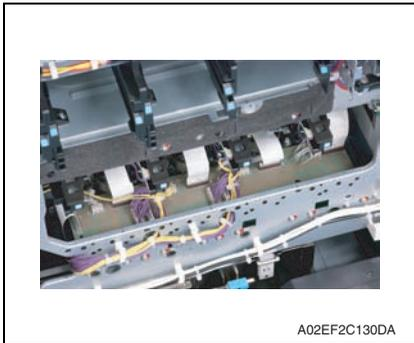
7. Remove all the connectors and the flat cables on the PH relay board.
