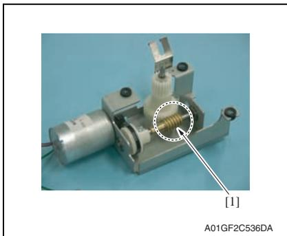
7. Apply the following grease to the worm gear [1].
