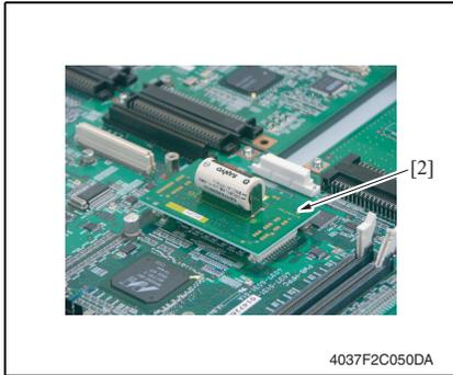
4. Remove the NVRAM [2] on the MFP Control Board.
