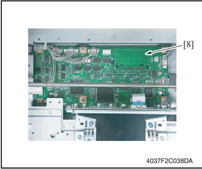
7. Remove all the Connectors and Flat Cables on the Image Processing Board [8].
