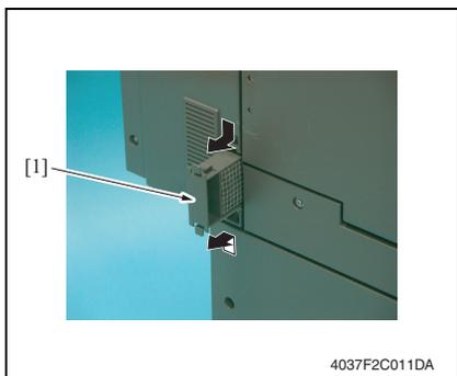
1. Holding onto the hook, remove the Ozone Filter [1].
