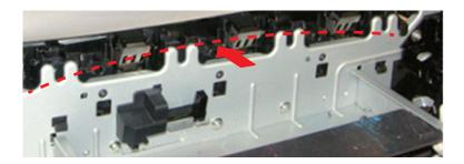
• Due to the CSIC contact ground plate failing to return or a bent contact pin, the imaging unit is unable to contact the CSIC.
