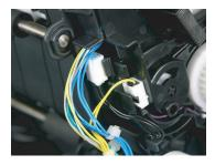
5. Route the harness of the duplex conveyance roller clutch as illustrated on the left.
