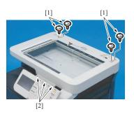
7. Remove four screws (rear side) [1] and three screws (front side) [2].
