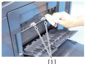
2. Using a cleaning pad dampened with alcohol, wipe the duplex unit transport roller [1] clean of dirt.
