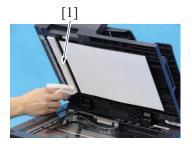
2. Using a cleaning pad dampened with alcohol, wipe the ADF paper guide [1] clean of dirt.
