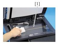
Using a cleaning pad dampened with alcohol, wipe the original glass [1] clean of dirt.
