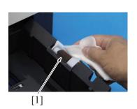
2. Using a cleaning pad dampened with alcohol, wipe the tray 1 separation roller [1] clean of dirt.
