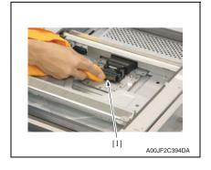
Using a cleaning pad dampened with alcohol, wipe the lens [1] clean of dirt.
