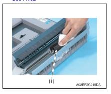
Using a cleaning pad dampened with alcohol, wipe the manual bypass tray feed roller [1] clean of dirt.
