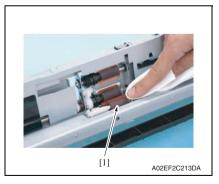
Using a cleaning pad dampened with alcohol, wipe the tray 2 separation roller [1] clean of dirt.
