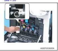
Wipe the areas around the waste toner collecting port clean of spilled toner and dirt using a cleaning pad with water or alcohol.
