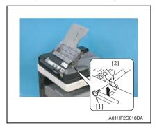
3. Remove the screw [1] and the mounting plate [2].
