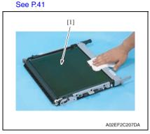
2. Using a cleaning pad, wipe the transfer belt [1].
