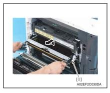
Hold the both sides and lift it to take out the transfer belt unit [1] a little.
