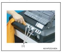
2. Using a soft cloth dampened with alcohol, wipe the roller [1].
