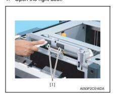
2. Using a cleaning pad dampened with alcohol, wipe the vertical transport roller [1] clean of dirt.
