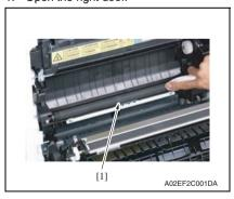
2. Using a cleaning pad with alcohol, wipe the timing roller [1] clean of dirt.
