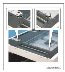
Adjust the guide support for the original glass moving unit by rotating the small screws (one on the near side and one on the far side) with the hexagon wrench (1.5 mm) to adjust the height.
