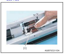
Using a cleaning pad dampened with alcohol, wipe the tray 2 feed roller [1] clean of dirt.
