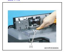
Wet a cloth with alcohol, and use it to wipe up the separation roller [1].
