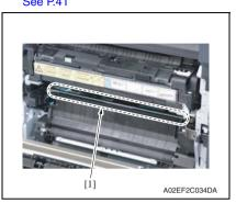
Wipe the image transfer entrance guide [1] clean of spilled toner and dirt using a cleaning pad with water or alcohol.
