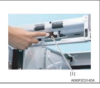
3. Using a cleaning pad dampened with alcohol, wipe the pick-up roller [1] clean of dirt.
