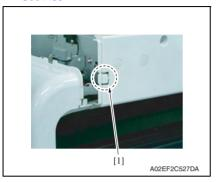
Remove the knockouts [1] on the IR right cover.
