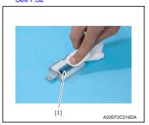
Using a cleaning pad dampened with alcohol, wipe the manual bypass tray separation roller [1] clean of dirt.
