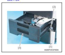
3. Remove the screw [1] and metal plate [2], and remove the tray 2 [3].
