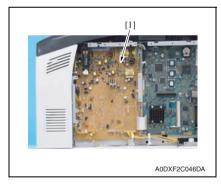
3. Remove ten screws [1], and remove the print control board protective shield [2].
