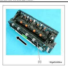
4. Slide the fusing front guide assy [1] for removal.
