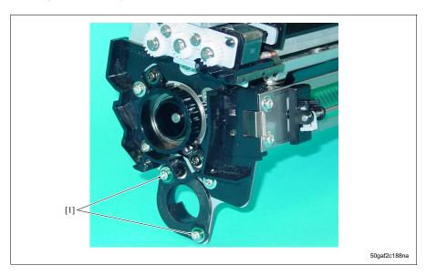
[1] Screws not allowed to be removed (Ds adjustment screws)
