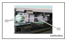
3. Remove two screws [2], and remove the Conveyance Front Cover /Rt [3].
