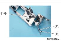
10. Remove the C-ring [14], the bearing [15], and remove the shaft Assy [16].
