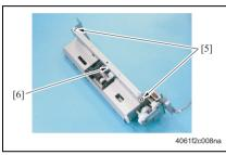
Remove two screws [5] and remove the Mounting Frame [6] for the Separation Roller Mounting Plate Assy.
