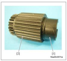
11. Remove the pick-up rubber [2] from the pick-up roller [1].
