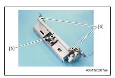
Remove two screws [4] and remove the Mounting Frame [5] for the Separation Roller Mounting Plate Assy.
