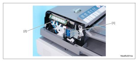
[1] Pressure roller release solenoid (SD1)
