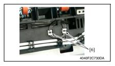
4. Remove two wiring saddles [6] and the harness.
