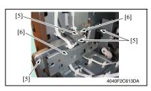
7. Remove four screws [5] and two harness protective metal brackets [6].
