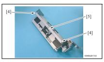
Remove two screws [4] and remove the Paper Separation Roller Mounting Bracket Assy [5] together with frame.
