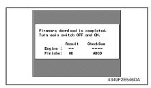
When the upgrading sequence is completed, turn OFF the main power switch.
