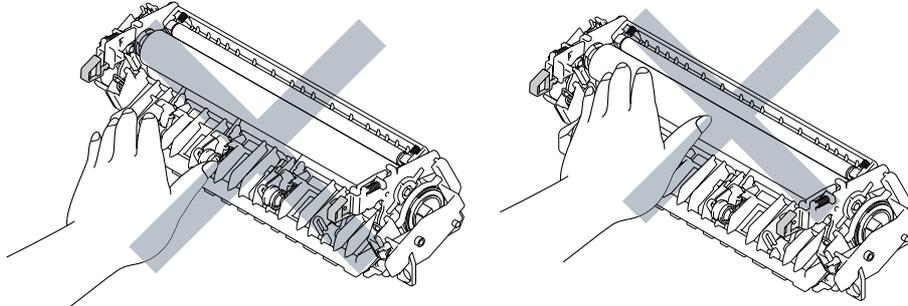
(5) Remove the pan B M4x20 Taptite screw, and then remove Fuser unit.
