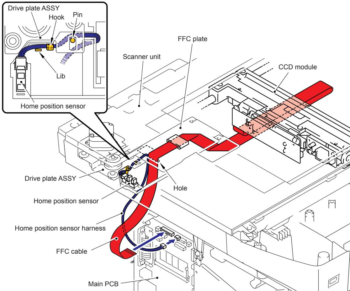
**20** Document scanner unit (Scanner motor, FB FG harness)
