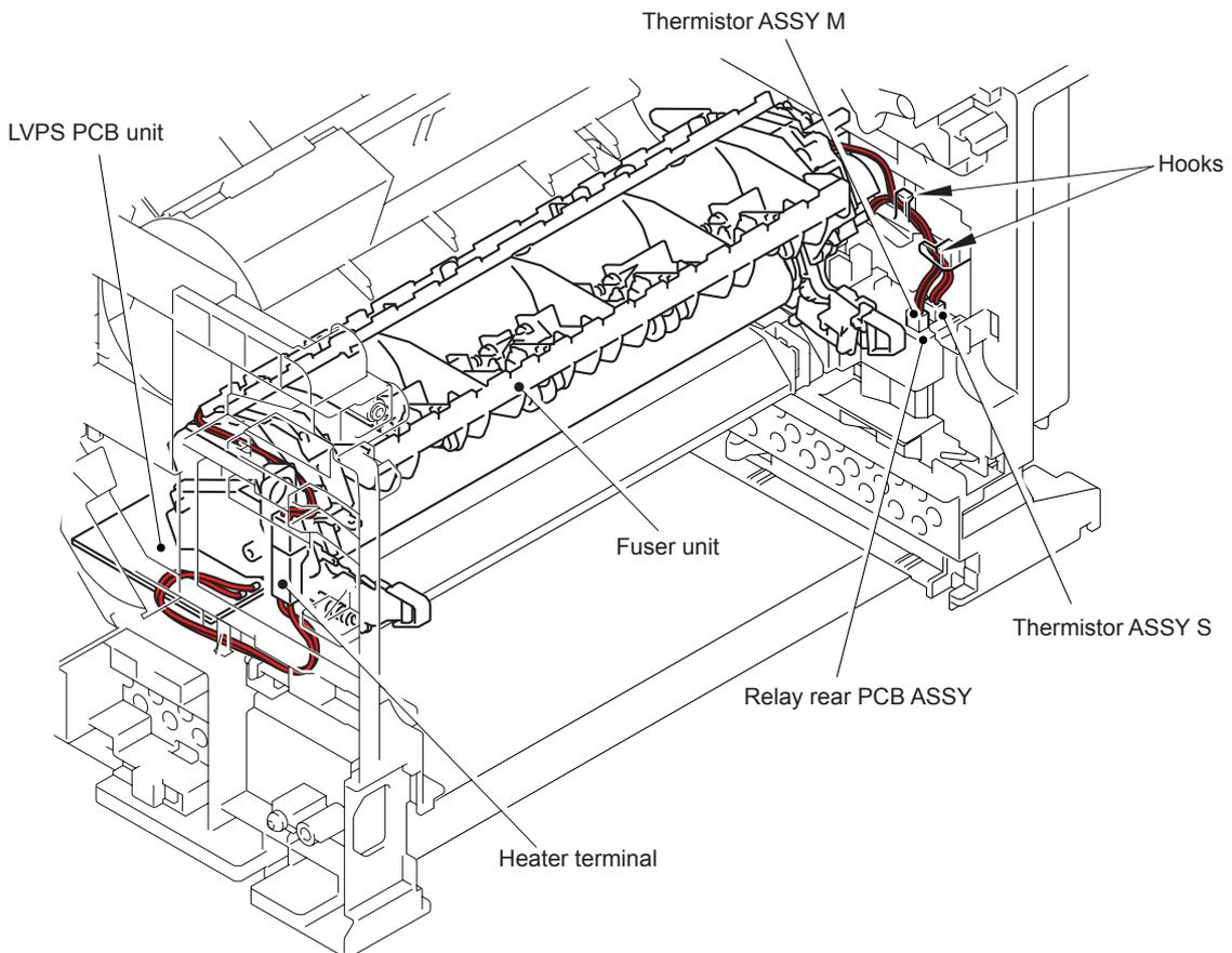
**25** Relay rear PCB ASSY, Ejector solenoid
