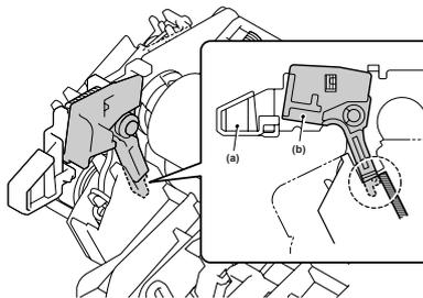
(22) Secure the Fuser unit with the pan B M4x20 Taptite screw.
