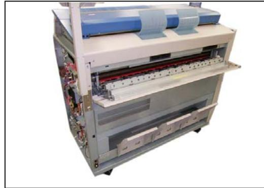
6. Remove the 4x6 screw (6) to remove the Plate 2 (7) on the right of machine.
