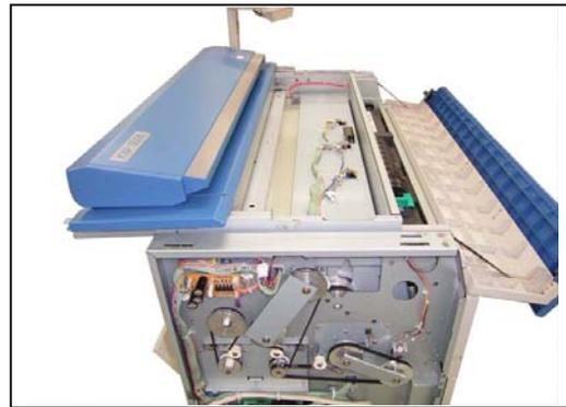
13. There are 2 pieces of Stopper (16) at both sides, which lock the LED Head Frame. Loosen the screw (17) and then slide the Stoppers (16) outside to unlock the LED Head Frame.
