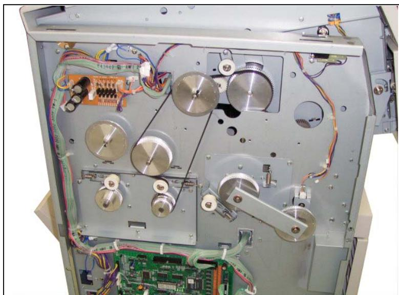
9. Loosen the 4x6 screw (17), move the Pulley 3 (18) toward the arrow mark, and then remove one more piece of **Belt 1** (19).
