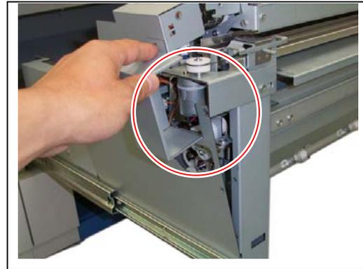
(2) Make sure that the step part (8) on the lower side of each Cover 3 (6) and Cover 7 (7) is inside of the plate (9).
