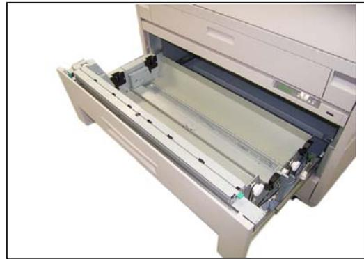
3. Remove the 4x6 screw (3) to remove the Bracket 5 (4).
