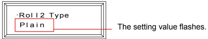
2. Pressing [←] key or [→] key, indicate the type of the roll paper installed in the Roll 2.
