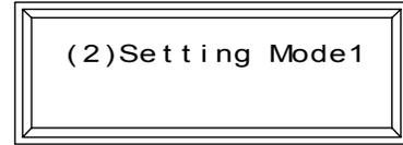
2. Press the [ENTER] key to enter the Setting Mode 1. The LCD initially indicates “Roll 1 Type”.
