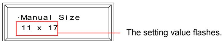
2. Indicate the same size with the used cut sheet paper pressing [←] key or [→] key.
