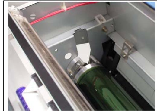
20. Remove the **Photoconductive Drum** (30), and replace it with the new one.
