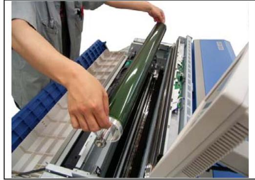
2. Wipe the surface of Photoconductive Drum with a dry cloth.
