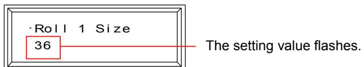
2. Indicate the same size with the roll paper in the Roll Deck 1 pressing [←] key or [→] key.
