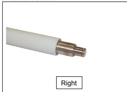
23. Pressing down Roller Holder Assy (41), slide the **Drive Roller 2** (42) to the left, and then remove it.
