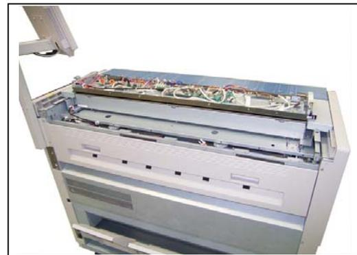
7. Pull up Lever 2 (8) to open the Engine Unit.
