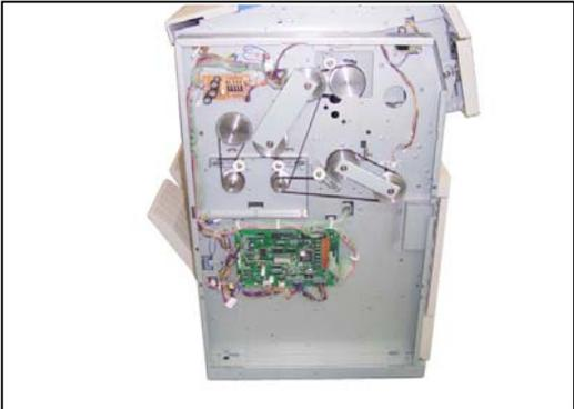
4. Loosen the 4x6 screw (4), move the Pulley 3 (5) toward the arrow mark, and then remove the **Belt 1** (6).
