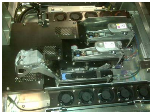
Picture 1: Black/Cyan Printhead latch in the open position
