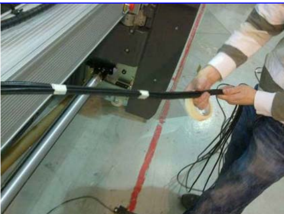
Route ink tubes pair by pair back into position
