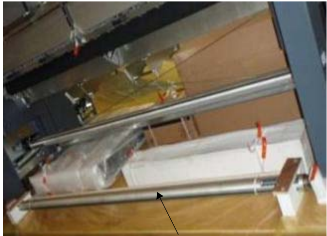
Media Drive Input spindle
