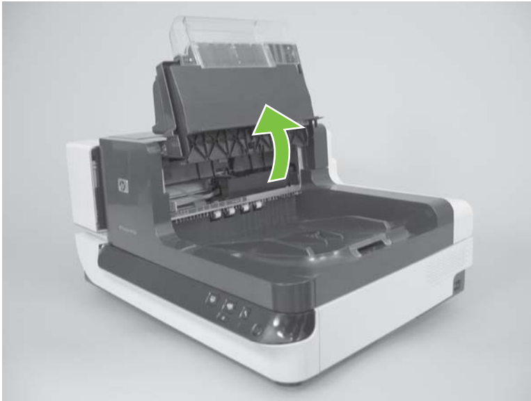
Figure 5-2 Remove the imprinter cartridge (1 of 4)
