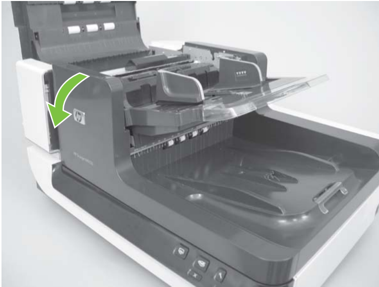
Figure 5-21 Remove the ADF front cover (3 of 5)
