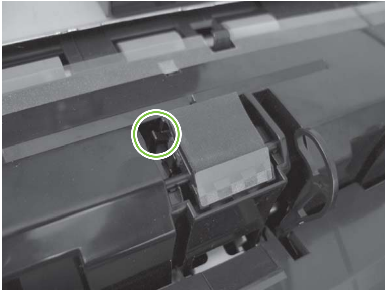
Figure 5-14 Remove the separation-pad assembly (1 of 3)
