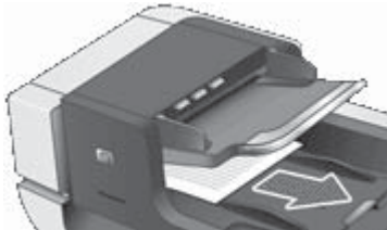
Figure 6-23 Clear jams from the ADF (4 of 5)
