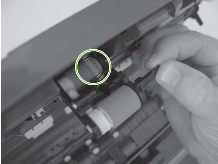
Figure 5-12 Reinstall the pickup-roller assembly (1 of 2)
