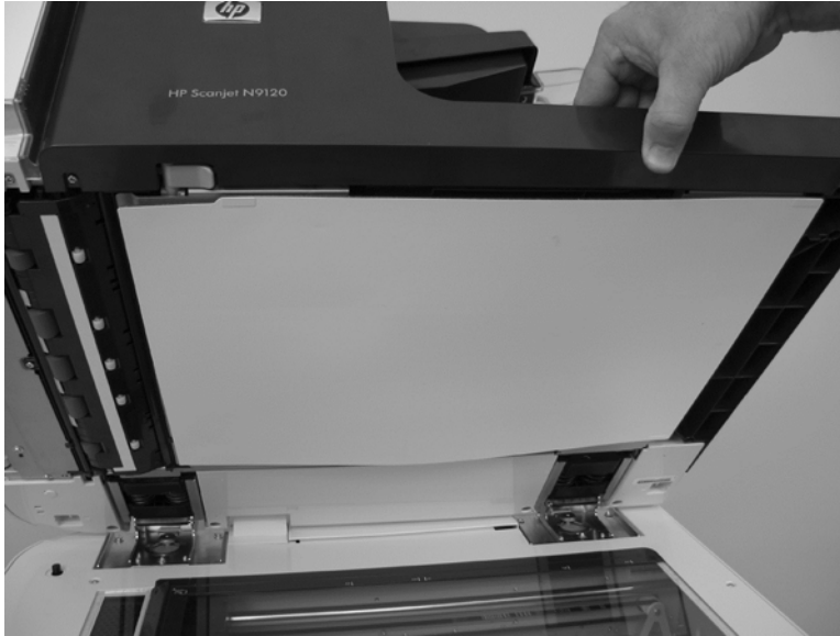
Figure 5-8 Remove the ADF base reflector (1 of 2)
