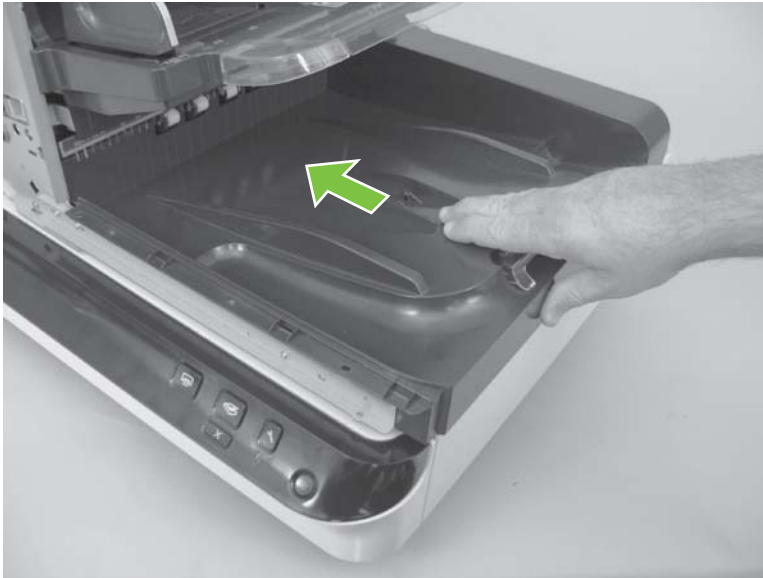
Figure 5-207 Reinstall the ADF output tray (1 of 4)
