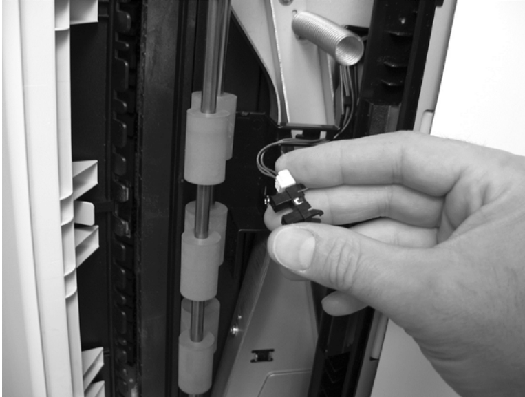
Figure 5-134 Remove the flatbed scan position sensor (2 of 2)
