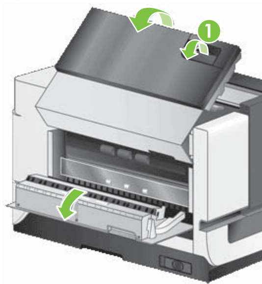
Figure 3-3 Clean the ADF (3 of 5)
