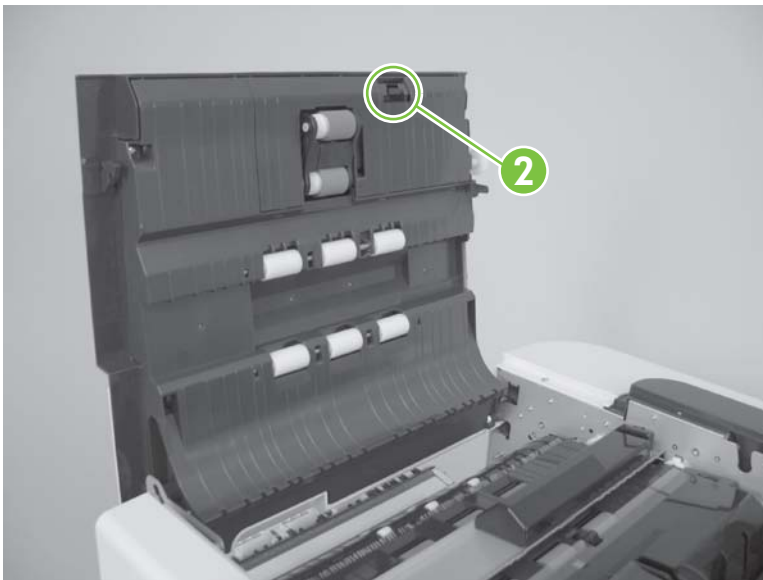
Figure 5-212 Remove the pickup-roller cover (2 of 3)
