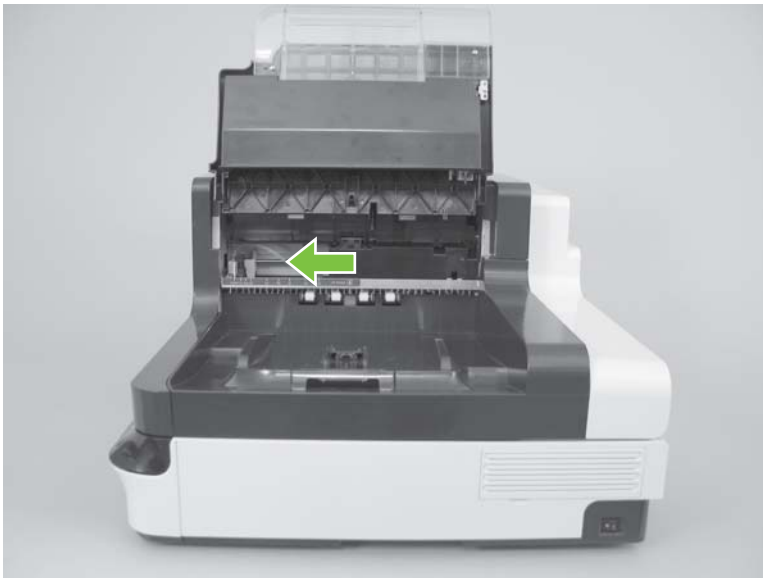
Figure 5-3 Remove the imprinter cartridge (2 of 4)
