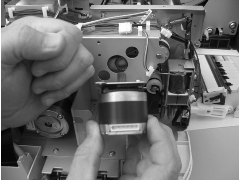
Figure 5-98 Remove the ADF feed-motor assembly (2 of 4)
