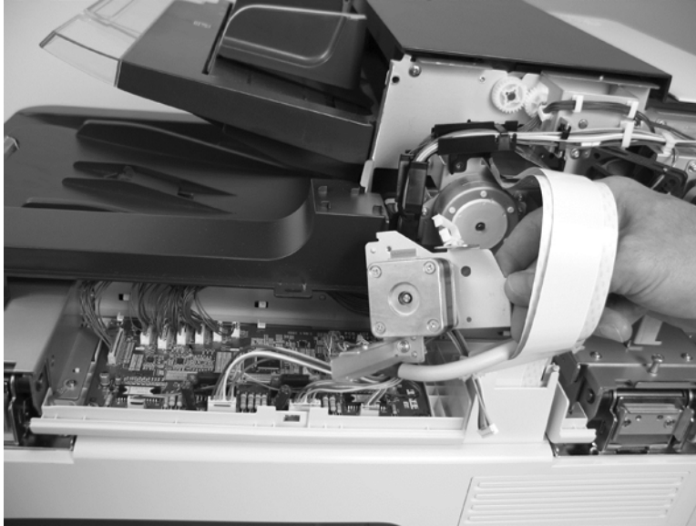
Figure 5-94 Remove the ADF exit-motor assembly (5 of 7)
