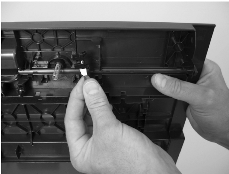
Figure 5-141 Remove the pick-up roller sensor (4 of 4)
