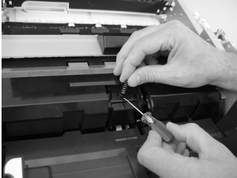
Figure 5-200 Remove the separation-pad spring
