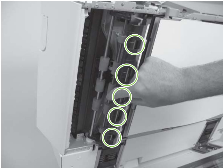
Figure 5-166 Reinstall the ADF cal-strip assembly (4 of 7)
