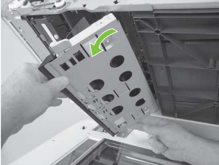
Figure 5-217 Remove ADF jam door 3 (3 of 4)
