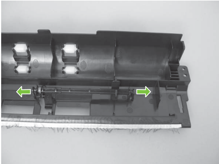
Figure 5-198 Remove the scan position sensor arm (2 of 2)
