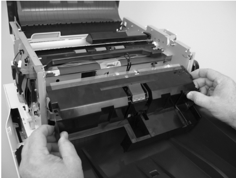
Figure 5-225 Remove the ADF shingle wall (4 of 4)
