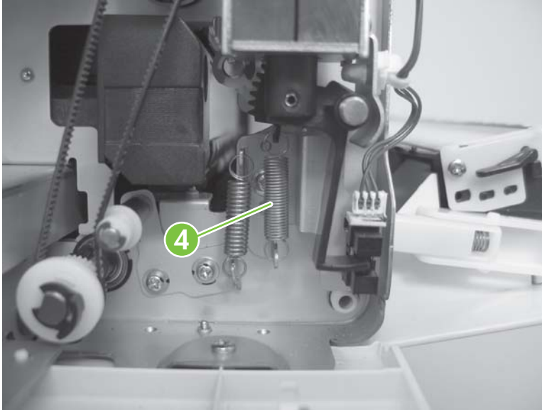
Figure 5-230 Remove the ADF background-solenoid assembly (3 of 5)
