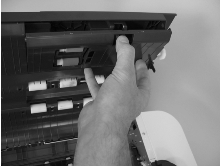
Figure 5-213 Remove the pickup-roller cover (3 of 3)
