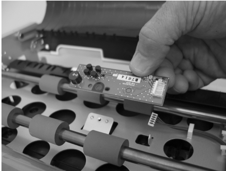
Figure 5-123 Remove the lower multi-pick sensor PCA (2 of 2)
