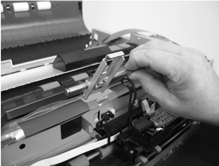
Figure 5-194 Remove the input-tray-elevator arm (5 of 5)
