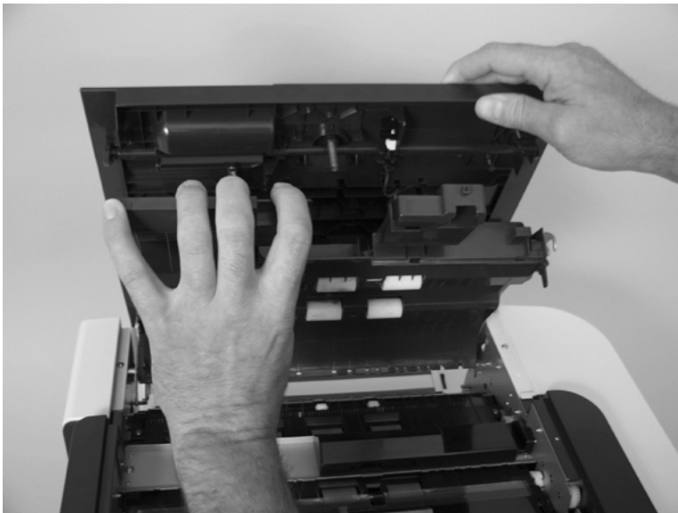
Figure 5-139 Remove the pick-up roller sensor (2 of 4)
