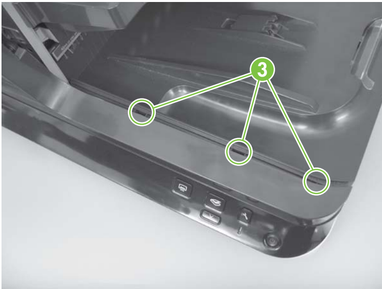
Figure 5-22 Remove the ADF front cover (4 of 5)
