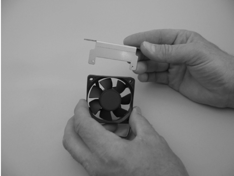
Figure 5-243 Remove the scanner carriage-motor fan (5 of 5)
