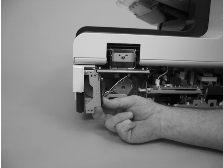
Figure 5-241 Remove the scanner carriage-motor fan (3 of 5)
