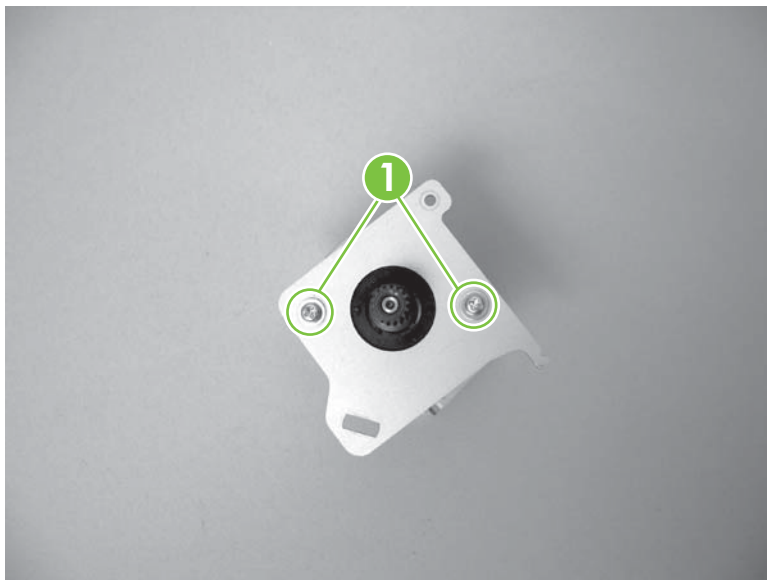
Figure 5-114 Reinstall the ADF pick-motor assembly (1 of 5)
