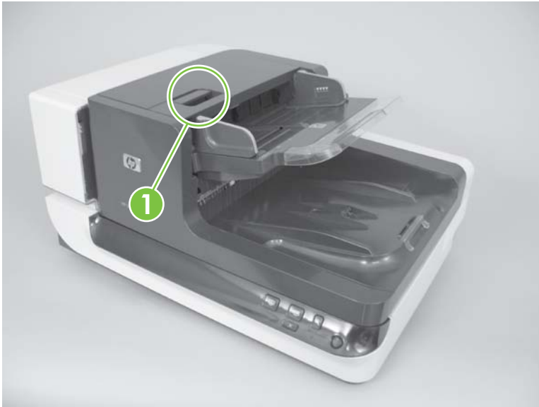
Figure 5-211 Remove the pickup-roller cover (1 of 3)
