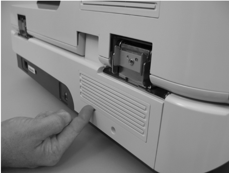
Figure 5-6 Remove the fan filter (1 of 2)
