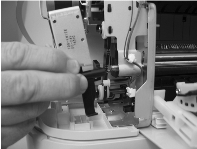
Figure 5-232 Remove the ADF background-solenoid assembly (5 of 5)
