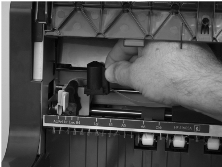
Figure 5-5 Remove the imprinter cartridge (4 of 4)
