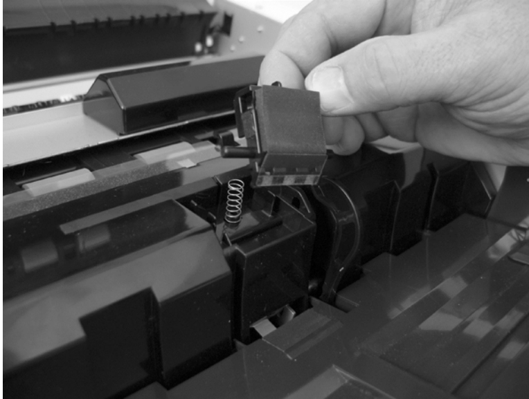
Figure 5-16 Remove the separation-pad assembly (3 of 3)
