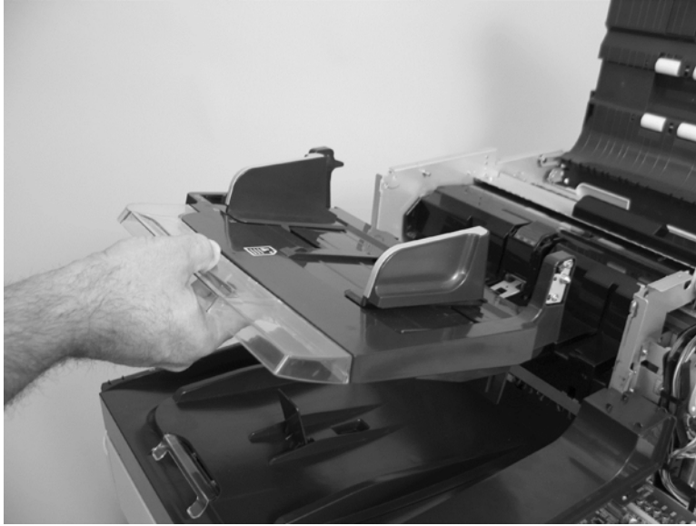
Figure 5-203 Remove the ADF input-tray assembly (3 of 3)
