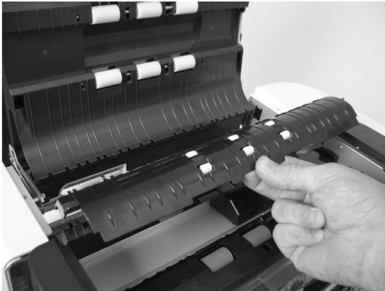
Figure 5-175 Remove the ADF top corner inner paper path guide (2 of 2)
