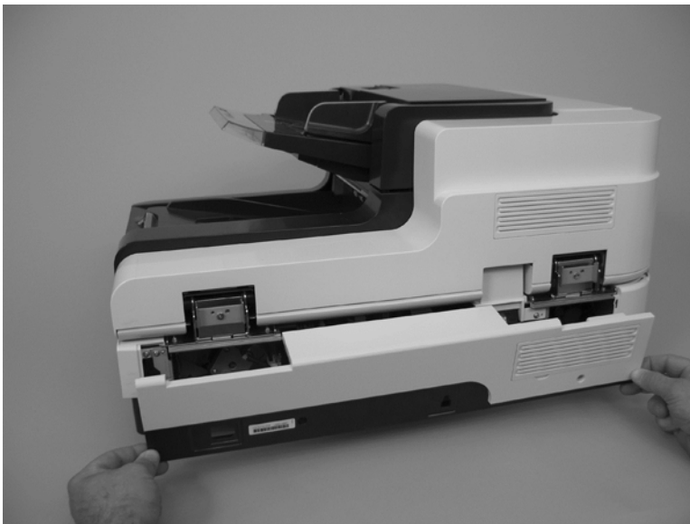
Figure 5-28 Remove the scanner back cover (2 of 2)
