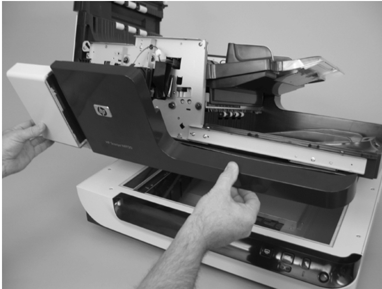
Figure 5-23 Remove the ADF front cover (5 of 5)
