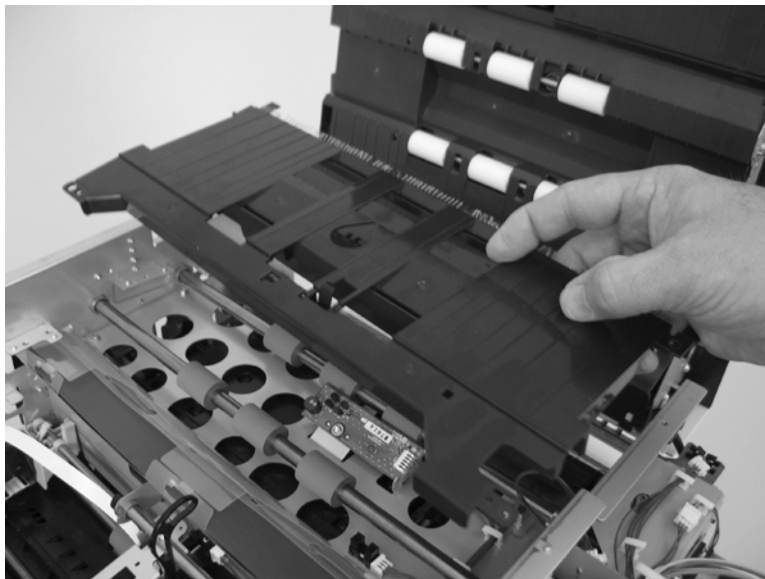
Figure 5-178 Remove the lower multi-pick sensor cover (3 of 3)
