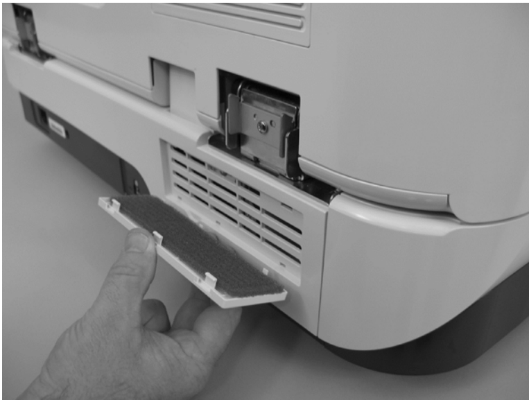
Figure 5-7 Remove the fan filter (2 of 2)
