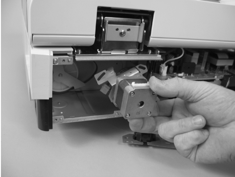
Figure 5-249 Remove the scanner carriage motor (3 of 5)
