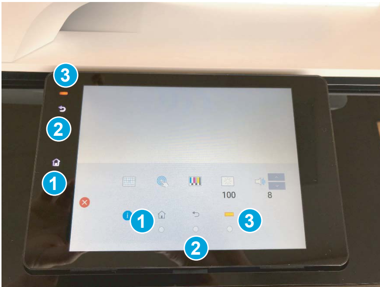
Figure 2-8 Test the control panel LED buttons
