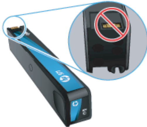
Figure 2-35 Examine the cartridges
