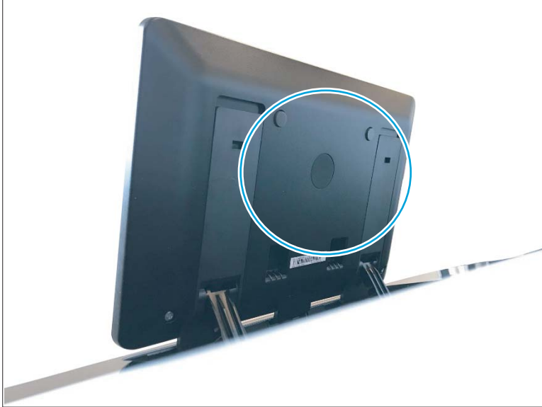
Figure 2-5 Press and hold down the diagnostics-access button
