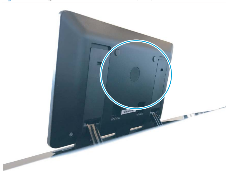
Figure 2-4 Diagnostic-tests access button (MFP)
