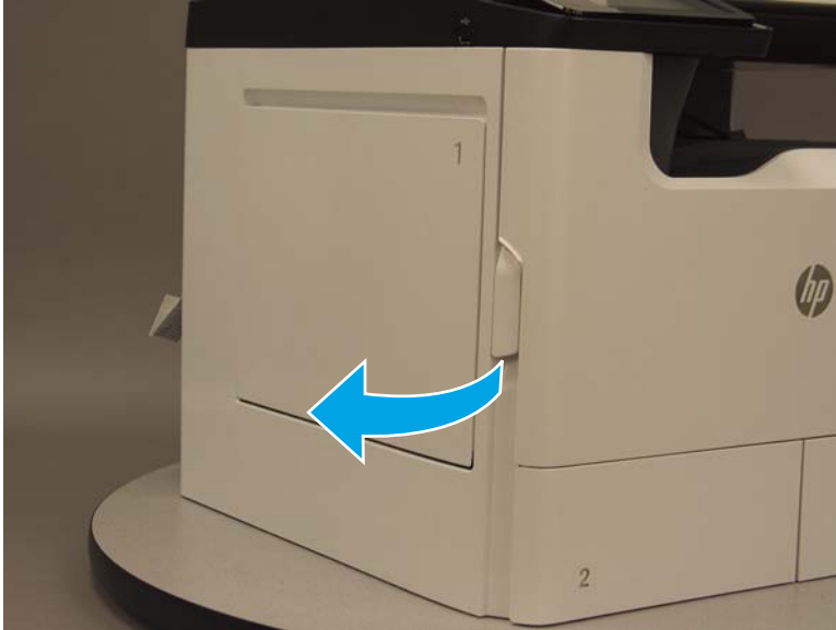
Figure 1-790 Open the left door
