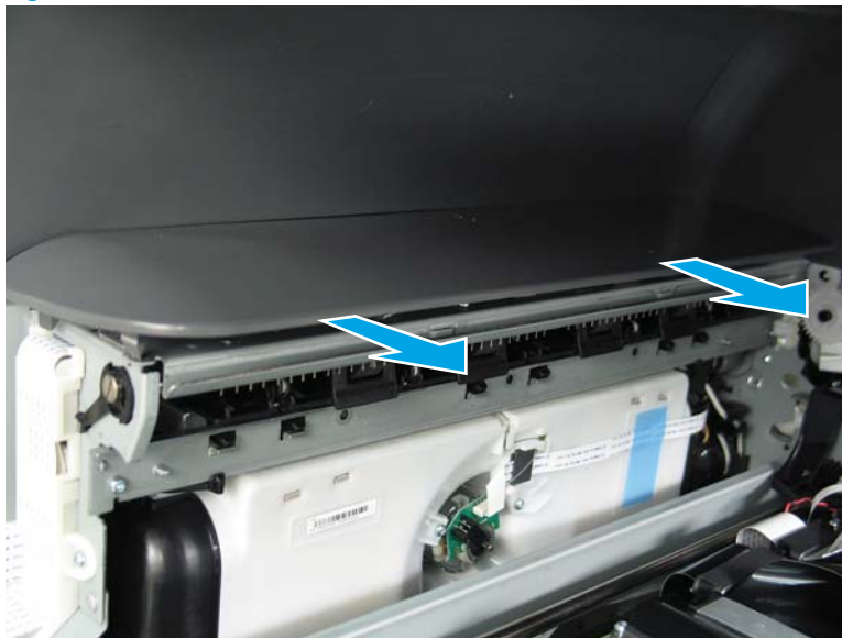
Figure 1-1115 Remove the cover
