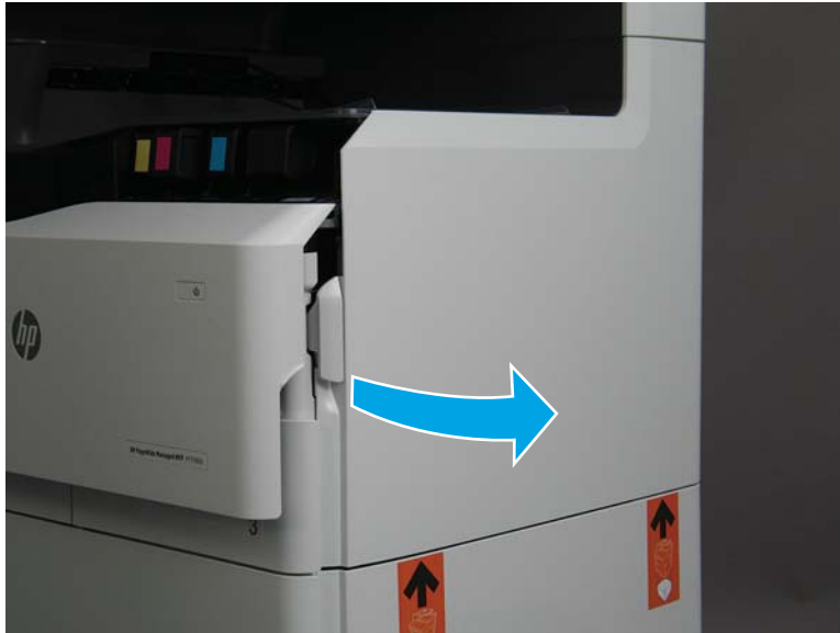
Figure 1-204 Open the right door
