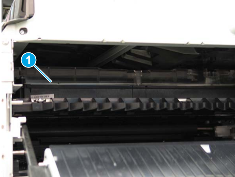
Figure 1-663 Printhead wiper in the home position
