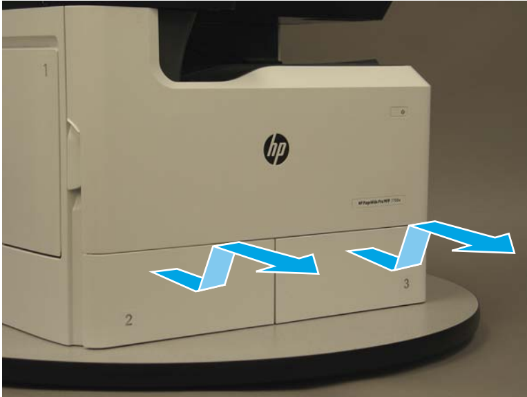
Figure 1-1690 Remove the tray or trays
