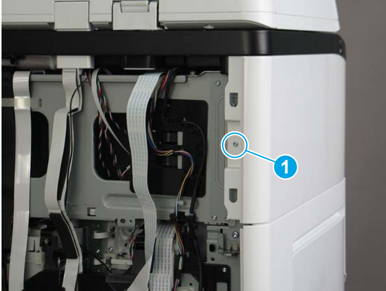
Figure 1-423 Remove one screw
