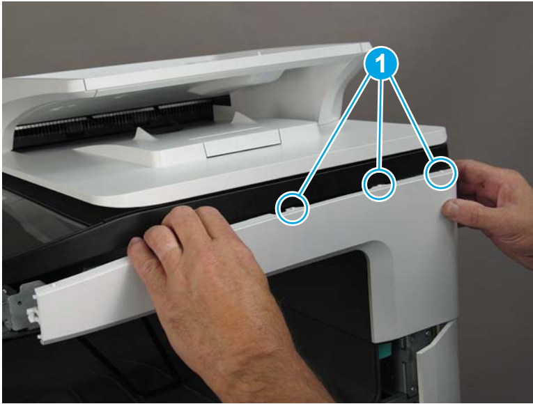
Figure 1-439 Release three bosses
