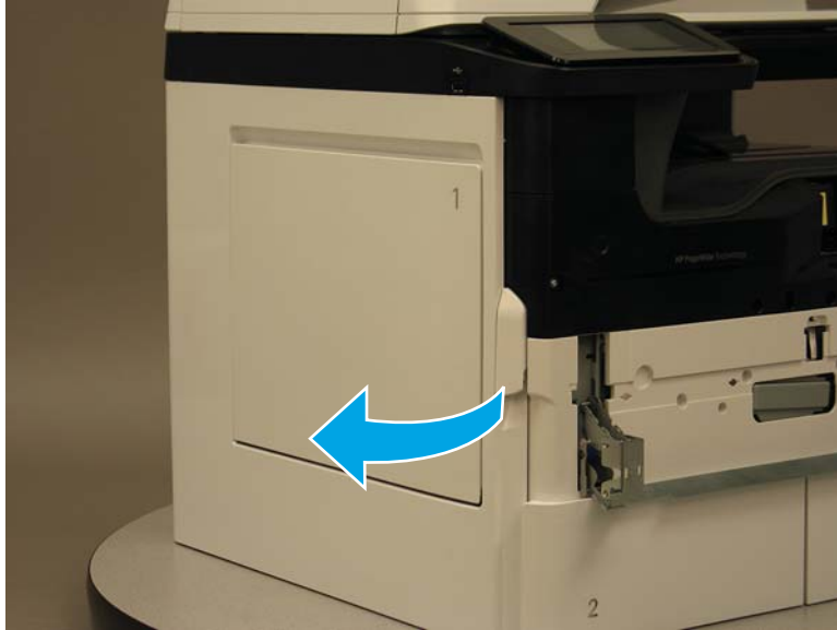
Figure 1-109 Open the left door
