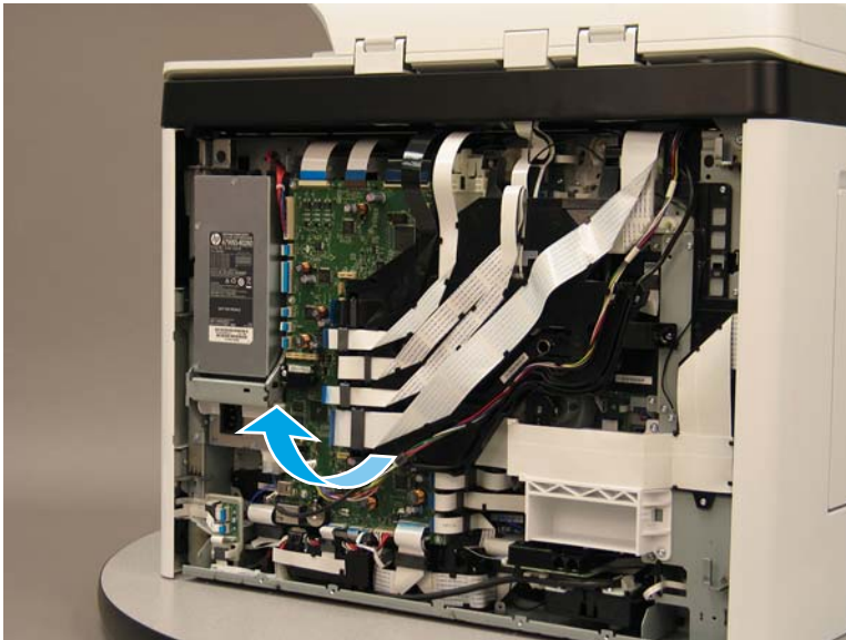
Figure 1-237 Rotate the FFC tray guide up (MFP models)
