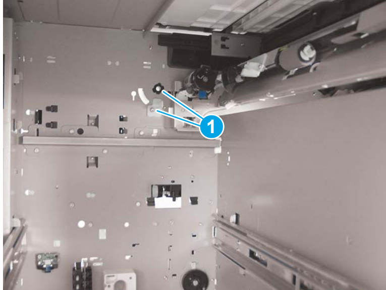
Figure 1-1804 Install the HCI pickup roller arm(s)
