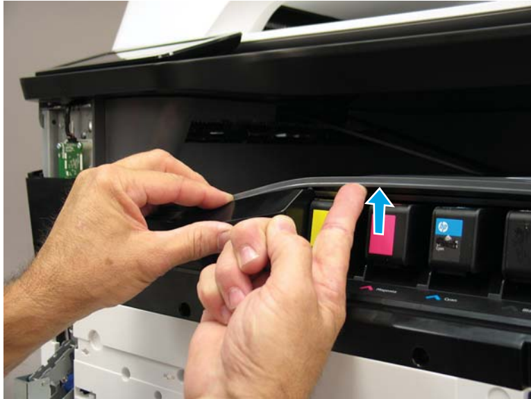
Figure 1-376 Release one tab
