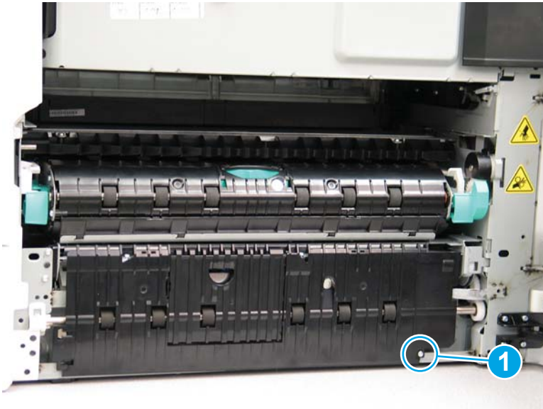
Figure 1-861 Remove one screw
