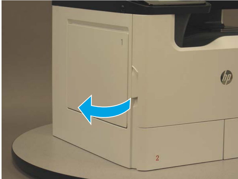
Figure 1-1231 Open the left door
