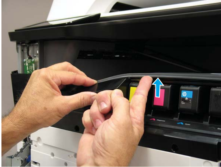
Figure 1-138 Release one tab
