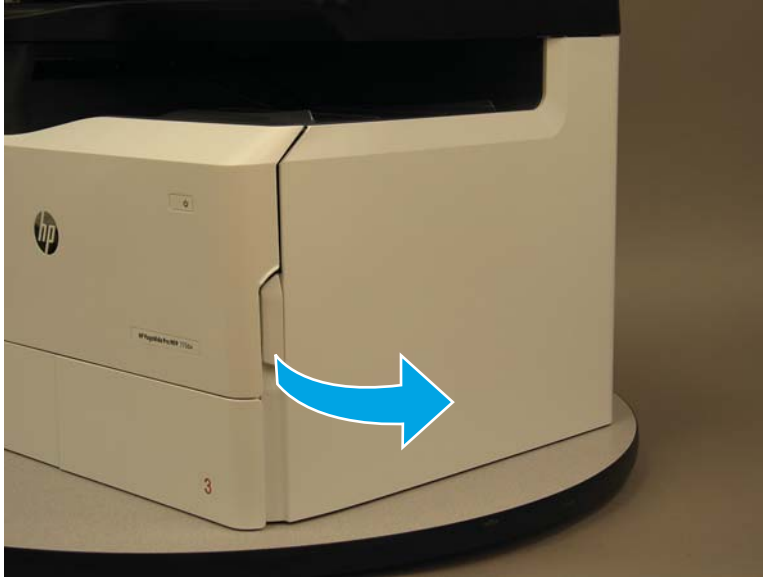
Figure 1-48 Open the right door
