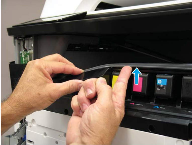
Figure 1-1484 Release one tab
