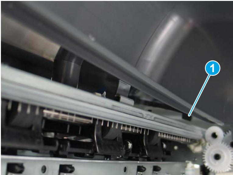
Figure 1-1113 Release one tab
