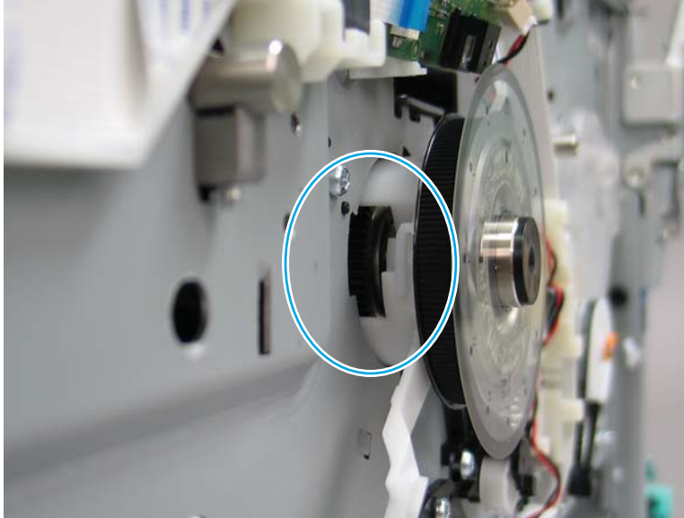
Figure 1-673 Note the clip on the bearing surface
