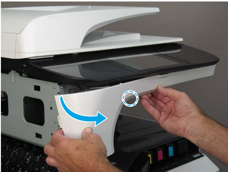
Figure 1-432 Release one tab
