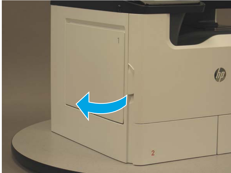
Figure 1-1345 Open the left door
