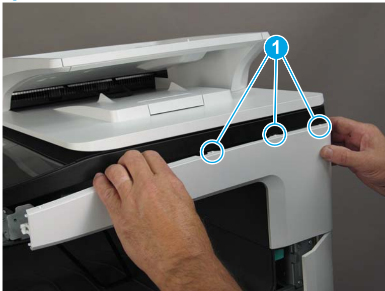
Figure 1-307 Release three bosses
