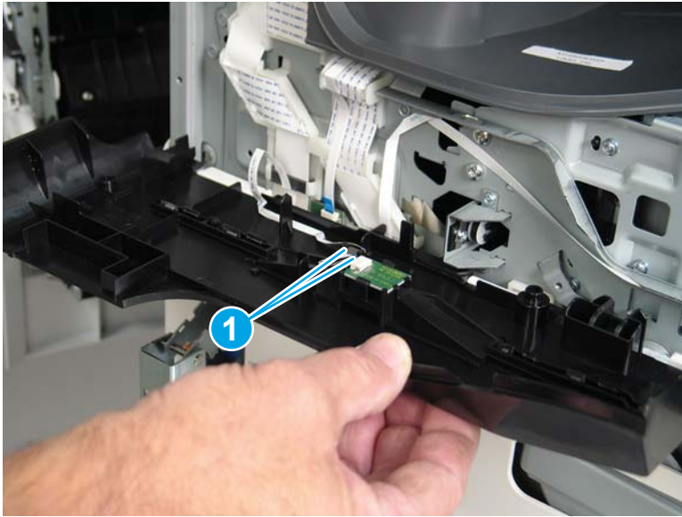
Figure 1-451 Release the cover
