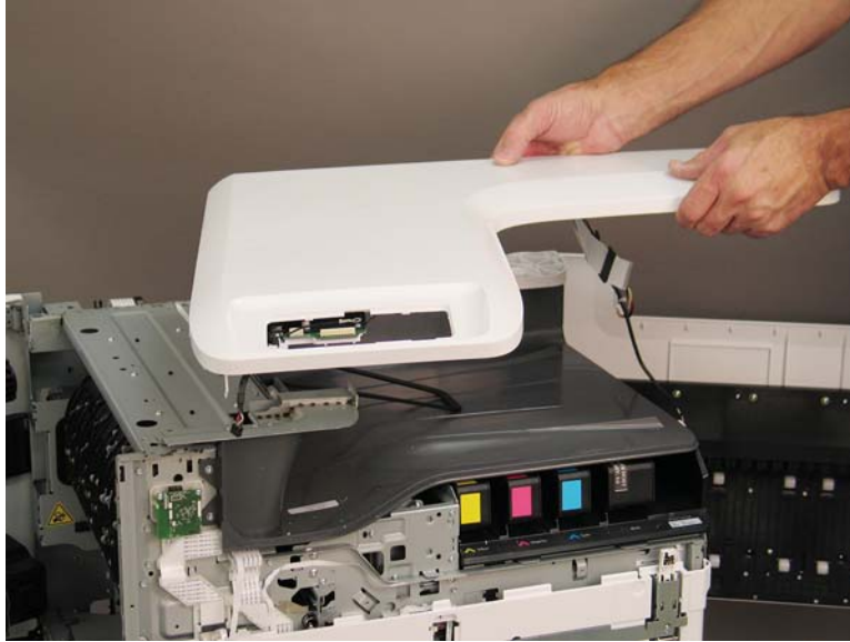
Figure 1-387 Remove the top cover
