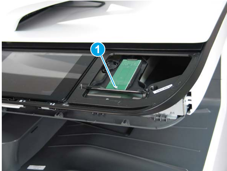
Figure 1-1194 Remove one screw
