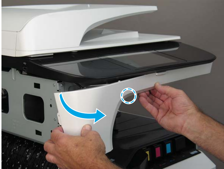
Figure 1-1082 Release one tab
