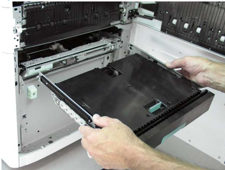
Figure 1-1797 Remove the cassette
