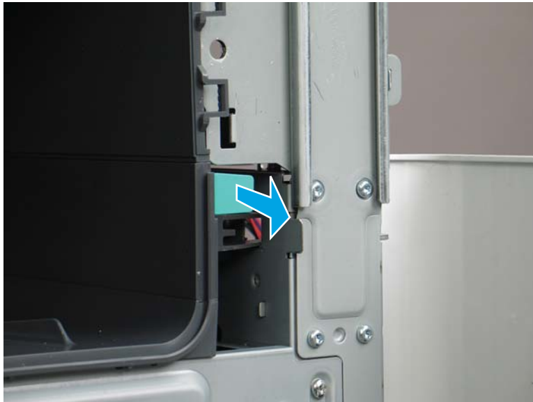
Figure 1-1370 Release the cover
