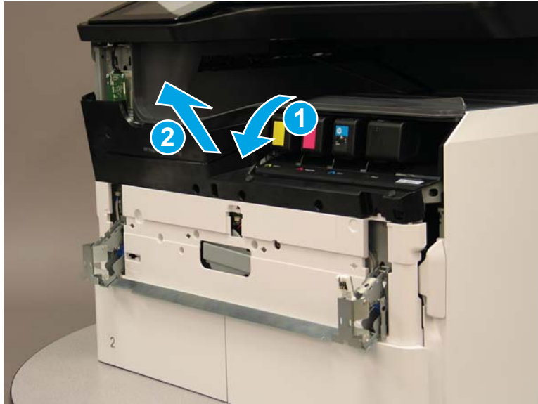
Figure 1-596 Release the cover
