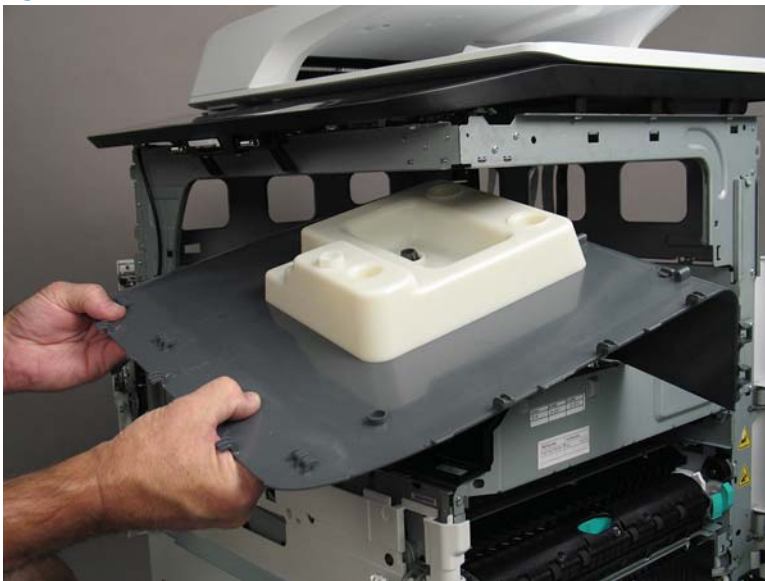
Figure 1-1117 Remove the cover
