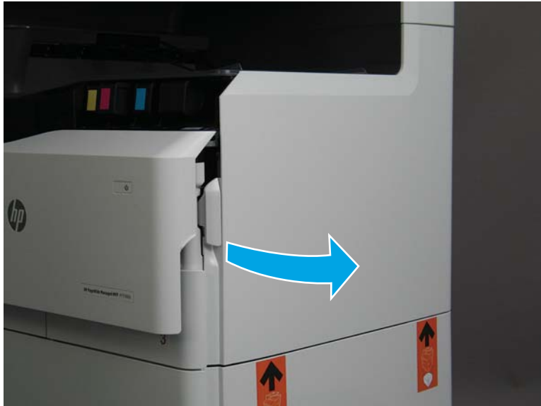
Figure 1-303 Open the right door
