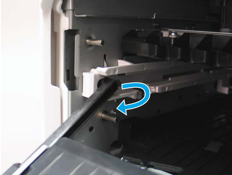
Figure 1-868 Release the left-side boss
