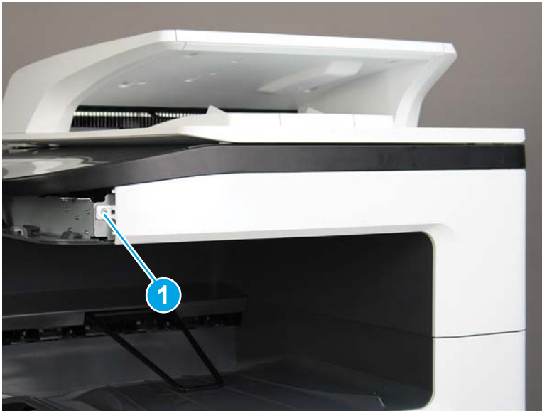
Figure 1-305 Remove one screw
