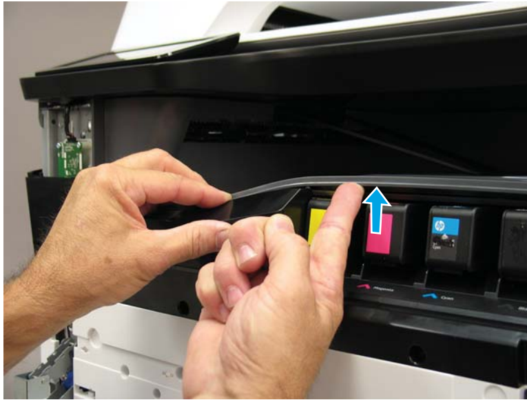
Figure 1-1159 Release one tab
