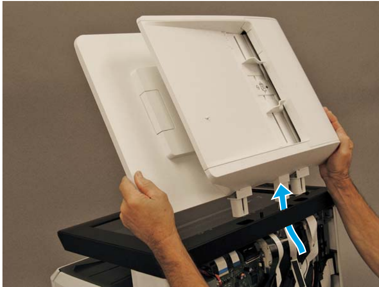
Figure 1-398 Remove the document feeder
