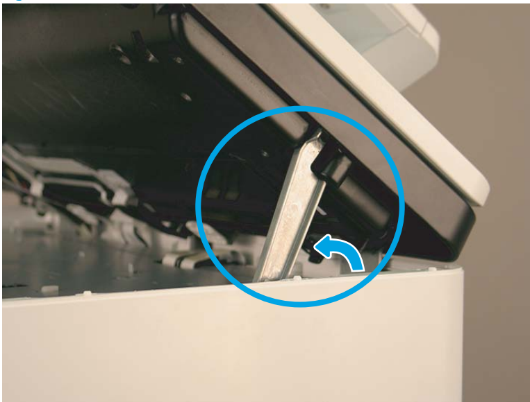
Figure 1-1203 Secure the ISA
