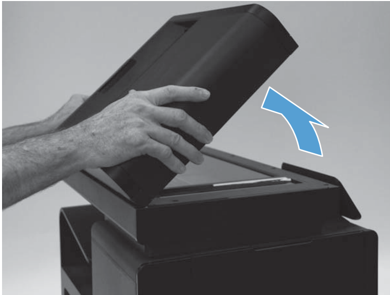
Figure 1-70 Remove the document feeder (1 of 5)
