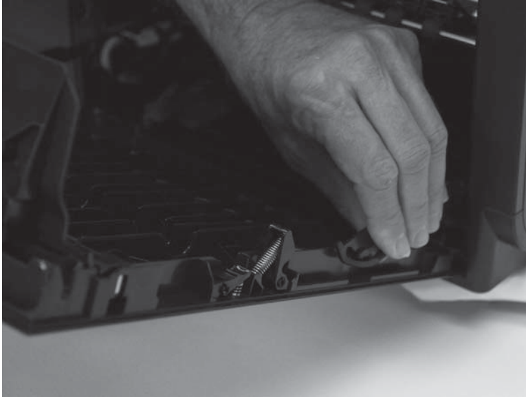
Figure 1-27 Remove the left door (3 of 6)
