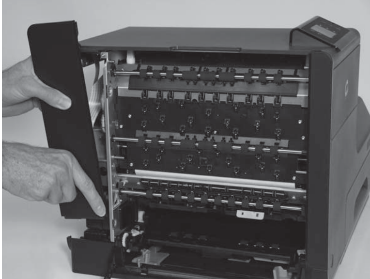
Figure 1-32 Remove the left rear cover (2 of 2)
