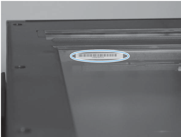
Figure 1-86 Calibrate the scanner (scanner barcode location)
