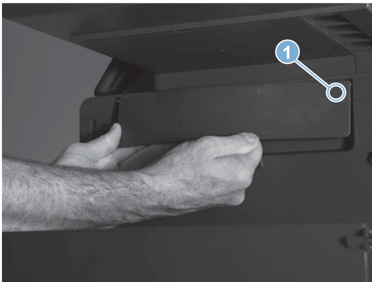
Figure 1-17 Remove the output bin flap
