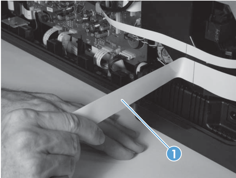
Figure 1-51 Remove the aerosol fan (3 of 12)
