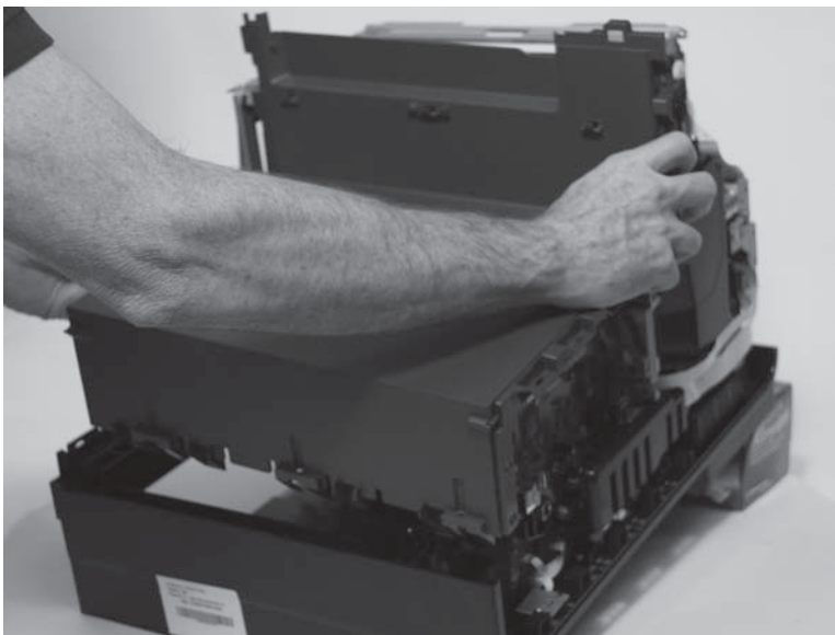
Figure 1-48 Remove the right cover (2 of 2)
