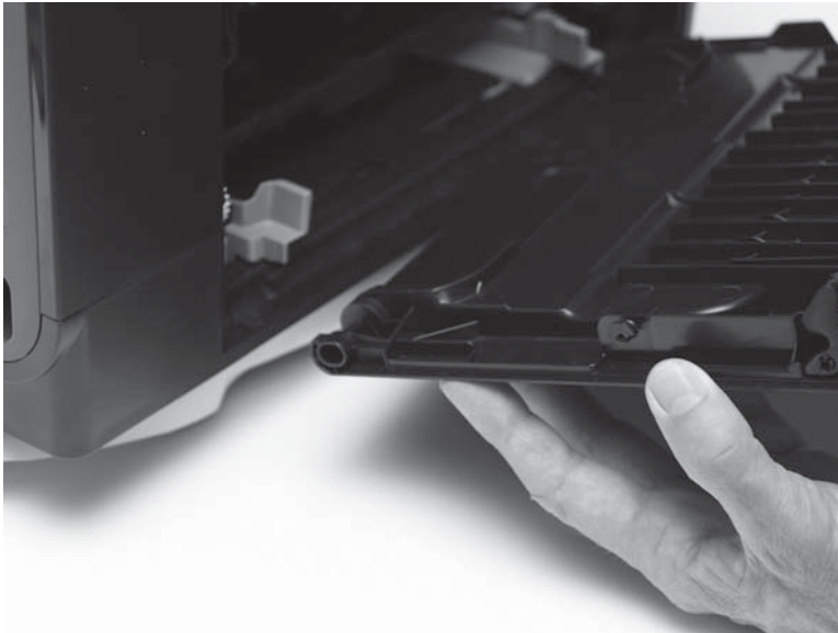
Figure 1-30 Remove the left door (6 of 6)
