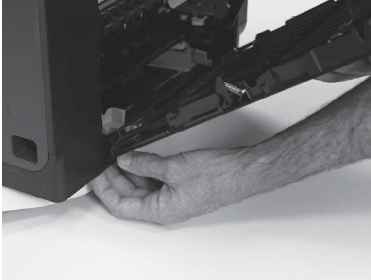
Figure 1-28 Remove the left door (4 of 6)
