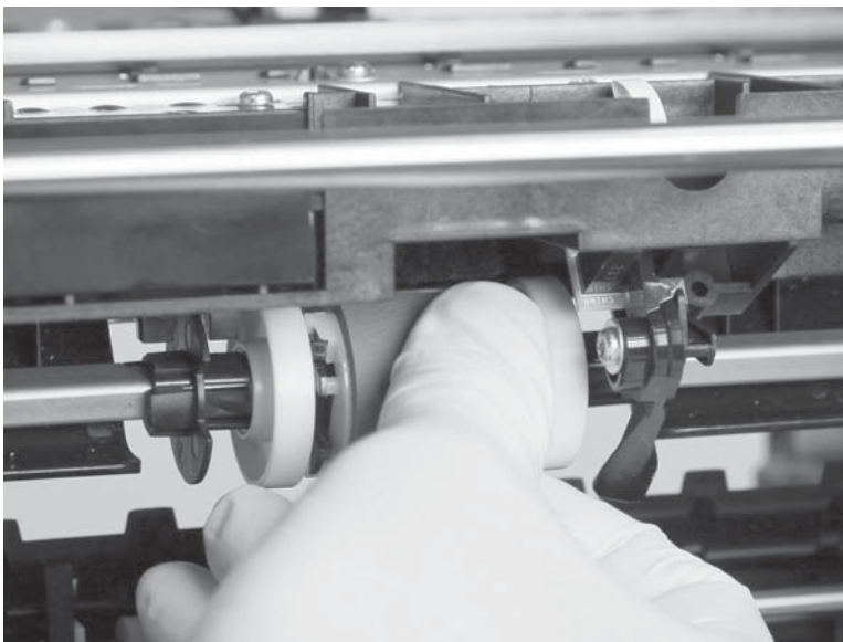
Figure 1-66 Reinstall the separator/pick assembly (2 of 5)
