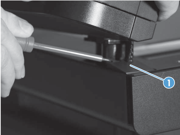
Figure 1-72 Remove the document feeder (3 of 5)
