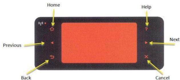
Figure 1-18 X476/X576 control panel button locations
