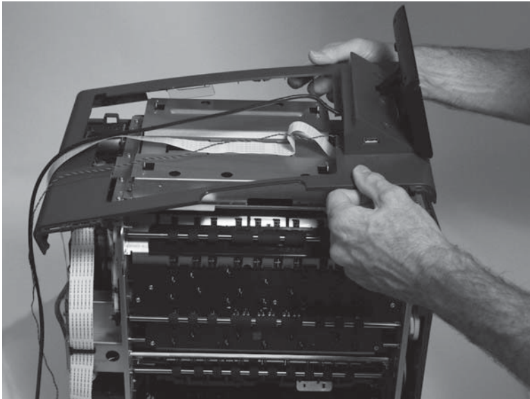
Figure 1-41 Remove the top cover and control panel (7 of 7)
