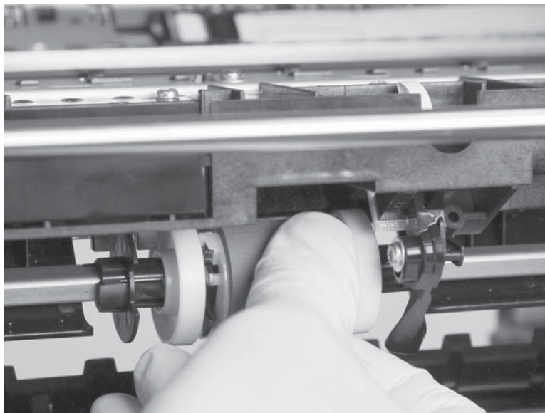
Figure 1-67 Reinstall the separator/pick assembly (4 of 5)
