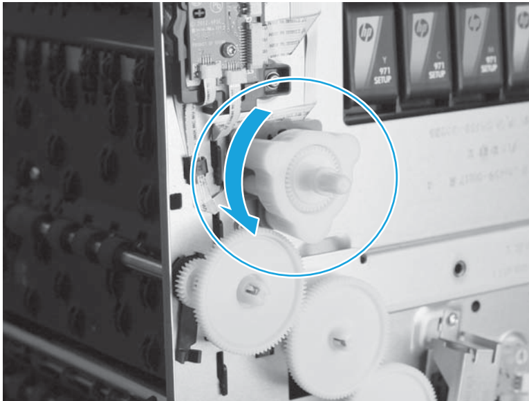
Figure 1-83 Remove the service sled assembly (2 of 6)
