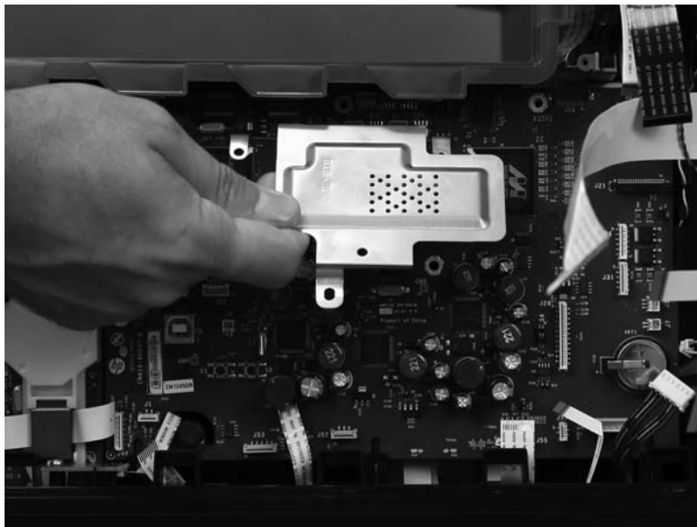
Figure 1-196 Remove the main PCA (6 of 8)
