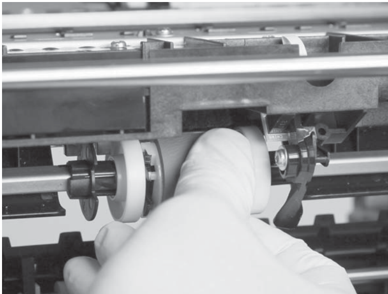
Figure 1-65 Reinstall the separator/pick assembly (2 of 5)
