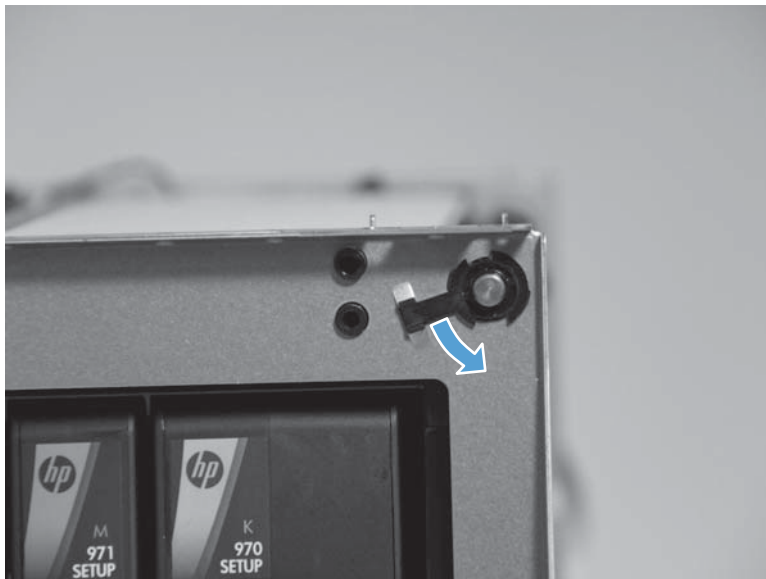
Figure 1-130 Remove the output drive shaft 6 (2 of 3)
