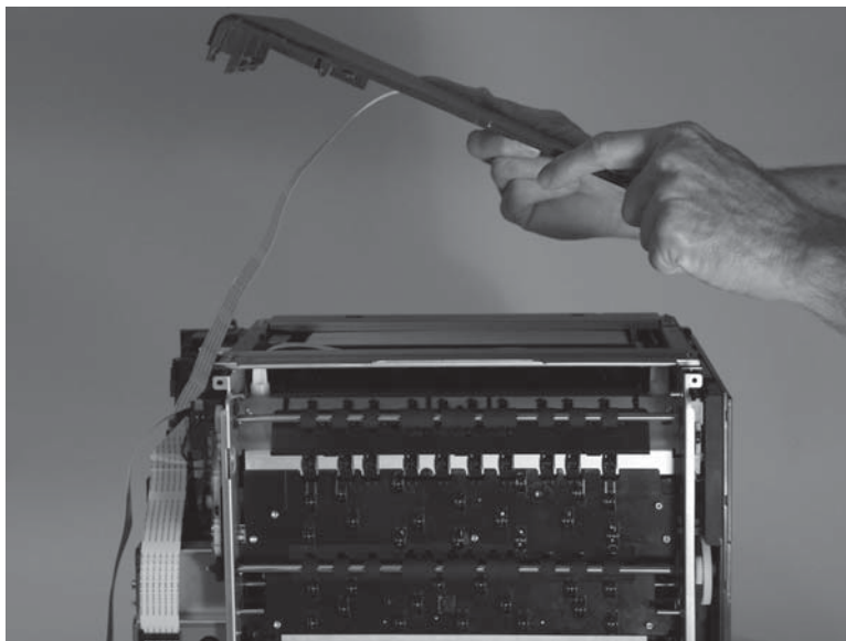
Figure 1-43 Remove the top cover (8 of 8)
