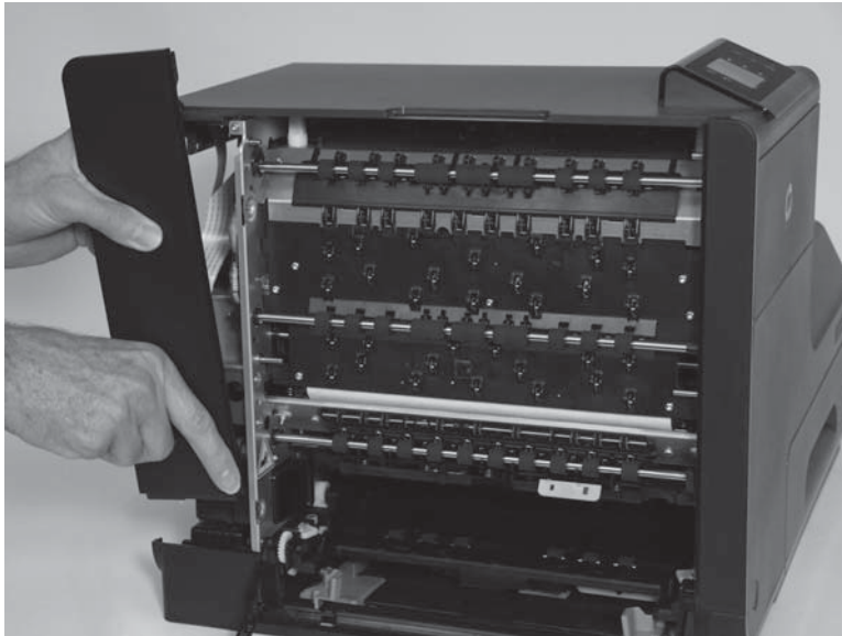
Figure 1-33 Remove the left rear cover (2 of 2)
