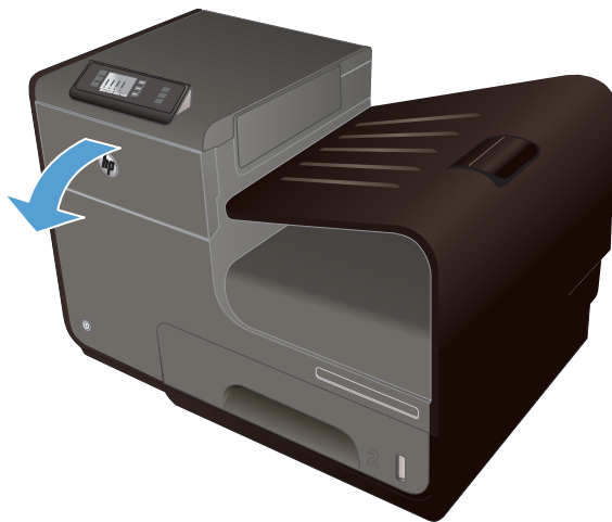
Figure 1-7 Replace the ink cartridges (1 of 7)
