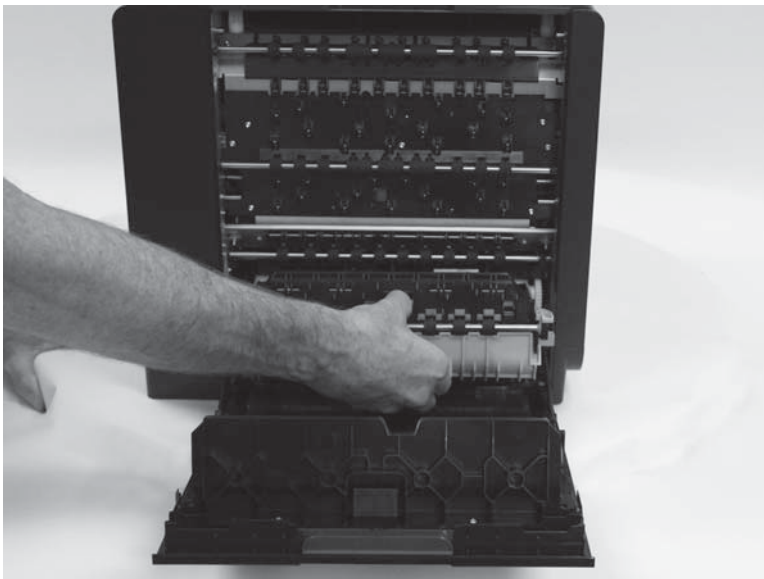
Figure 1-15 Remove the duplex module (2 of 2)
