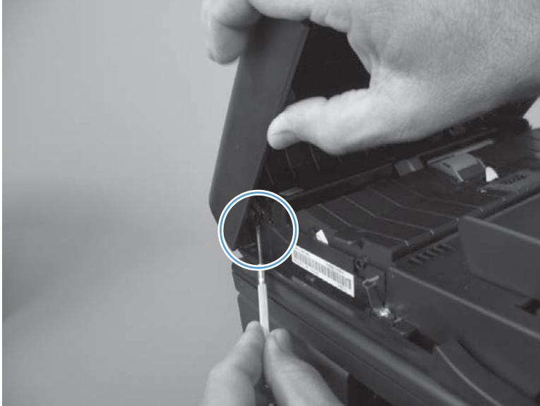
Figure 1-8 Remove the ADF pre-pickup arm and pickup roller assembly (2 of 4)
