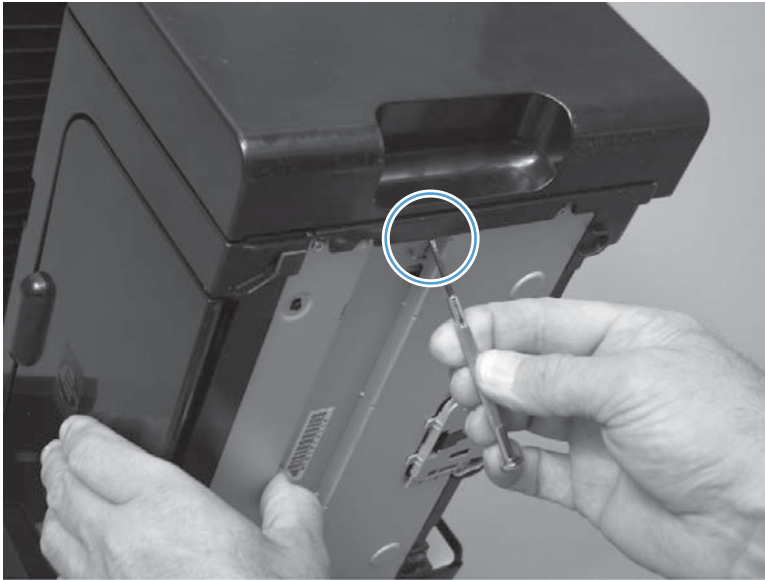
Figure 1-35 Remove the right cover (3 of 5)
