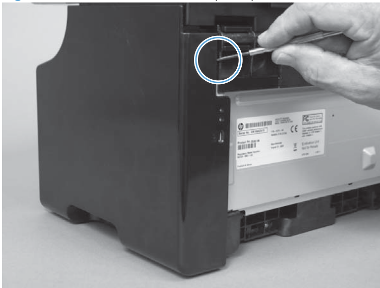
Figure 1-34 Remove the left cover (2 of 5)
