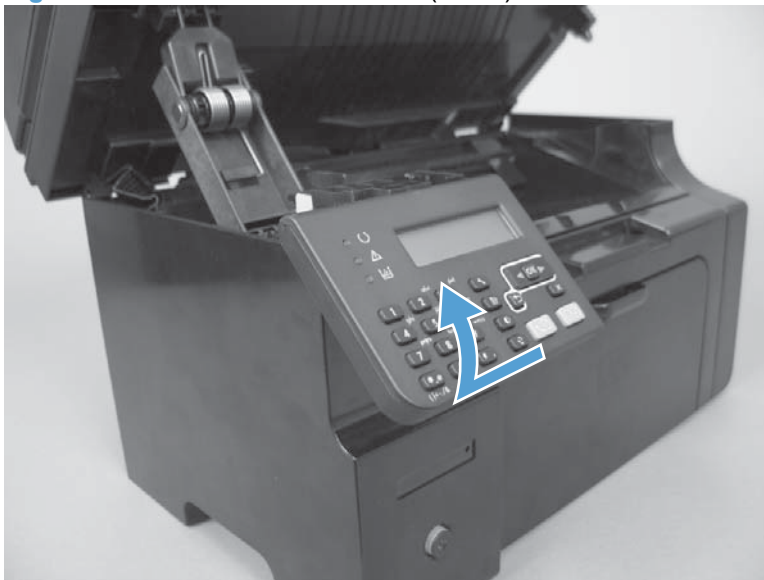
Figure 1-30 Remove the left cover (4 of 6)
