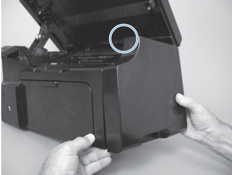
Figure 1-37 Remove the right cover (5 of 5)
