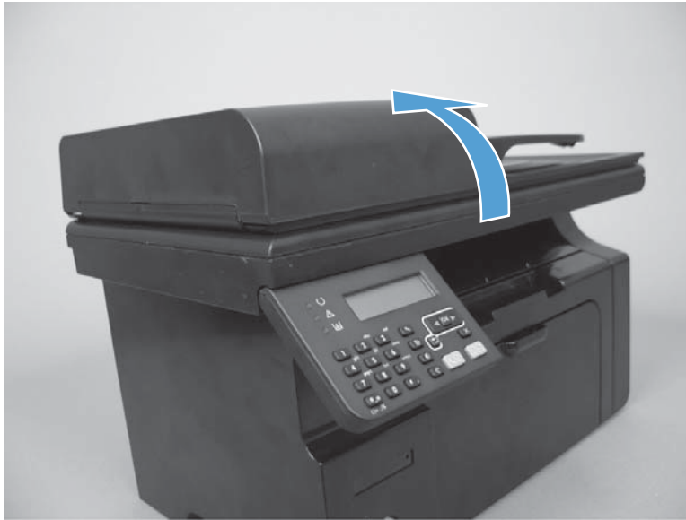
Figure 1-29 Remove the left cover (3 of 6)
