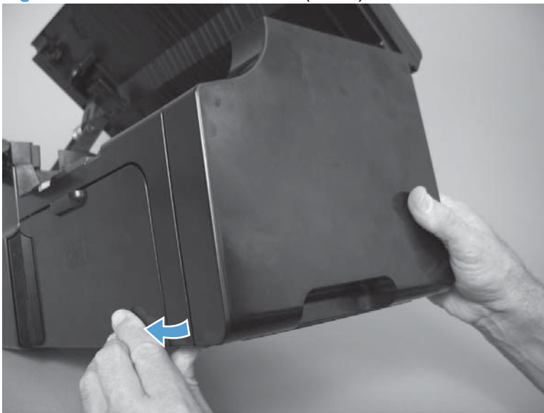
Figure 1-36 Remove the left cover (4 of 5)
