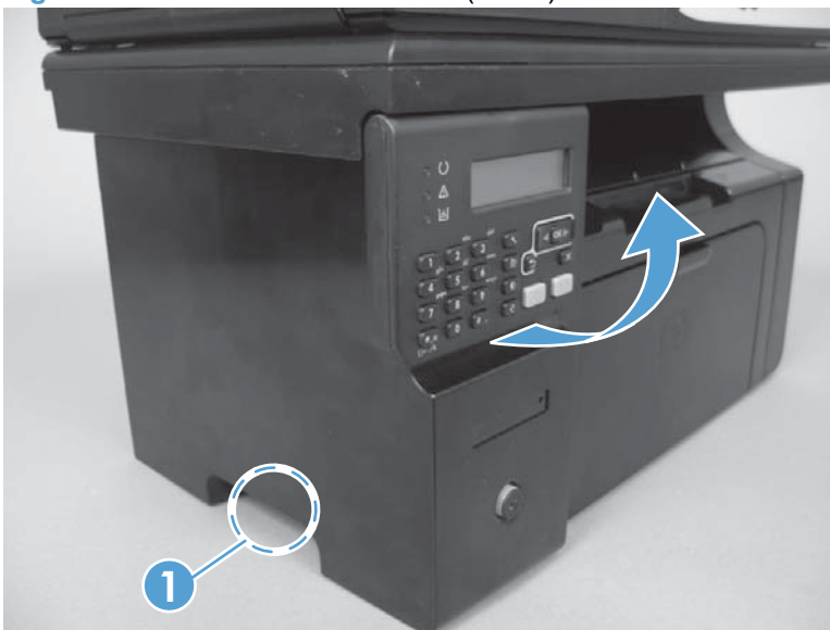
Figure 1-28 Remove the left cover (2 of 6)
