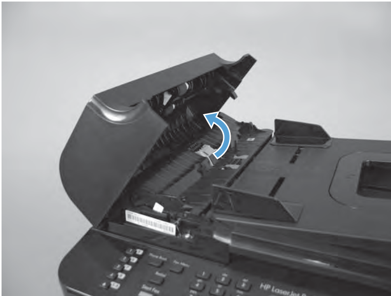
Figure 1-121 Remove the document feeder cover (1 of 3)
