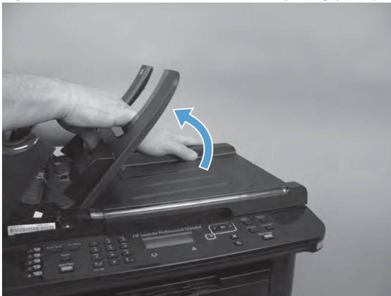
Figure 1-120 Remove the document feeder input tray (2 of 2)
