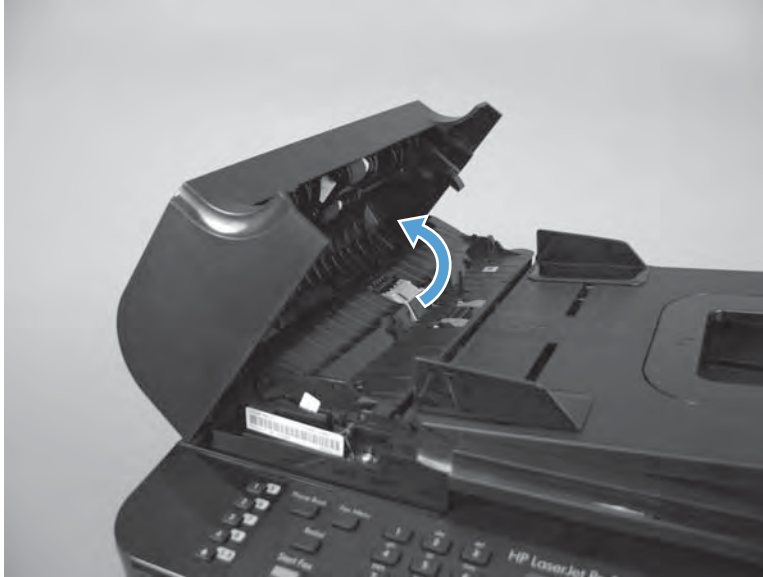
Figure 1-119 Remove the document feeder input tray (1 of 2)
