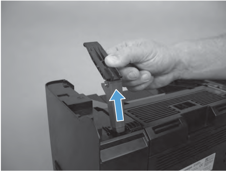
Figure 1-23 Remove the scanner hinges (2 of 2)
