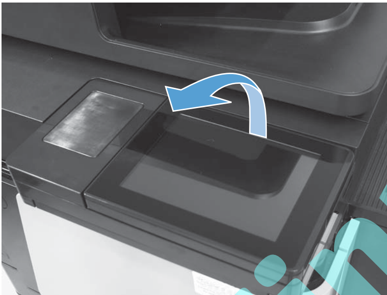
Figure 1-74 Remove the control-panel assembly (M830; 1 of 7)
