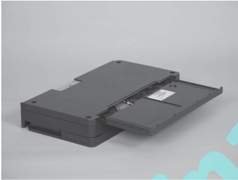
Figure 1-65 Remove the keyboard assembly (M830; 6 of 7)
