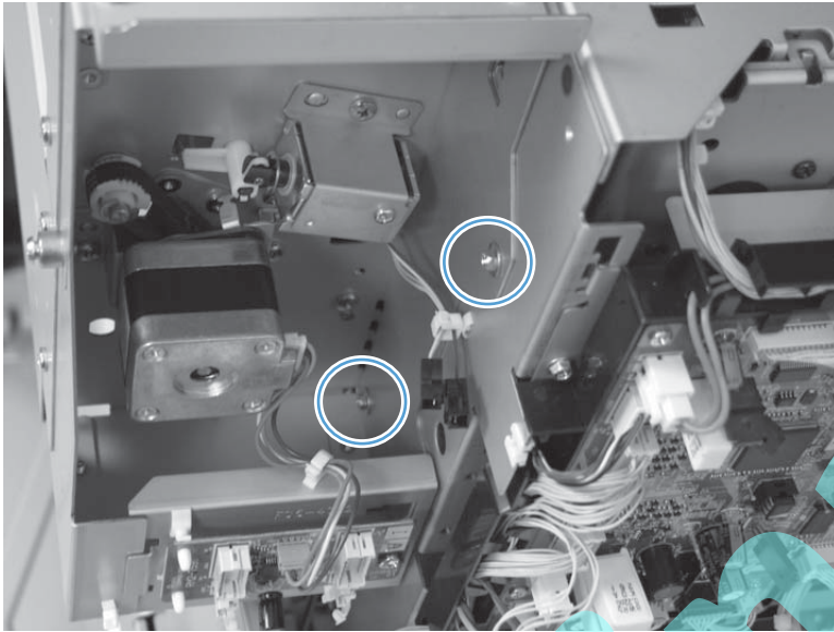
Figure 1-712 Remove the paper pass assembly (4 of 7)
