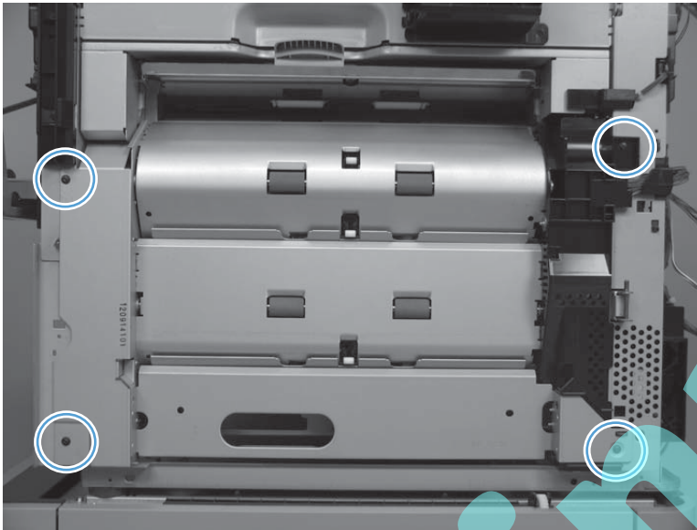
Figure 1-255 Remove the paper-pickup assembly (6 of 7)
