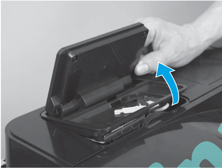
Figure 1-53 Remove the control-panel assembly (M806; 5 of 10)
