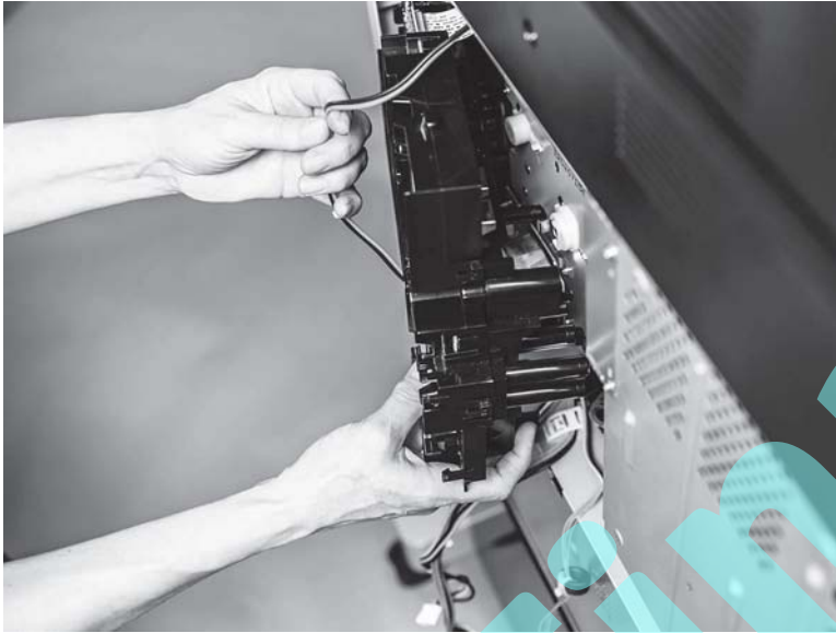
Figure 1-284 Reinstall the high-voltage power supply (M830; 1 of 2)
