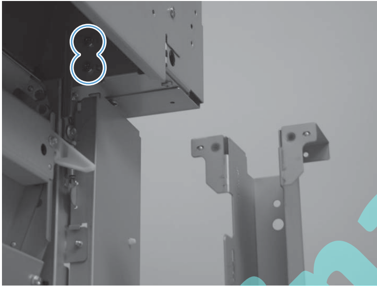
Figure 1-714 Remove the paper pass assembly (6 of 7)
