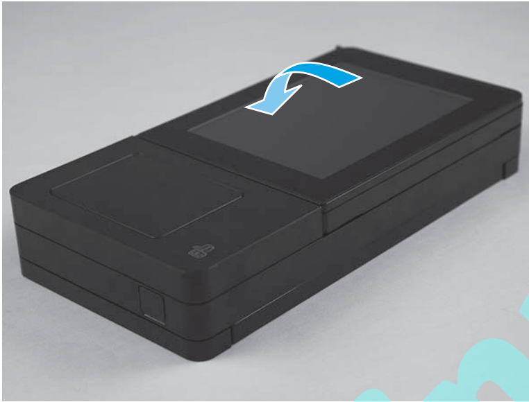
Figure 1-63 Remove the keyboard assembly (M830; 4 of 7)
