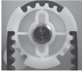
Figure 1-655 Reinstall the operation tray assembly (5 of 5)
