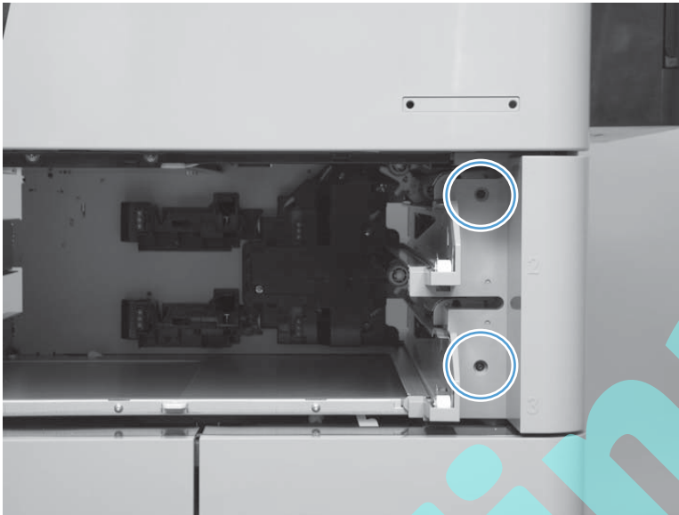
Figure 1-192 Remove the right lower front cover (1 of 3).
