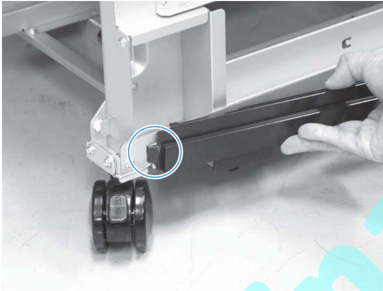
Figure 1-431 Remove the HCI lower right cover (3 of 3)
