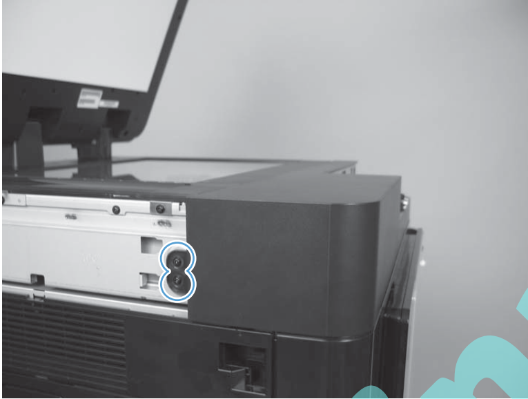
Figure 1-121 Remove the scanner front cover (M830; 4 of 7)
