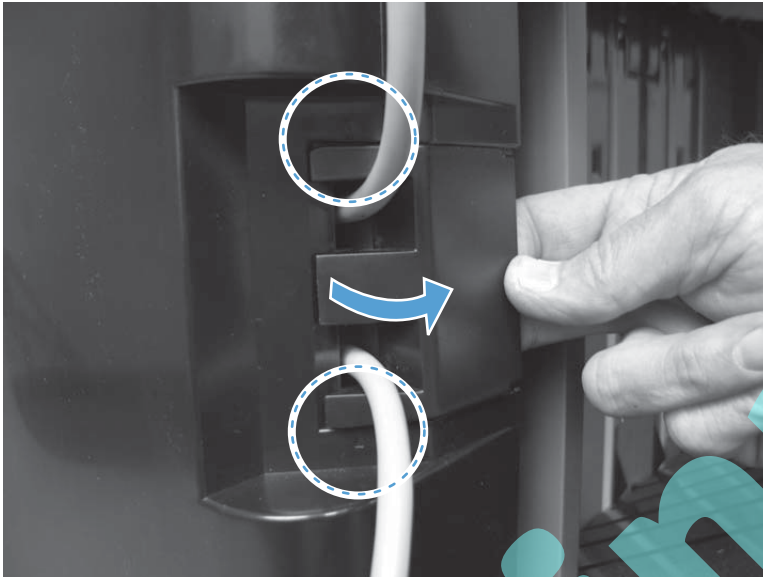
Figure 1-479 Remove the bin cable guide cover (3 of 6)
