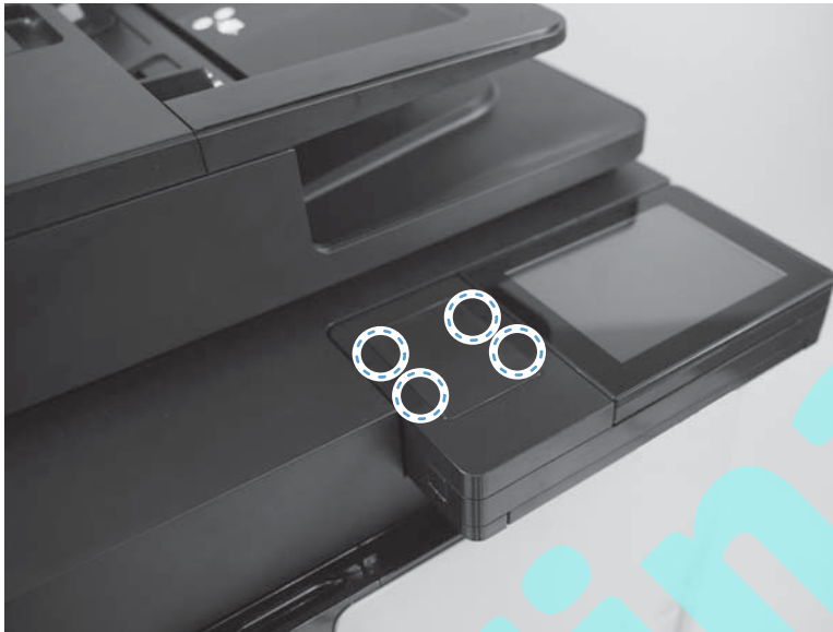
Figure 1-135 Remove the HIP cover (M830; 1 of 3)
