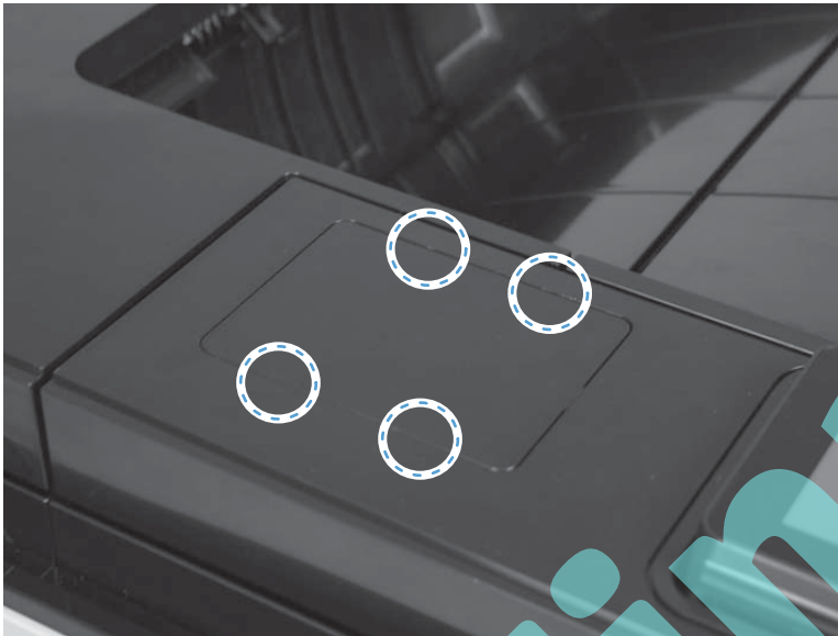
Figure 1-130 Remove the HIP cover (M806; 1 of 3)
