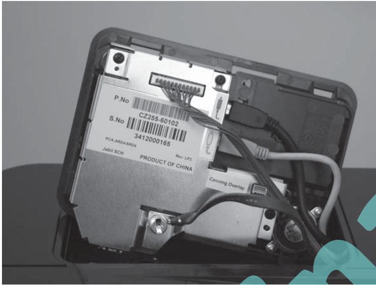
Figure 1-55 Remove the control-panel assembly (M806; 7 of 10)
