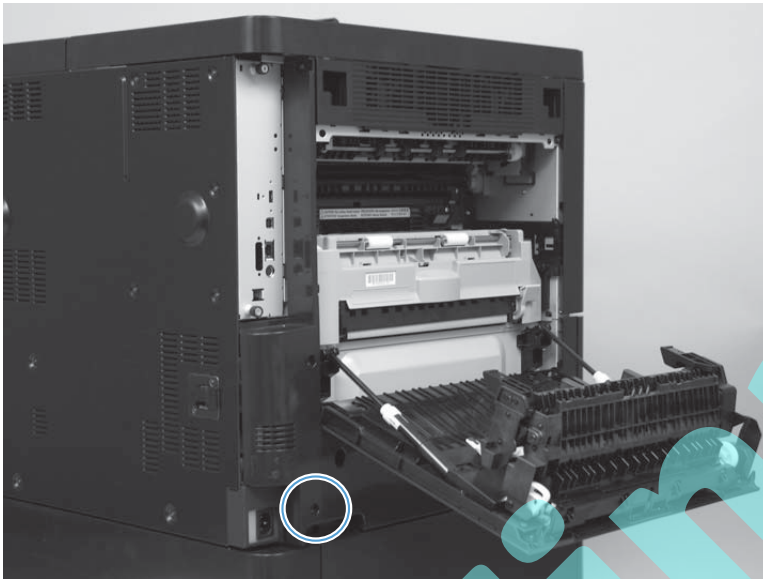
Figure 1-165 Remove the rear cover (1 of 3)
