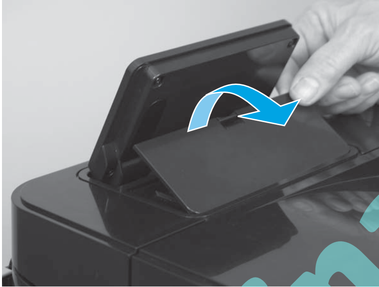
Figure 1-51 Remove the control-panel assembly (M806; 3 of 10)
