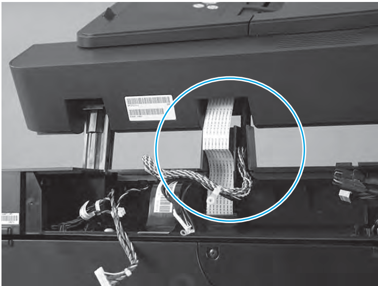
Figure 1-305 Route the document feeder FFC and cables
