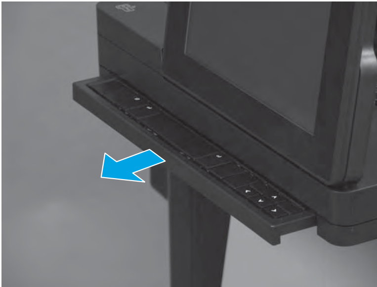
Figure 1-117 Slide the keyboard out
