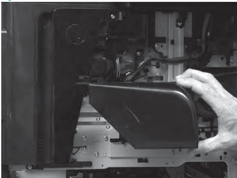
Figure 1-719 Remove the fan duct
