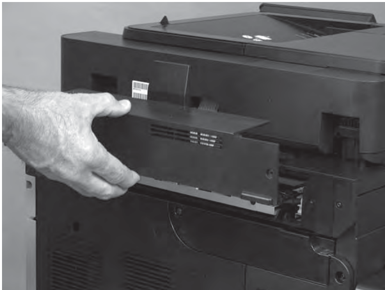
Figure 1-337 Remove the cover
