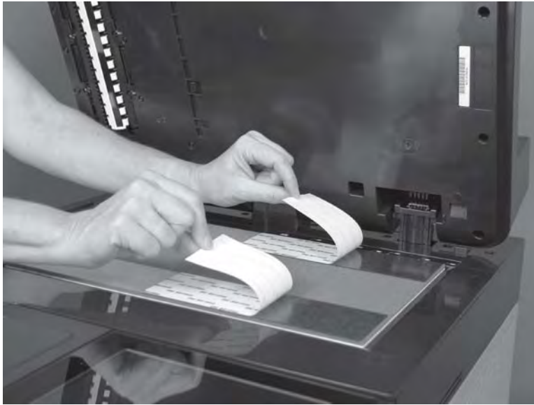
Figure 1-406 Peel off the adhesive backing
