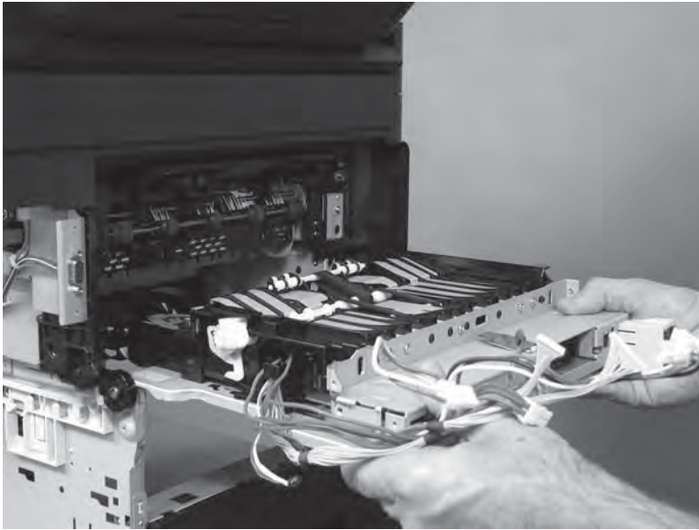
Figure 1-865 Remove the HVPS
