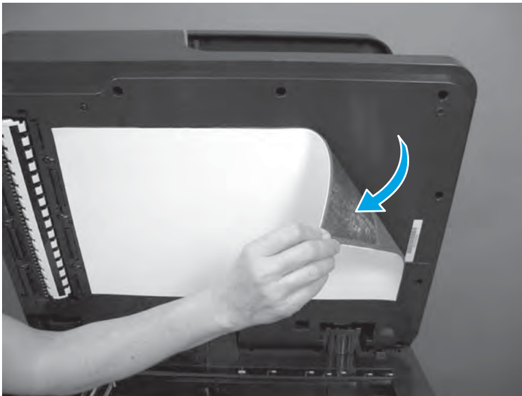
Figure 1-401 Remove the white backing
