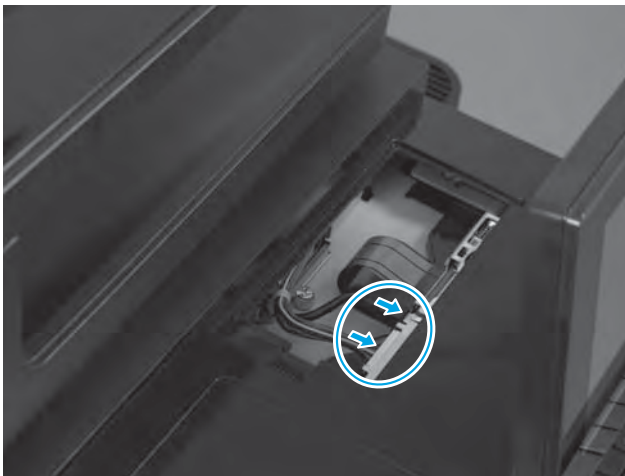
Figure 1-171 Connect two connectors
