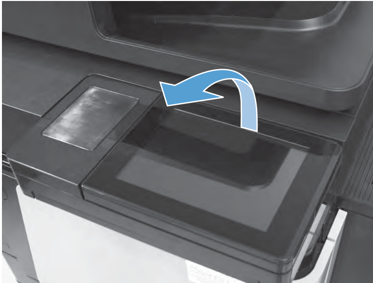
Figure 1-146 Tilt the control panel up
