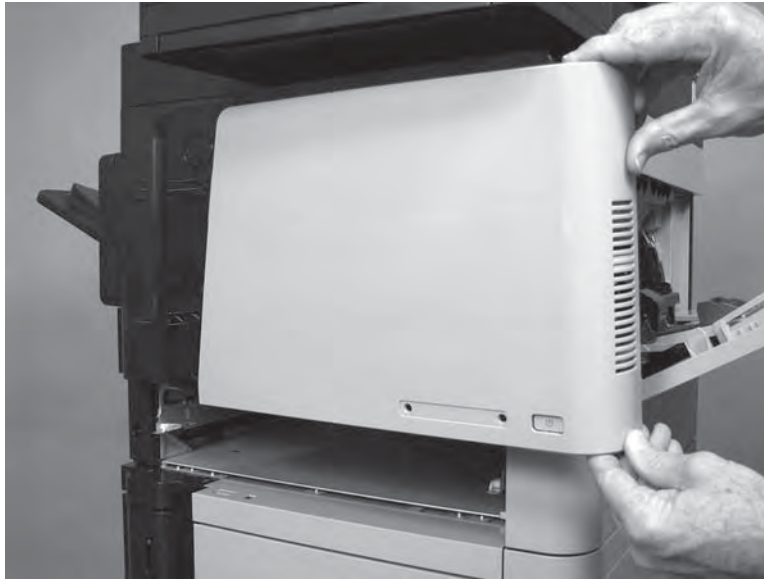
Figure 1-477 Remove the cover
