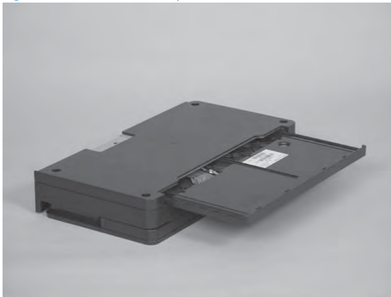
Figure 1-158 Turn the control panel face-down
