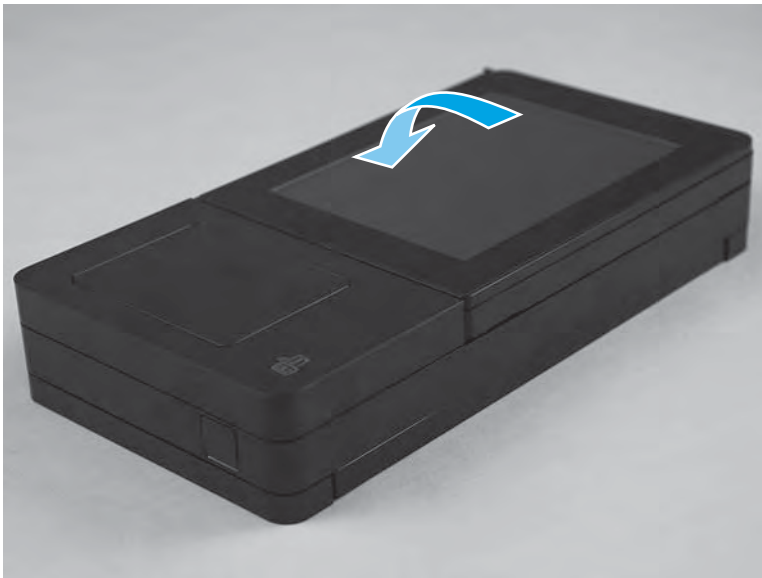
Figure 1-156 Tilt the screen down
