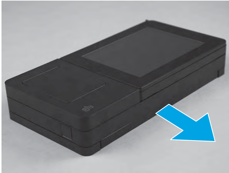
Figure 1-157 Slide the keyboard tray out
