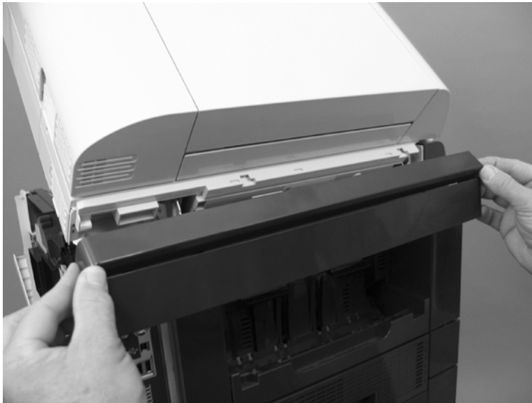
Figure 1-542 Remove the document feeder hinge cover
