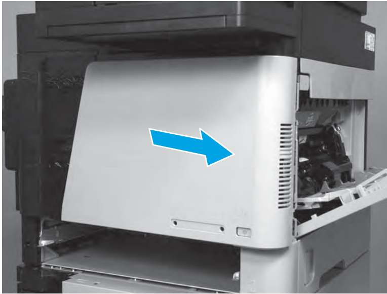
Figure 1-823 Slide the cover to the right
