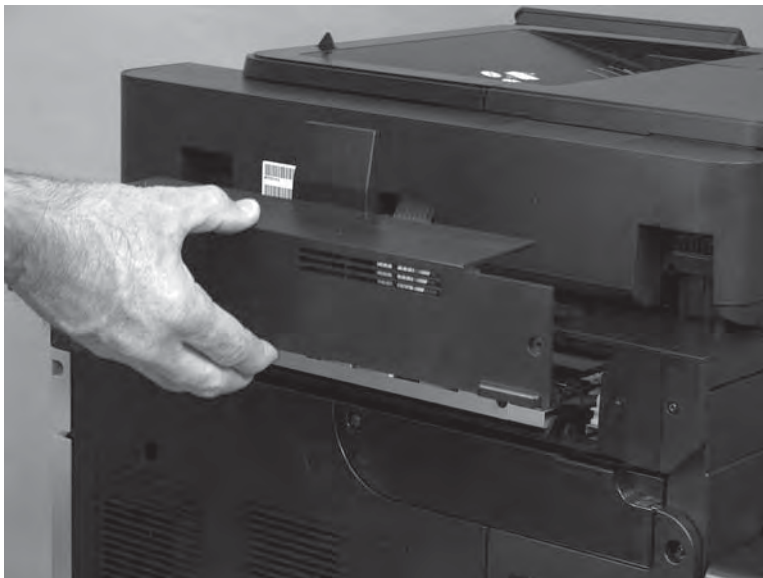
Figure 1-283 Install the cover
