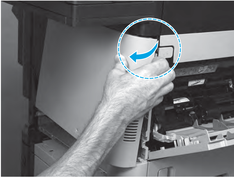
Figure 1-475 Release the right-upper corner
