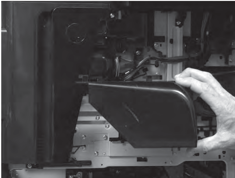
Figure 1-856 Remove the fan duct
