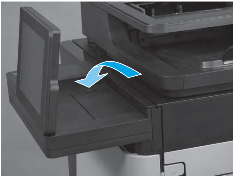
Figure 1-143 Install the cover
