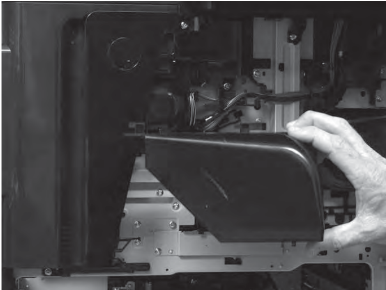
Figure 1-704 Remove the fan duct
