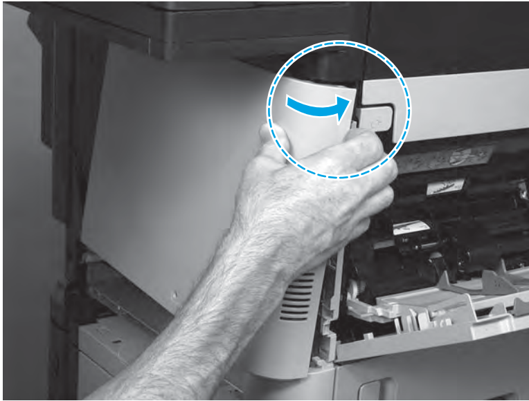
Figure 1-918 Engage one locking pin
