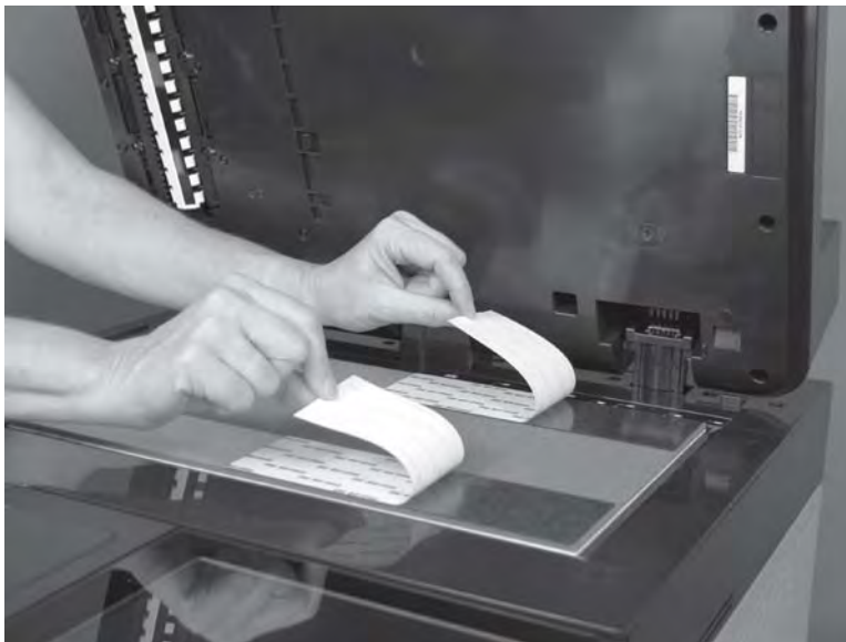
Figure 1-225 Peel off the adhesive backing
