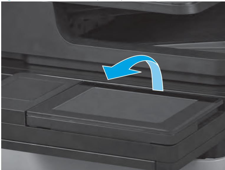
Figure 1-115 Tilt the control panel up
