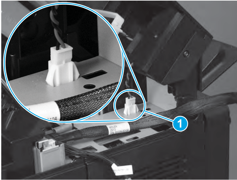
Figure 1-379 Connect one connector
