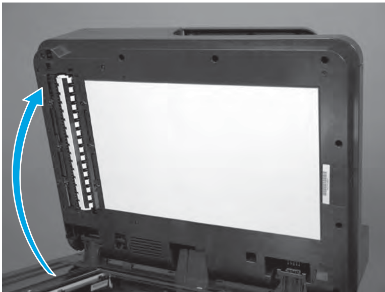
Figure 1-219 Open the document feeder
