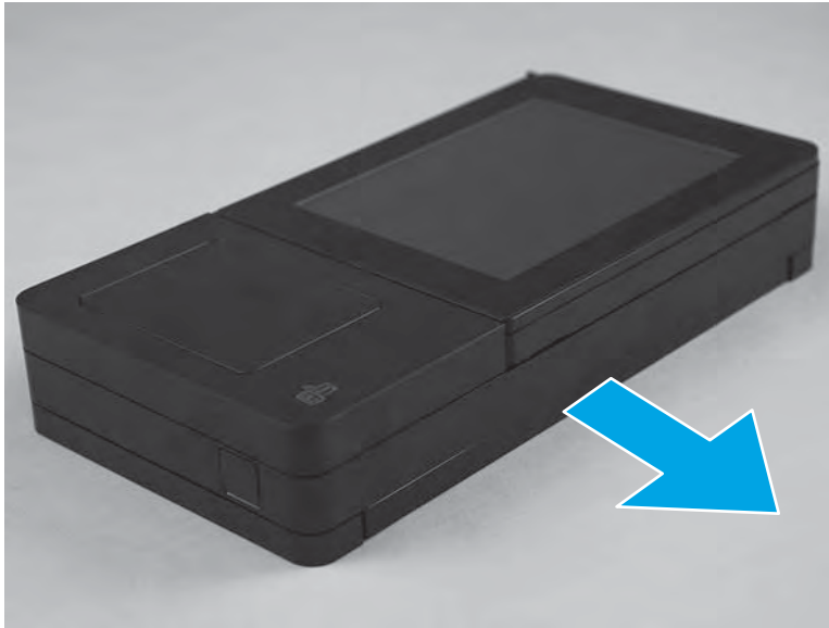
Figure 1-126 Slide the keyboard tray out
