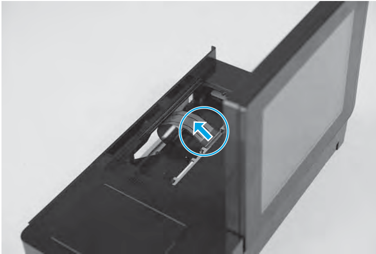
Figure 1-155 Disconnect the flat cable
