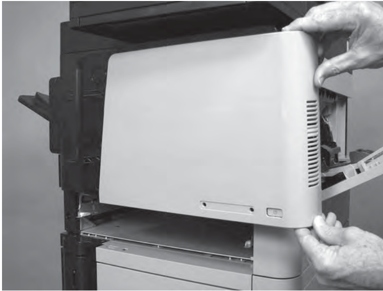
Figure 1-418 Remove the cover
