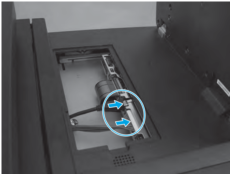
Figure 1-141 Connect two connectors
