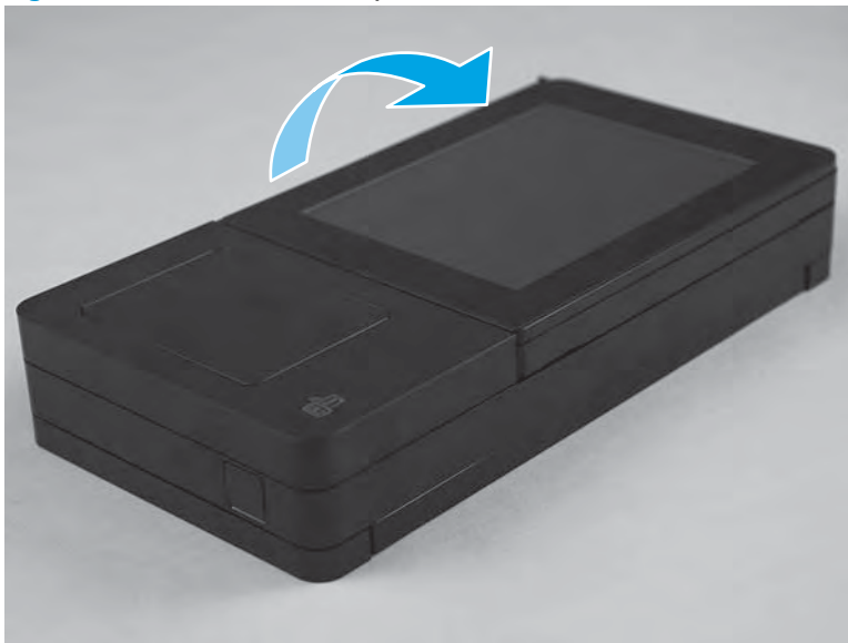
Figure 1-133 Tilt the screen up
