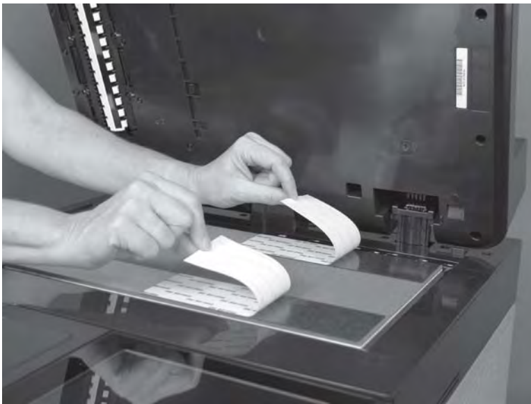
Figure 1-328 Peel off the adhesive backing
