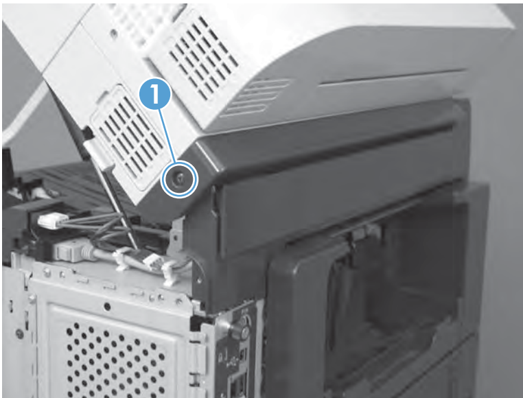
Figure 1-540 Remove one screw
