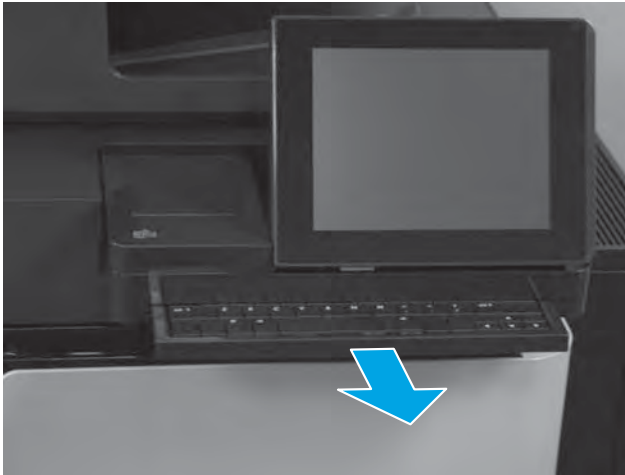
Figure 1-170 Slide the keyboard out
