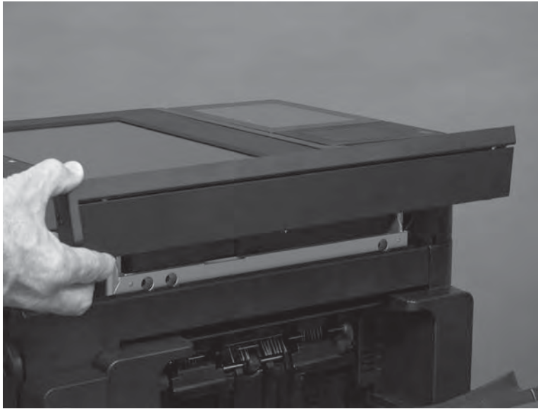
Figure 1-364 Remove the cover
