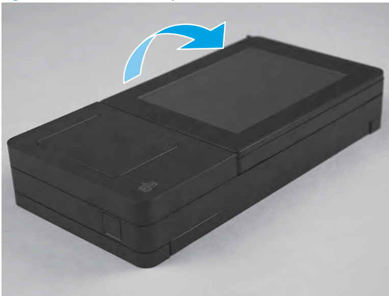
Figure 1-163 Tilt the screen up
