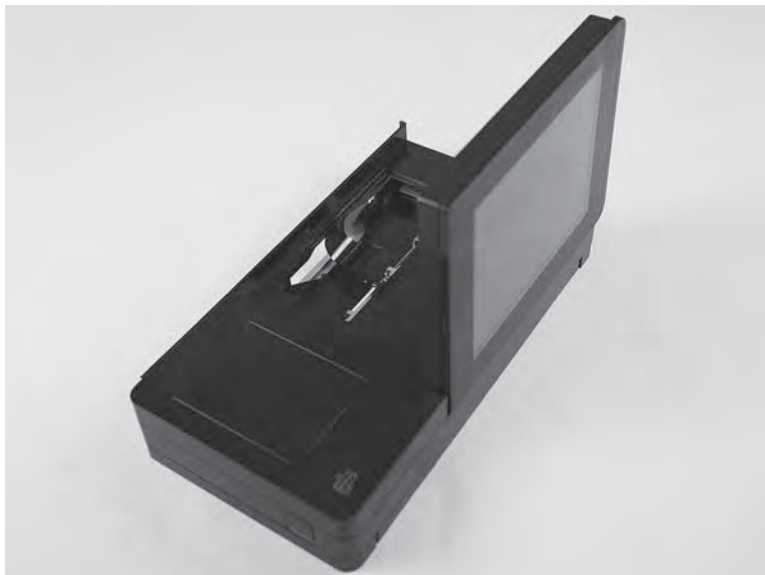
Figure 1-153 Place the control-panel assembly on a flat surface
