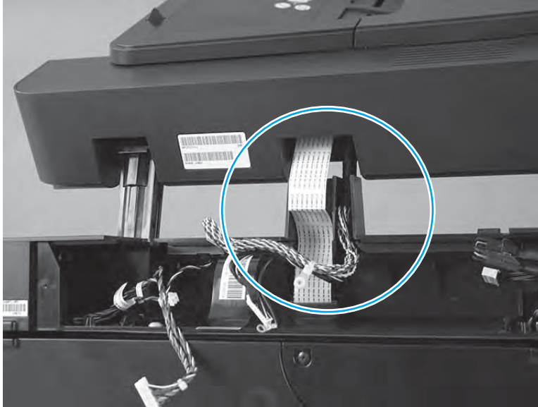
Figure 1-383 Route the document feeder FFC and cables
