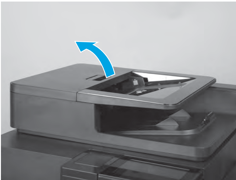
Figure 1-16 Open the document-feeder door
