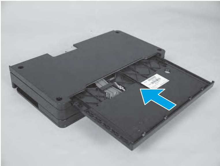
Figure 1-131 Slide the keyboard tray in
