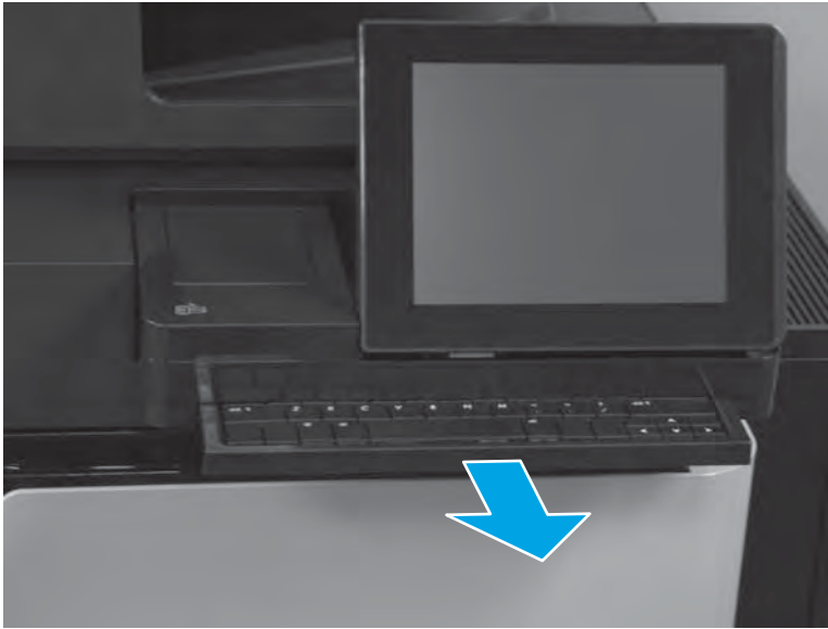
Figure 1-148 Slide the keyboard out
