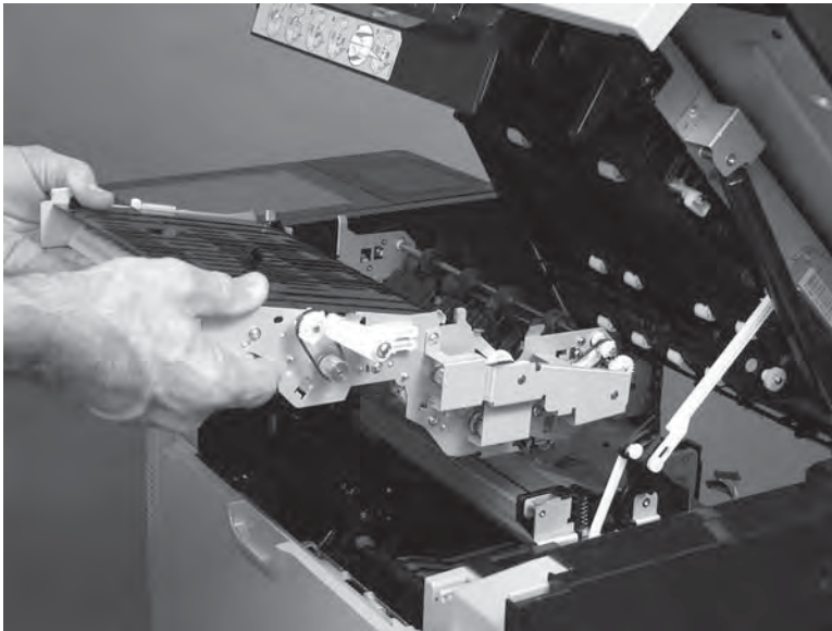
Figure 1-563 Remove the reverse assembly
