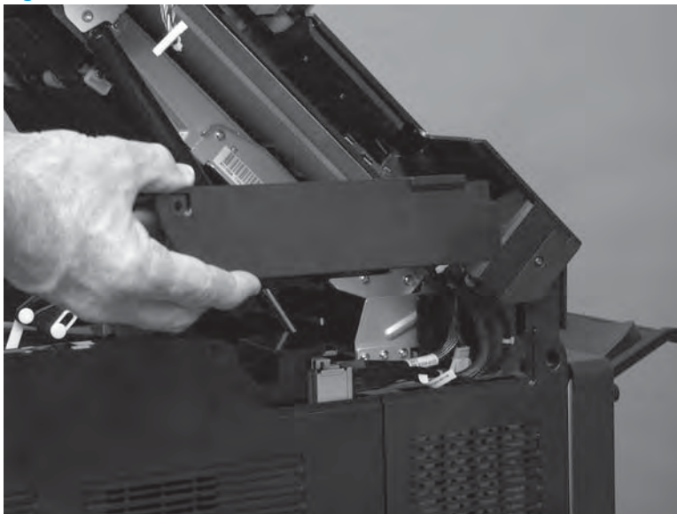
Figure 1-357 Remove the scanner cable cover
