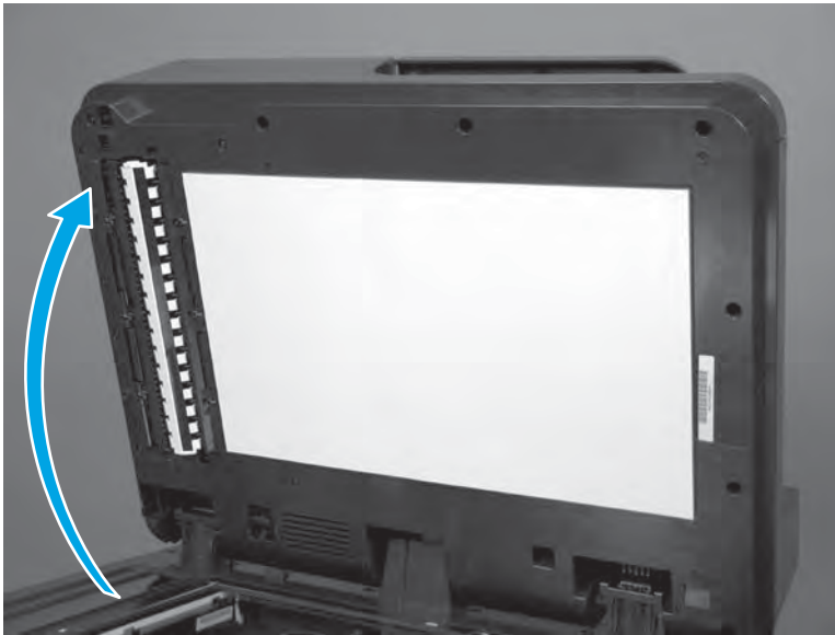
Figure 1-400 Open the document feeder
