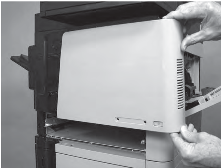
Figure 1-824 Remove the cover
