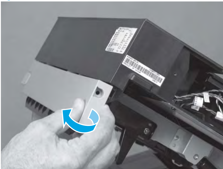
Figure 1-355 Release one tab
