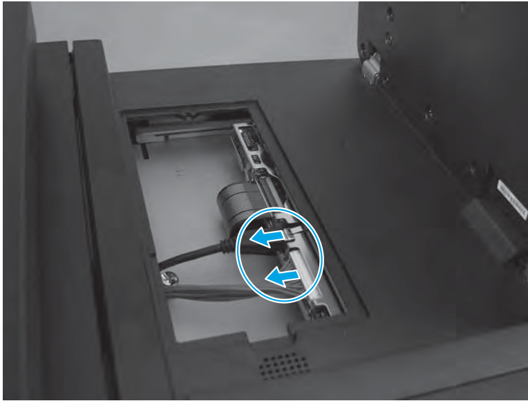
Figure 1-118 Disconnect two connectors
