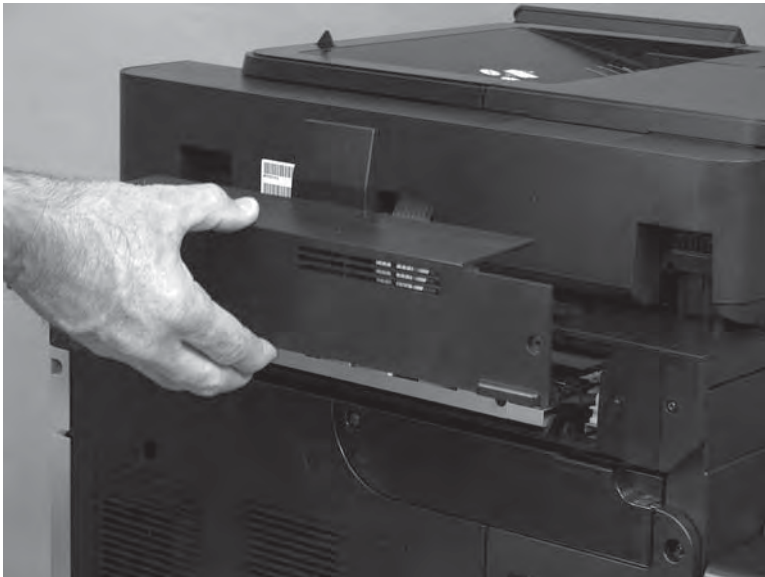
Figure 1-290 Remove the cover
