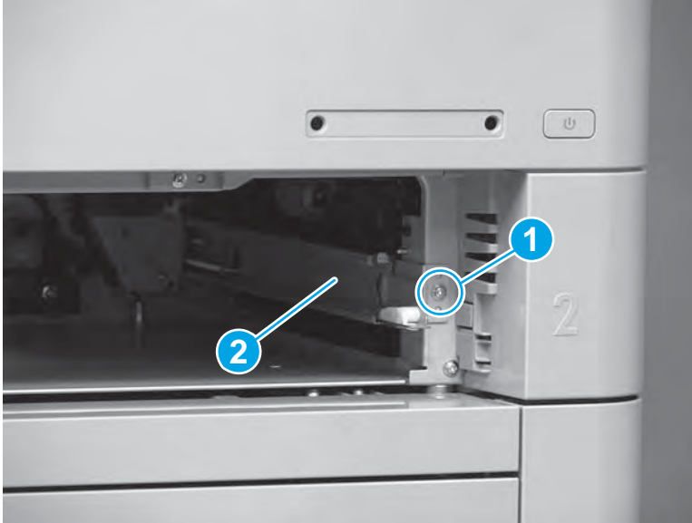
Figure 1-1014 Remove one screw and the cassette rail
