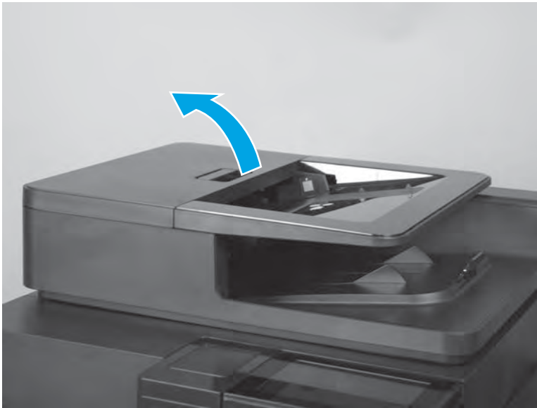
Figure 1-285 Open the document-feeder door
