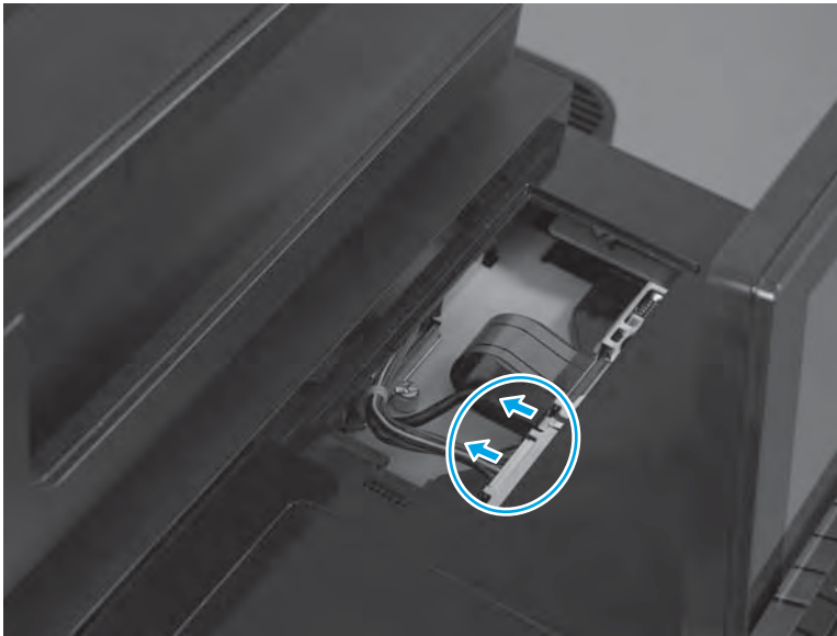
Figure 1-149 Disconnect two connectors
