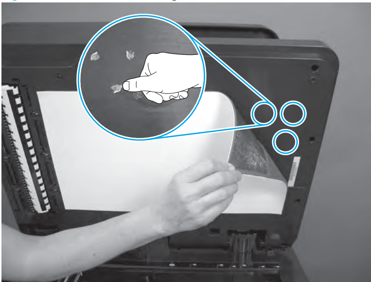
Figure 1-221 Remove remaining adhesive
