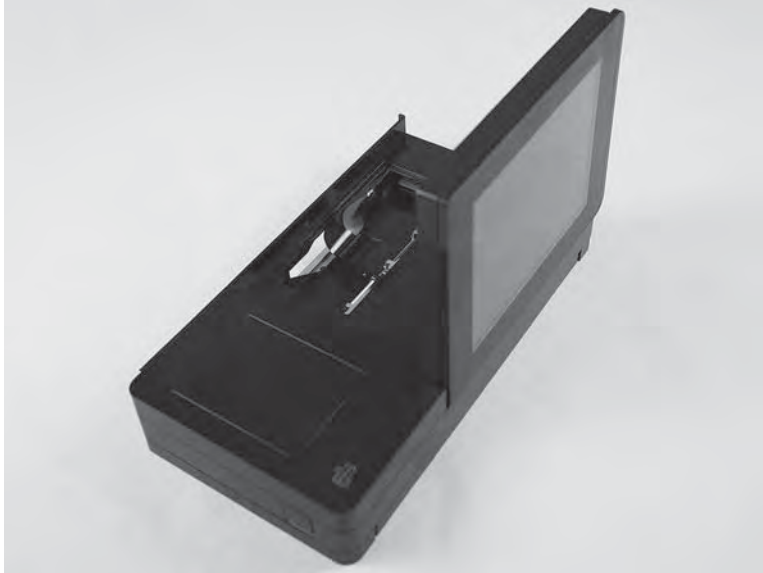
Figure 1-122 Place the control-panel assembly on a flat surface
