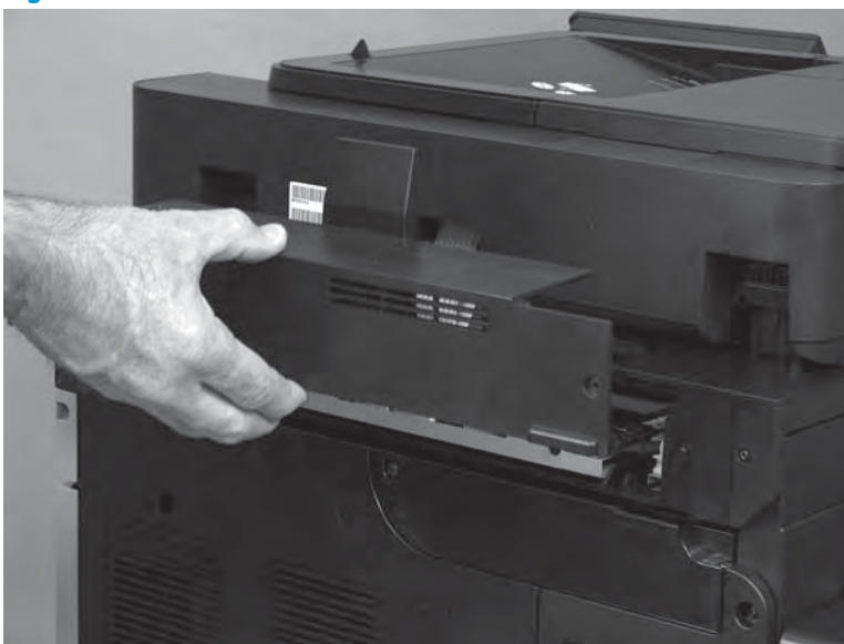
Figure 1-398 Install the cover
