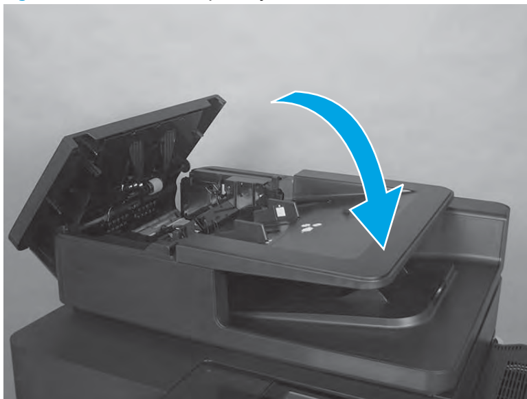
Figure 1-323 Rotate the input tray down
