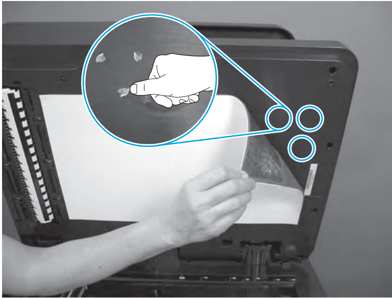
Figure 1-402 Remove remaining adhesive
