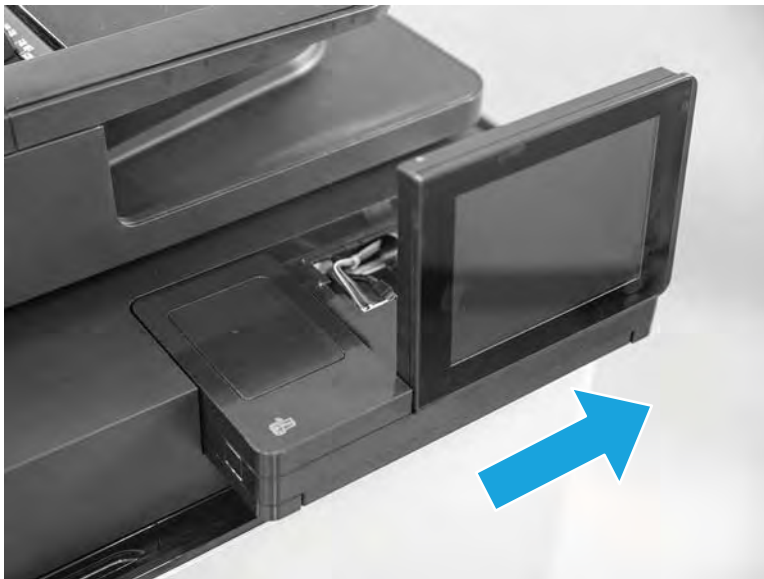
Figure 1-151 Slide the control panel to the right
