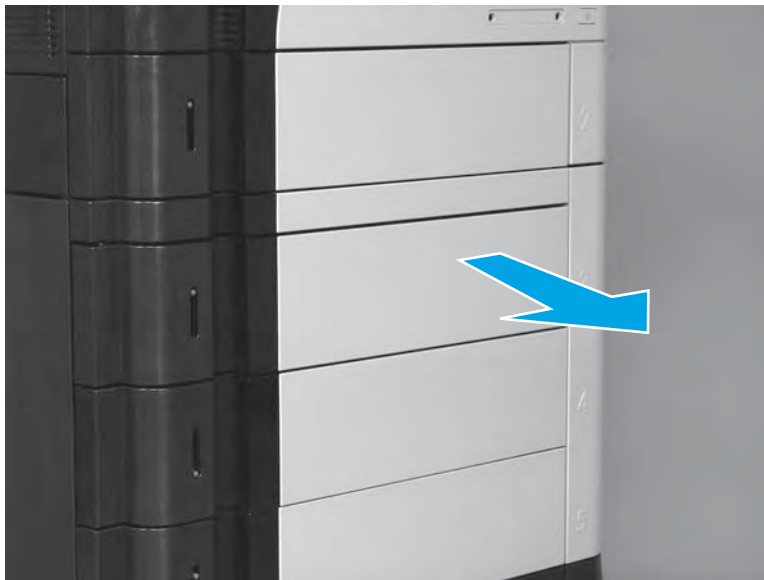
Figure 1-442 Open the tray
