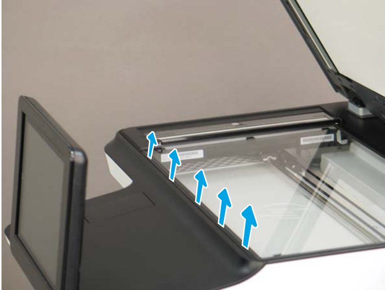
Figure 1-899 Release five tabs
