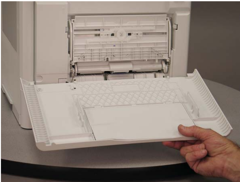
Figure 1-1874 Remove the MP cover
