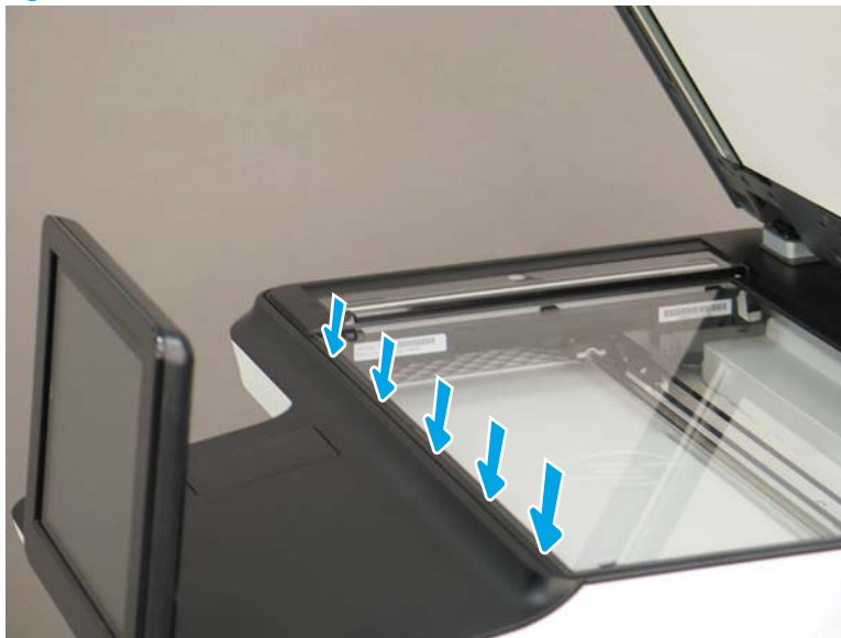
Figure 1-99 Install five tabs
