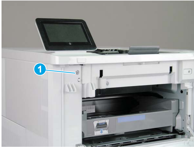
Figure 1-1838 Remove one screw
