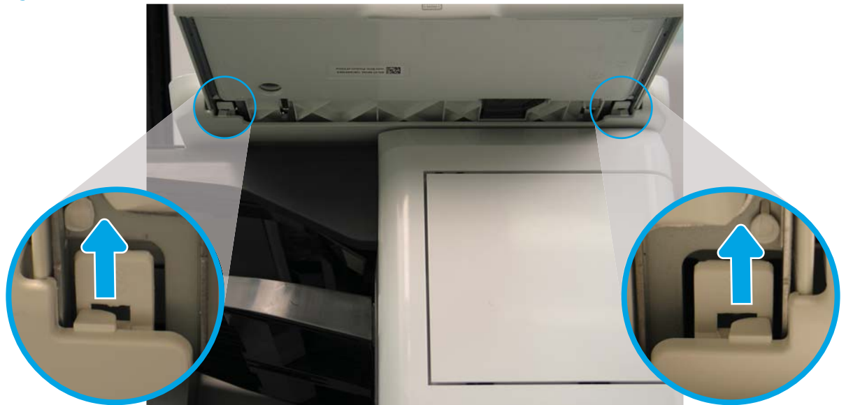
Figure 1-185 Release two tabs
