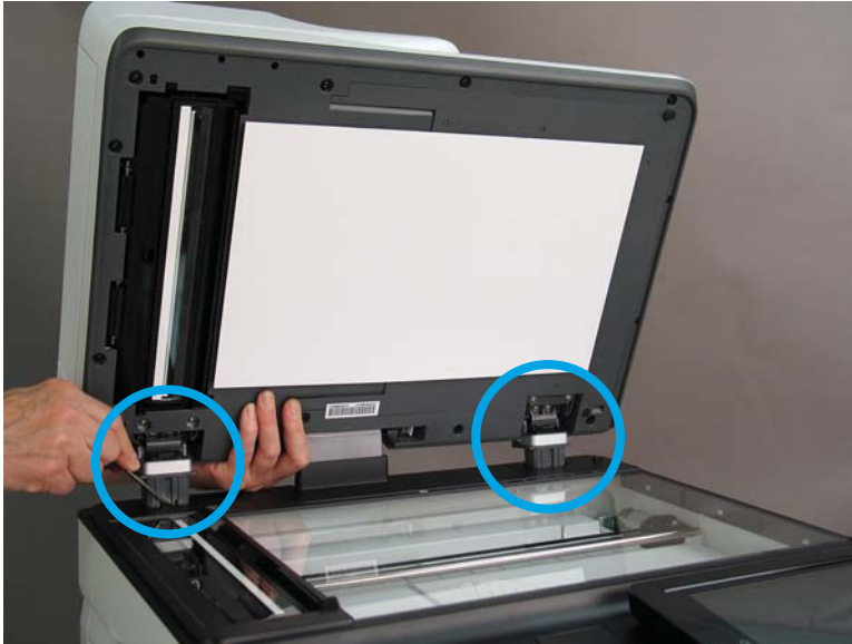
Figure 1-1099 Release two tabs on the ADF
