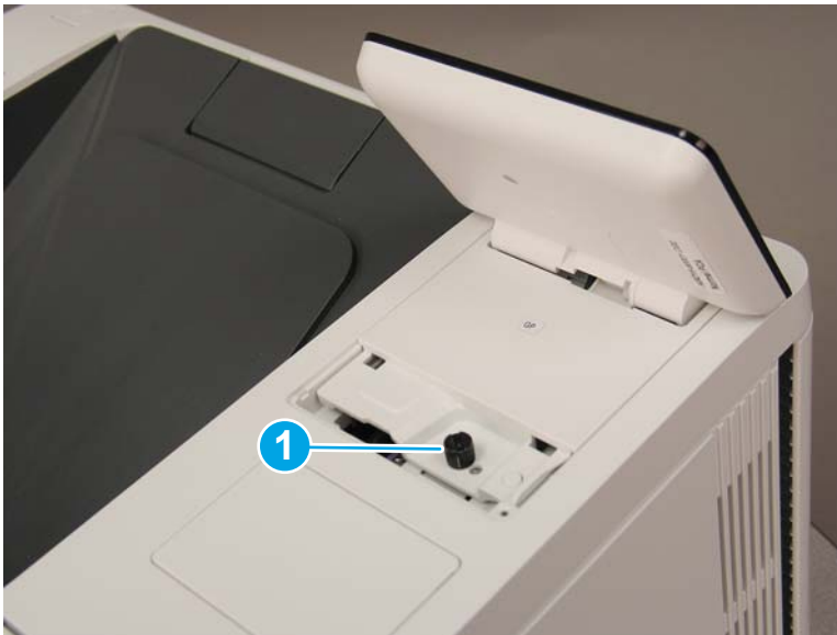
Figure 1-2175 Remove one thumbscrew
