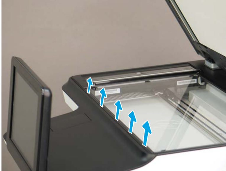
Figure 1-760 Release five tabs
