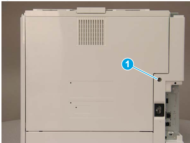
Figure 1-1938 Remove one screw
