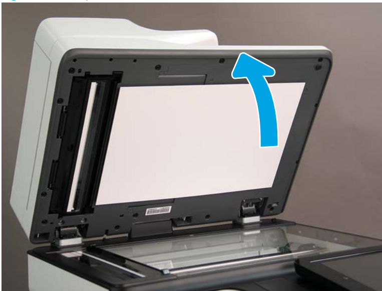
Figure 1-195 Open the ADF
