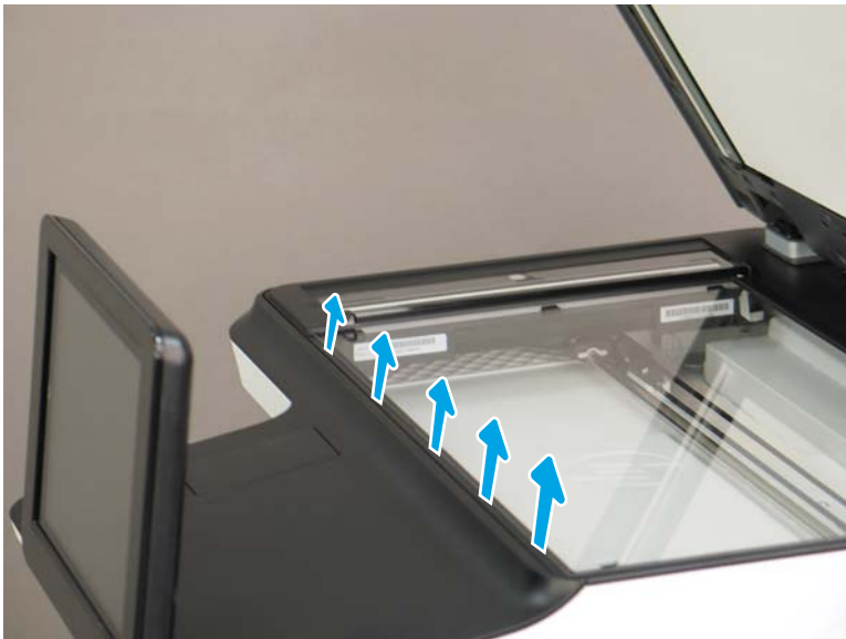
Figure 1-248 Release five tabs
