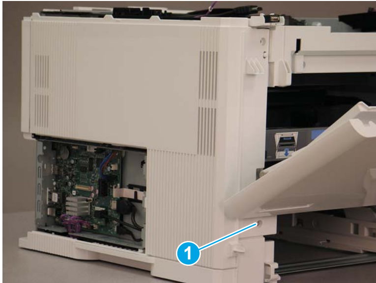
Figure 1-2222 Open the cartridge door and remove one screw
