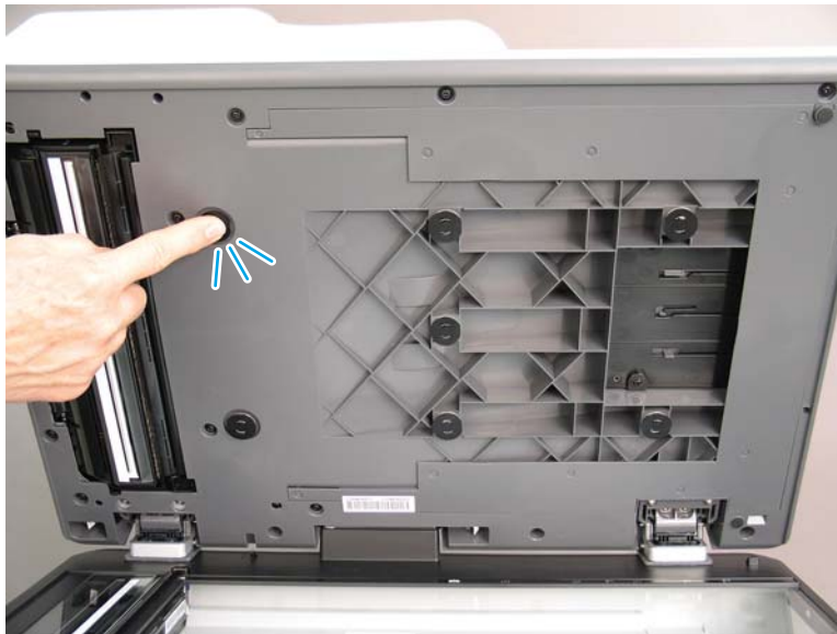
Figure 1-41 Press on each clip
