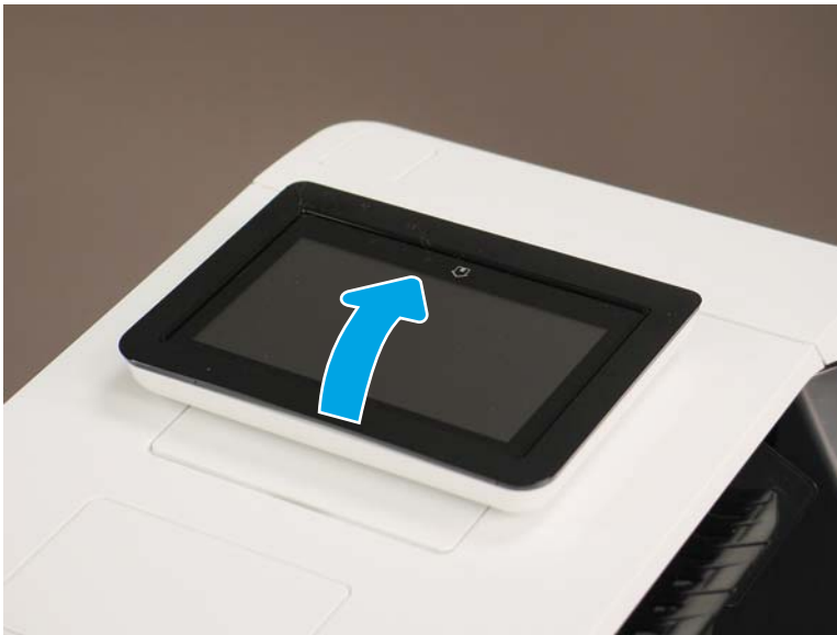
Figure 1-2208 Raise the control panel screen
