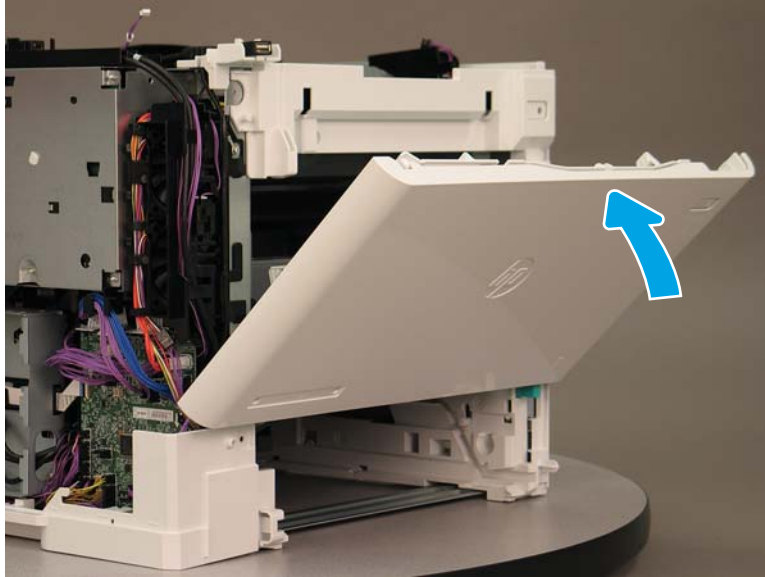
Figure 1-2125 Partially close the cartridge door
