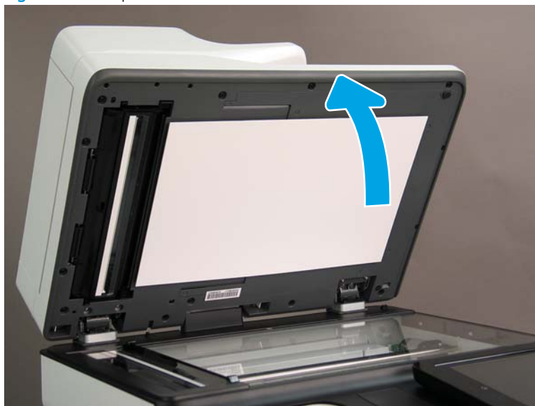
Figure 1-602 Open the ADF
