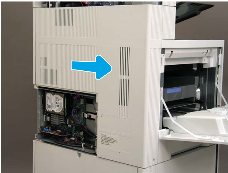
Figure 1-535 Slide the rear cover
