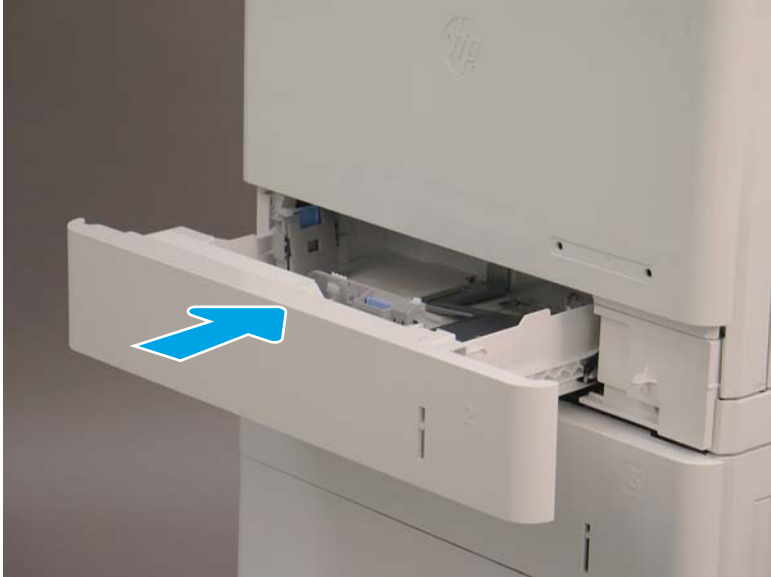
Figure 1-2495 Install the tray
