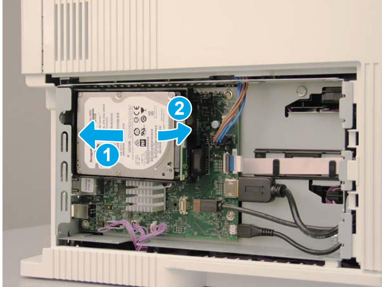
Figure 1-1751 Install the tab into the slot and rotate the connector end
