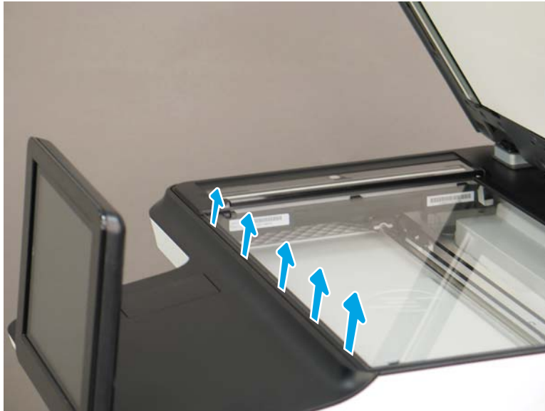
Figure 1-430 Release five tabs
