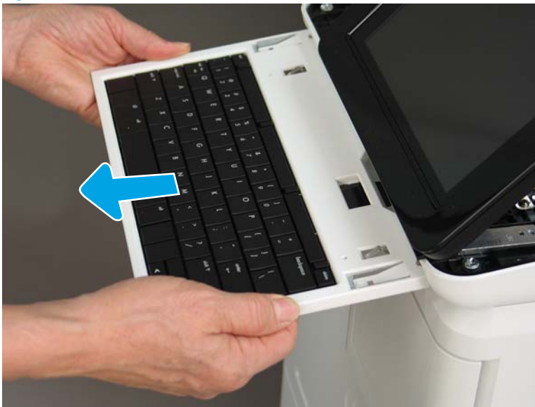
Figure 1-904 Remove the keyboard
