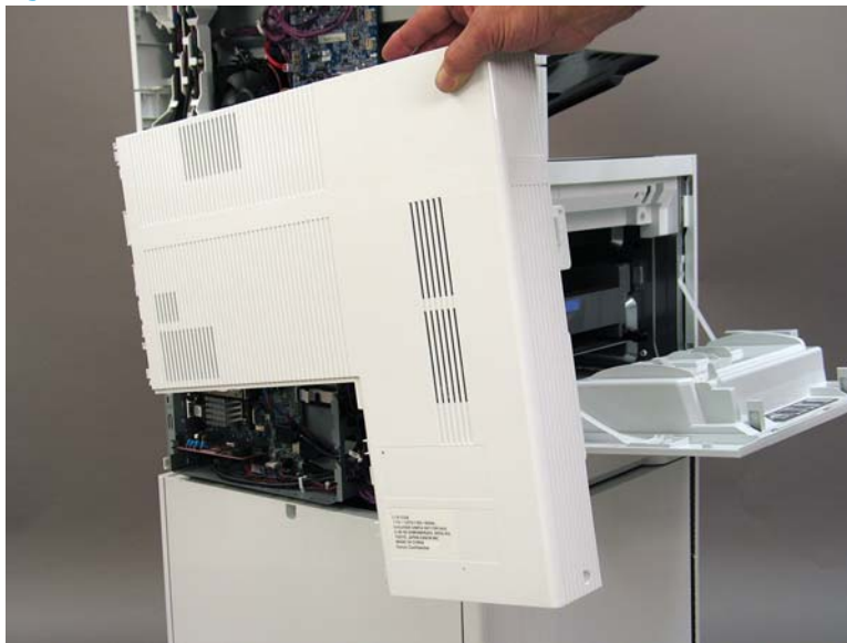
Figure 1-346 Remove the rear cover
