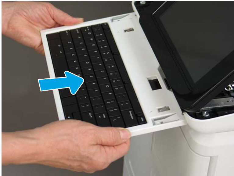
Figure 1-95 Slide the keyboard tray into the slot
