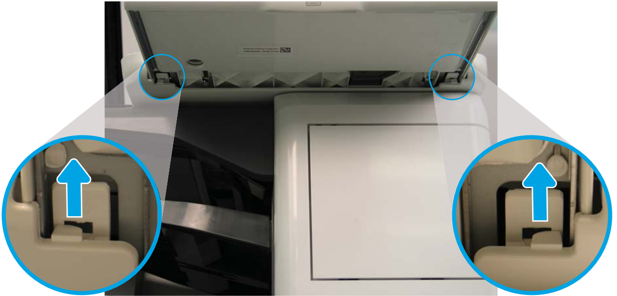
Figure 1-1009 Release two tabs
