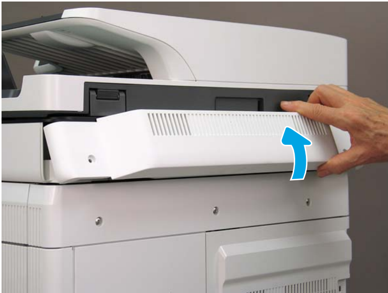
Figure 1-583 Remove the image scanner back cover
