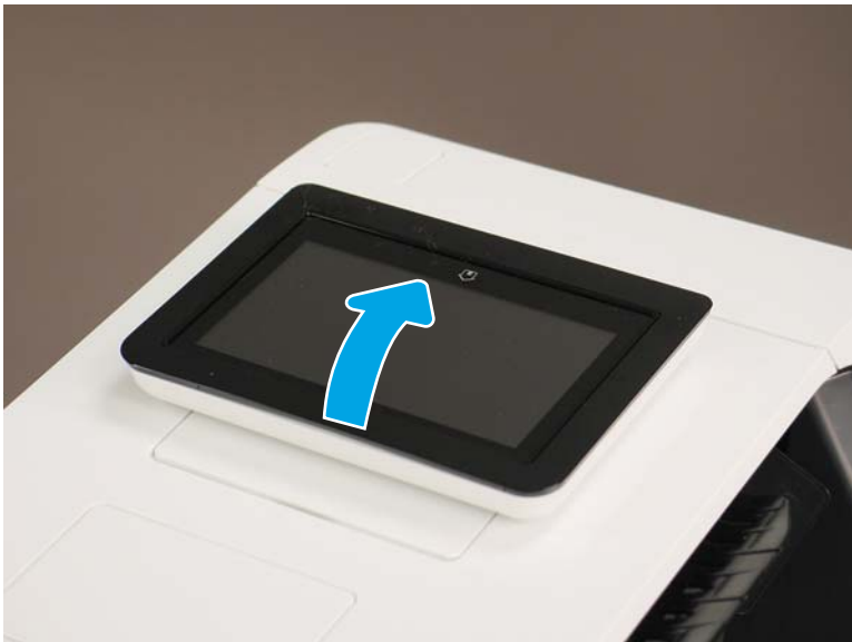
Figure 1-1949 Raise the control panel screen
