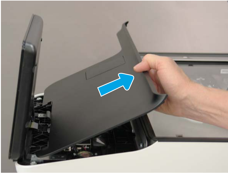
Figure 1-359 Remove the cover
