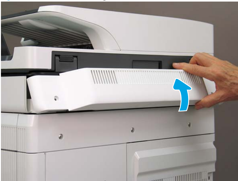
Figure 1-368 Remove the image scanner back cover
