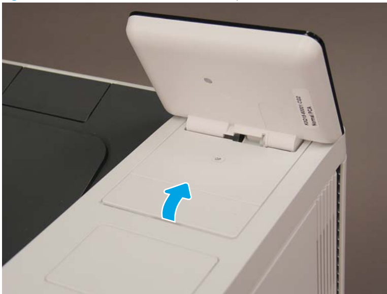
Figure 1-2382 Lift and remove the control panel cover
