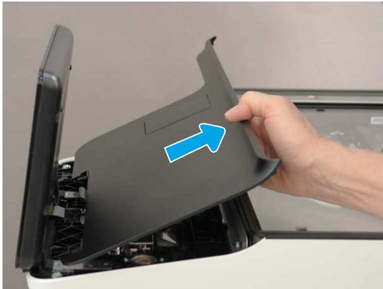
Figure 1-761 Remove the cover
