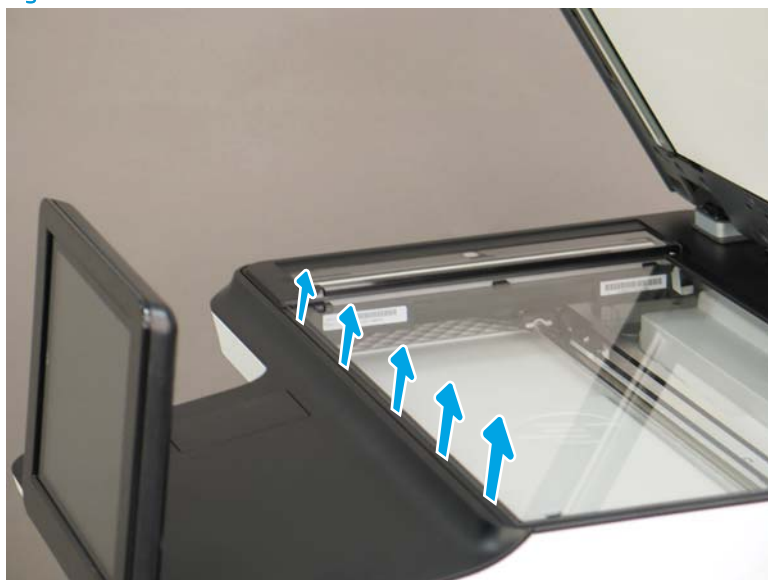
Figure 1-358 Release five tabs
