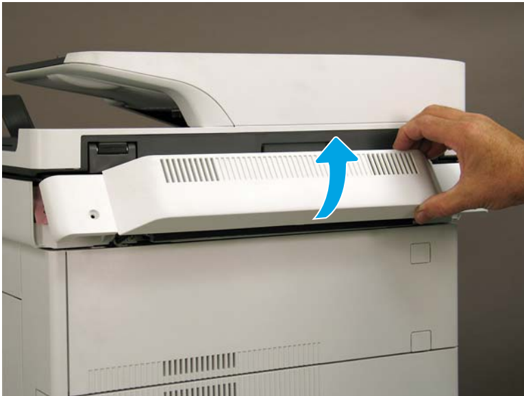
Figure 1-561 Remove the SCB cover
