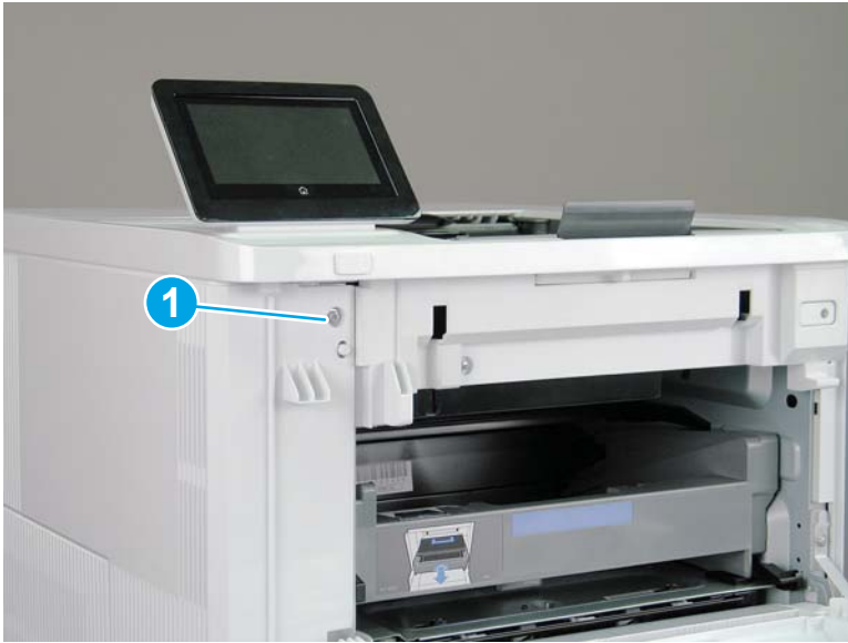
Figure 1-1849 Remove one screw
