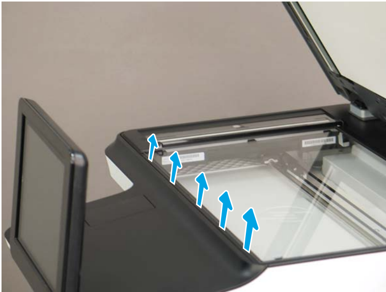
Figure 1-324 Release five tabs
