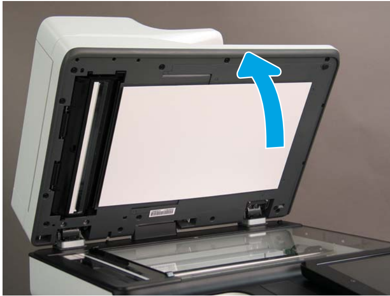
Figure 1-913 Open the ADF
