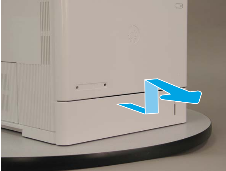
Figure 1-1217 Open and remove the cassette tray 2
