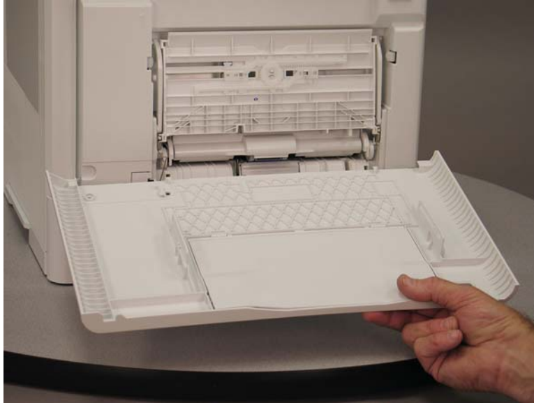
Figure 1-1890 Remove the MP cover
