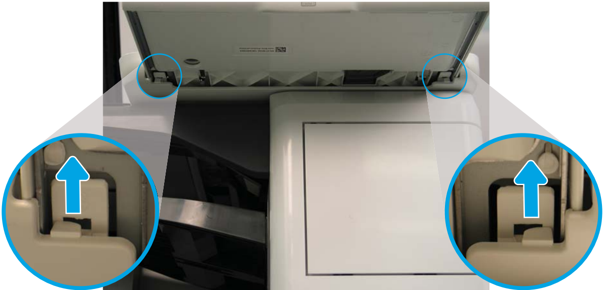
Figure 1-592 Release two tabs
