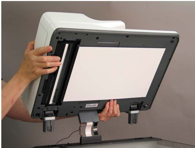
Figure 1-410 Lift and remove the ADF
