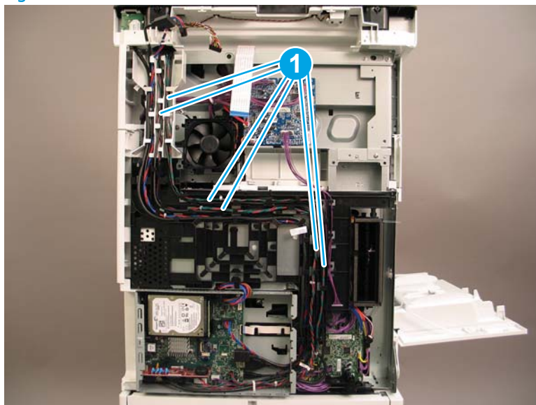
Figure 1-785 Release the formatter cables
