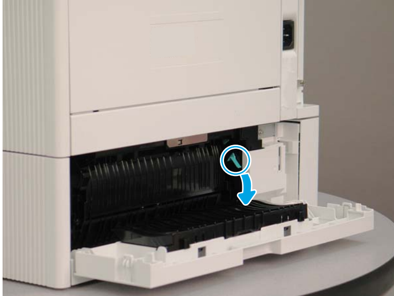
Figure 1-1771 Lower the access cover
