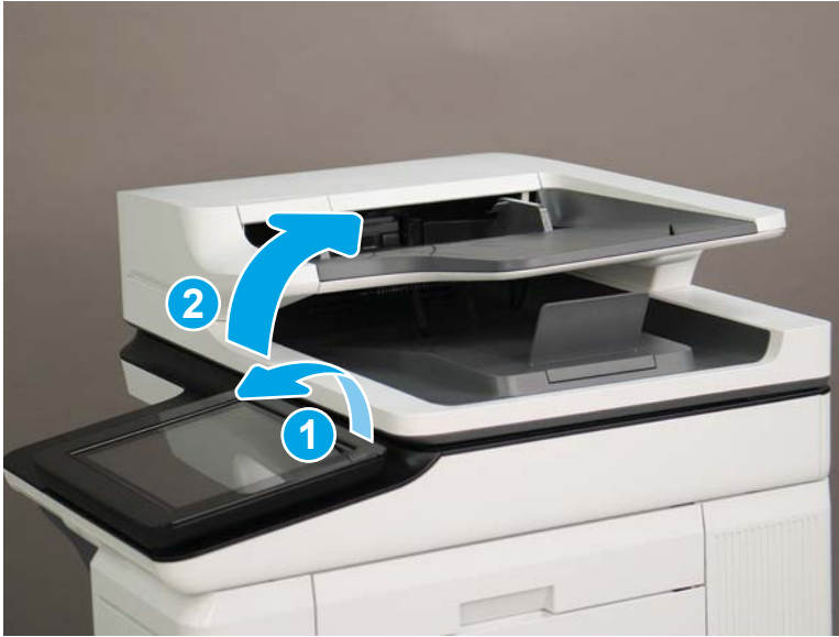
Figure 1-587 Tilt the control panel and open the document feeder
