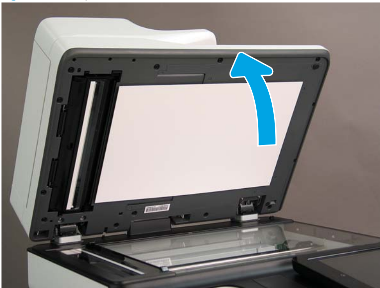
Figure 1-372 Open the ADF
