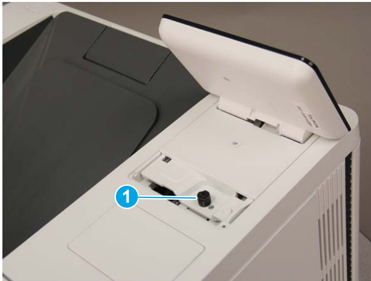
Figure 1-2133 Remove one thumbscrew
