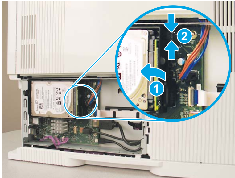
Figure 1-1745 Release the locking connector and release the HDD retainer
