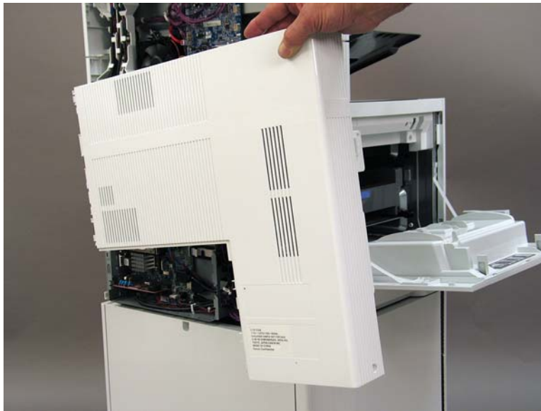
Figure 1-696 Remove the rear cover
