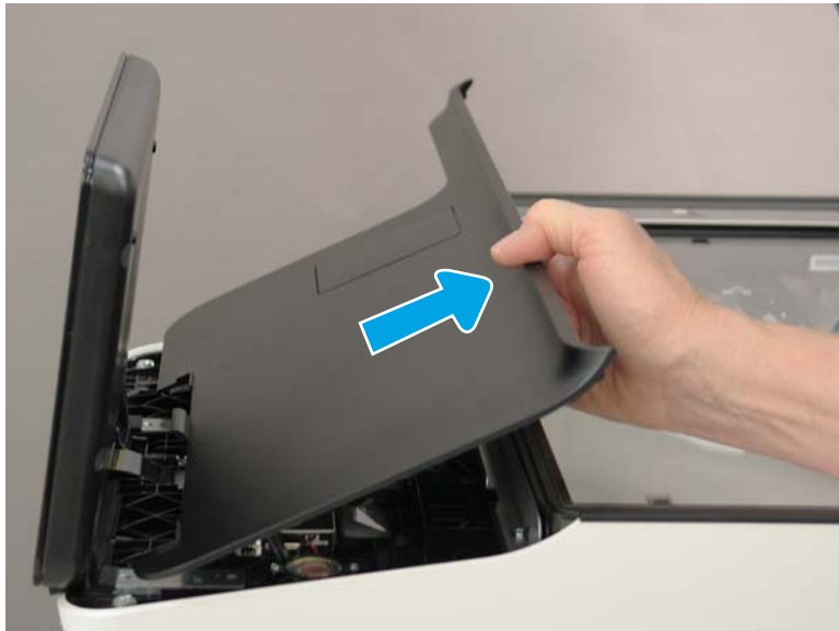
Figure 1-947 Remove the cover
