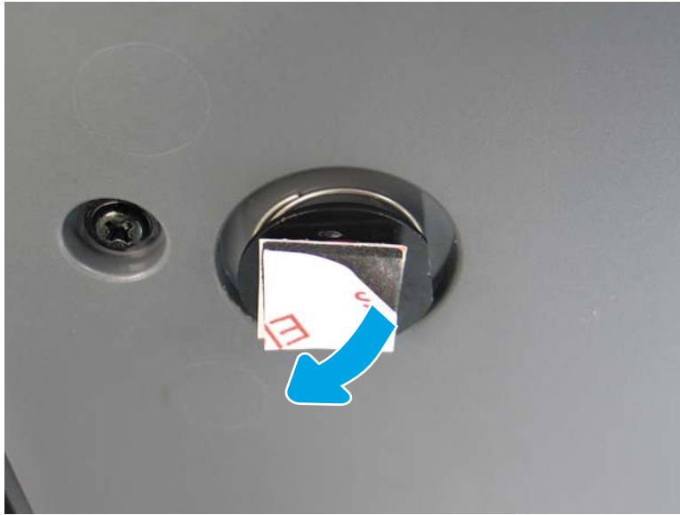
Figure 1-44 Remove the protective film
