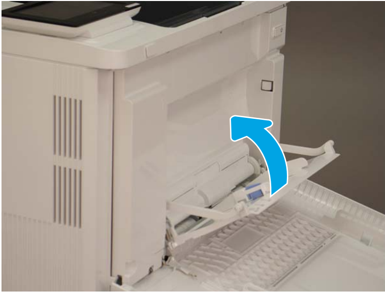
Figure 1-2442 Close the smaller MP tray assembly
