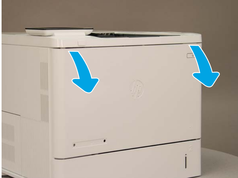
Figure 1-1875 Open the MP cover
