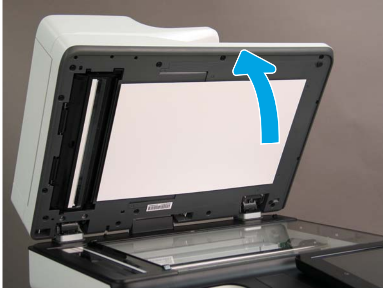
Figure 1-37 Open the document feeder
