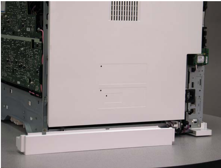
Figure 1-1926 Remove the rear lower cover
