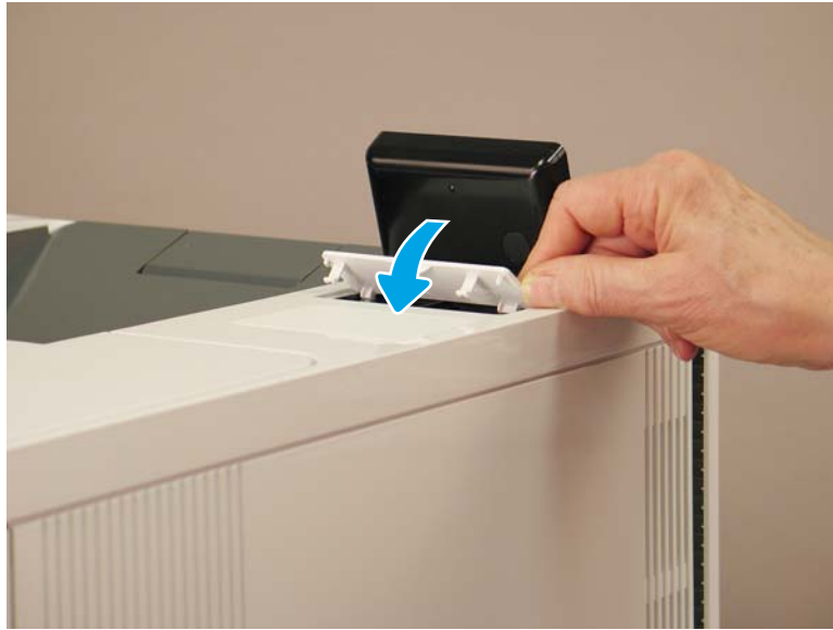
Figure 1-1709 Align the control panel cover and pivot down to install it
