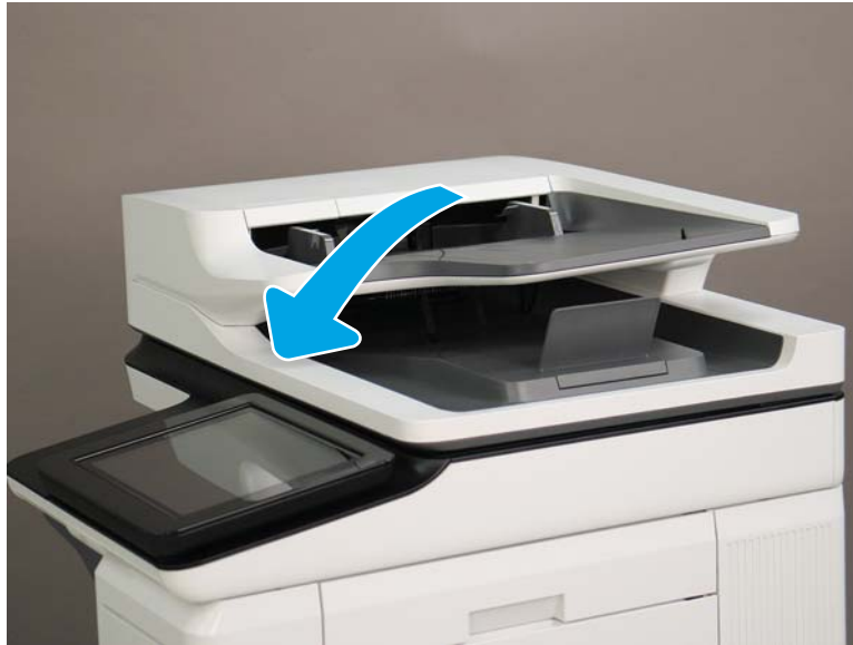
Figure 1-116 Close the document feeder
