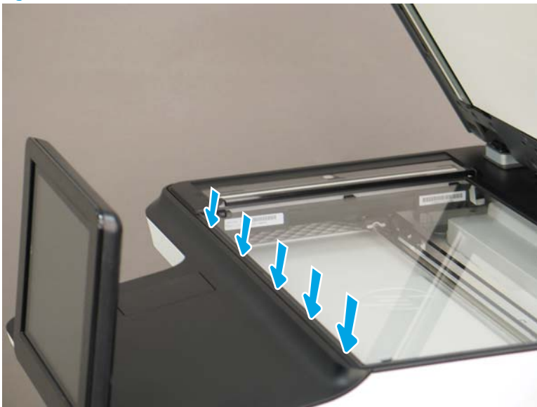
Figure 1-115 Install five tabs
