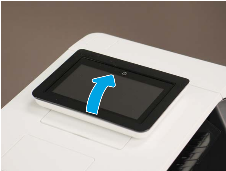
Figure 1-2469 Raise the control panel screen
