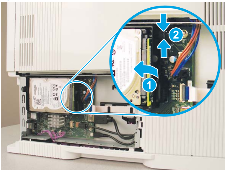
Figure 1-1733 Release the HDD locking connector and pinch the retainer to release it
