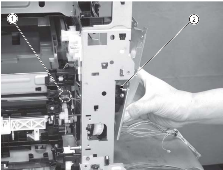
Figure 1-2307 Disconnect one connector and remove the main drive assembly
