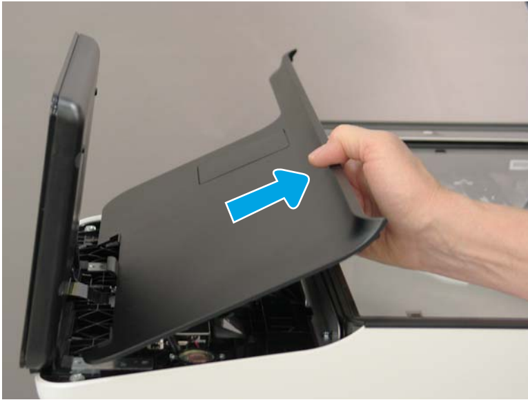
Figure 1-89 Remove the cover
