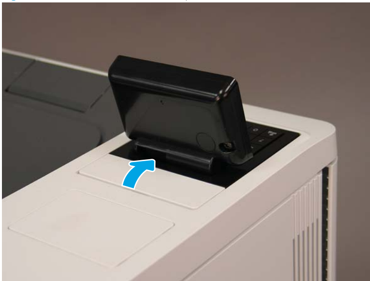
Figure 1-1701 Release the control panel cover and remove it
