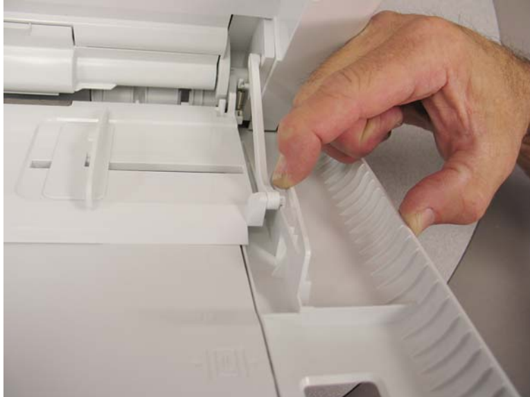
Figure 1-1876 Release the MP tray assembly lift arms from the MP cover
