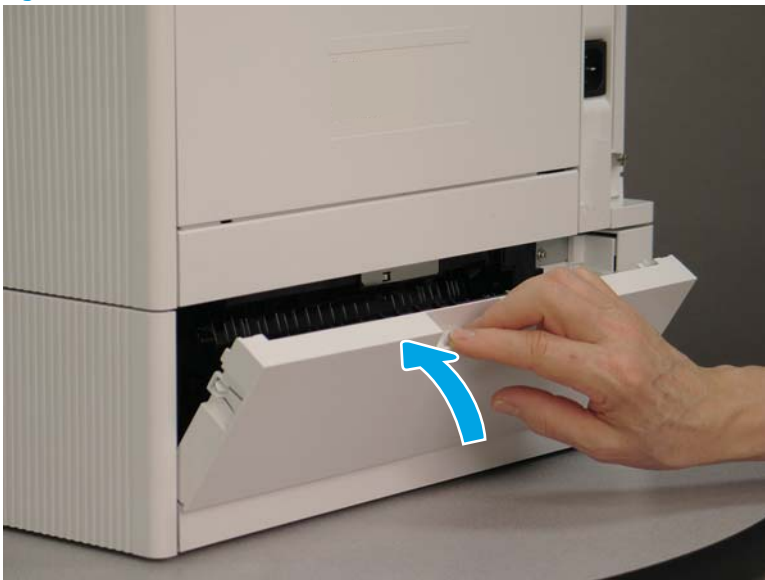
Figure 1-1798 Close the rear lower cover
