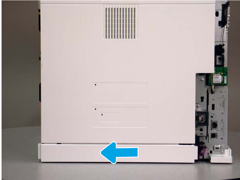
Figure 1-1925 Slide the rear lower cover
