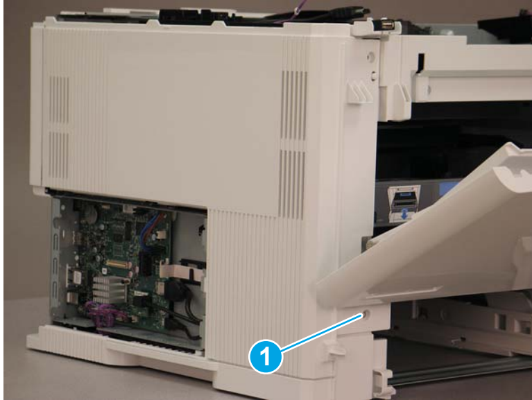
Figure 1-2371 Open the cartridge door and remove one screw
