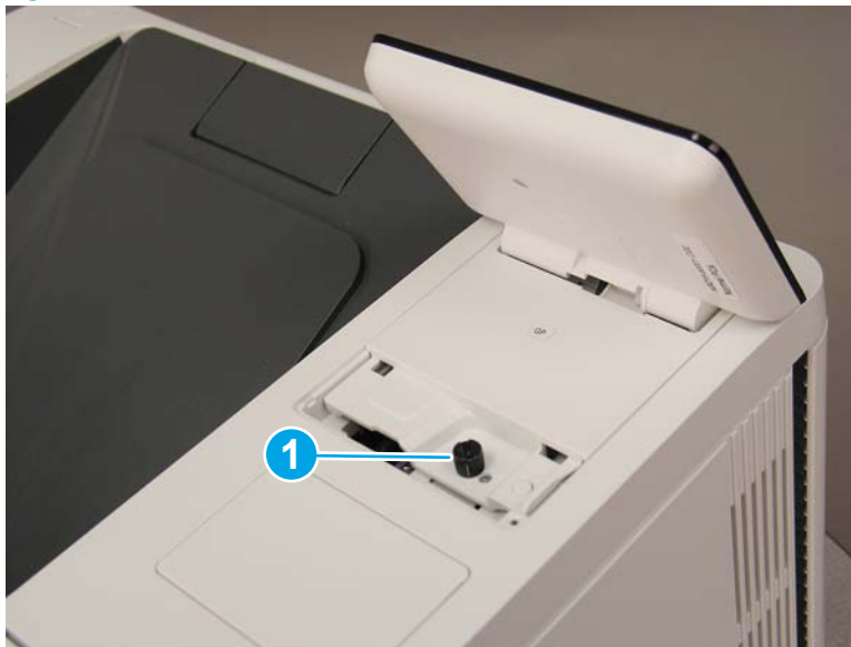
Figure 1-2471 Remove one thumbscrew
