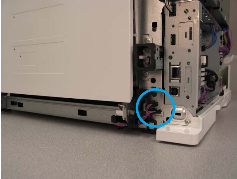
Figure 1-2270 Disconnect two connectors
