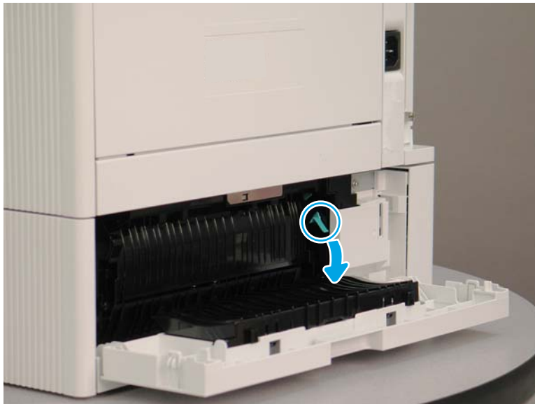
Figure 1-122 Lower the access cover
