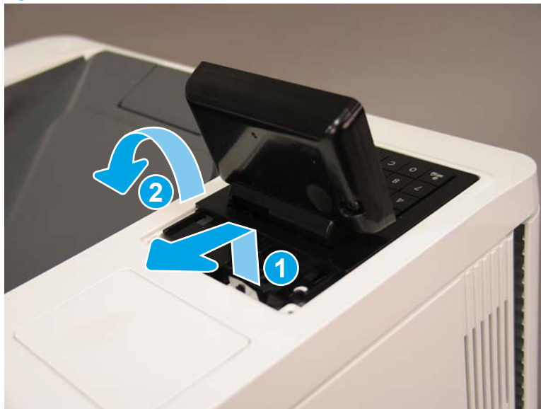
Figure 1-1703 Release the control panel and turn it over
