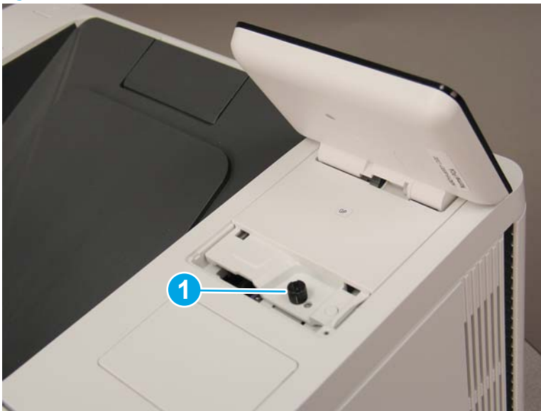
Figure 1-2251 Remove one thumbscrew
