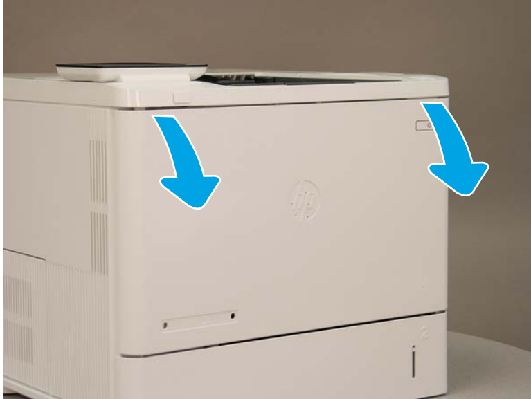
Figure 1-2440 Open the MP cover
