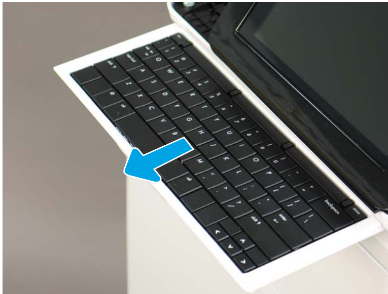
Figure 1-217 Slide the keyboard tray out
