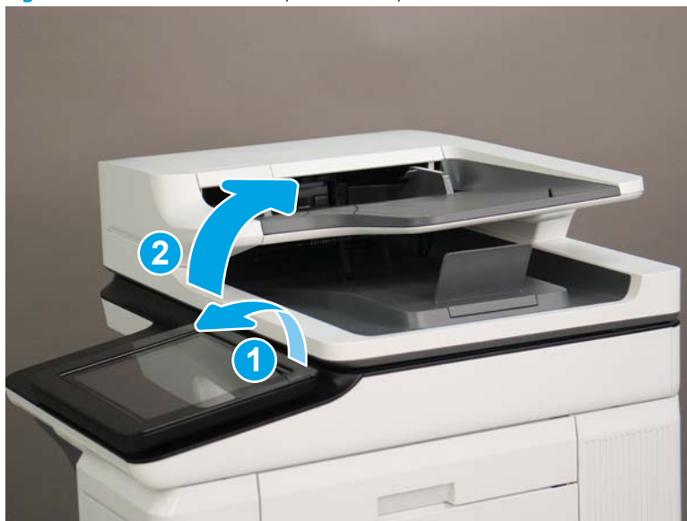
Figure 1-470 Tilt the control panel and open the document feeder
