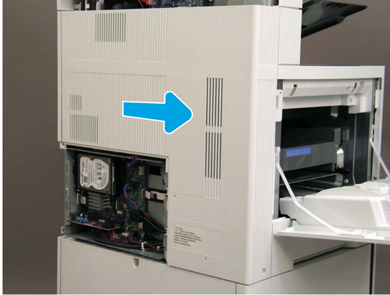
Figure 1-414 Slide the rear cover
