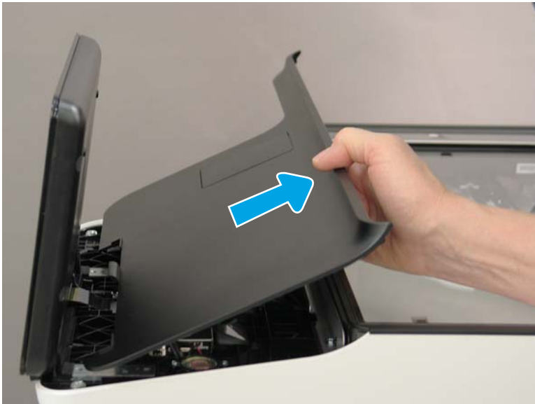
Figure 1-472 Remove the cover
