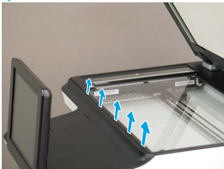
Figure 1-1170 Release five tabs
