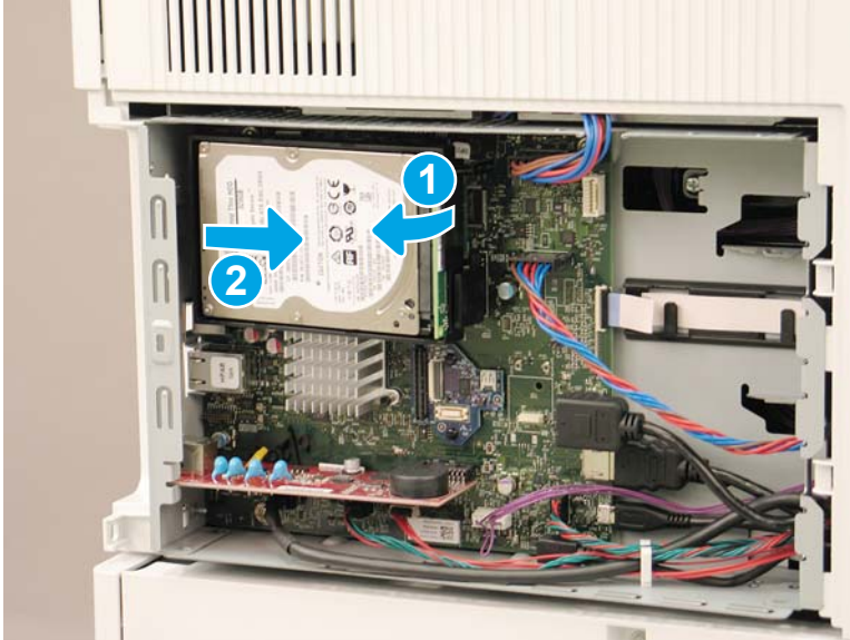
Figure 1-52 Rotate the HDD away from the formatter and remove the HDD
