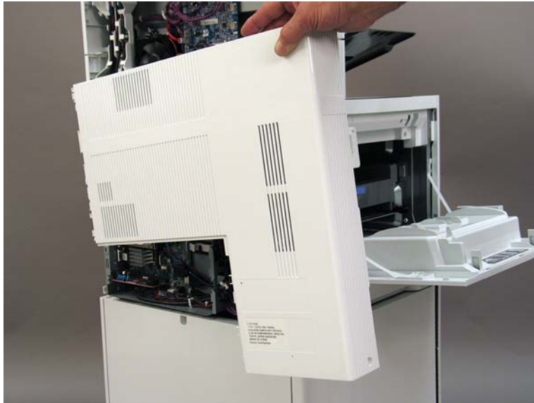
Figure 1-415 Remove the rear cover
