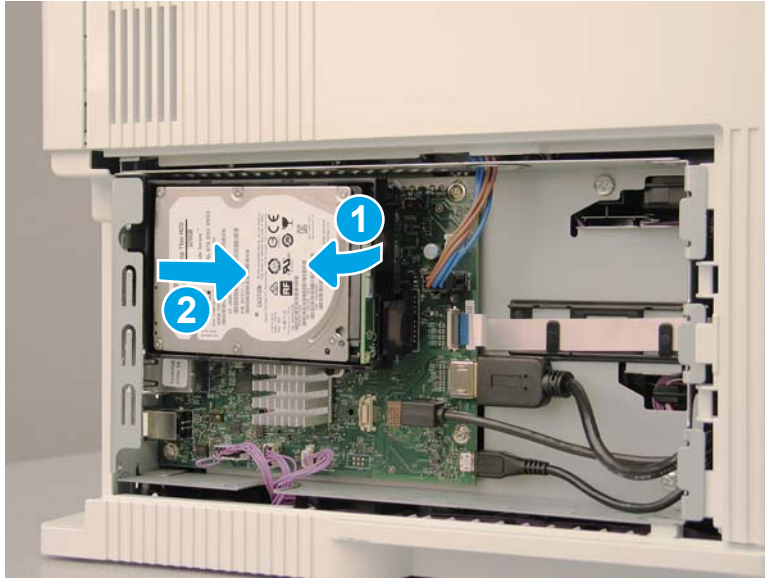
Figure 1-1734 Rotate the HDD away from the formatter and remove the HDD
