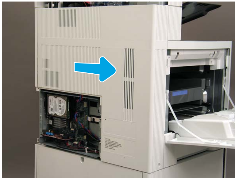
Figure 1-644 Slide the rear cover
