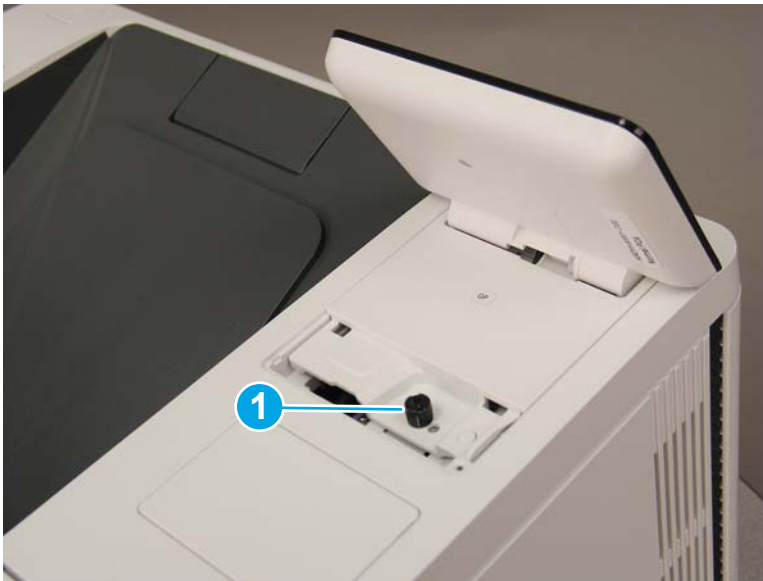
Figure 1-1824 Remove one thumbscrew
