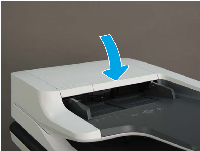
Figure 1-36 Close the document feeder cover
