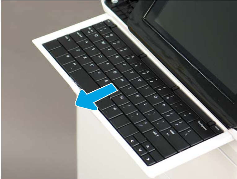
Figure 1-396 Slide the keyboard tray out
