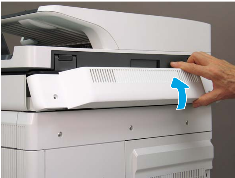
Figure 1-1180 Remove the image scanner back cover
