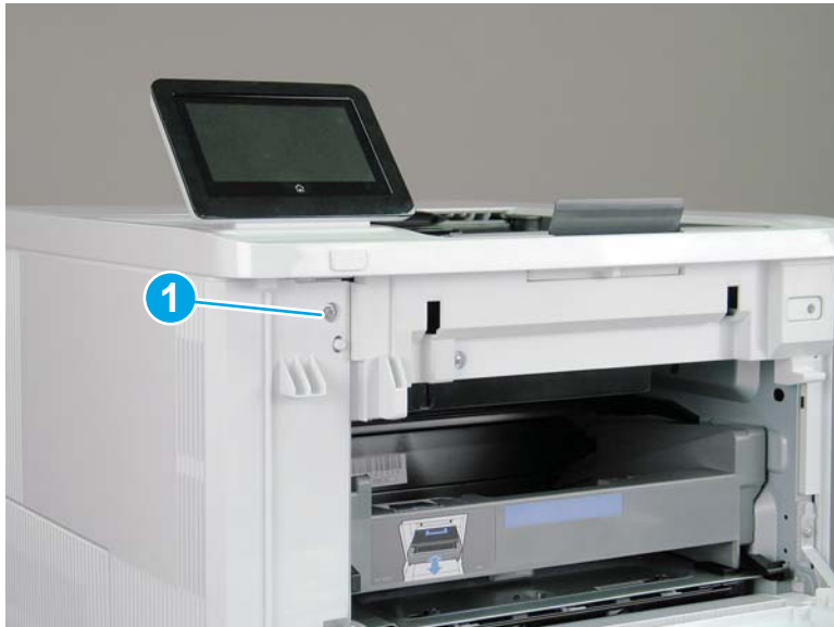
Figure 1-2372 Remove one screw
