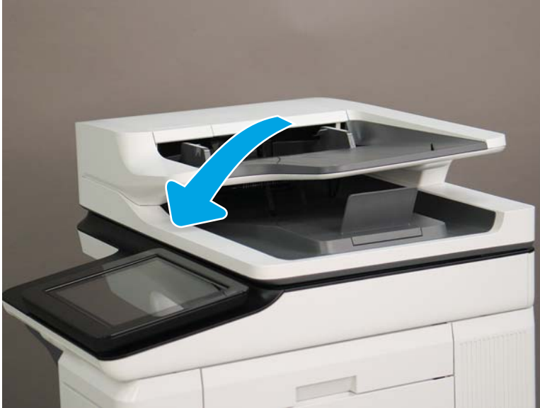
Figure 1-100 Close the document feeder
