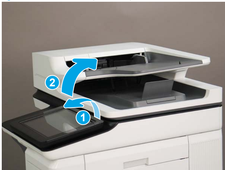
Figure 1-357 Tilt the control panel and open the document feeder
