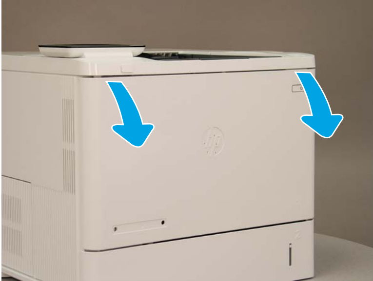
Figure 1-1869 Open the MP cover
