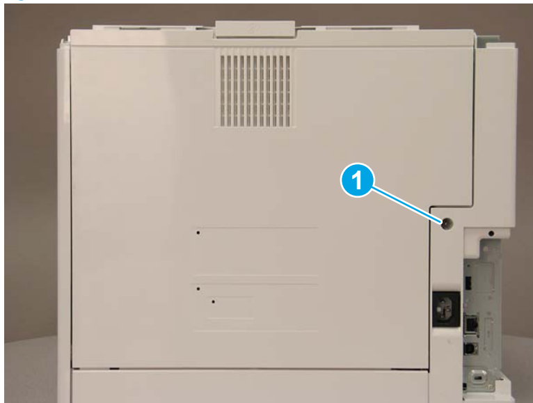
Figure 1-2067 Remove one screw
