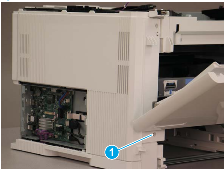
Figure 1-1984 Open the cartridge door and remove one screw
