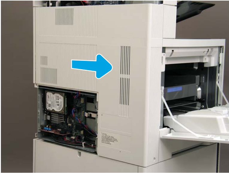
Figure 1-235 Slide the rear cover
