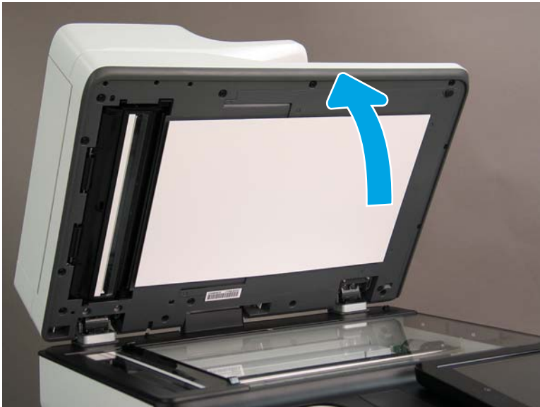
Figure 1-565 Open the ADF
