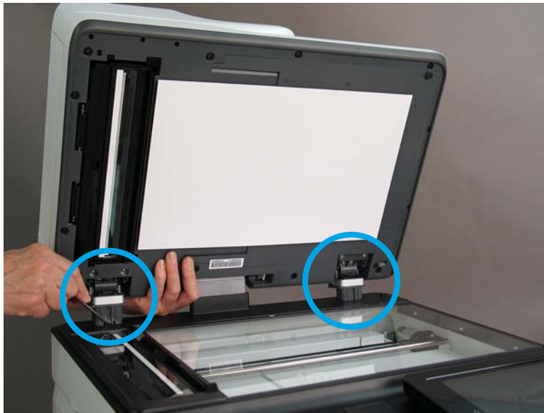
Figure 1-962 Release two tabs on the ADF
