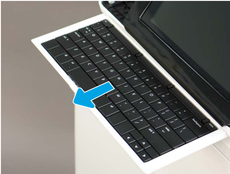
Figure 1-808 Slide the keyboard tray out
