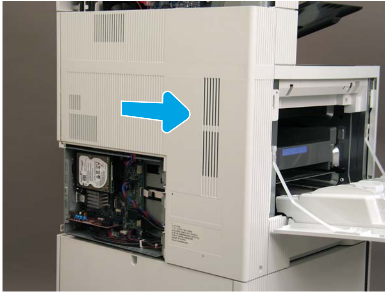
Figure 1-345 Slide the rear cover
