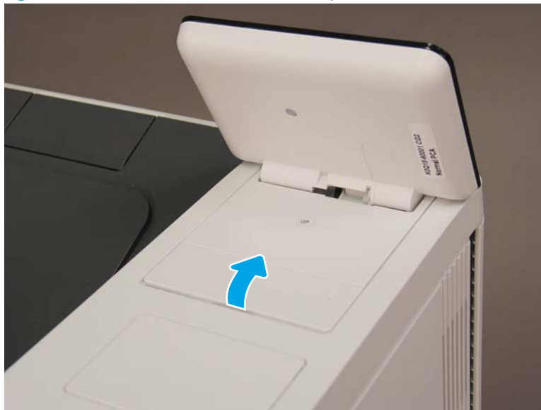
Figure 1-1691 Lift and remove the control panel cover
