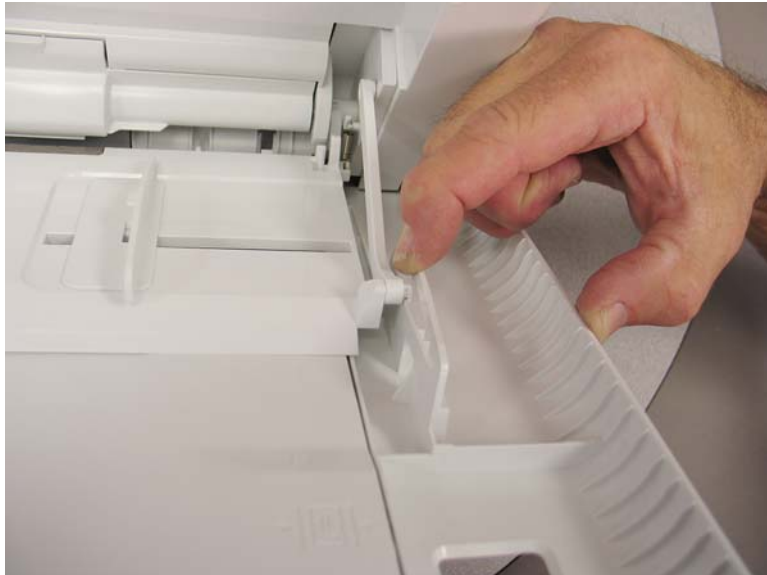
Figure 1-2441 Release the MP tray assembly lift arms from the MP cover
