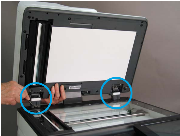
Figure 1-230 Release two tabs on the ADF
