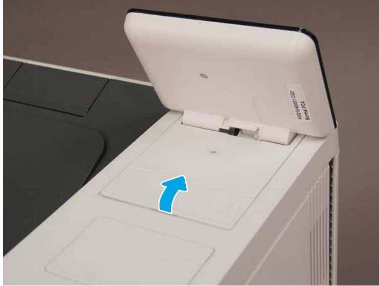
Figure 1-1950 Lift and remove the control panel cover
