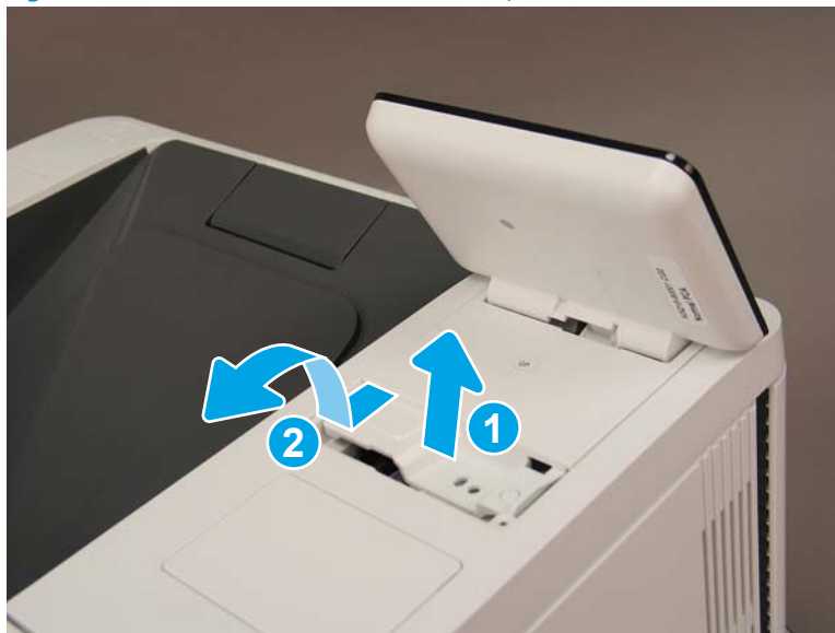
Figure 1-2324 Lift and release the control panel
