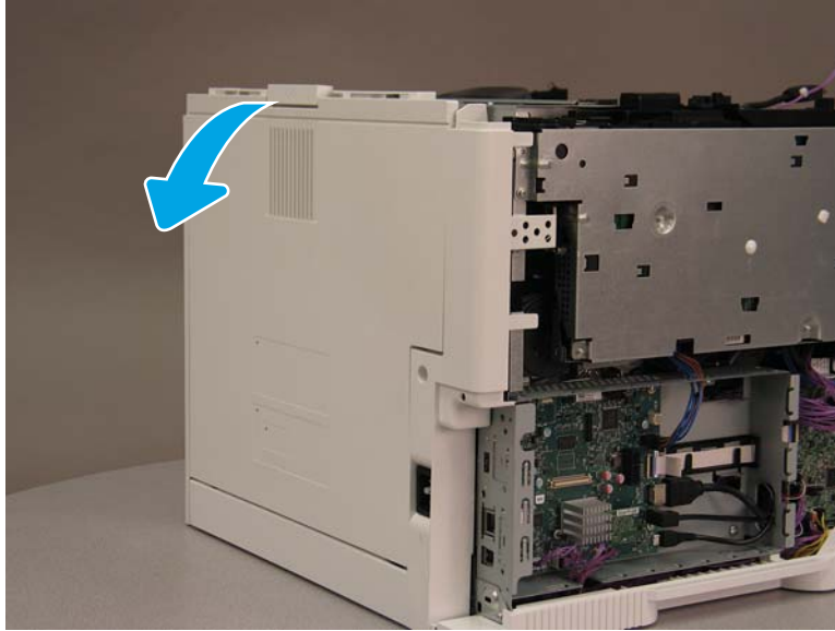
Figure 1-2185 Unlatch and open the rear door
