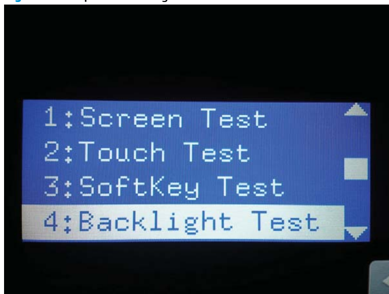
Figure 2-38 Open the backlight test
