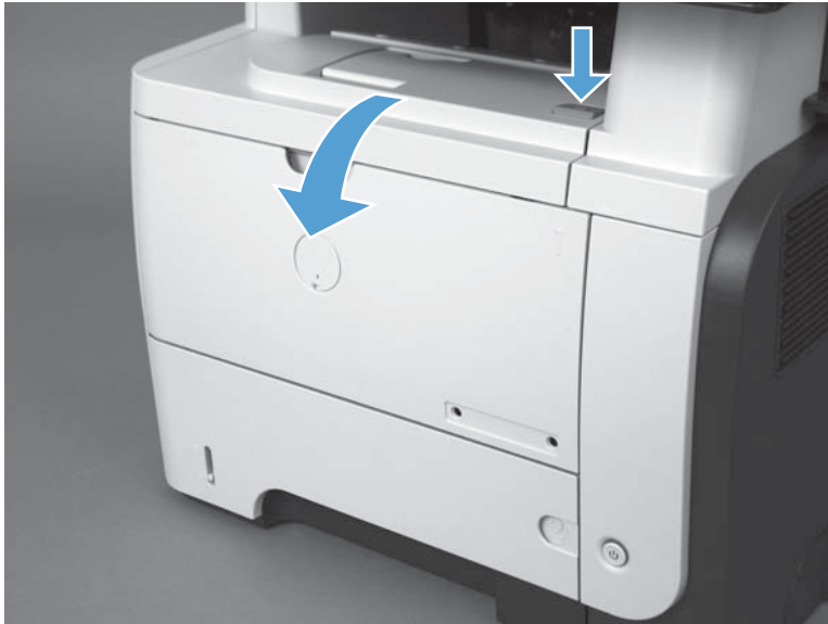
Figure 1-103 Remove the Tray 1 pickup roller (1 of 2)
