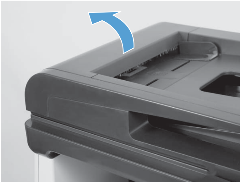
Figure 1-12 Remove the document feeder separation pad (1 of 2)
