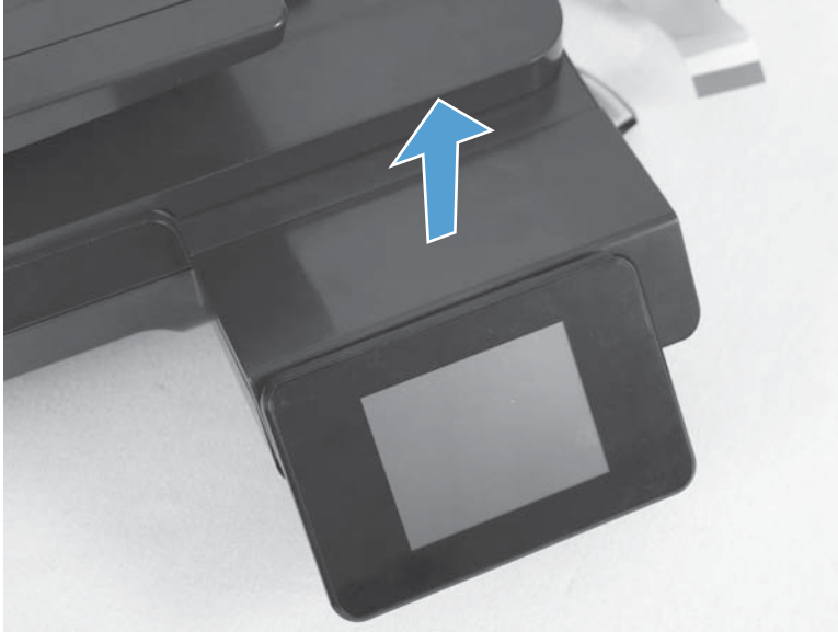
Figure 1-78 Remove the control-panel top-cover (2 of 2)
