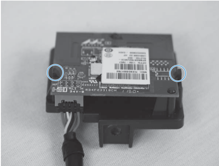
Figure 1-101 Remove the Wi-Fi module and cable (5 of 6)
