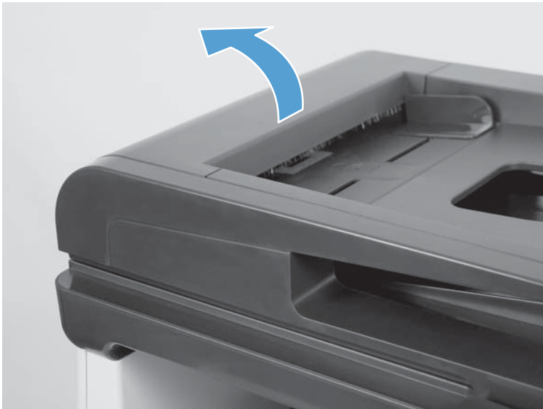
Figure 1-8 Remove the document feeder pickup roller (1 of 2)
