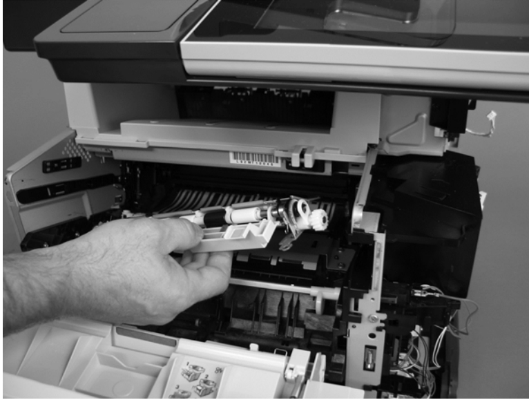
Figure 1-127 Removing the registration roller assembly (3 of 3)
