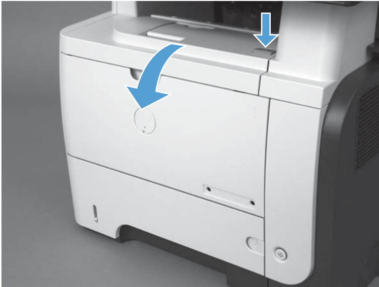
Figure 1-113 Remove the transfer roller (1 of 3)
