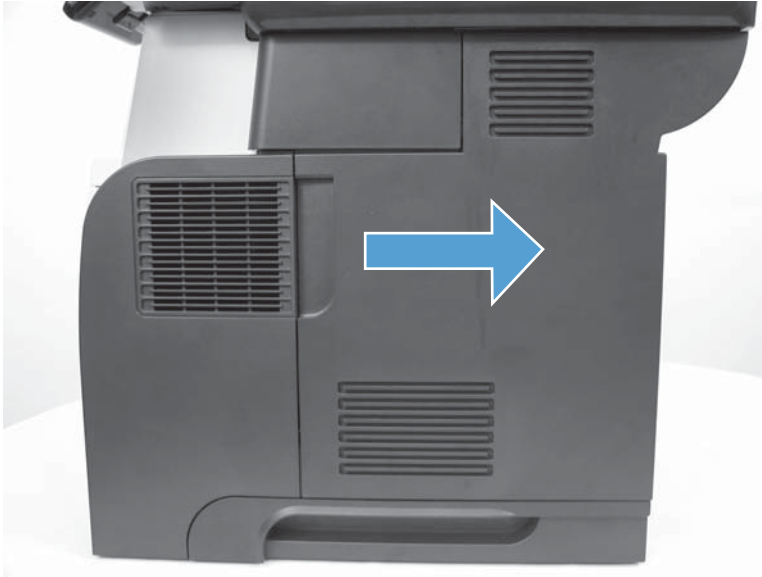
Figure 1-14 Remove the formatter cover
