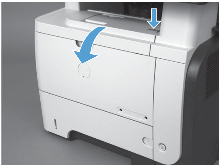
Figure 1-5 Remove the toner cartridge (1 of 2)
