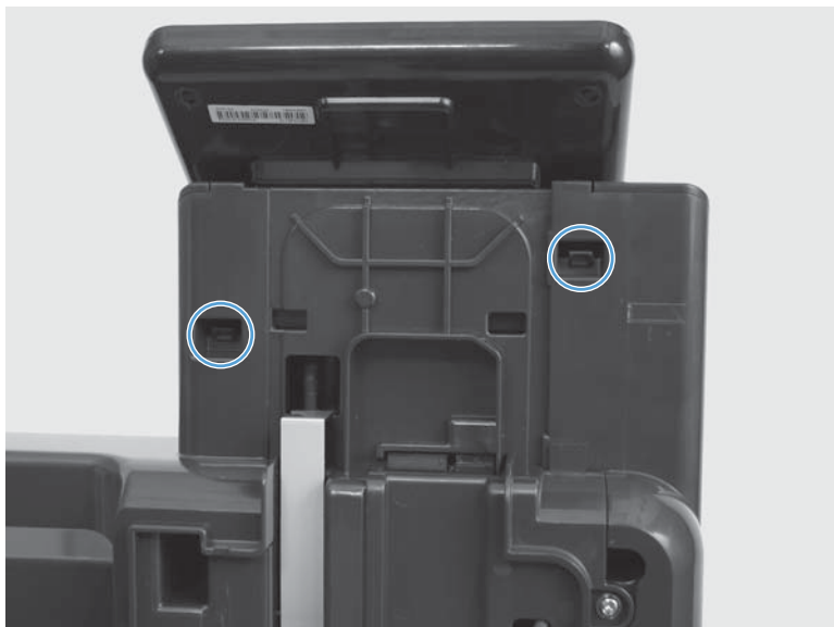
Figure 1-77 Remove the control-panel top-cover (1 of 2)
