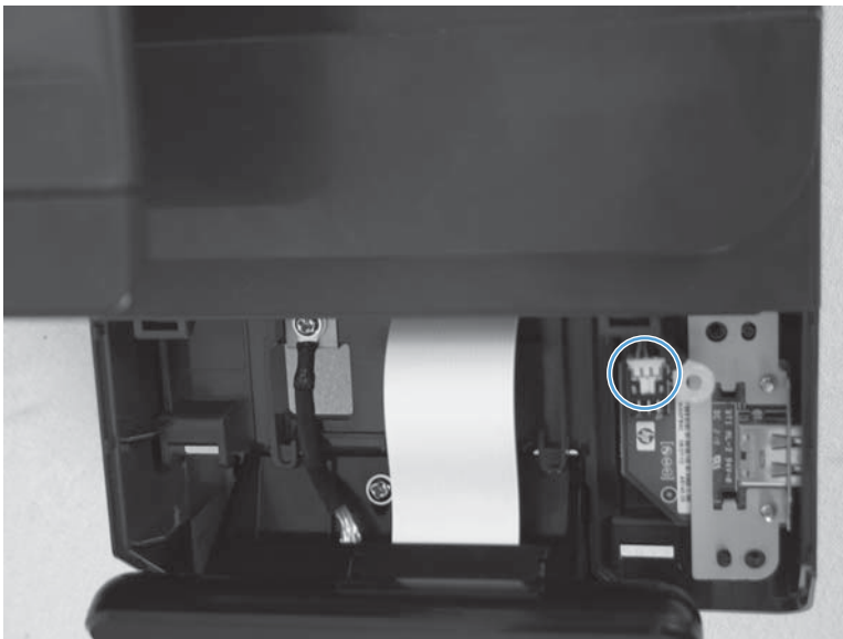
Figure 1-82 Remove the USB PCA (2 of 4)
