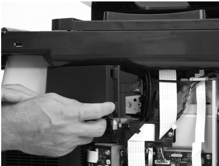
Figure 1-23 Remove the dummy cover (2 of 2)
