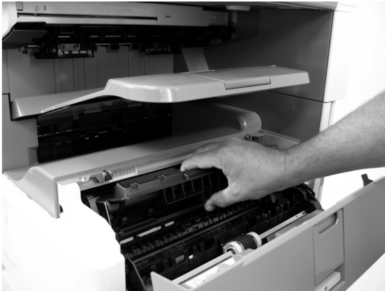
Figure 5-3 Remove the print cartridge (2 of 2)
