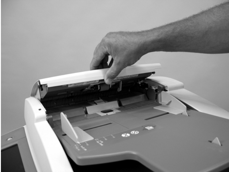
Figure 5-44 Remove the ADF separation floor assembly (1 of 4)
