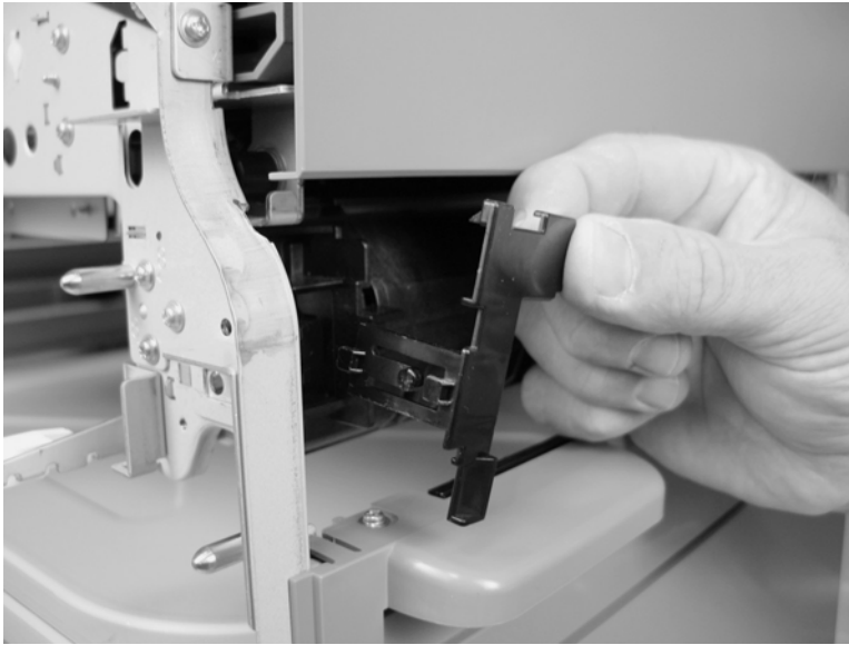
Figure 5-224 Remove the print cartridge door (10 of 12)
