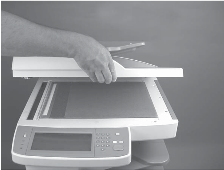
Figure 5-61 Remove the ADF white backing (3 of 4)
