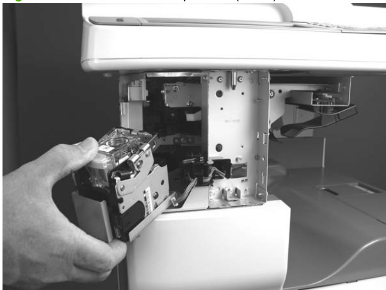
Figure 5-151 Remove the stapler unit (2 of 2)
