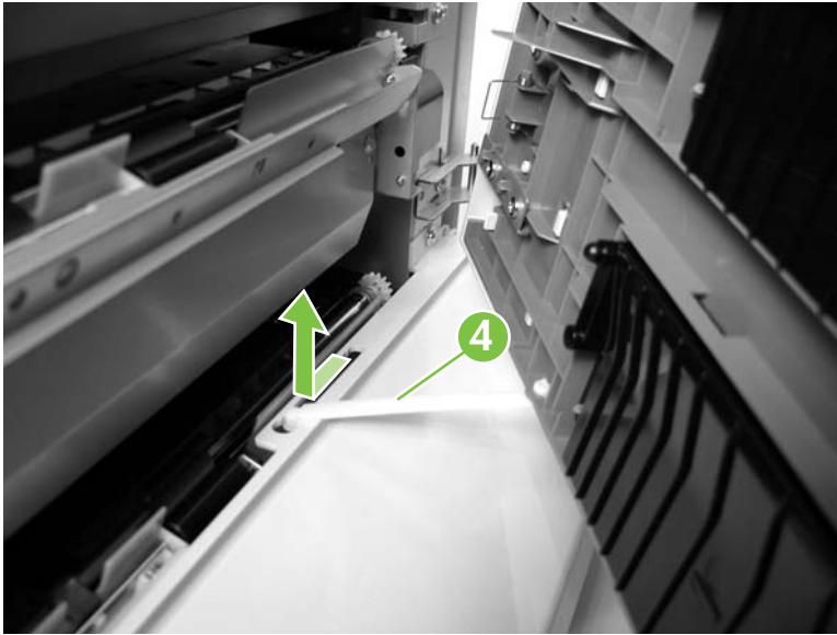
Figure 5-302 Remove the HCI right door (5 of 5)
