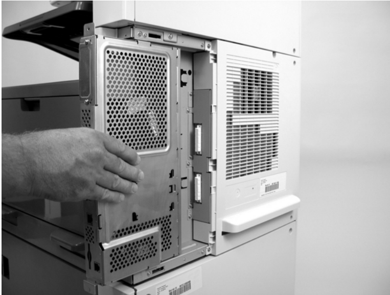
Figure 5-32 Remove the formatter cover and cage (3 of 3)
