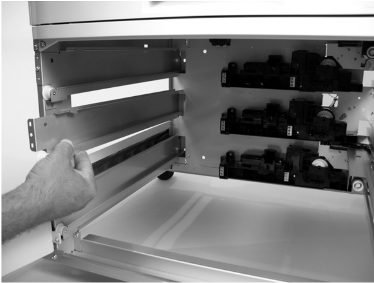
Figure 5-317 Remove the HCI left side tray rail(s) (3 of 3)
