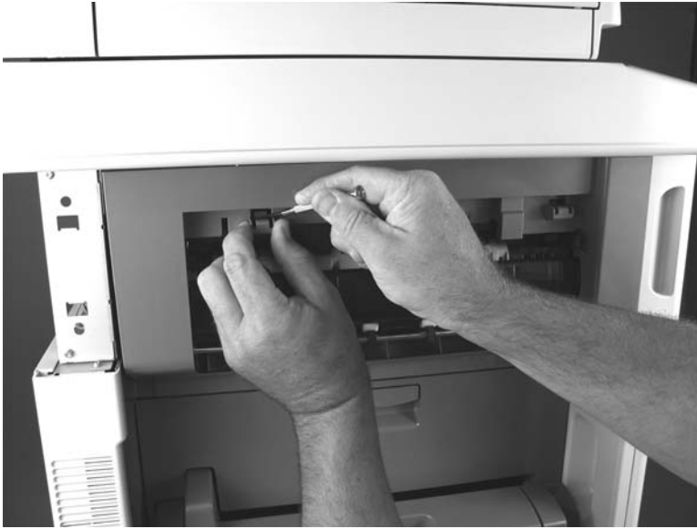
Figure 5-133 Remove the stapler left cover (2 of 3)
