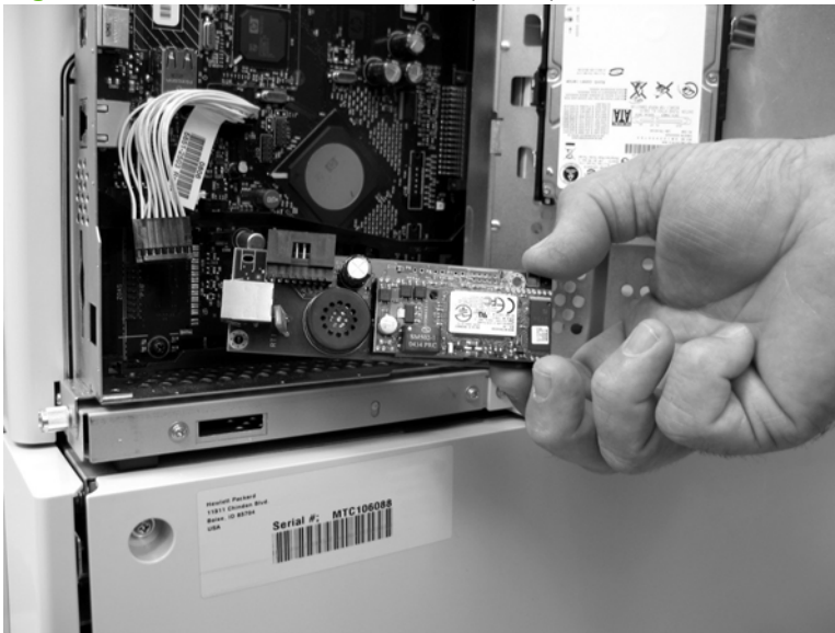
Figure 5-37 Remove the Fax PCA (2 of 2)
