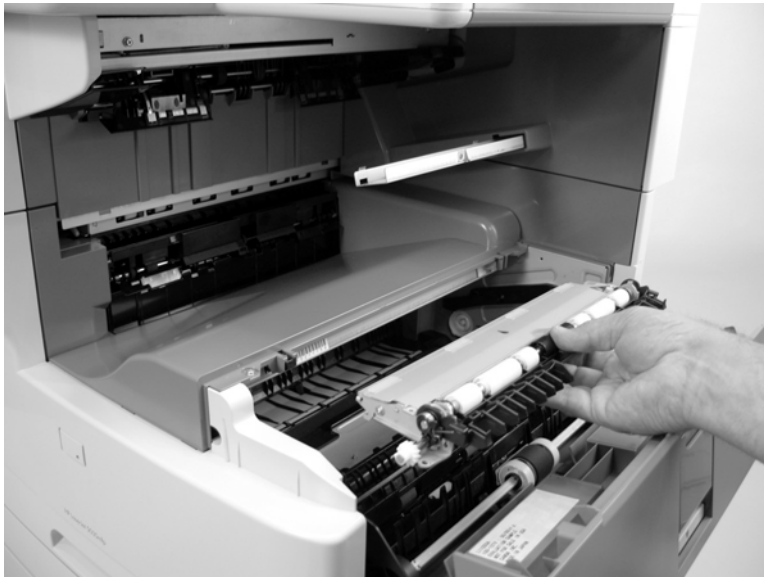
Figure 5-230 Remove the registration assembly (4 of 5)
