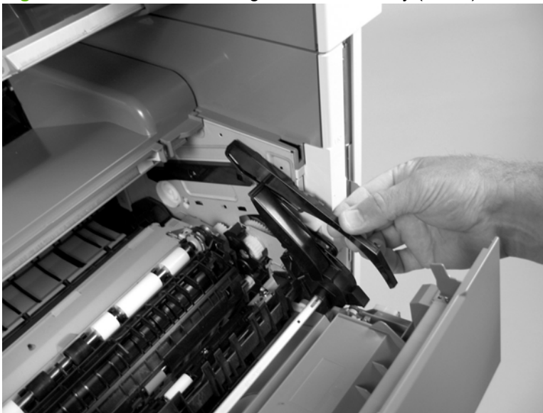
Figure 5-228 Remove the registration assembly (2 of 5)
