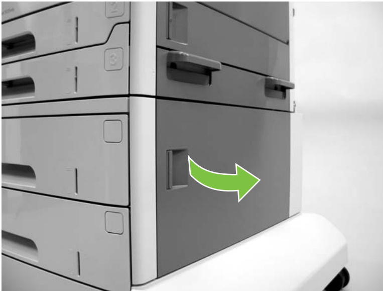
Figure 5-298 Remove the HCI right door (1 of 5)
