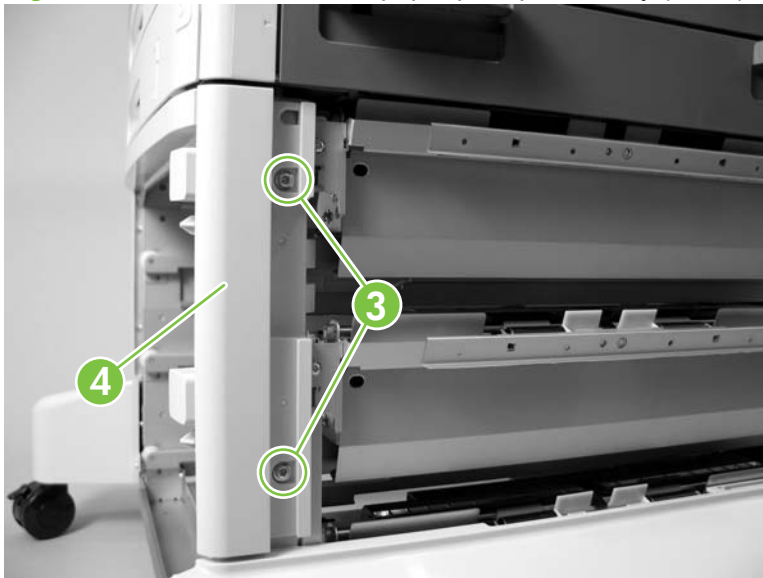
Figure 5-308 Remove the HCI paper pickup assembly (2 of 6)
