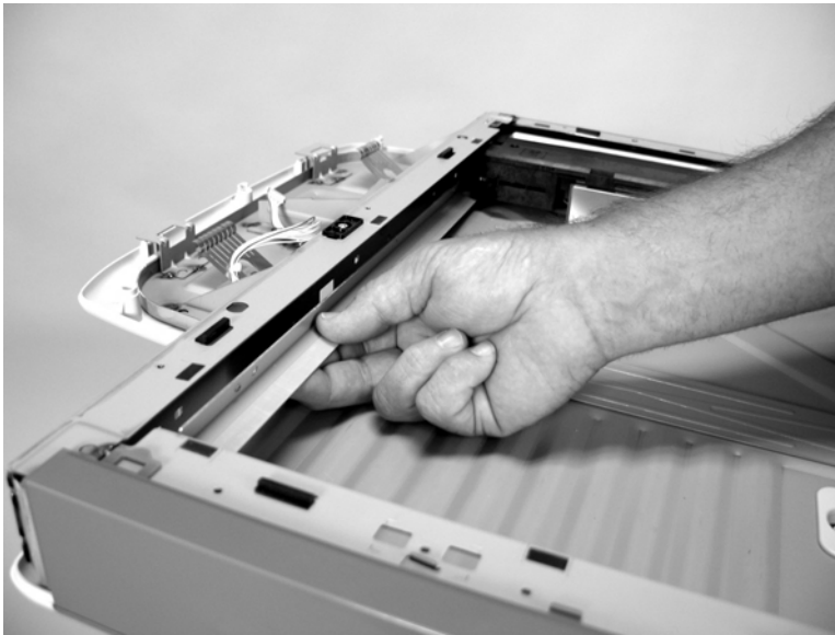
Figure 5-119 Remove the scanner transmission assemblies and slide rail (5 of 5)
