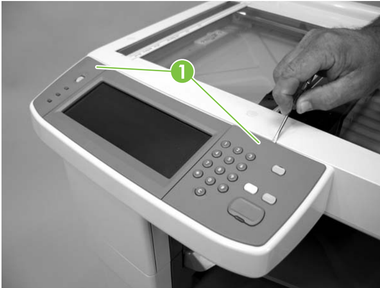
Figure 5-78 Remove the control panel (1 of 3)
