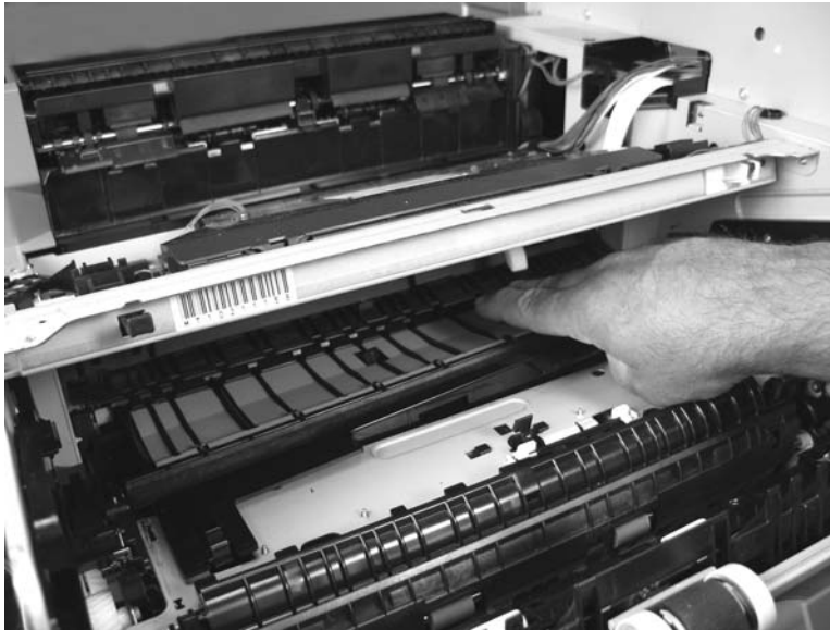
Figure 5-244 Reinstall the paper feed assembly (6 of 8)
