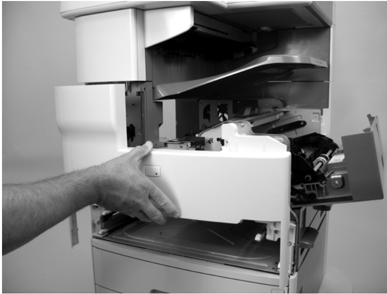
Figure 5-191 Remove the base unit front cover (7 of 7)
