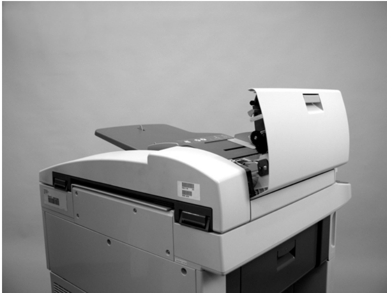
Figure 5-50 Remove the ADF jam cover (1 of 3)
