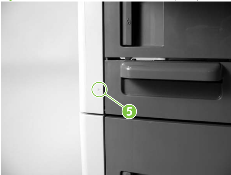
Figure 5-190 Remove the base unit front cover (6 of 7)
