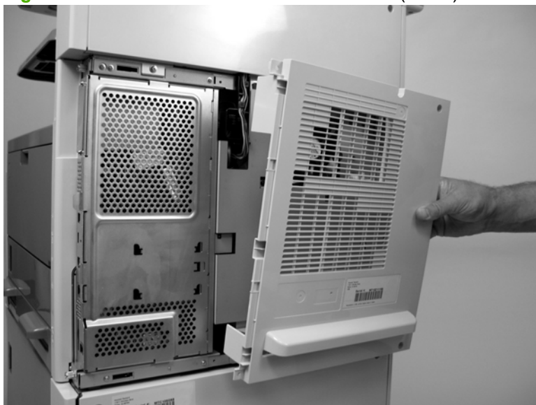
Figure 5-184 Remove the base unit rear cover (2 of 2)
