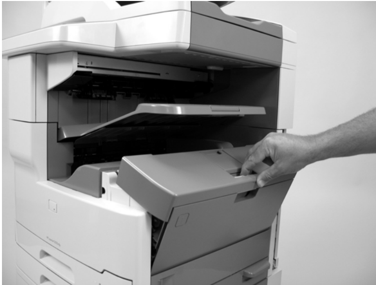
Figure 5-2 Remove the print cartridge (1 of 2)
