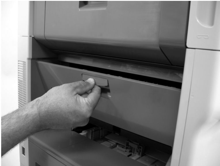
Figure 5-24 Remove the fuser (2 of 6)
