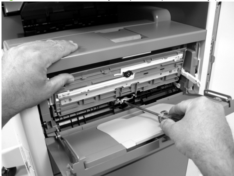
Figure 5-14 Remove the Tray 1 separation pad assembly (2 of 3)
