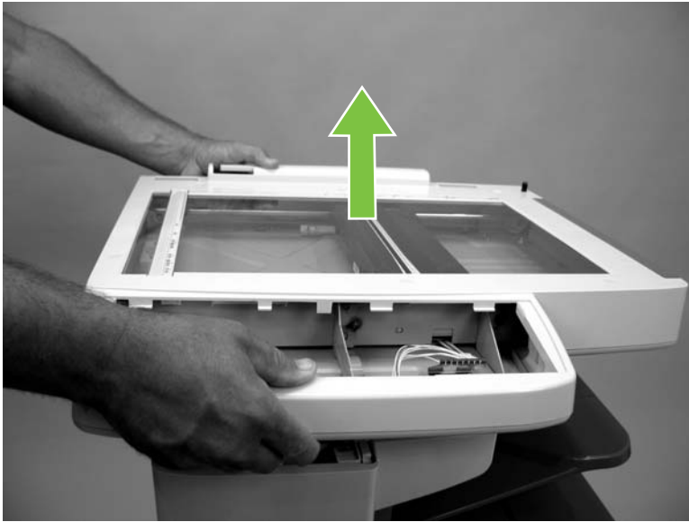
Figure 5-88 Remove the scanner (4 of 4)
