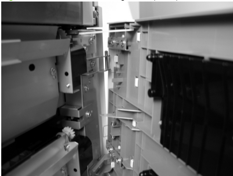
Figure 5-301 Remove the HCI right door (4 of 5)
