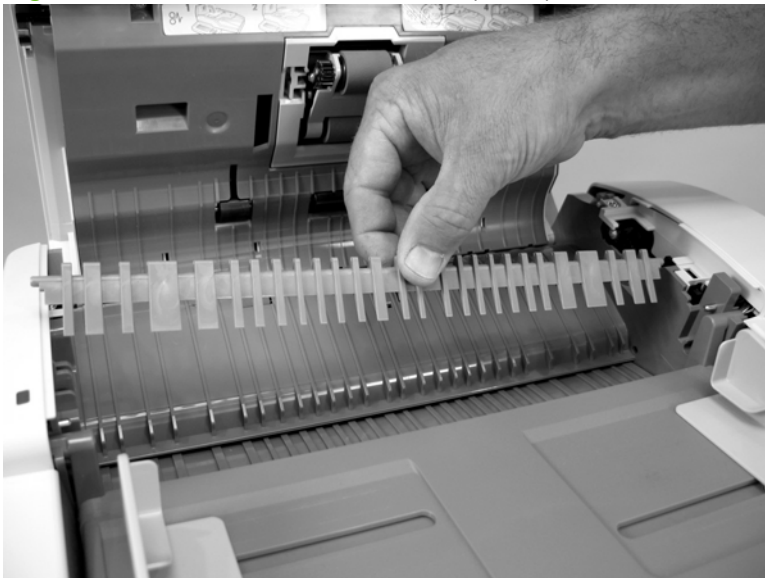
Figure 5-49 Remove the ADF diverter (2 of 2)
