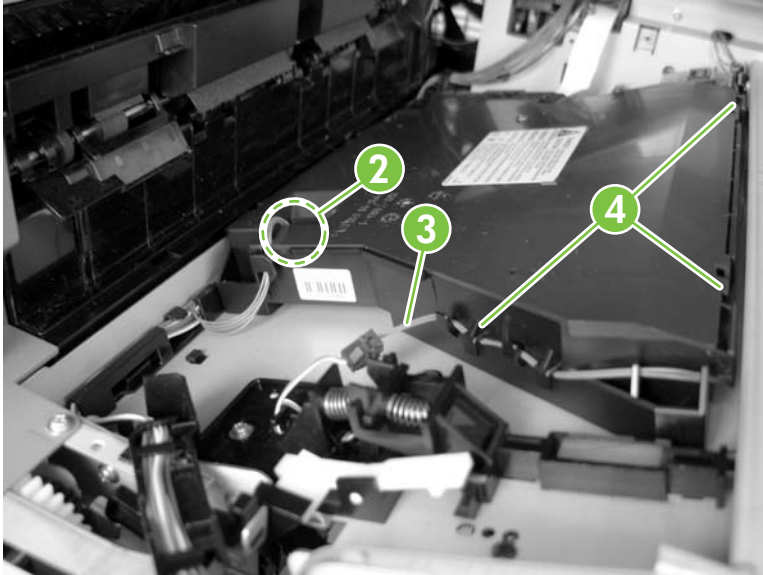
Figure 5-250 Remove the laser/scanner (2 of 3)
