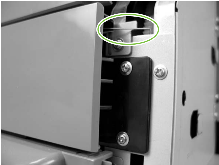
Figure 5-200 Install the base unit right door
