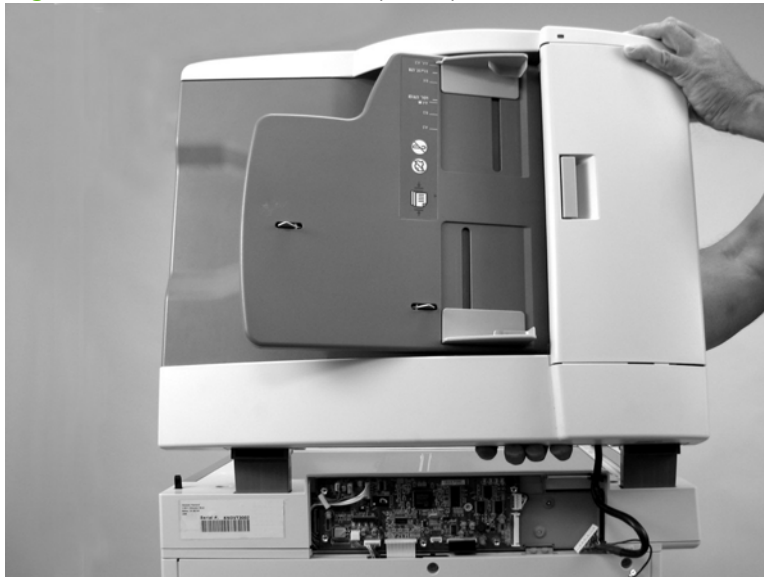
Figure 5-41 Remove the ADF (4 of 4)
