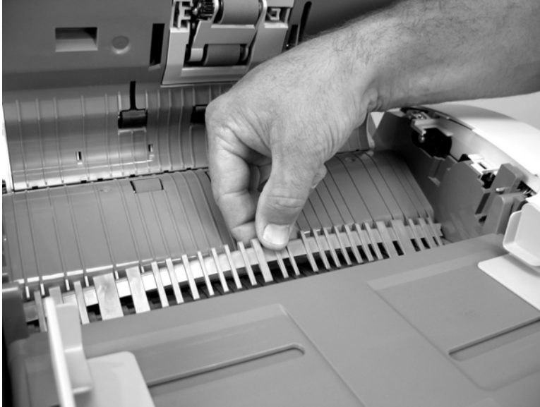
Figure 5-48 Remove the ADF diverter (1 of 2)
