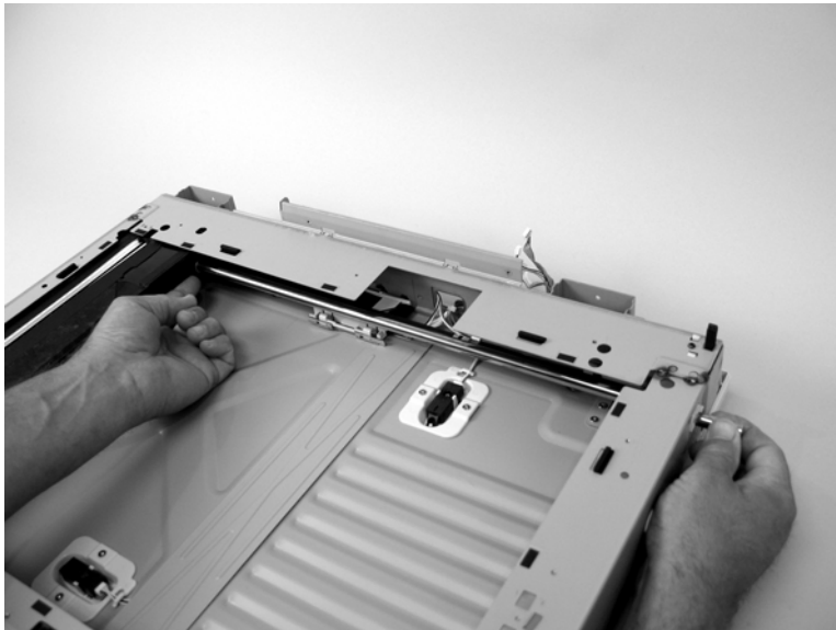
Figure 5-99 Remove the scanner optic assembly (4 of 13)
