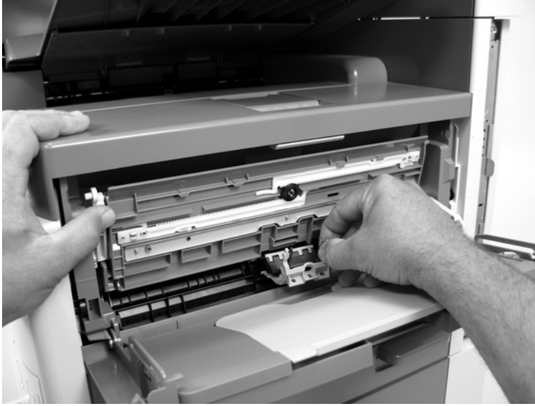
Figure 5-15 Remove the Tray 1 separation pad assembly (3 of 3)
