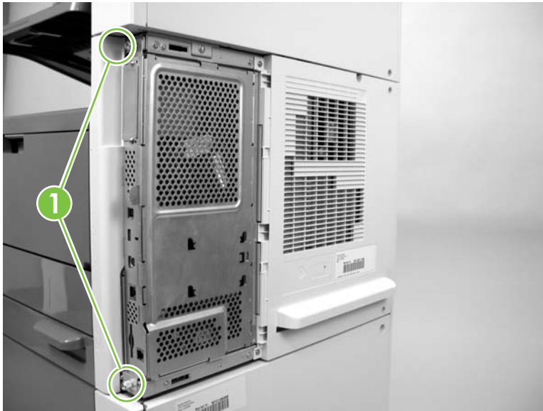
Figure 5-31 Remove the formatter cover and cage (2 of 3)
