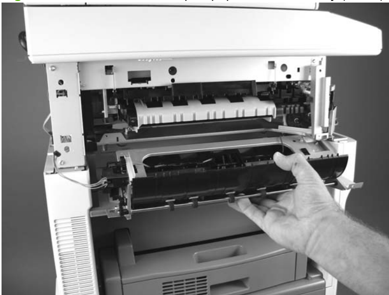
Figure 5-155 Remove the stapler paper feed assembly (3 of 3)
