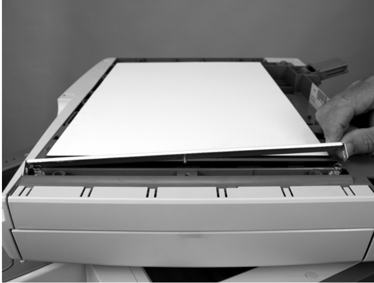
Figure 5-56 Remove the ADF float assembly (3 of 5)
