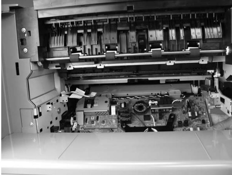
Figure 5-268 Reinstall the high-voltage power supply assembly (1 of 3)
