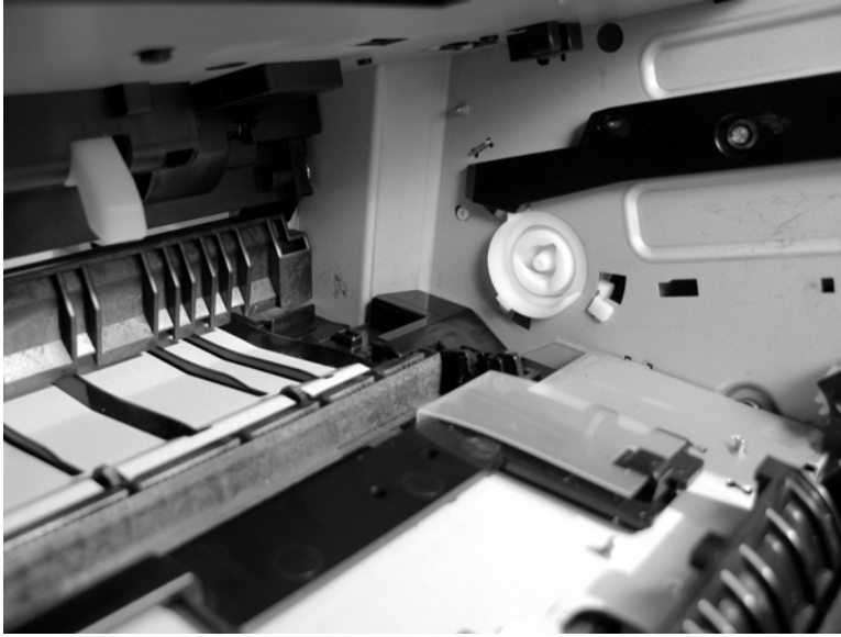
Figure 5-246 Reinstall the paper feed assembly (8 of 8)
