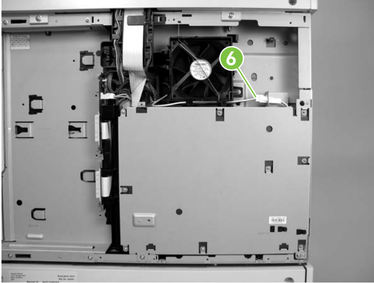
Figure 5-253 Remove the low-voltage power supply assembly (2 of 4)
