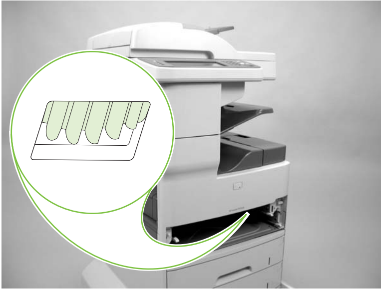
Figure 5-270 Reinstall the high-voltage power supply assembly (3 of 3)
