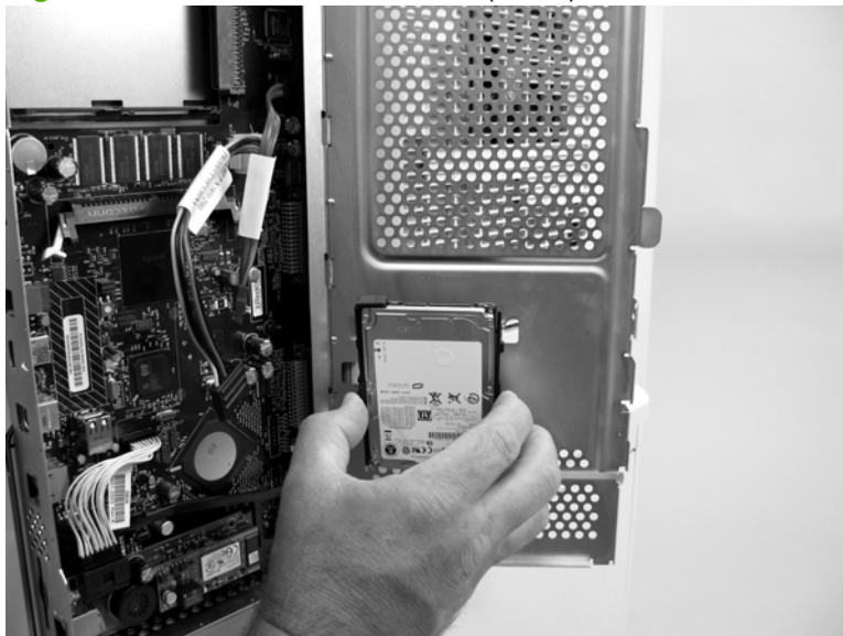
Figure 5-35 Remove the hard drive (2 of 2)
