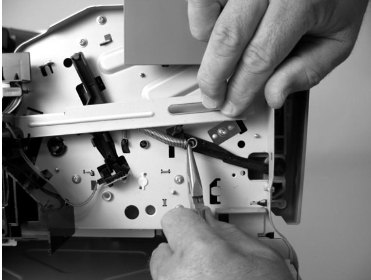
Figure 5-218 Remove the print cartridge door (4 of 12)
