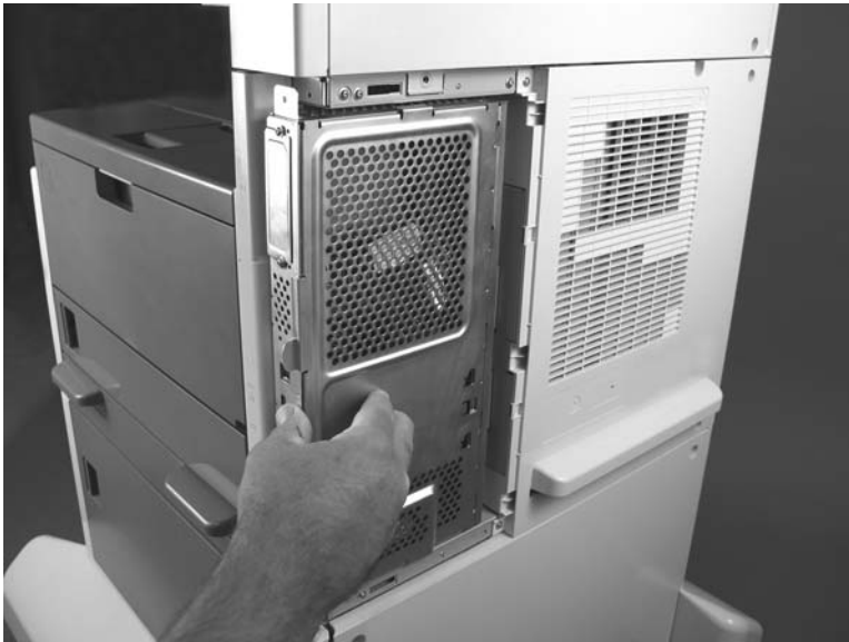
Figure 5-33 Reinstall the formatter cage
