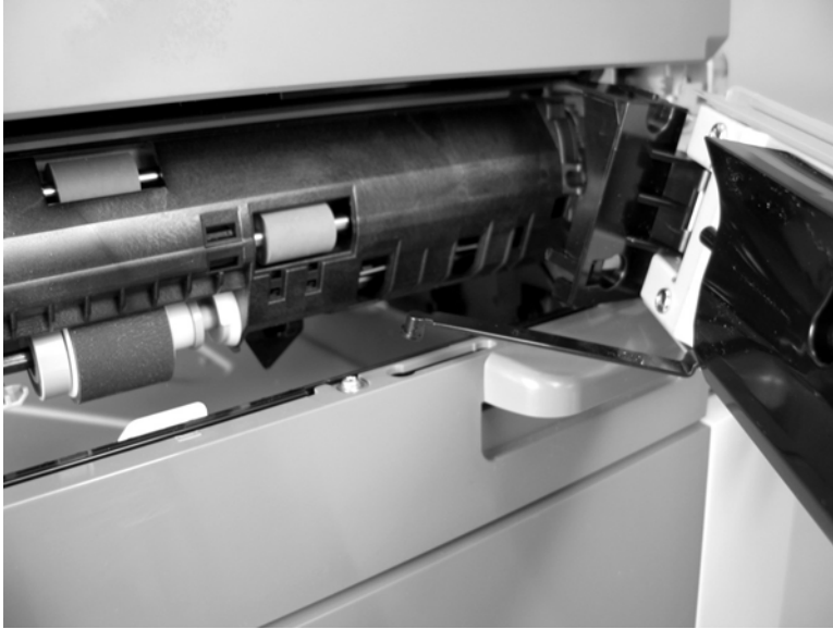
Figure 5-199 Remove the base unit right door (2 of 2)
