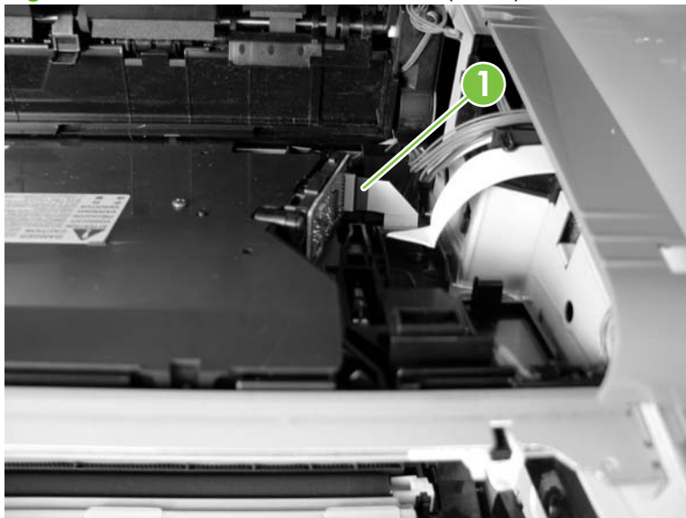
Figure 5-249 Remove the laser/scanner (1 of 3)
