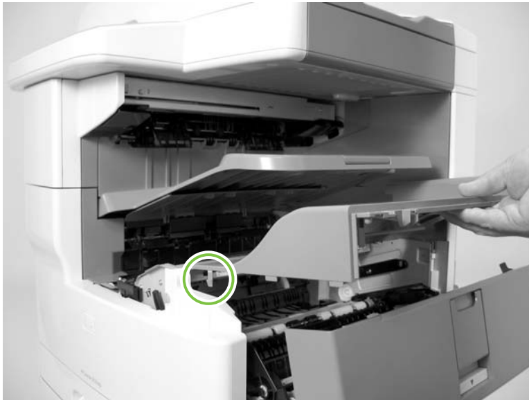
Figure 5-177 Remove the base unit face-down cover (2 of 2)
