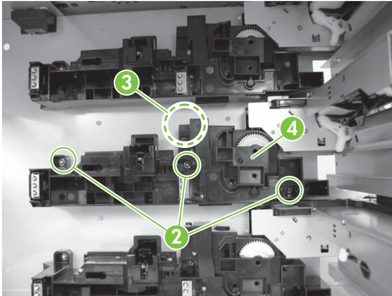
Figure 5-319 Remove the HCI lifter driver assembly (2 of 2)
