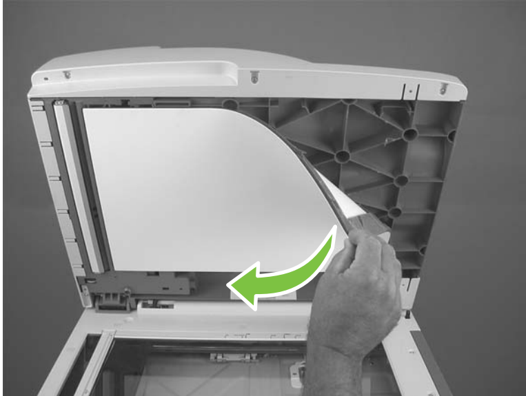
Figure 5-59 Remove the ADF white backing (1 of 4)
