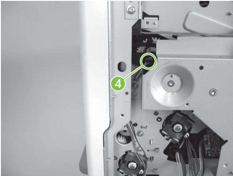
Figure 5-285 Remove the main motor (4 of 7)
