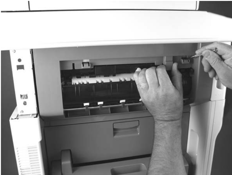
Figure 5-134 Remove the stapler left cover (1 of 3)
