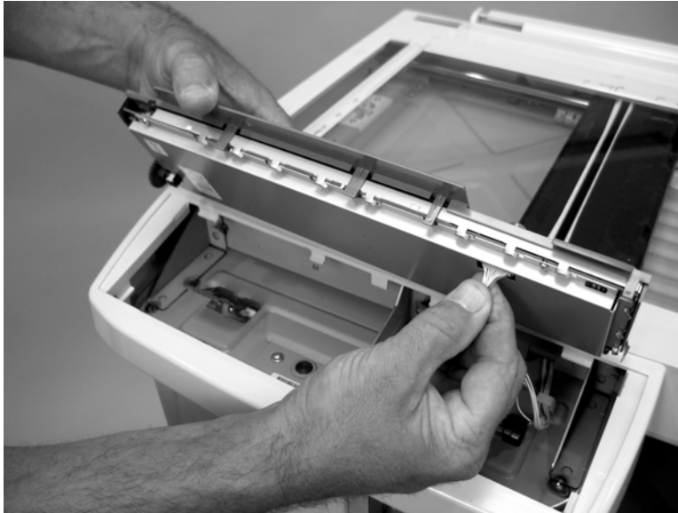
Figure 5-80 Remove the control panel (3 of 3)
