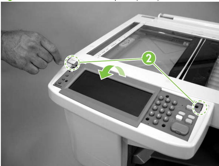
Figure 5-79 Remove the control panel (2 of 3)
