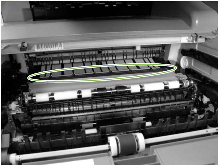
Figure 5-10 Remove the transfer roller (2 of 2)
