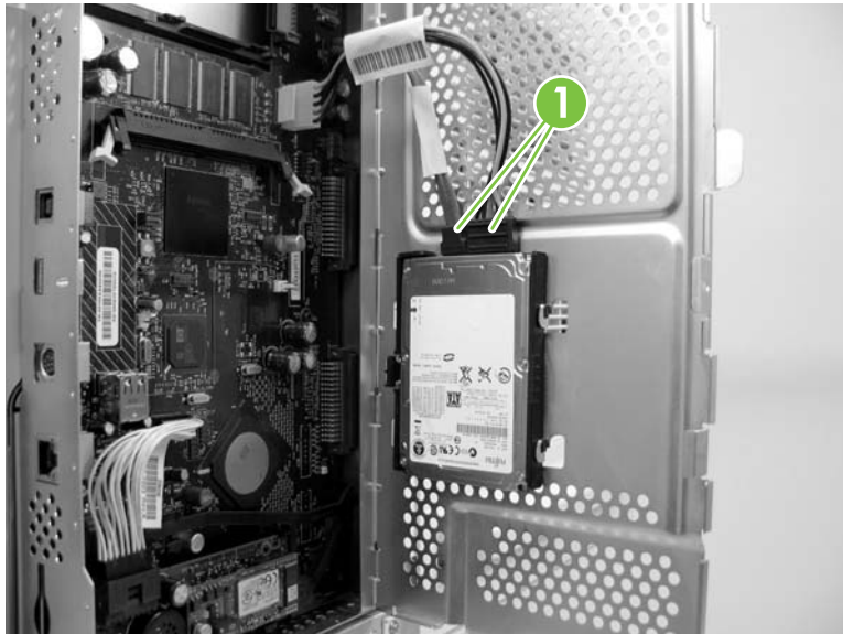
Figure 5-34 Remove the hard drive (1 of 2)
