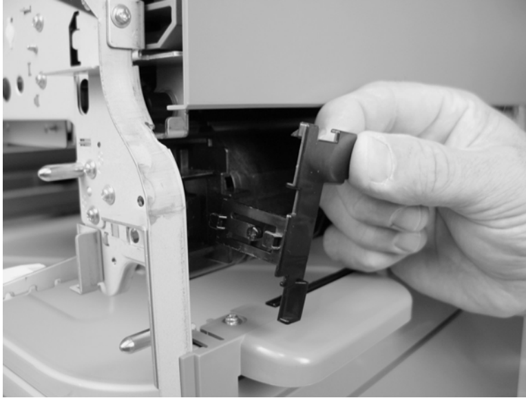
Figure 5-294 Remove the lower cassette pickup assembly (4 of 5)
