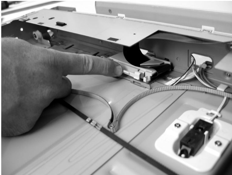
Figure 5-107 Remove the scanner opti assembly (12 of 13)
