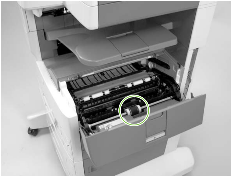
Figure 5-11 Remove the Tray 1 pickup roller (1 of 2)
