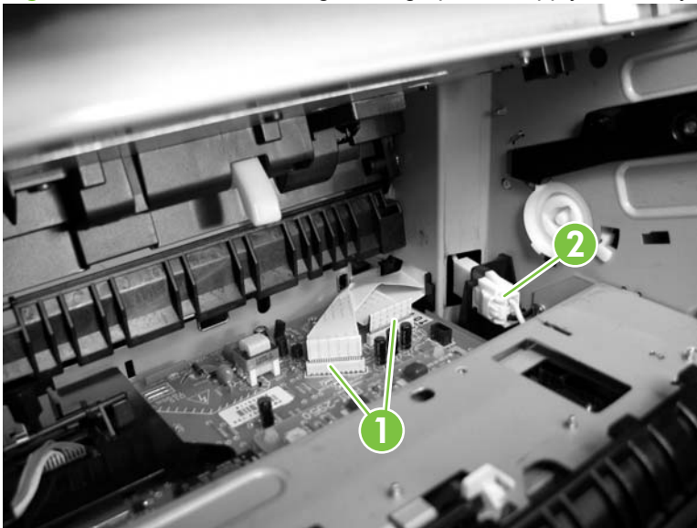
Figure 5-259 Remove the high-voltage power supply assembly (1 of 9)
