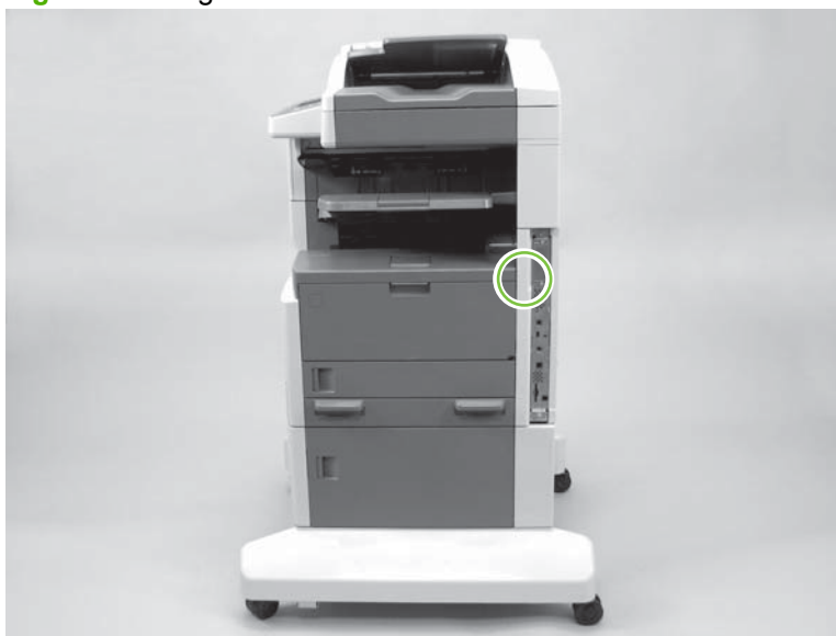
Figure 6-1 Engine test button location
