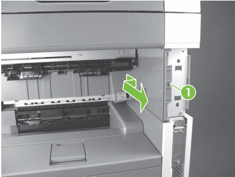
Figure 5-148 Remove the stapler rear inner cover
