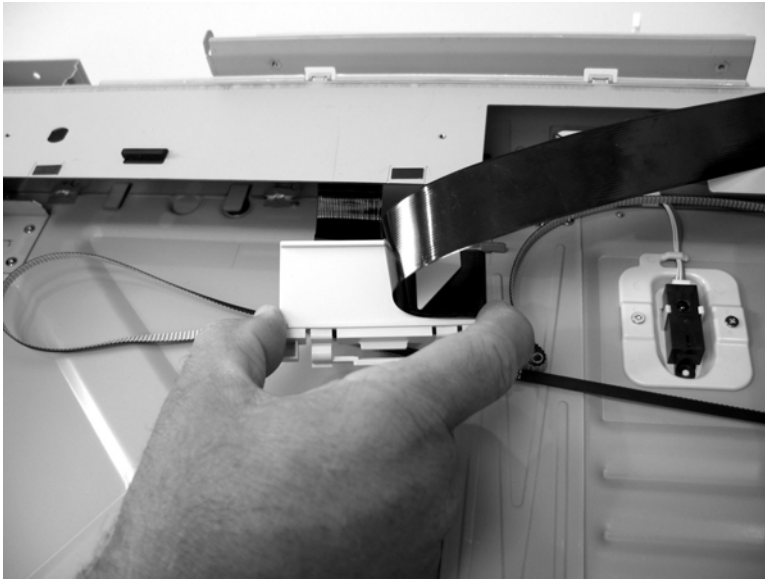
Figure 5-108 Remove the scanner optic assembly (13 of 13)
