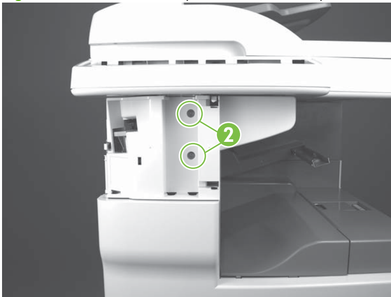
Figure 5-143 Remove the stapler front door and stapler unit cover (4 of 7)
