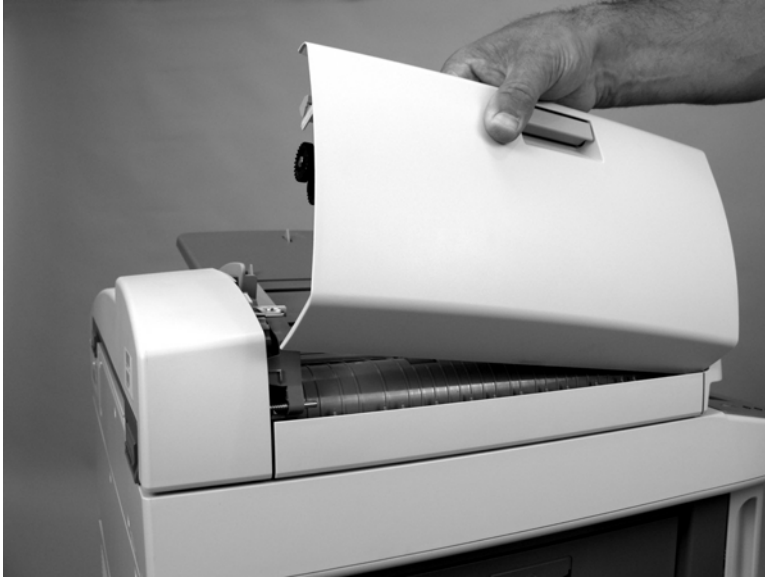
Figure 5-52 Remove the ADF jam cover (3 of 3)
