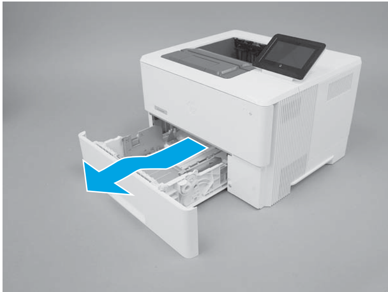
Figure 1-1688 Release and remove the tray
