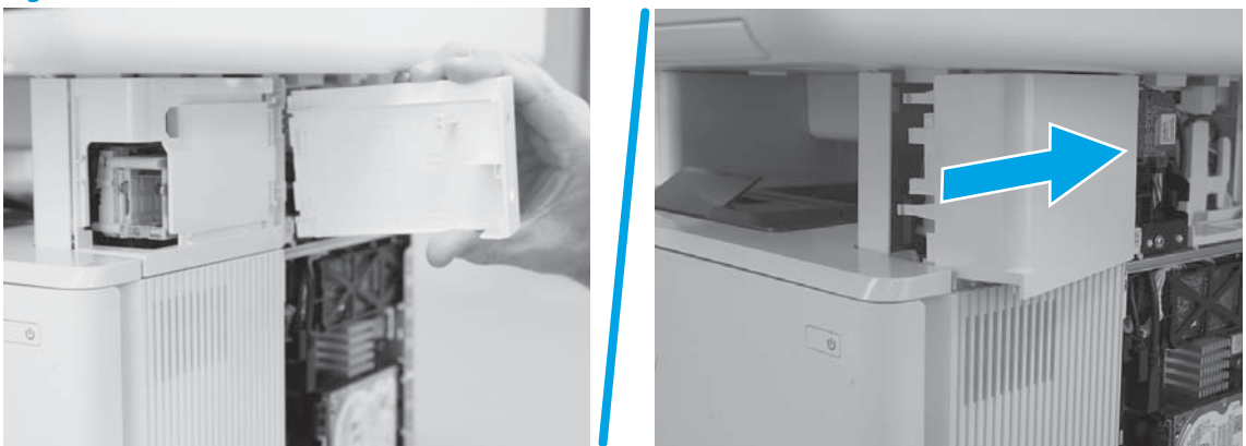
Figure 1-672 Install the door or cover
