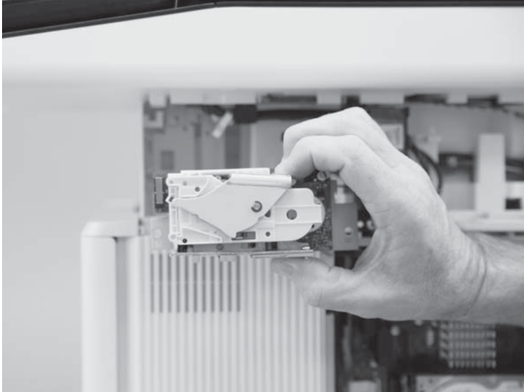
Figure 1-967 Install the stapler unit
