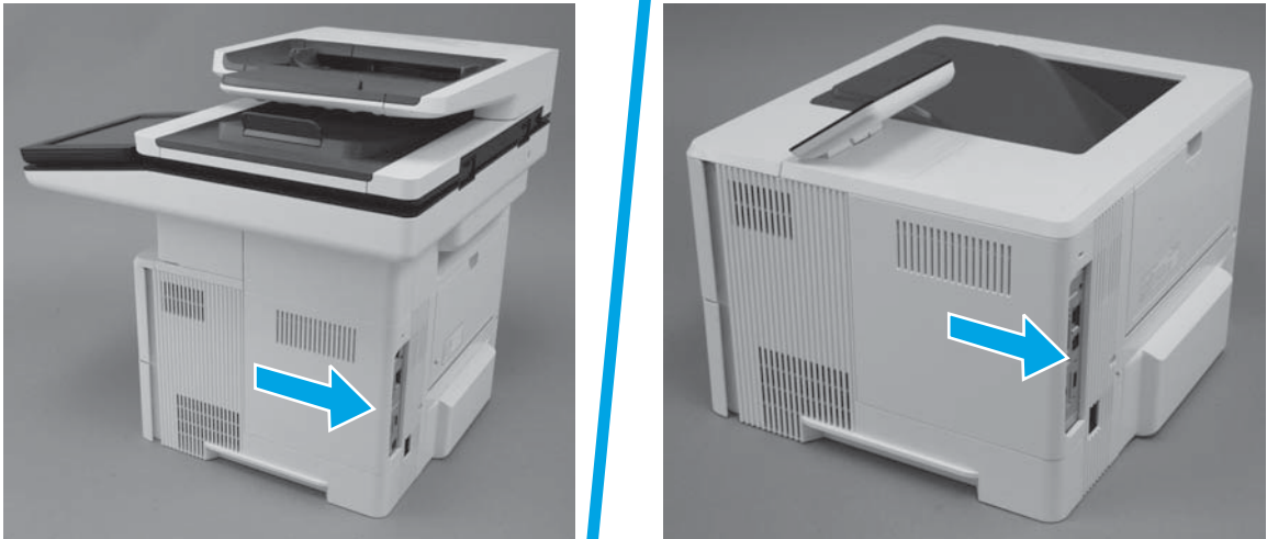
Figure 1-955 Remove the formatter cover
