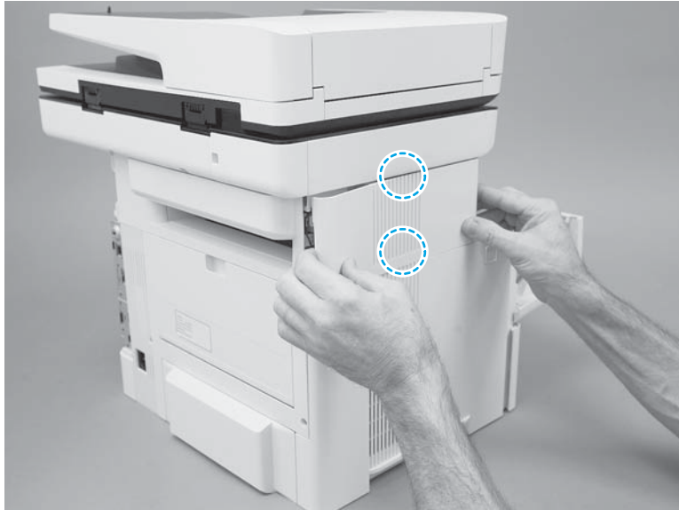
Figure 1-202 Release two tabs
