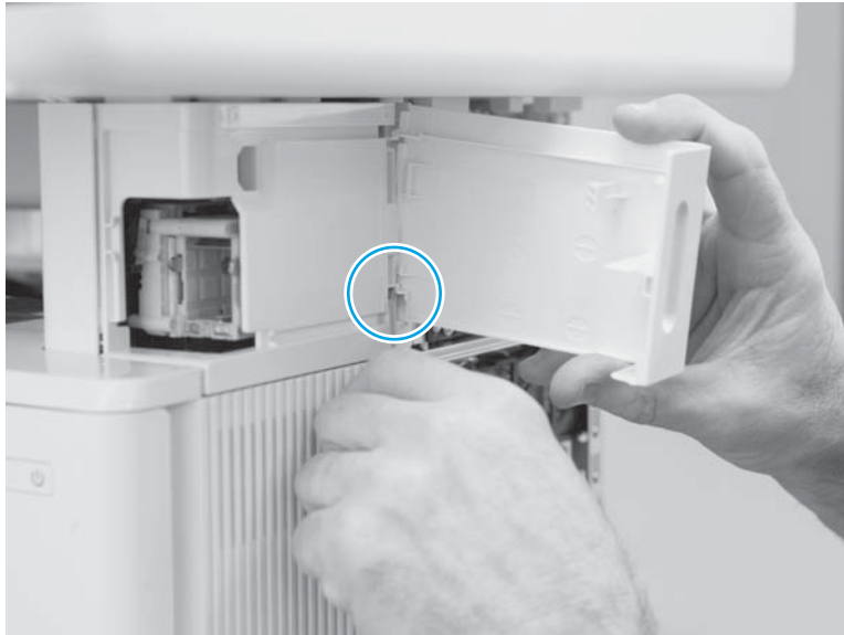
Figure 1-958 Release the lower hinge
