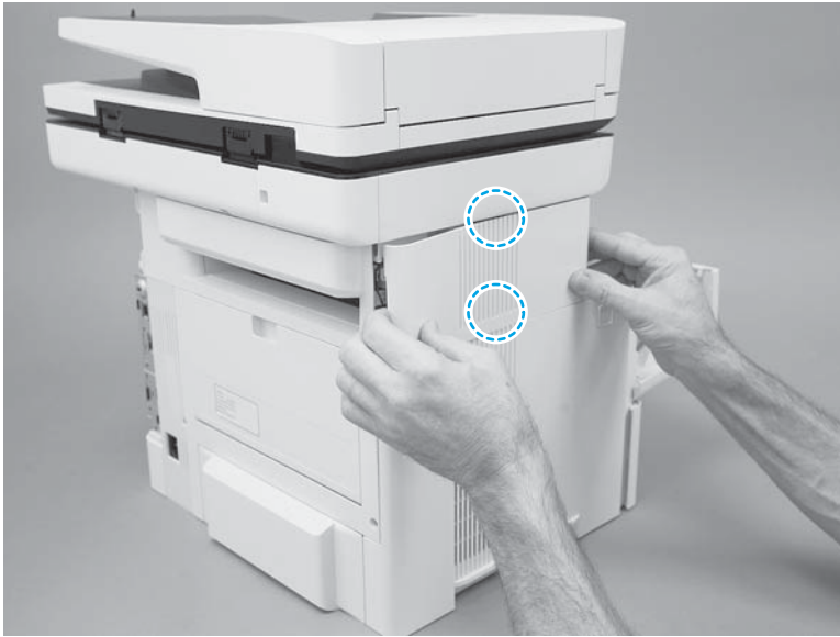
Figure 1-1172 Release two tabs
