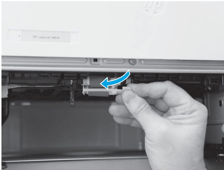
Figure 1-137 Remove the roller assembly
