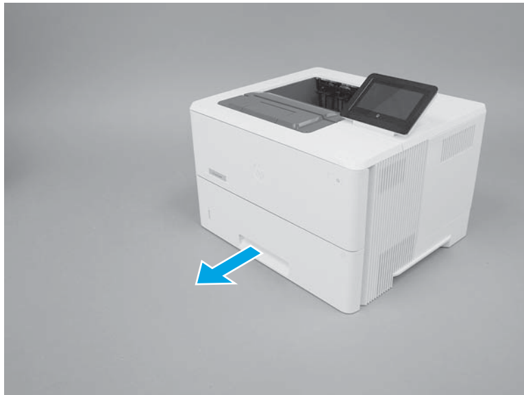
Figure 1-133 Pull the tray out until it stops
