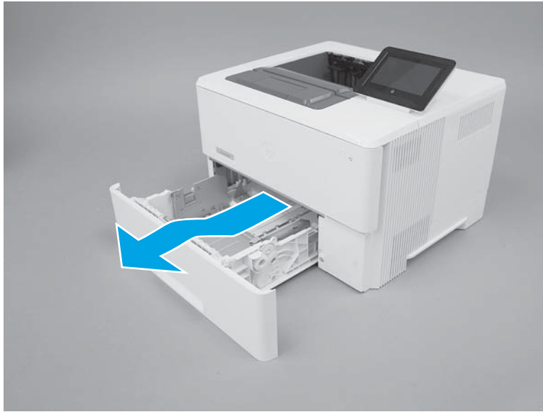
Figure 1-1847 Release and remove the tray
