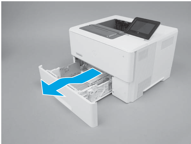
Figure 1-235 Release and remove the tray
