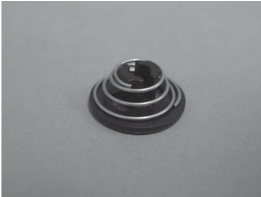
Figure 1-97 Check the retention clip spring
