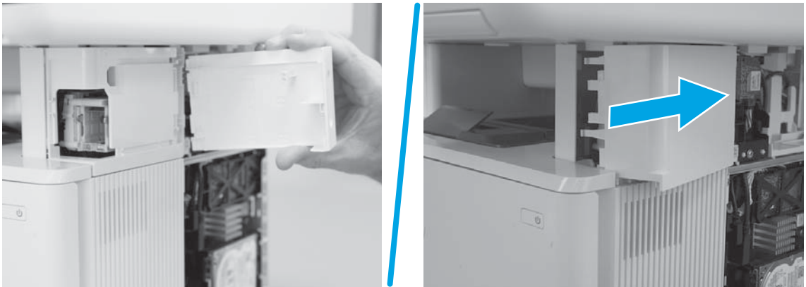
Figure 1-834 Install the door or cover
