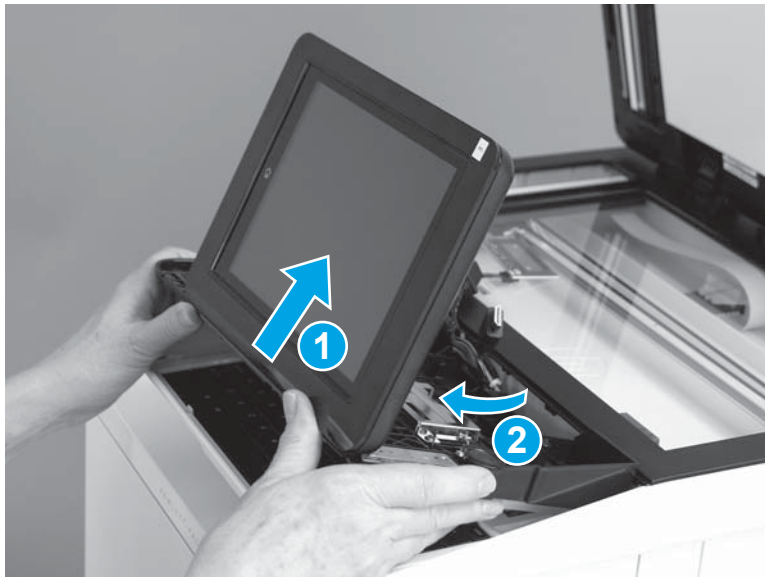
Figure 1-701 Remove the control panel
