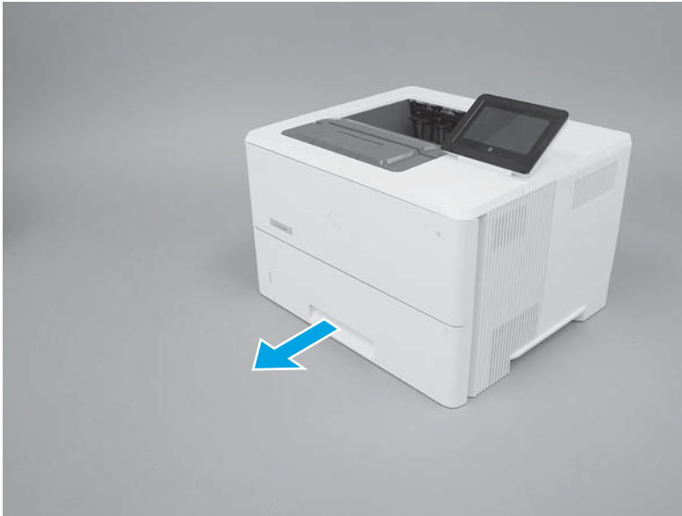
Figure 1-301 Pull the tray out until it stops
