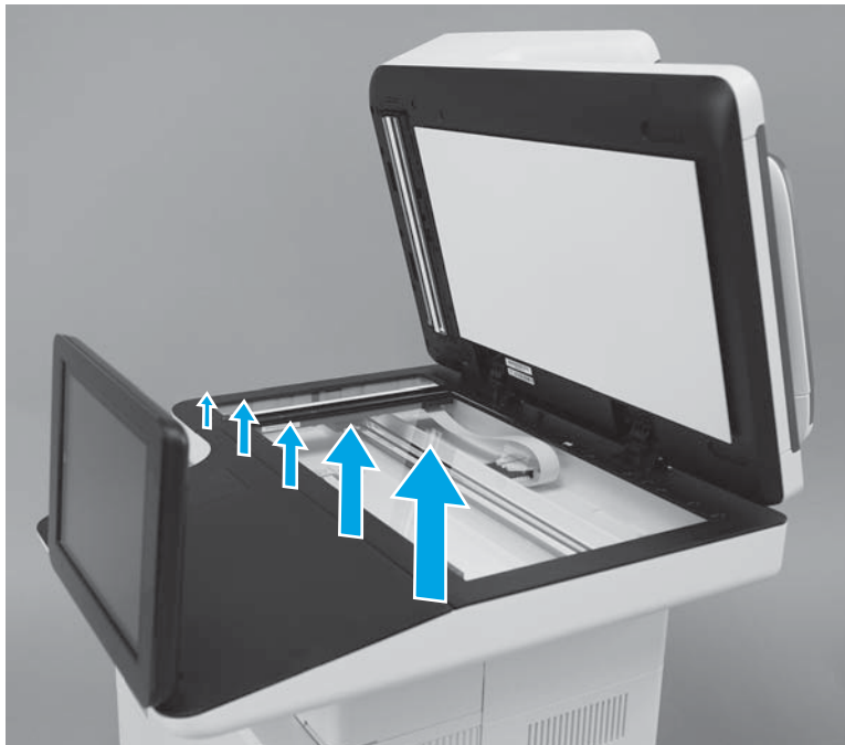
Figure 1-105 Remove the control-panel cover
