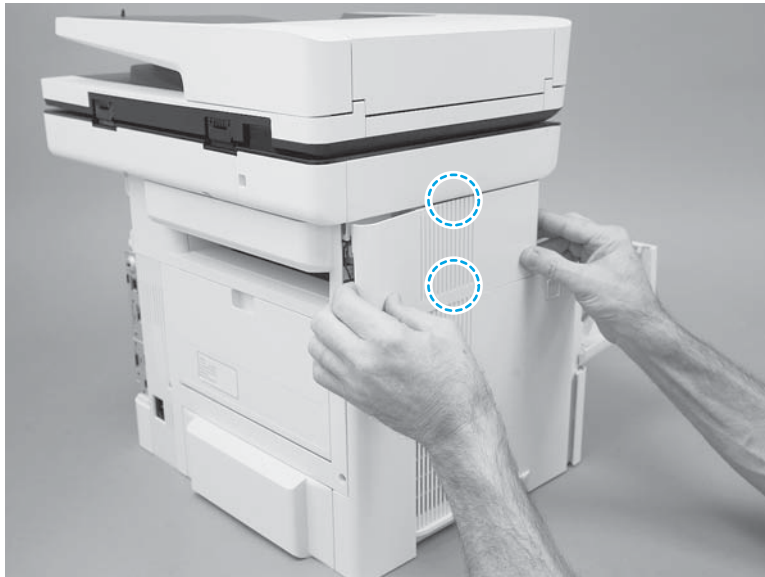
Figure 1-193 Release two tabs
