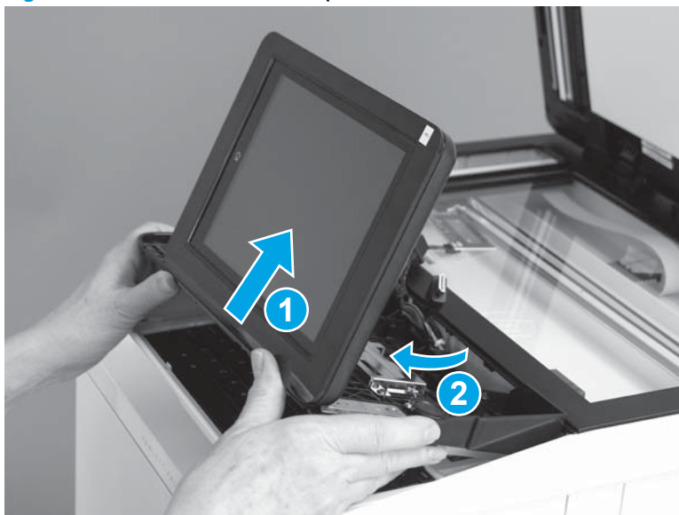
Figure 1-57 Remove the control panel
