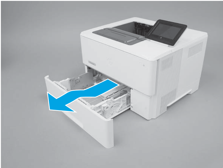
Figure 1-302 Release and remove the tray
