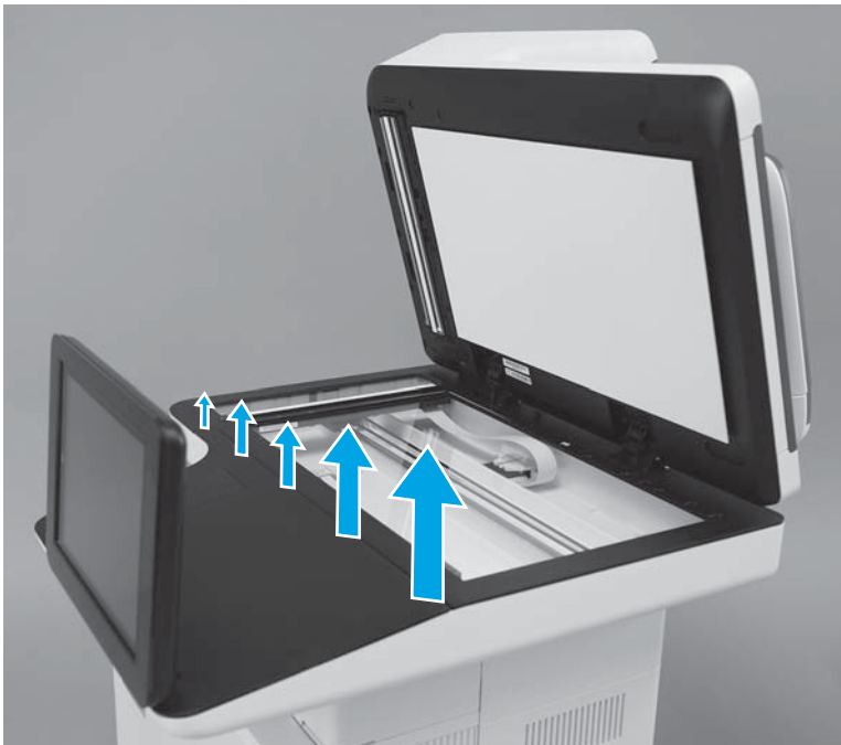
Figure 1-51 Release five tabs
