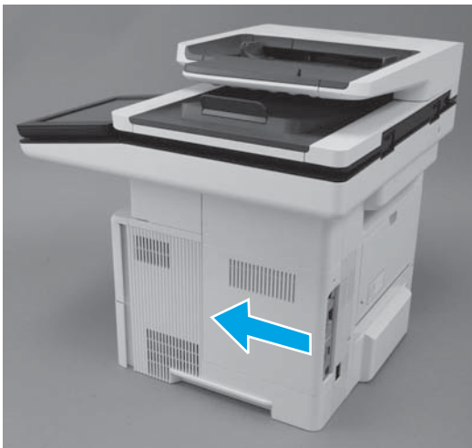
Figure 1-2131 Install the formatter cover
