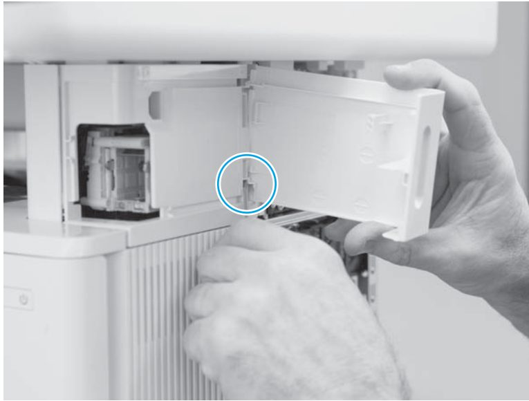
Figure 1-570 Release the lower hinge
