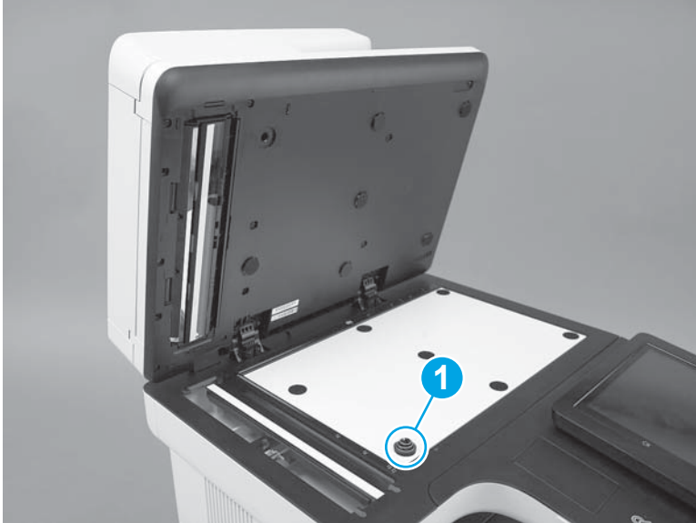
Figure 1-83 Check the retention clips
