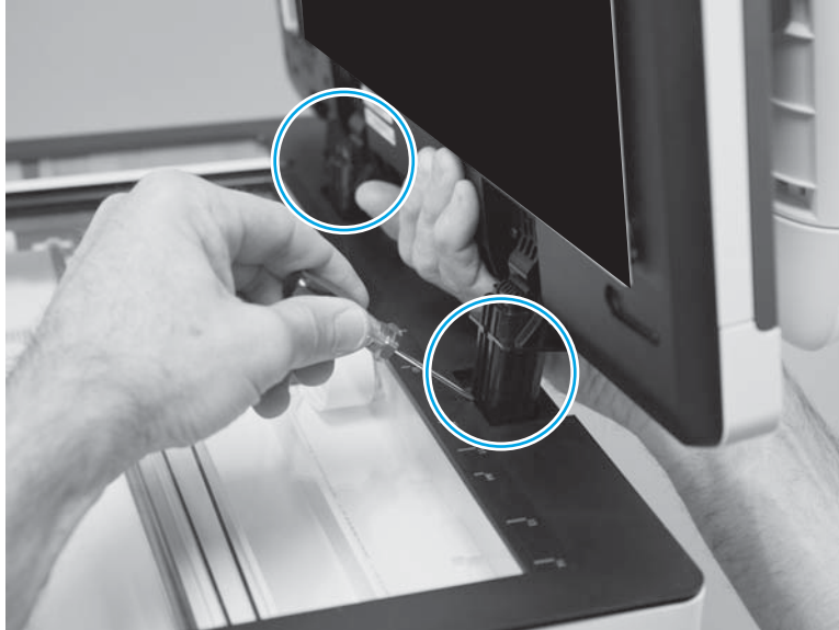
Figure 1-732 Release two tabs
