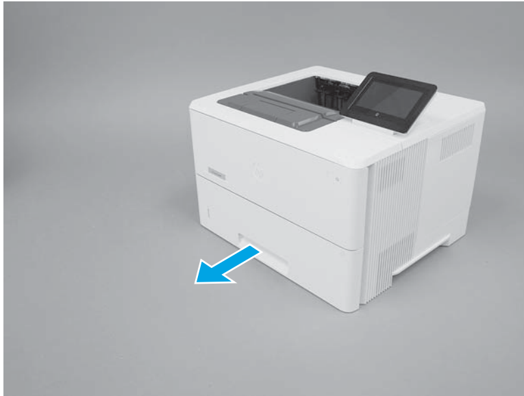
Figure 1-234 Pull the tray out until it stops
