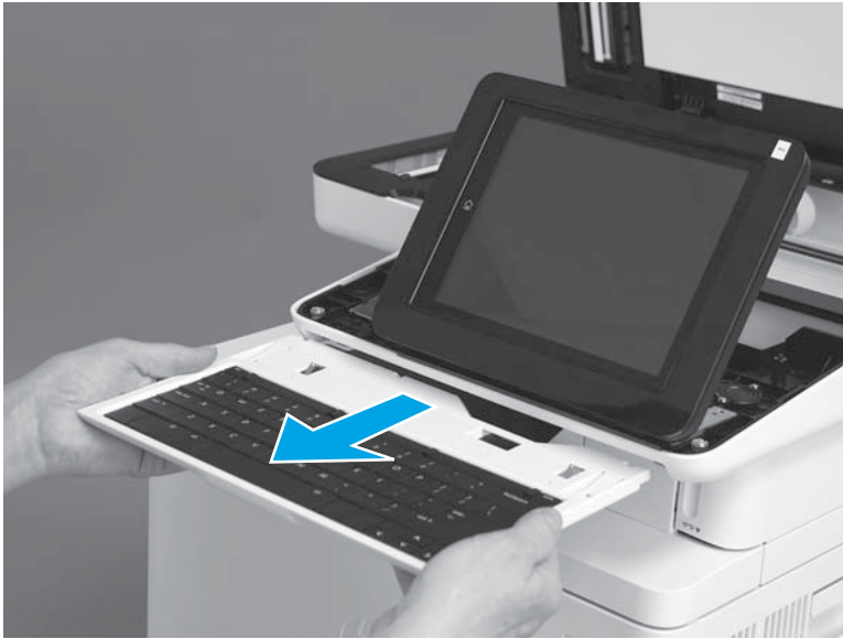
Figure 1-110 Remove the keyboard
