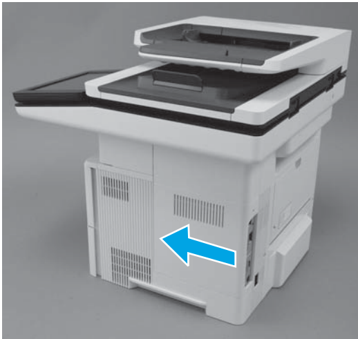
Figure 1-345 Install the formatter cover
