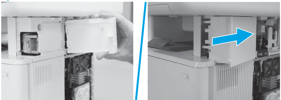
Figure 1-1824 Install the door or cover
