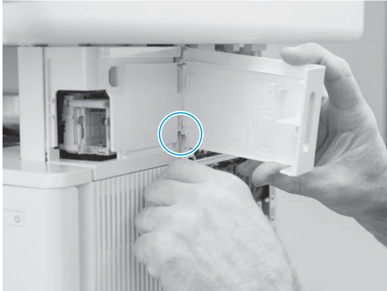
Figure 1-1700 Release the lower hinge
