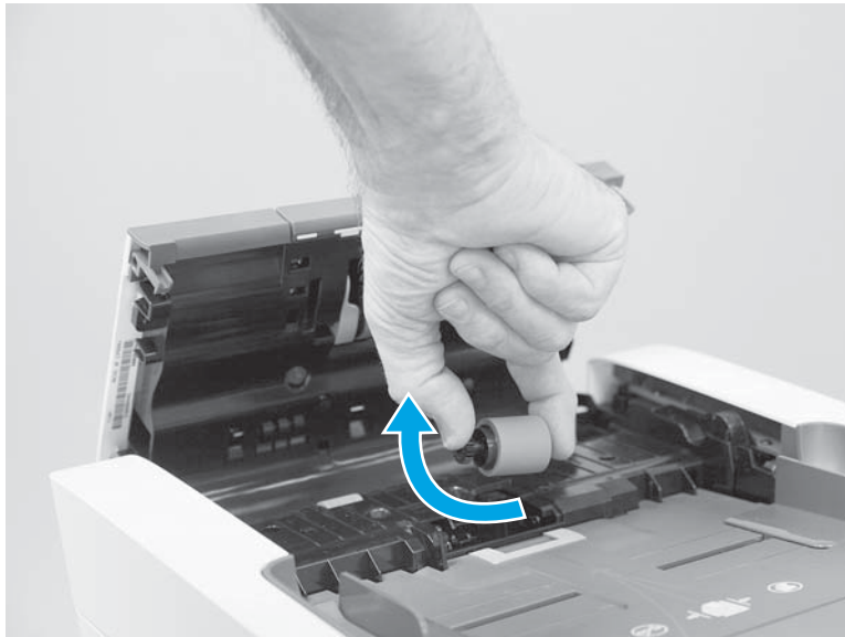
Figure 1-2090 Remove the roller assembly
