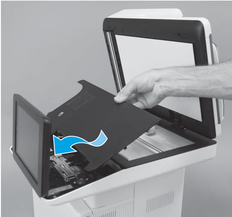
Figure 1-786 Position the control-panel cover on the printer
