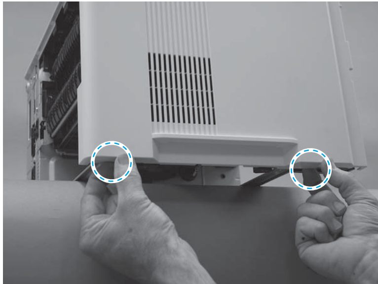
Figure 1-1199 Release two tabs
