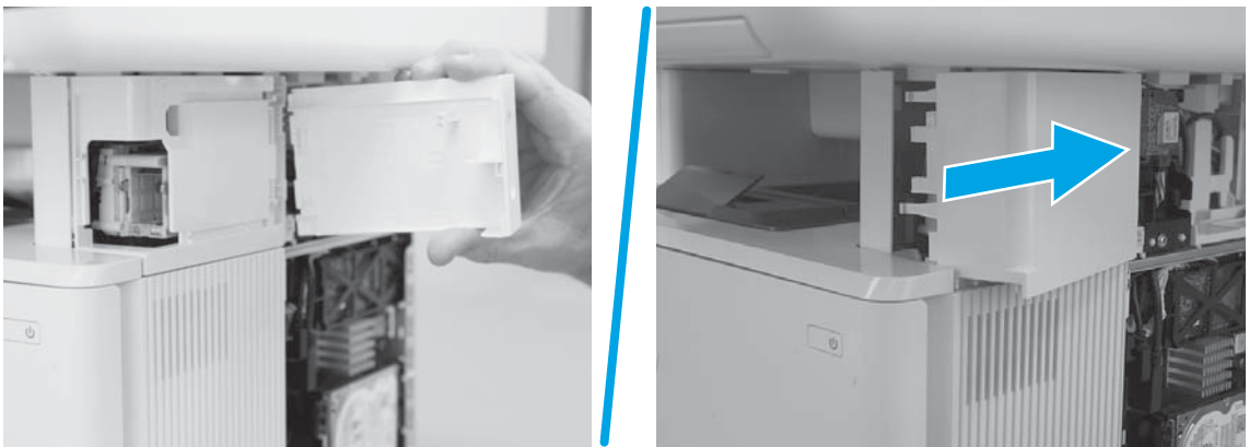
Figure 1-464 Install the door or cover
