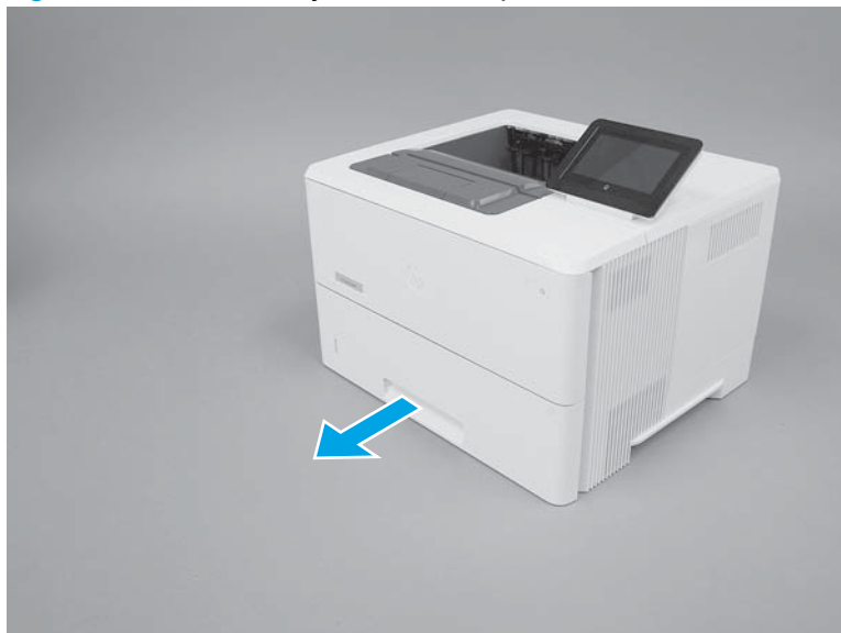
Figure 1-475 Pull the tray out until it stops
