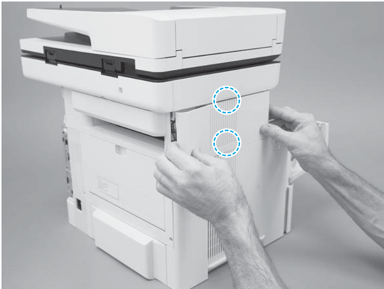
Figure 1-845 Release two tabs
