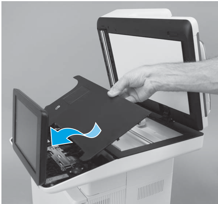
Figure 1-67 Position the control-panel cover on the printer
