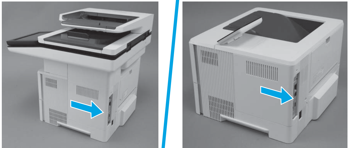
Figure 1-843 Remove the formatter cover
