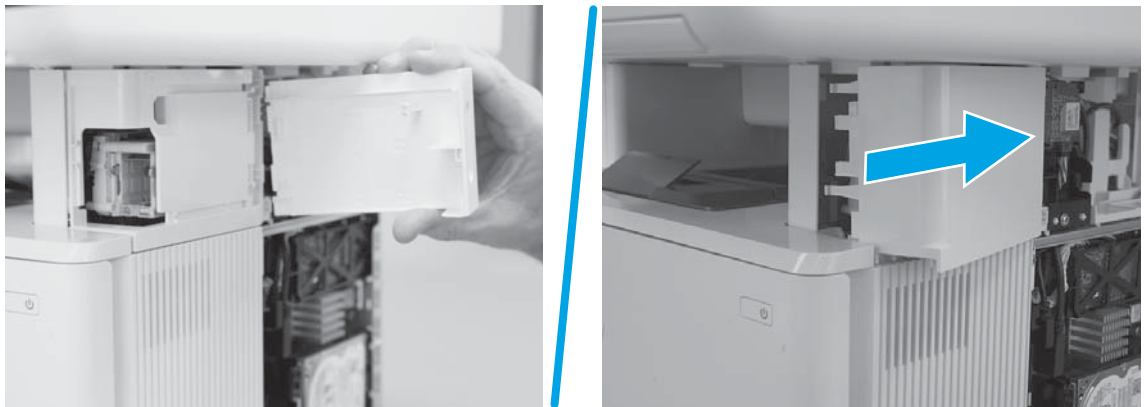
Figure 1-2041 Install the door or cover
