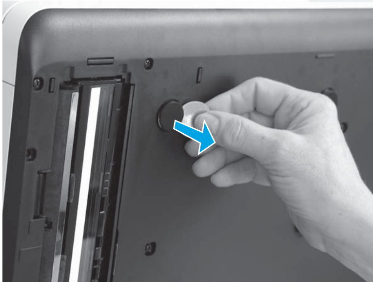
Figure 1-94 Loosen damaged clips
