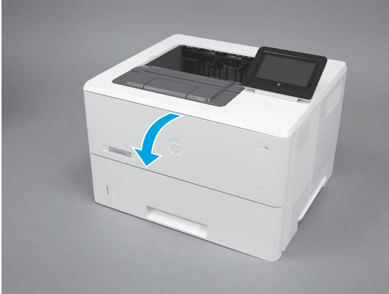
Figure 2-130 Open the toner-cartridge door
