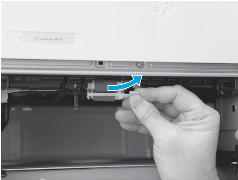
Figure 2-148 Install the roller assembly
