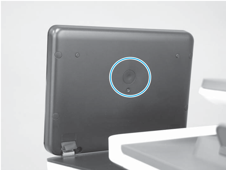
Figure 2-23 Diagnostic-tests access button (M527/E52545/M528/E52645)
