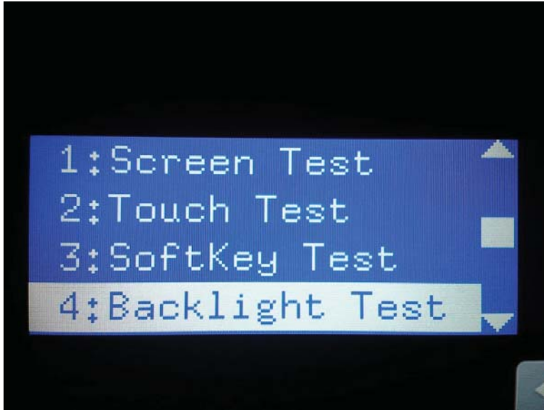
Figure 2-41 Open the backlight test
