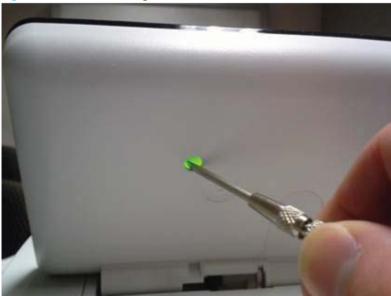
Figure 2-28 Press the diagnostics-access button (M507x and E50145dn)
