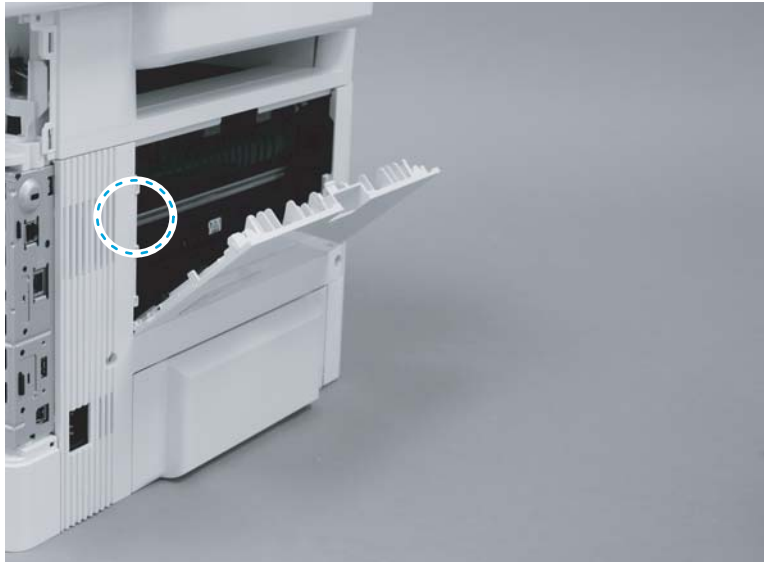
Figure 2-53 Defeat the rear door interlock
