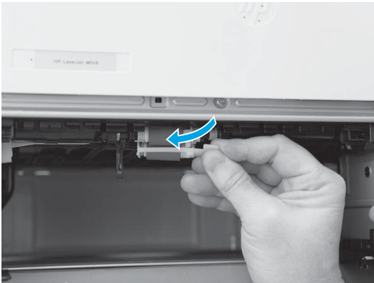
Figure 2-145 Remove the roller assembly
