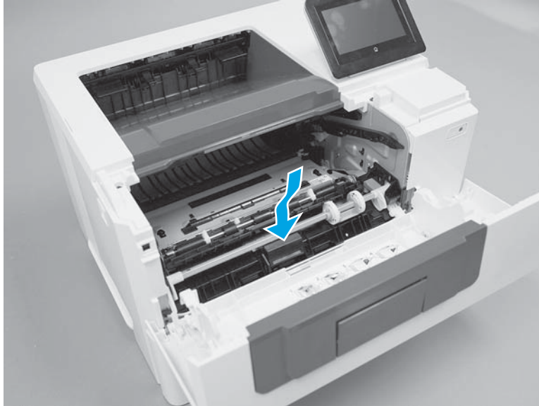
Figure 2-136 Install the pad assembly
