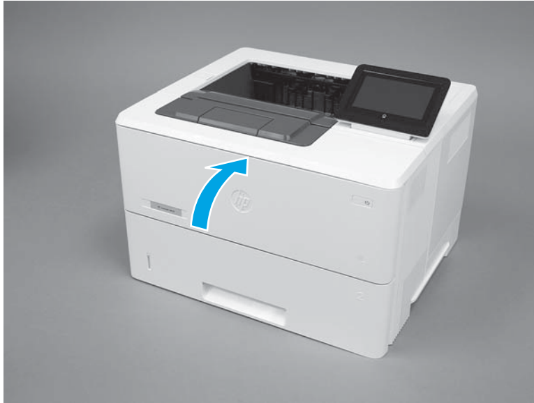
Figure 2-140 Close the toner-cartridge door
