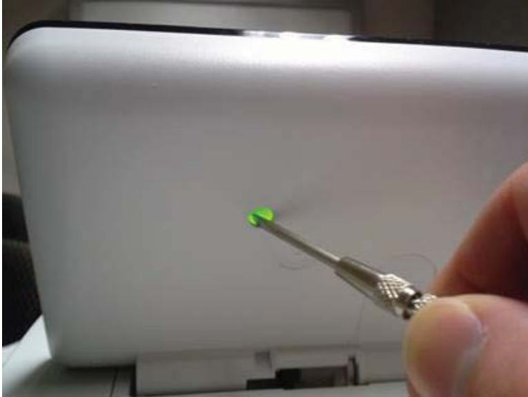
Figure 2-22 Press the diagnostics-access button (M506x)
