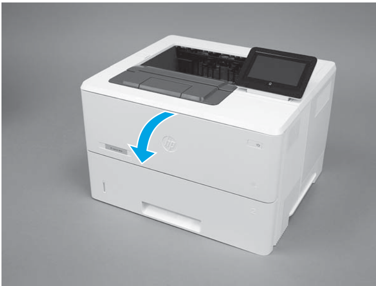
Figure 2-127 Open the toner-cartridge door
