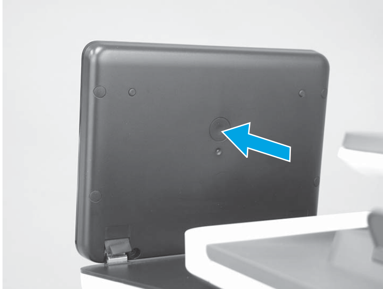
Figure 2-24 Press the diagnostics-access button (M527/E52545/M528/E52645)
