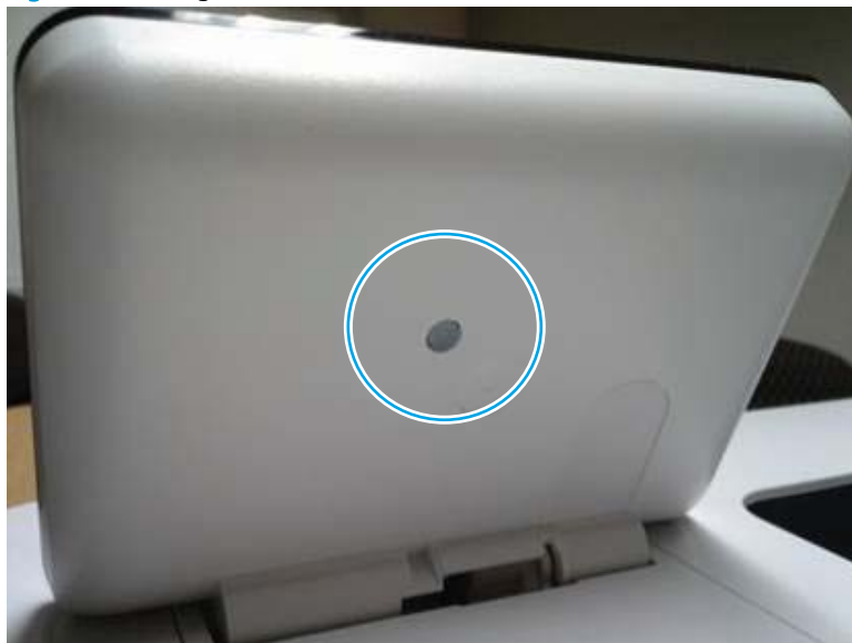
Figure 2-21 Diagnostic-tests access button (M506x)
