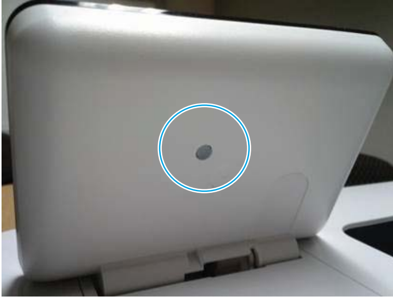
Figure 2-27 Diagnostic-tests access button (M507x and E50145dn)
