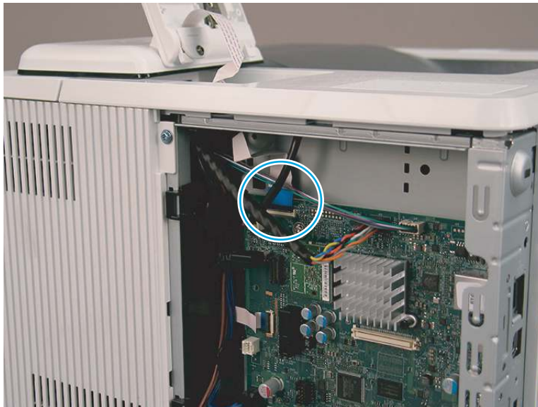
Figure 1-78 Disconnect one FFC (M507/E50145)
