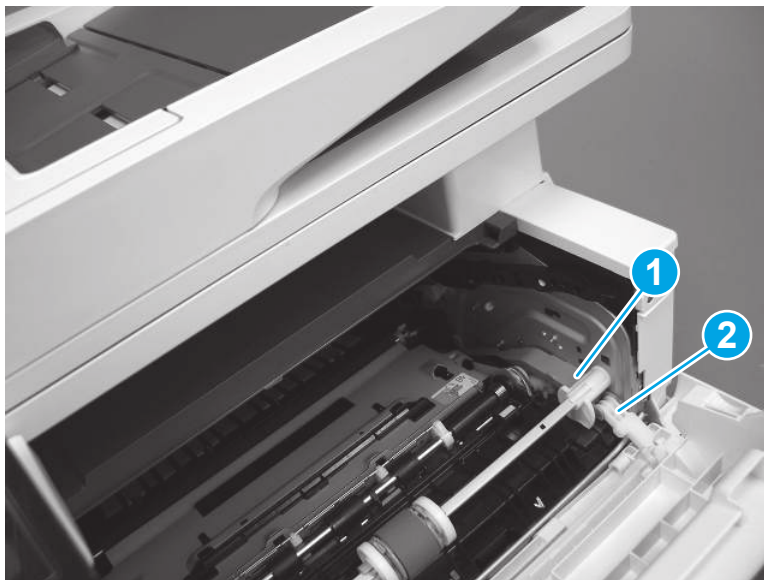
Figure 1-301 Release the pressure-release link
