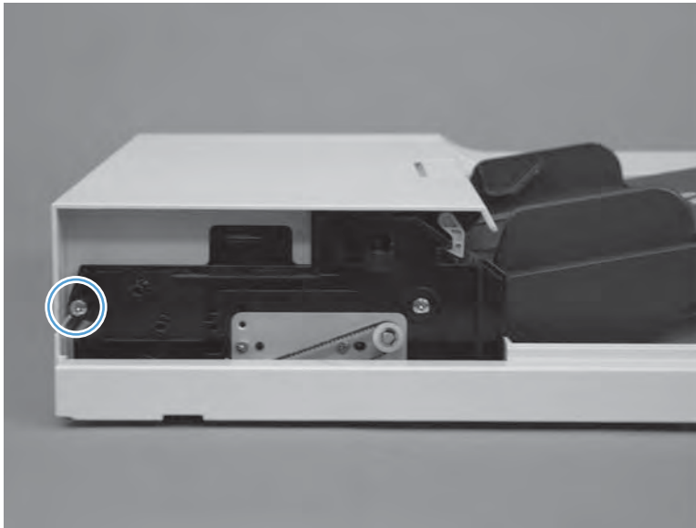
Figure 2-183 Remove the document feeder jam-access cover (1 of 2)
