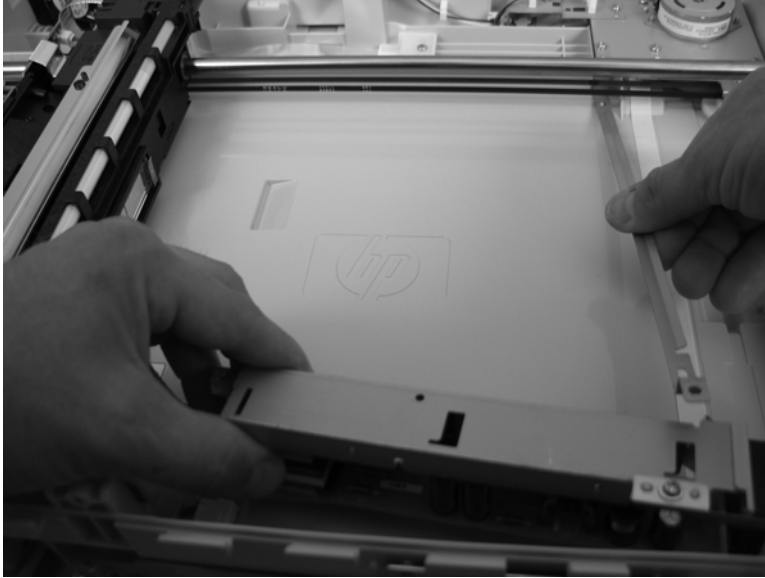
Figure 2-219 Remove the inverter (2 of 2)
