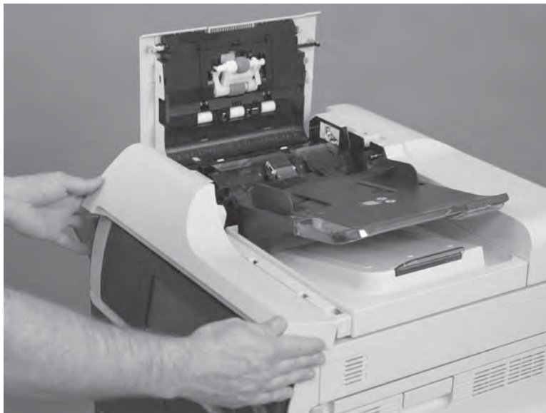
Figure 2-177 Remove document feeder front cover (4 of 4)
