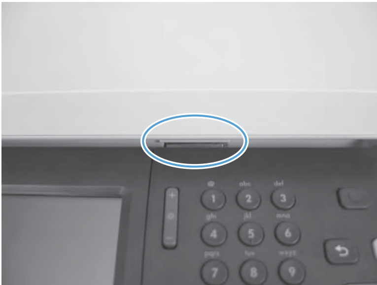
Figure 2-19 Correct installation of the control panel
