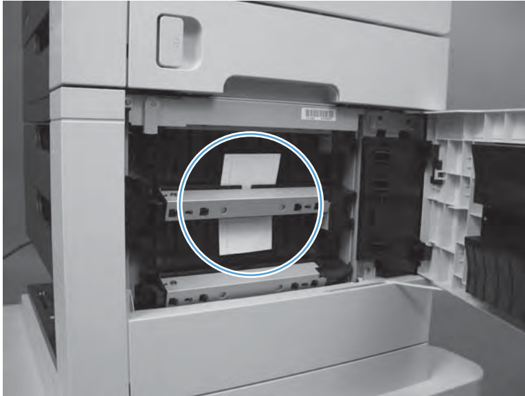
Figure 3-7 Test the SR7 Tray 4 feed sensor
