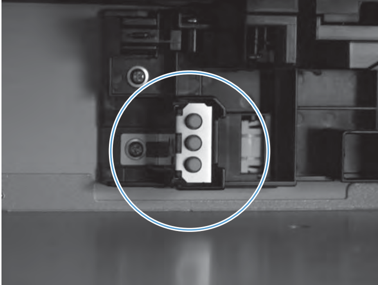
Figure 3-22 Test the SW102 Tray 2 paper size switches
