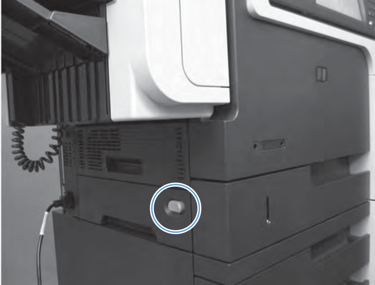
Figure 3-27 Test the SW1 power switch
