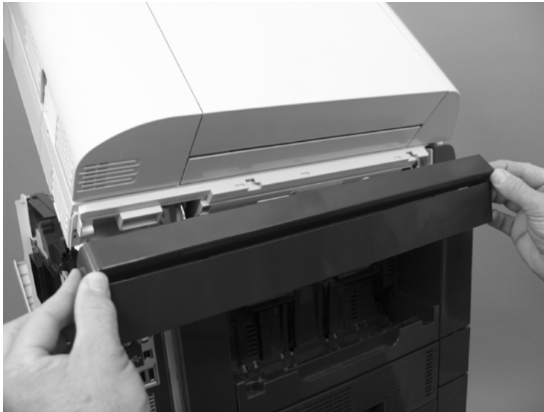
Figure 2-81 Remove the document feeder hinge cover (3 of 3)
