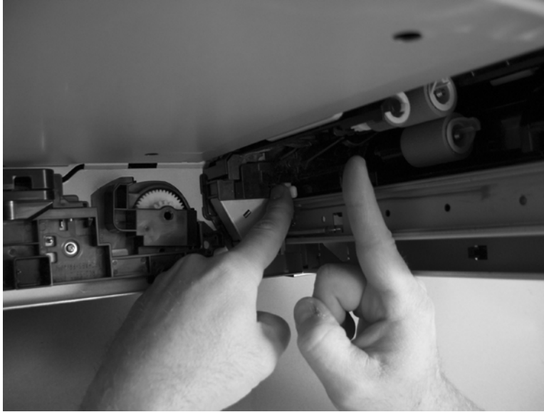
Figure 3-21 Test the PS107/PS907 Tray 2 paper surface sensor
