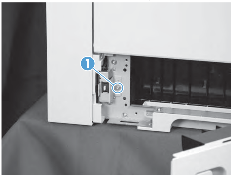
Figure 2-54 Remove the cassette-door-open detection switch (2 of 4)
