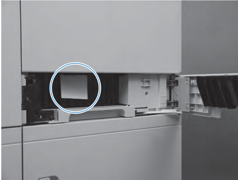
Figure 3-9 Test the PS102 pre-feed sensor
