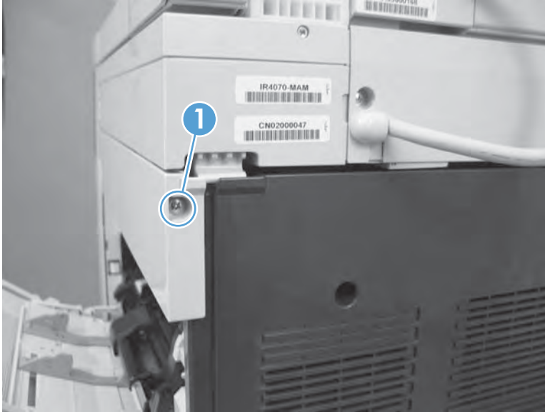
Figure 2-65 Remove the image scanner right cover (1 of 3)
