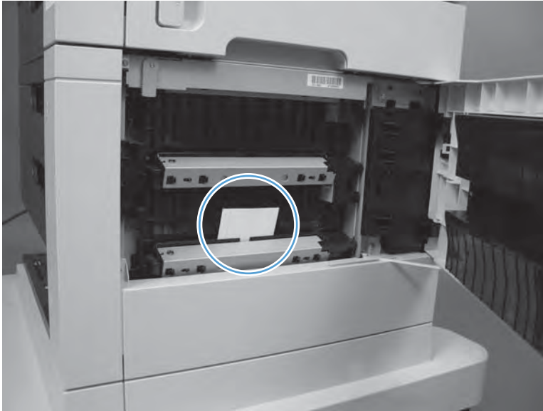
Figure 3-6 Test the SR10 Tray 5 feed sensor
