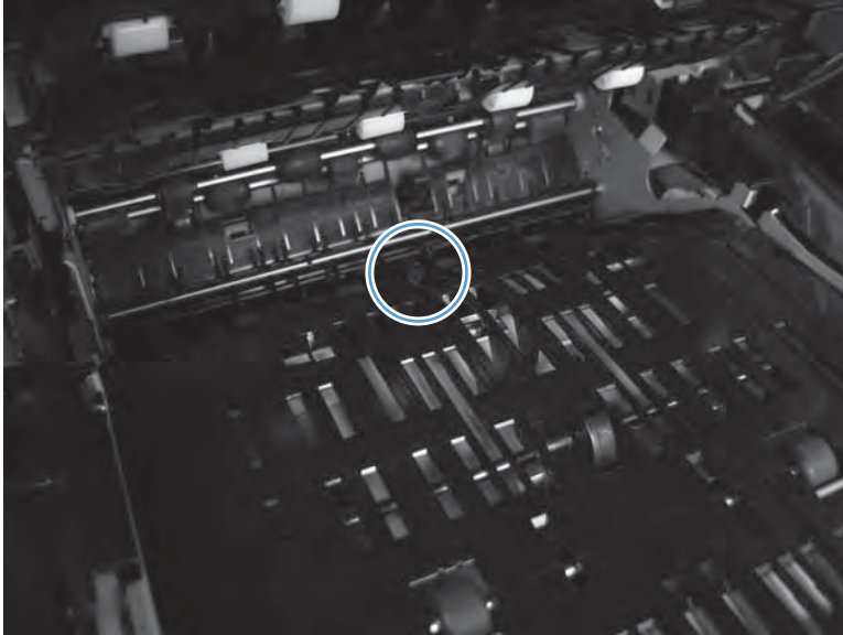
Figure 3-13 Test the PS110 intermediate switchback sensor
