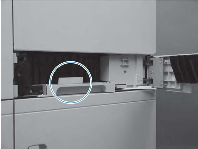
Figure 3-23 Test the SR4 Tray 3 feed sensor
