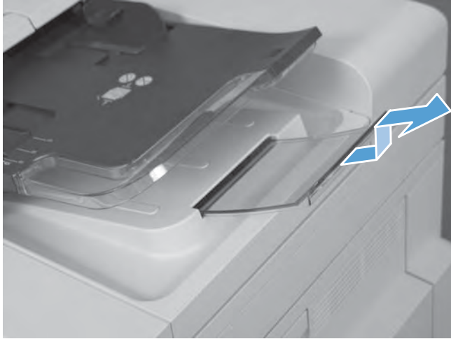
Figure 2-42 Remove the document feeder tray extender
