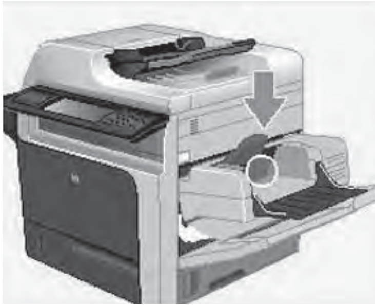
Figure 3-18 Test the PS1802 envelope feeder paper sensor
