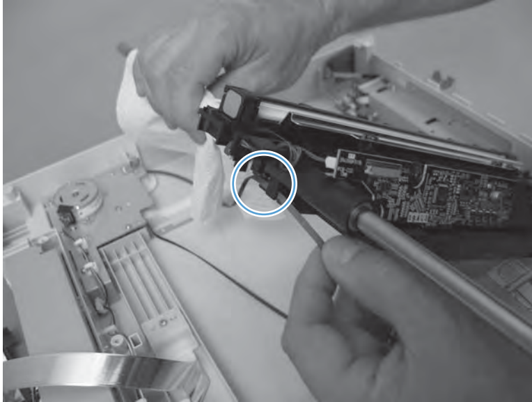
Figure 2-226 Remove the optical assembly (6 of 6)
