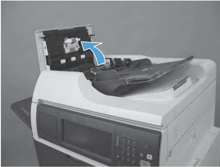
Figure 2-178 Remove the document feeder rear cover (1 of 5)
