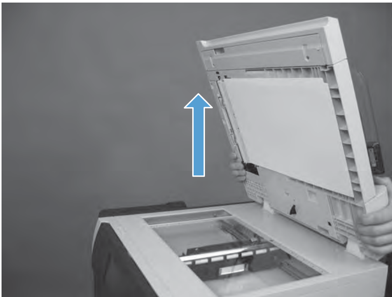
Figure 2-171 Remove the document feeder scanner lid (3 of 3)
