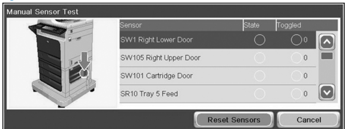
Figure 3-2 Manual Sensor Test screen
