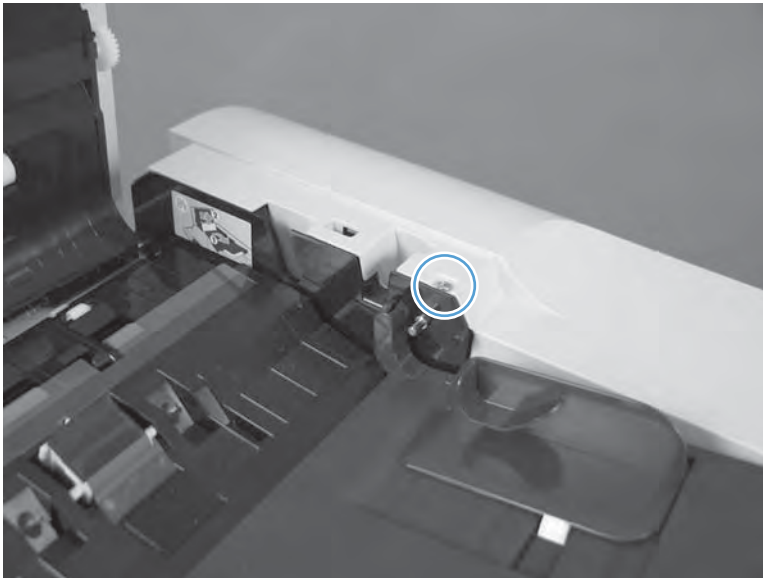
Figure 2-179 Remove the document feeder rear cover (2 of 5)
