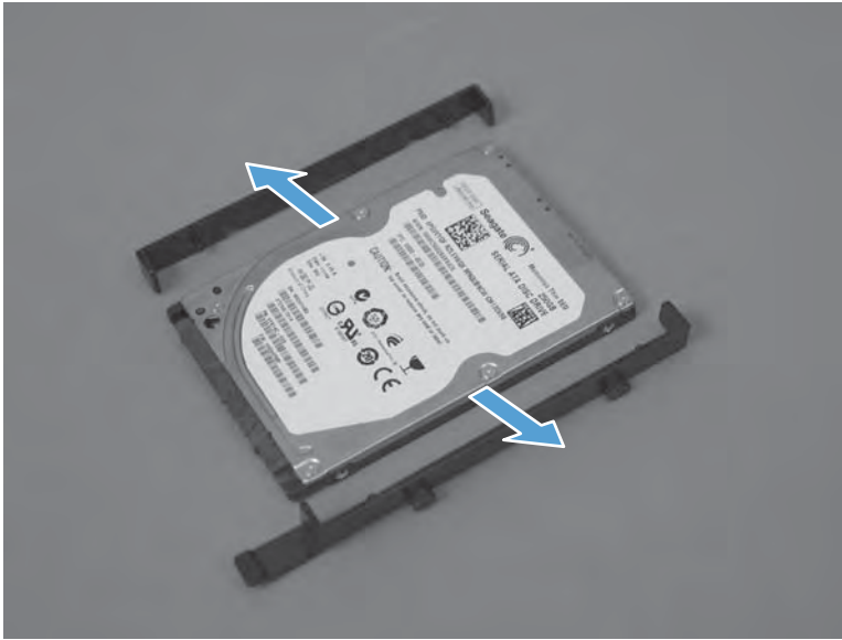
Figure 2-40 Remove the encrypted HDD (5 of 5)
