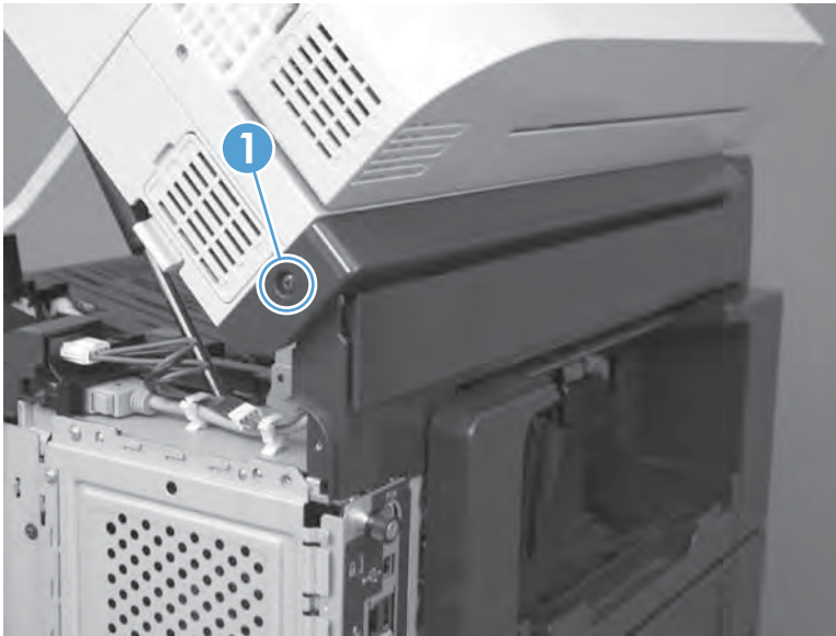
Figure 2-79 Remove the document feeder hinge cover (1 of 3)
