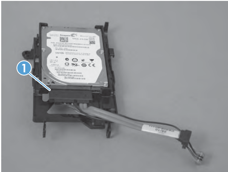
Figure 2-38 Remove the encrypted HDD (3 of 5)
