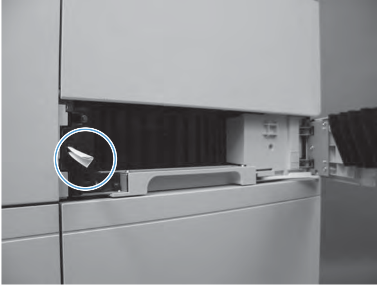
Figure 3-4 Test the SW105 right upper door switch
