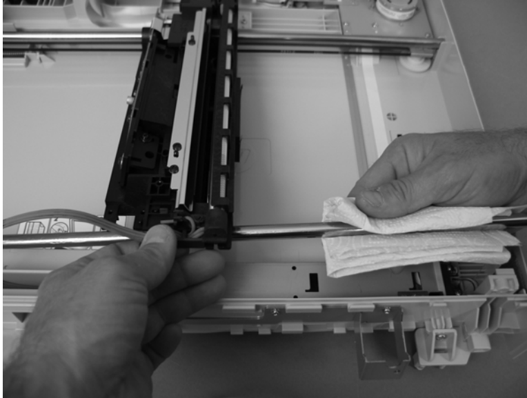
Figure 2-215 Remove the interconnect board and size sensor (2 of 4)
