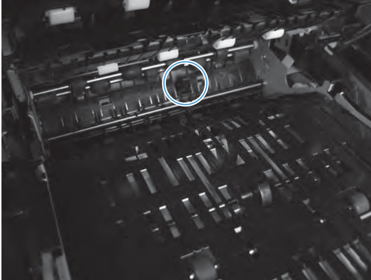
Figure 3-15 Test the PS112 output sensor
