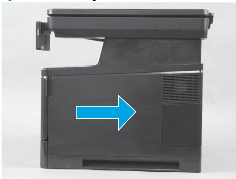
Figure 1-24 Remove the right cover (2 of 2)
