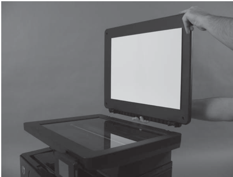
Figure 1-65 Remove the SSA lid (2 of 2)
