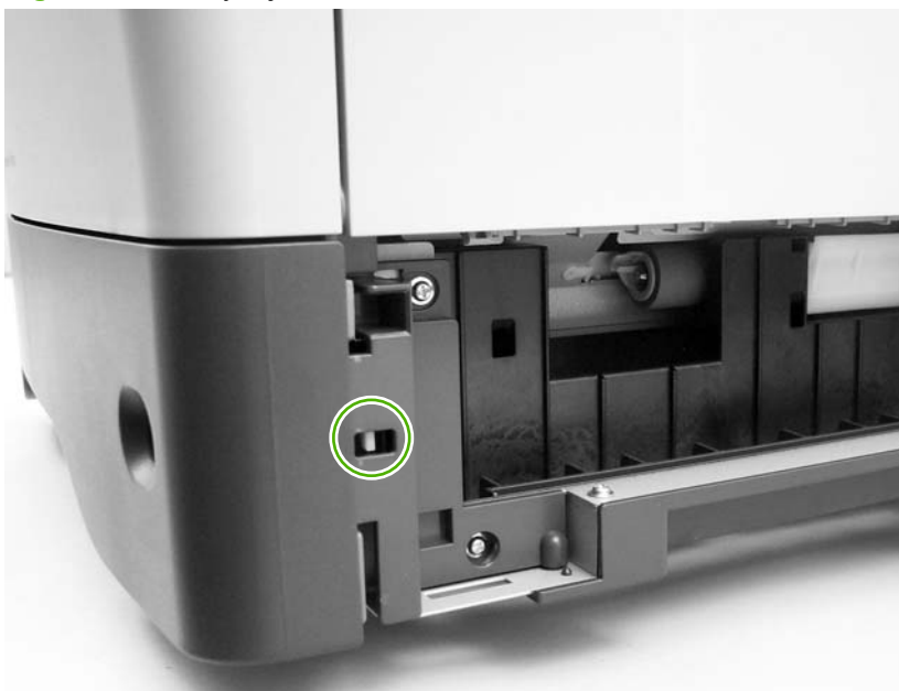
Figure 4-76 Tray 2 jam-access-cover switch, SW105
