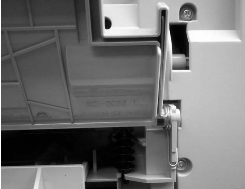
Figure 5-79 Correct tray 1 rear-hinge-spring placement
