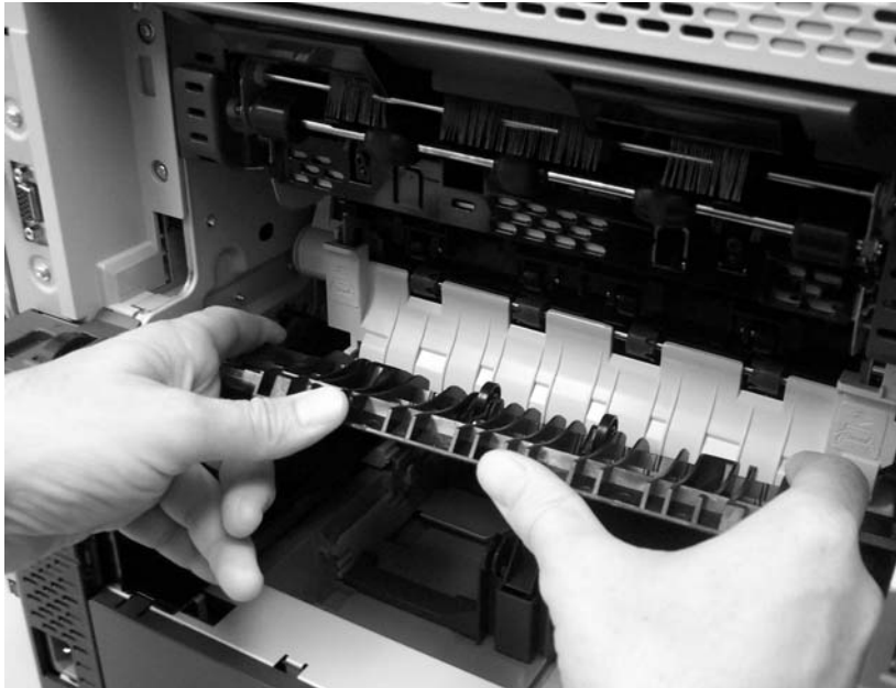
Figure 5-20 Remove the fuser-entrance guide
