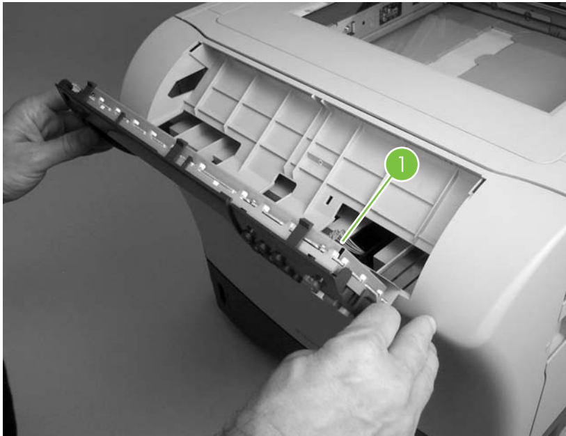
Figure 5-3 Remove the control panel (2 of 2)
