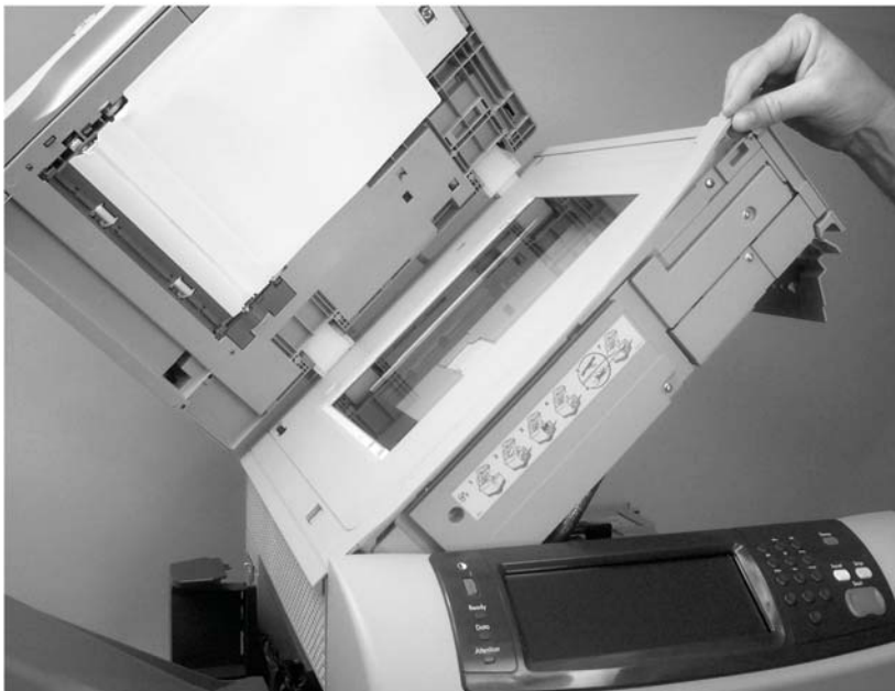
Figure 5-37 Remove the top-cover flatbed flange (1 of 2)
