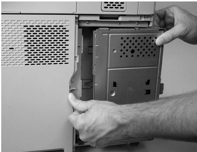
Figure 5-32 Remove the formatter cover and formatter (3 of 3)
