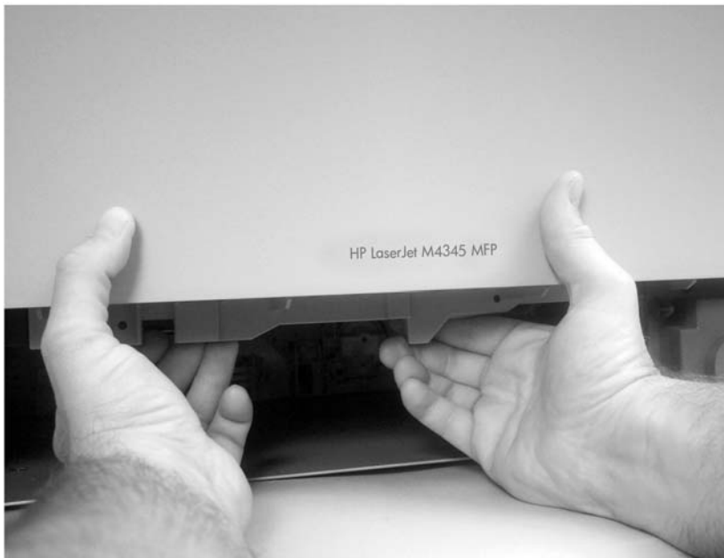
Figure 5-44 Remove the front cover (6 of 7)
