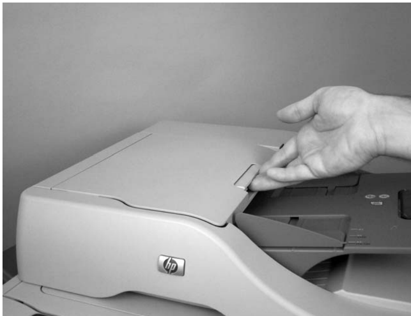
Figure 5-5 Remove the ADF input tray (1 of 3)
