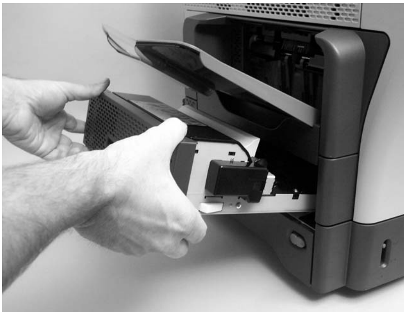
Figure 5-19 Remove the duplex-printing unit (2 of 2)
