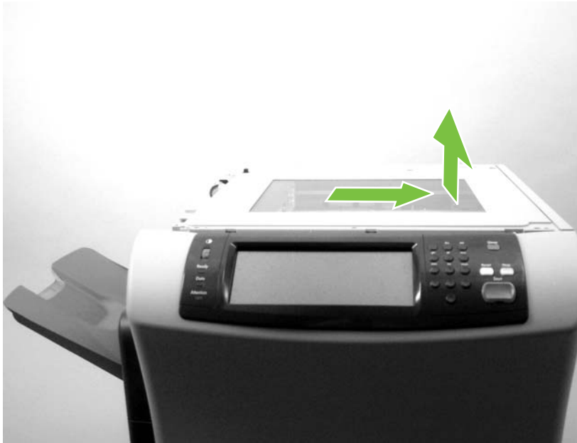
Figure 5-178 Remove the scanner assembly (8 of 8)
