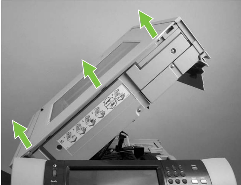
Figure 5-171 Remove the scanner assembly (1 of 8)
