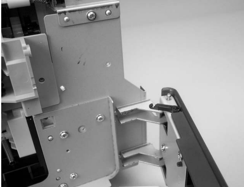
Figure 5-83 Remove the tray 1 feed-assembly (1 of 13)
