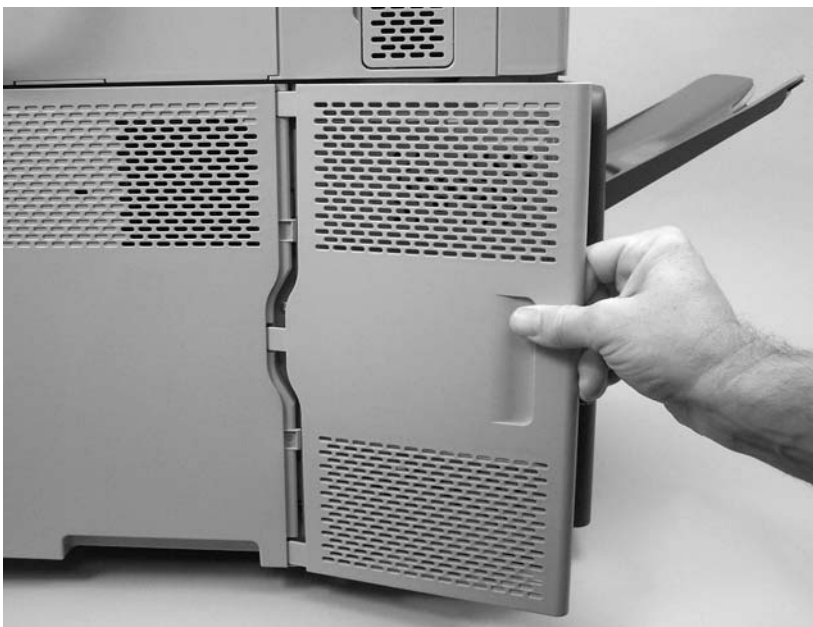
Figure 5-30 Remove the formatter cover and formatter (1 of 3)
