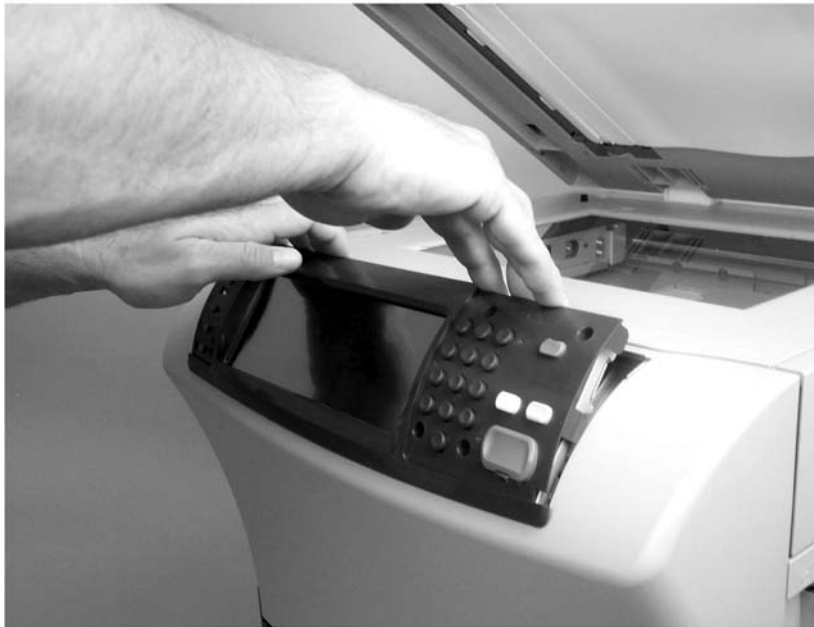
Figure 5-2 Remove the control panel (1 of 2)
