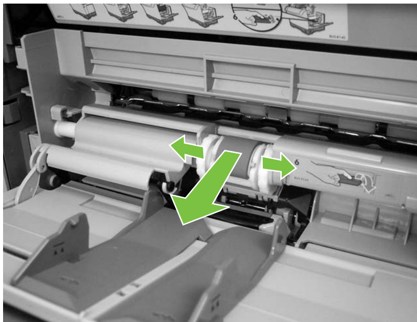
Figure 5-24 Remove the tray 1 pickup roller
