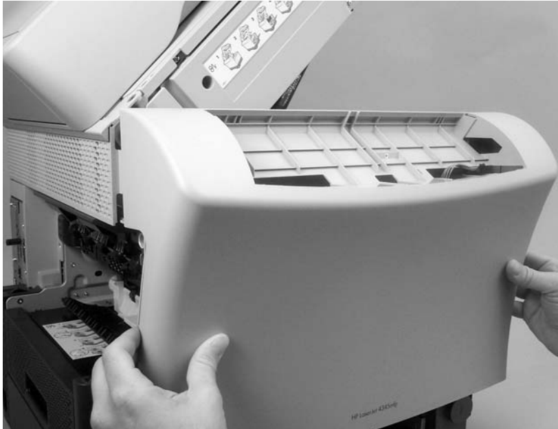
Figure 5-45 Remove the front cover (7 of 7)
