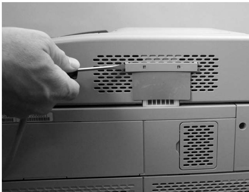
Figure 5-28 Remove the ADF-hinge flap (2 of 3)
