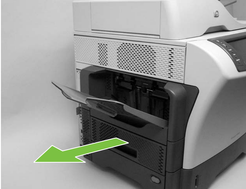
Figure 5-18 Remove the duplex-printing unit (1 of 2)
