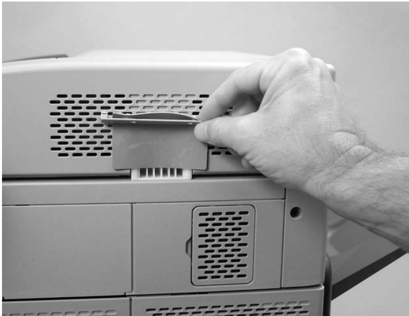
Figure 5-29 Remove the ADF-hinge flap (3 of 3)
