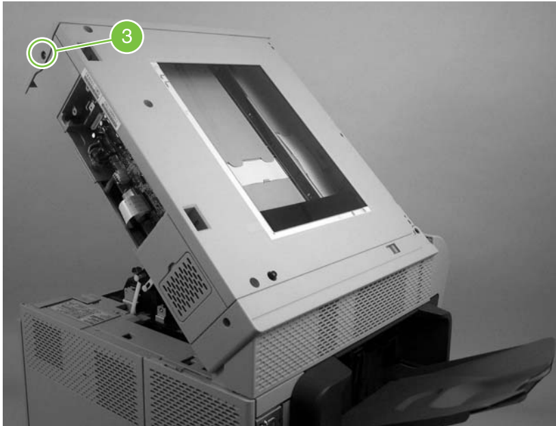
Figure 5-173 Remove the scanner assembly (3 of 8)
