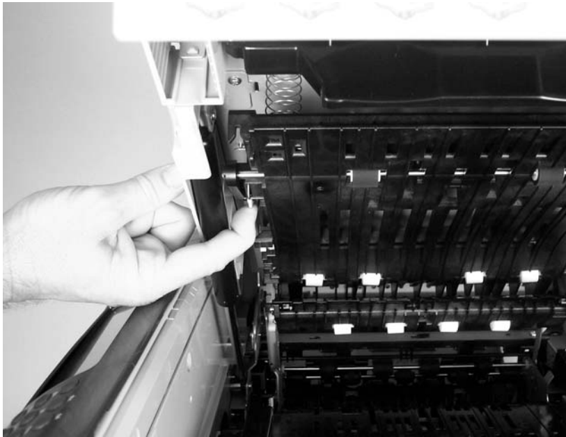
Figure 5-49 Remove the reversing-separation-guide assembly (1 of 2)
