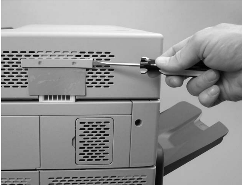
Figure 5-27 Remove the ADF-hinge flap (1 of 3)
