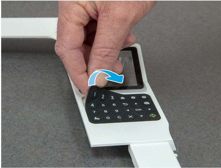
Figure 5-273 Remove the keypad
