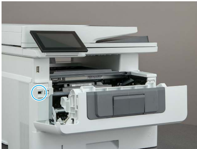
Figure 4-22 Defeat the front (cartridge) door interlock
