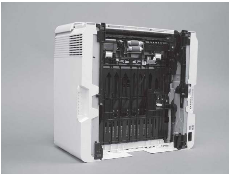
Figure 2-10 Place the printer bottom-side face forward
