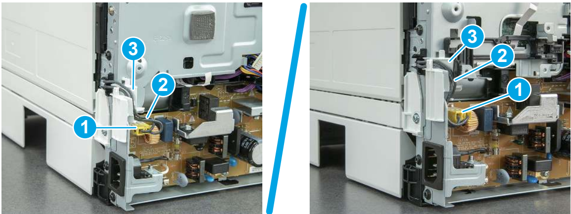
Figure 5-801 SFP/MFP: Remove the wire harness
