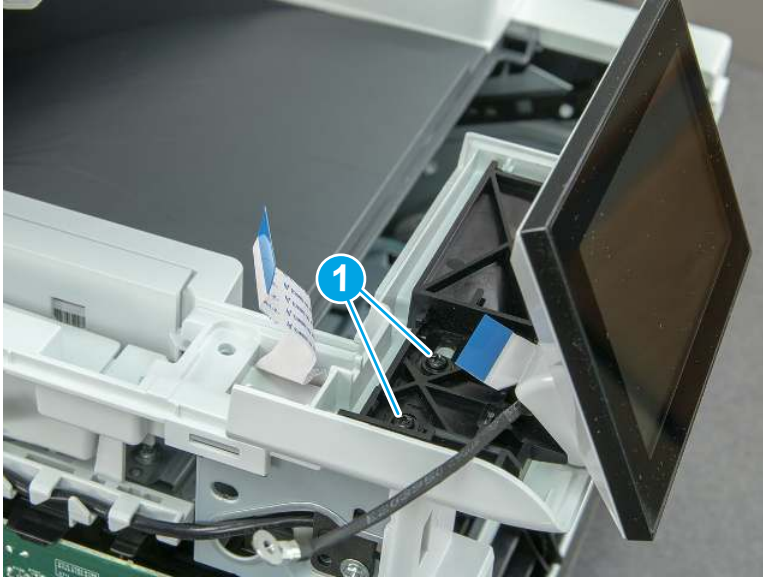
Figure 5-833 Remove two screws and remove the control panel assembly
