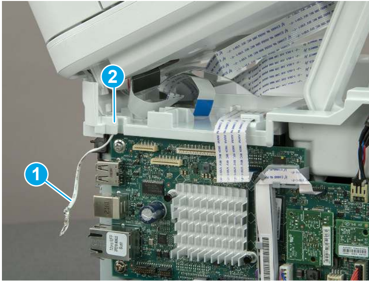
Figure 5-218 Release the ground wire
