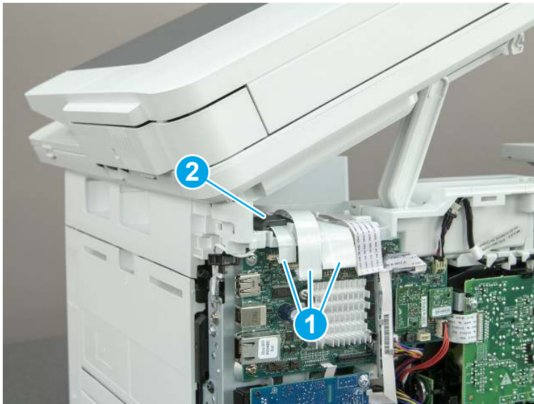
Figure 5-215 Disconnect three FFCs
