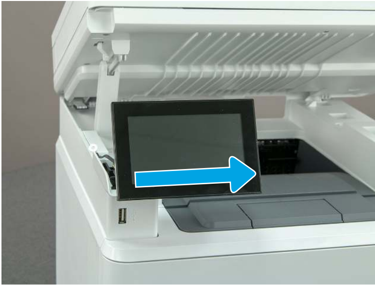
Figure 5-956 Slide the control panel display
