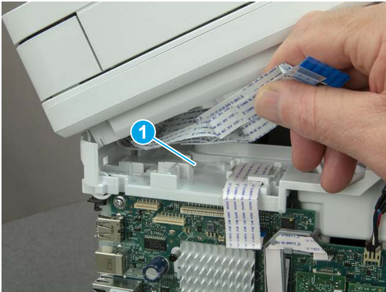
Figure 5-666 Release the tape
