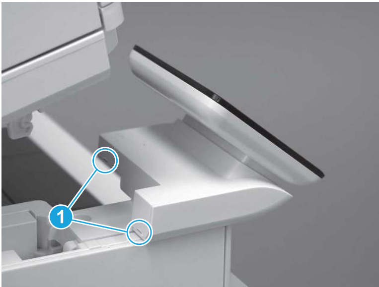
Figure 5-188 Release two tabs
