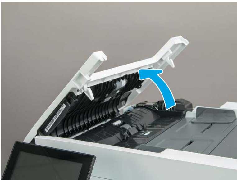
Figure 5-52 Open the document feeder top cover
