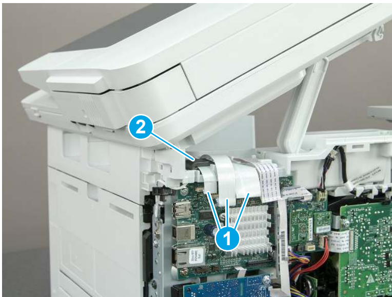
Figure 5-76 Disconnect three FFCs
