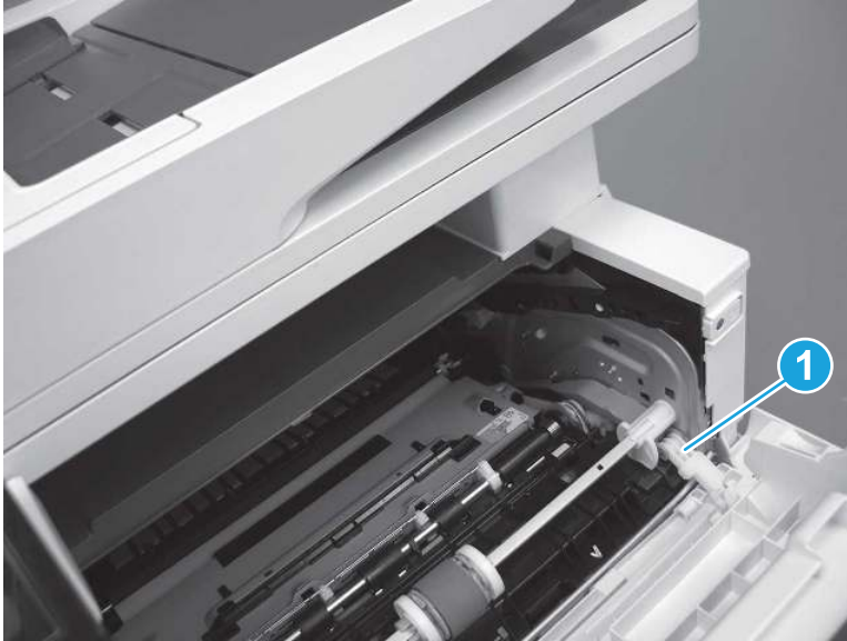
Figure 5-817 Release the pressure-release link
