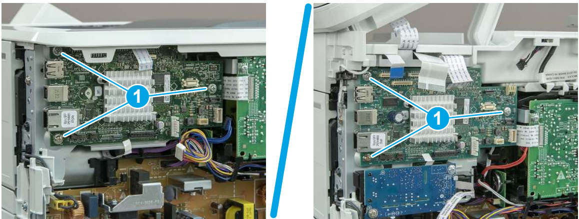
Figure 5-507 Remove three screws
