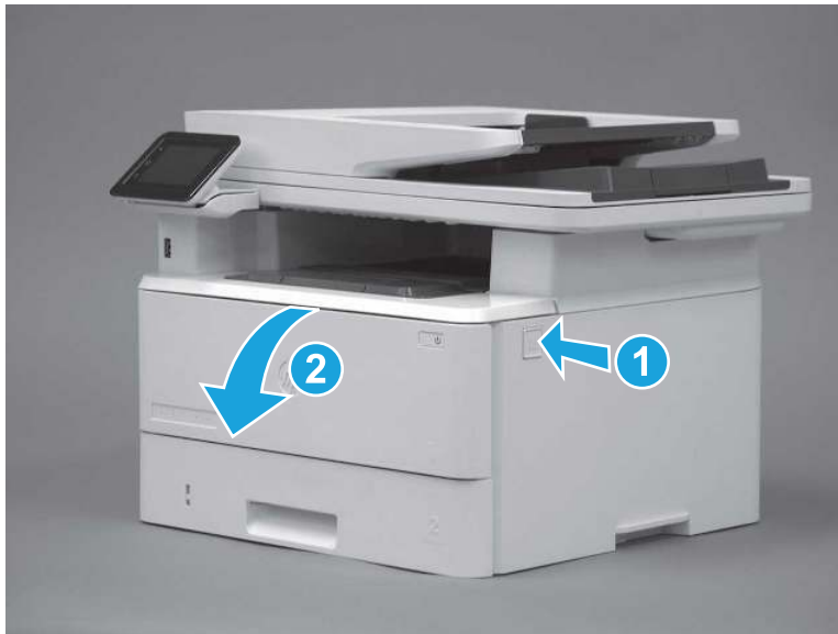
Figure 2-1 Open the toner-cartridge door
