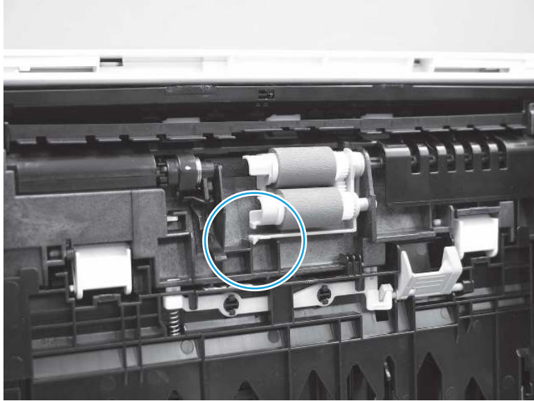
Figure 4-86 Check the tab
