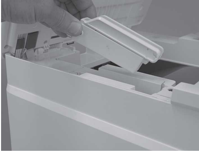
Figure 5-62 Remove the support arm
