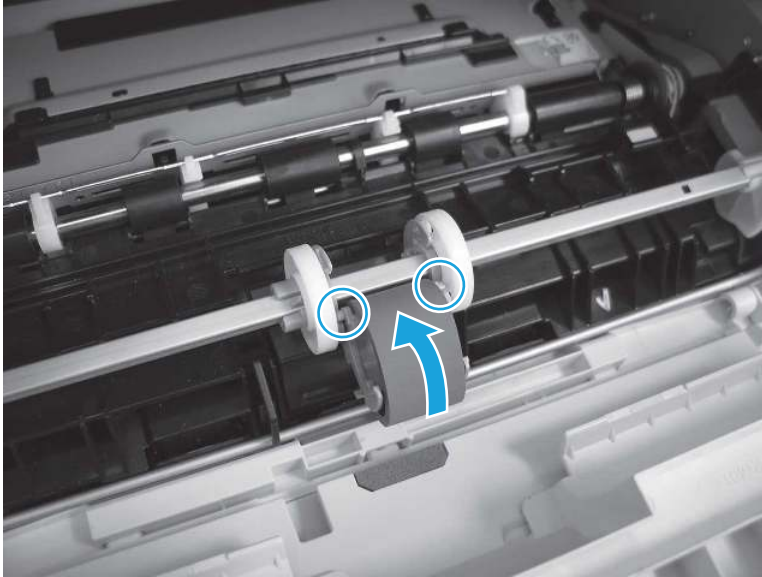
Figure 4-78 Install the roller
