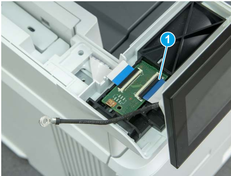
Figure 5-955 Disconnect one flat cable
