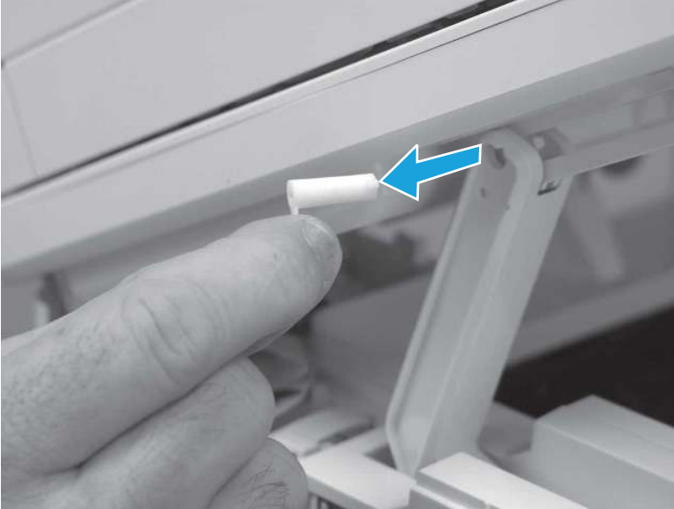
Figure 5-81 Remove the slider pin
