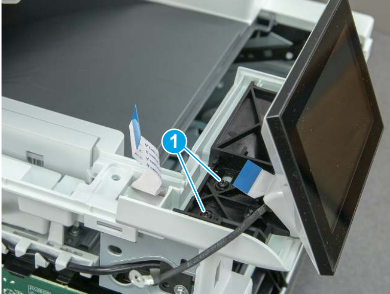
Figure 5-561 Remove two screws and remove the control panel assembly
