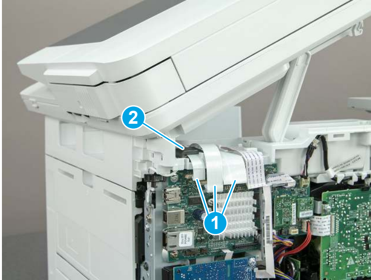
Figure 5-839 Disconnect three FFCs
