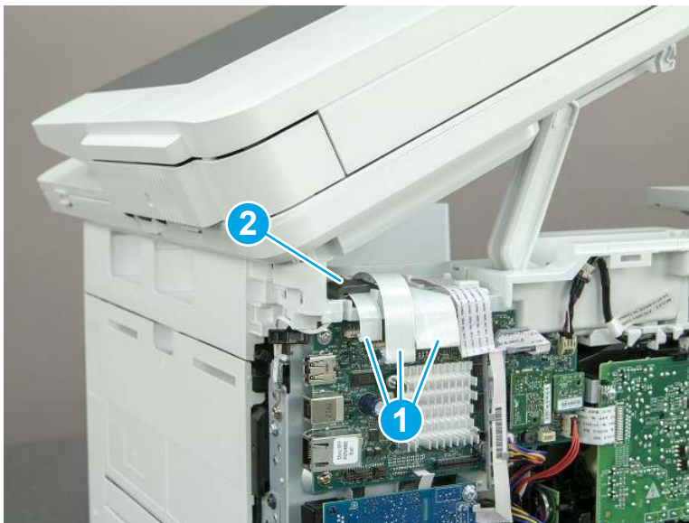
Figure 5-291 Disconnect three FFCs
