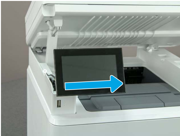
Figure 5-973 Slide the control panel display
