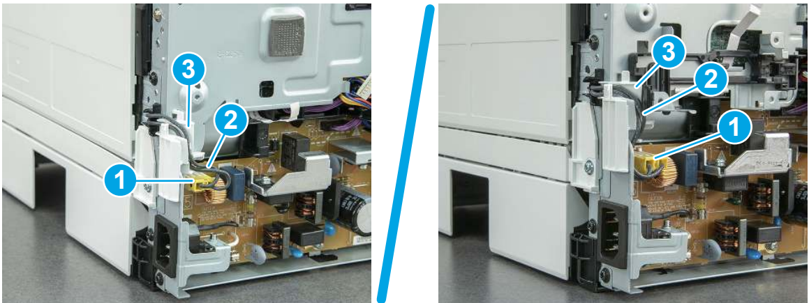
Figure 5-633 SFP/MFP: Remove the wire harness
