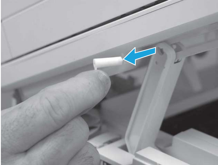
Figure 5-616 Remove the slider pin
