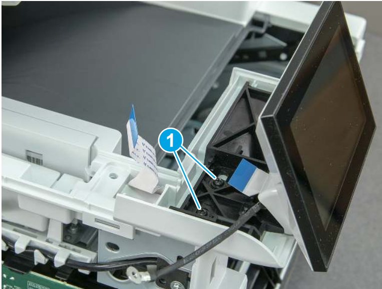
Figure 5-361 Remove two screws and remove the control panel assembly
