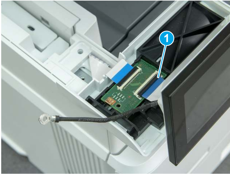
Figure 5-972 Disconnect one flat cable
