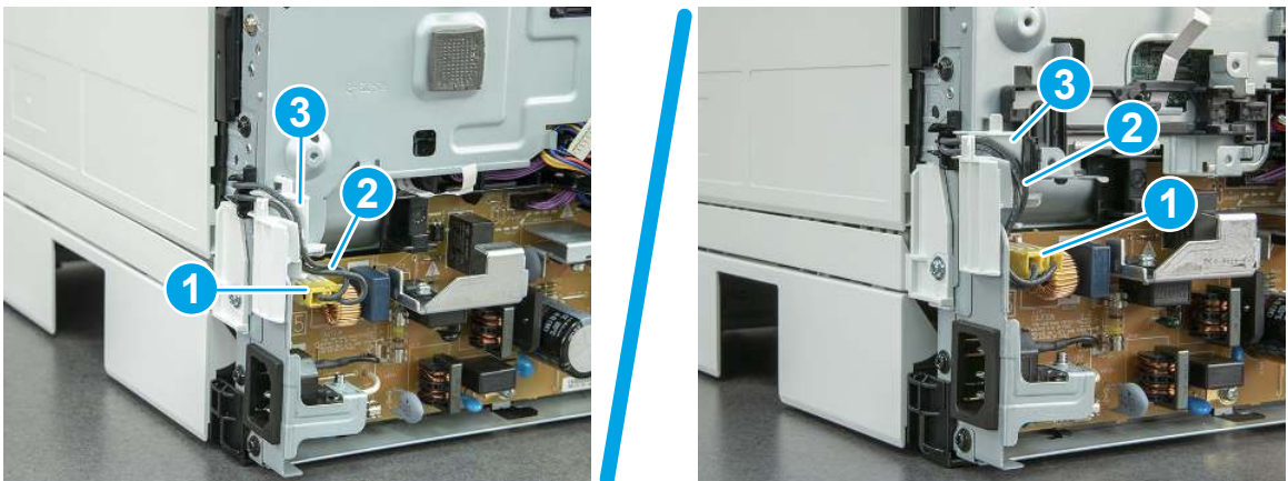
Figure 5-687 SFP/MFP: Remove the wire harness
