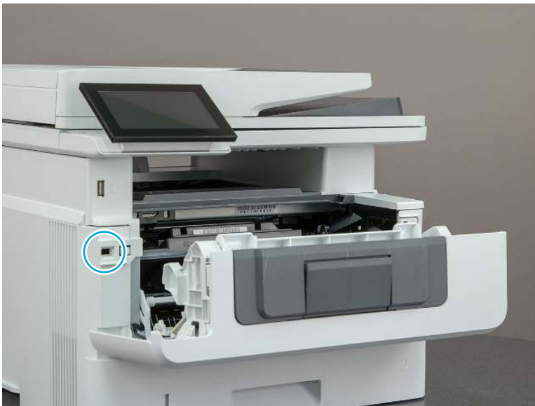
Figure 4-43 Defeat the front (cartridge) door interlock
