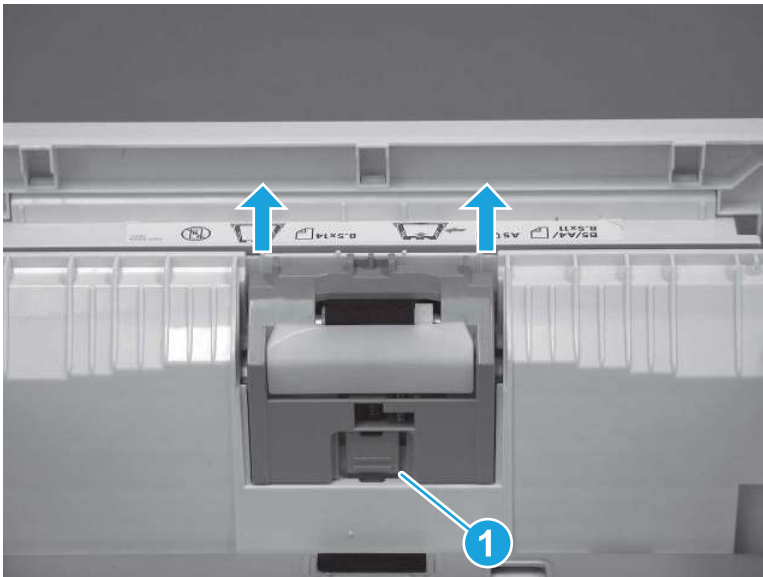
Figure 5-28 Release the assembly
