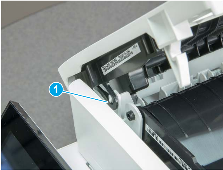
Figure 5-53 Release one hinge pin
