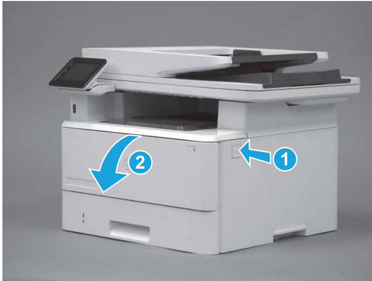
Figure 5-11 Open the toner-cartridge door
