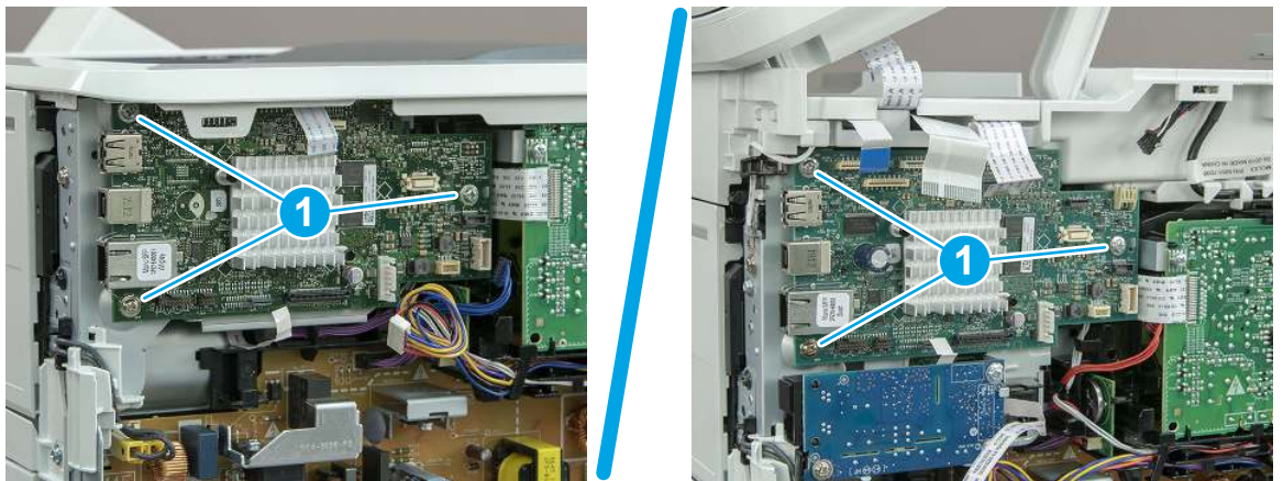
Figure 5-860 Remove three screws
