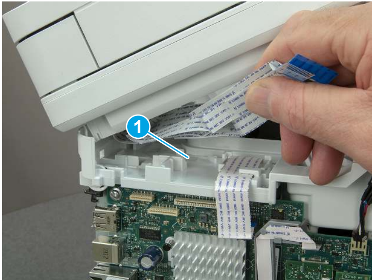
Figure 5-840 Release the tape
