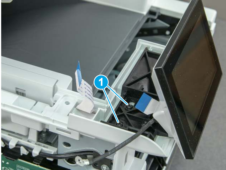
Figure 5-193 Remove two screws and remove the control panel assembly
