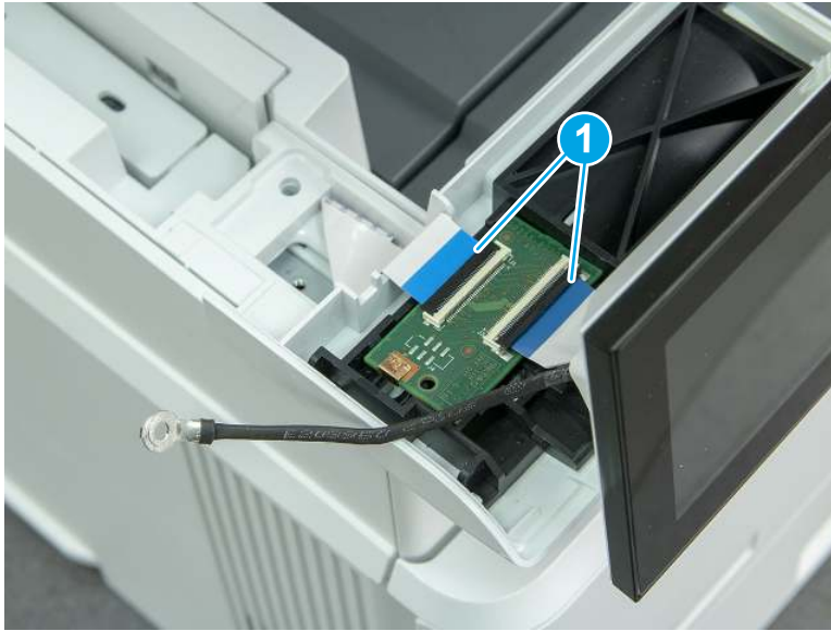
Figure 5-559 Disconnect two FFC
