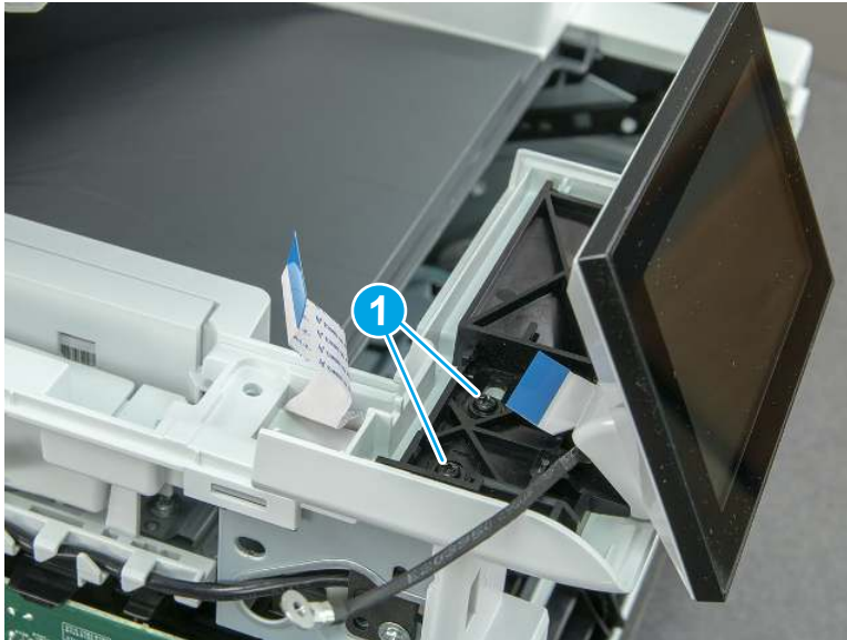
Figure 5-307 Remove two screws and remove the control panel assembly
