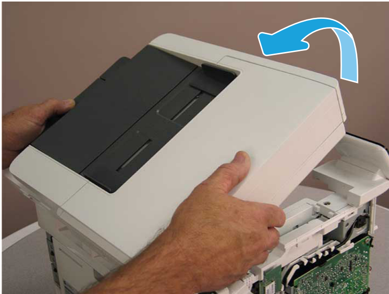
Figure 5-297 Rotate the ISA towards the rear of the printer
