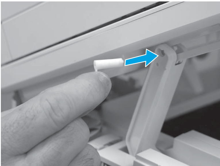
Figure 1-573 Install the slider pin
