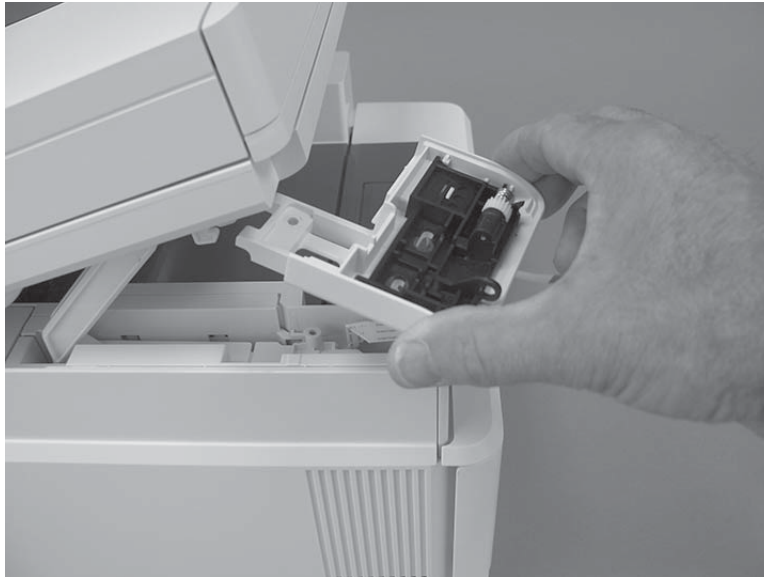
Figure 1-2168 Release the control panel mount base
