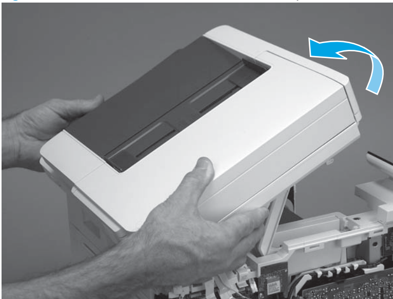
Figure 1-314 Rotate the ISA towards the rear of the printer
