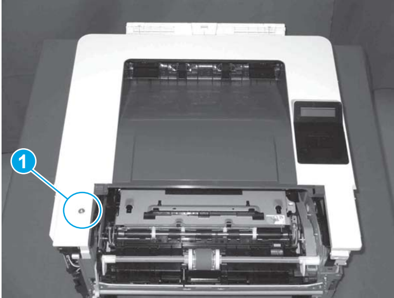
Figure 1-1780 Remove one screw
