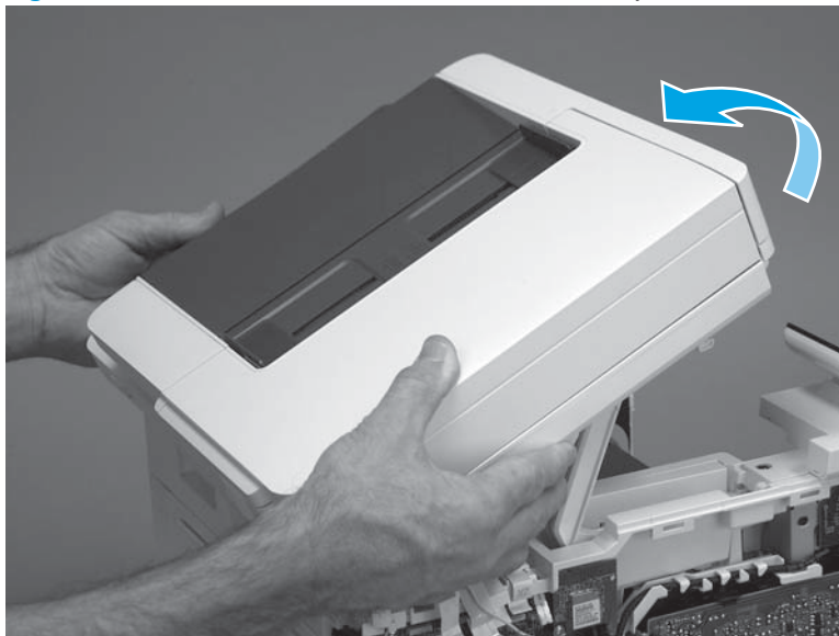
Figure 1-965 Rotate the ISA towards the rear of the printer
