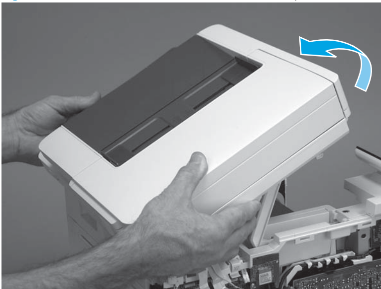
Figure 1-2052 Rotate the ISA towards the rear of the printer
