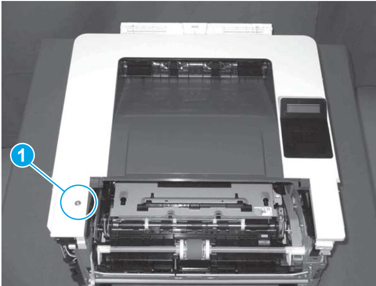
Figure 1-234 Remove one screw
