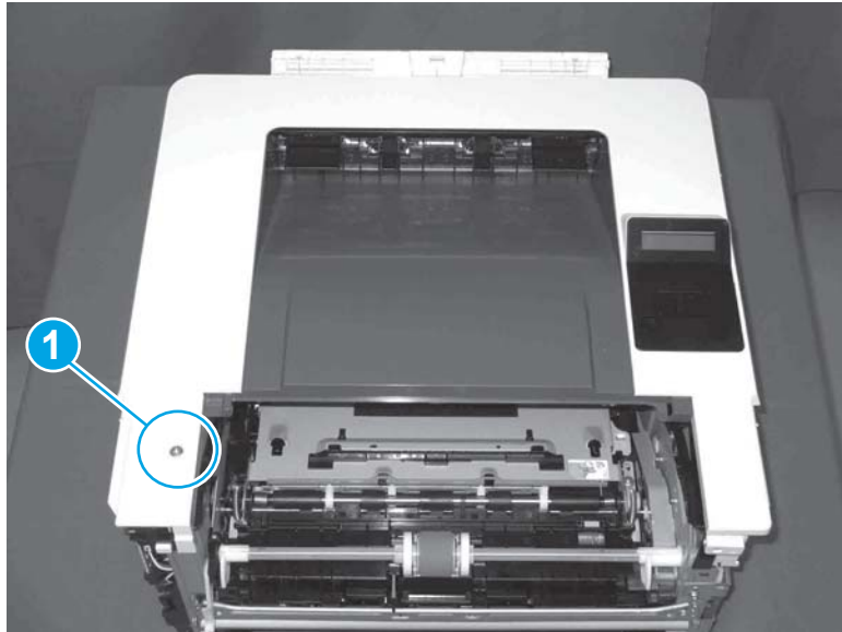
Figure 1-218 Remove one screw
