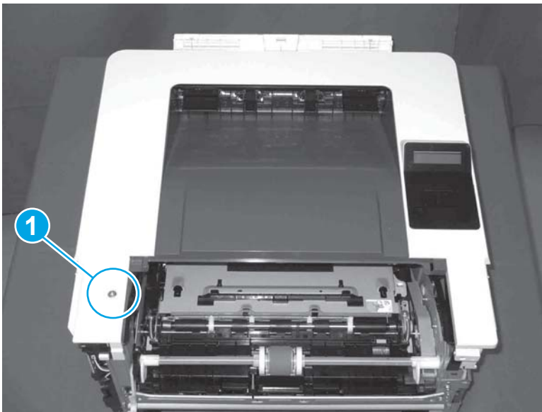
Figure 1-526 Remove one screw
