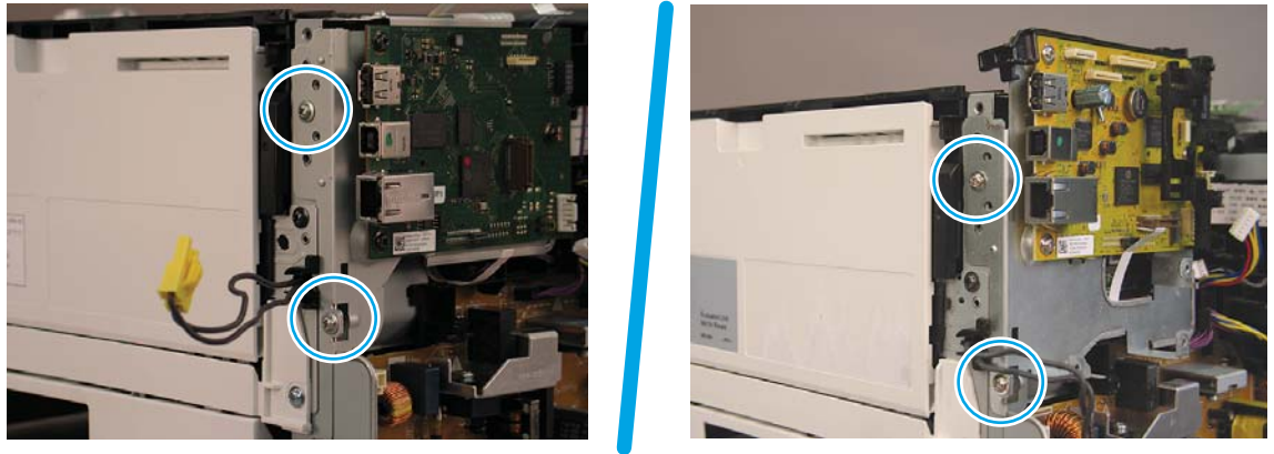
Figure 1-742 Remove two screws
