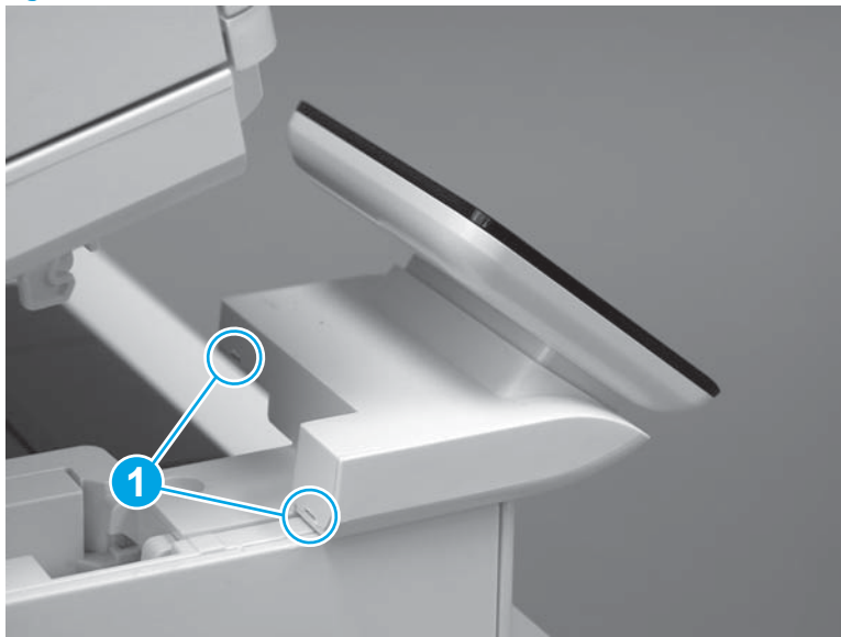
Figure 1-985 Release two tabs
