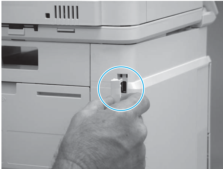
Figure 1-78 Remove the cover
