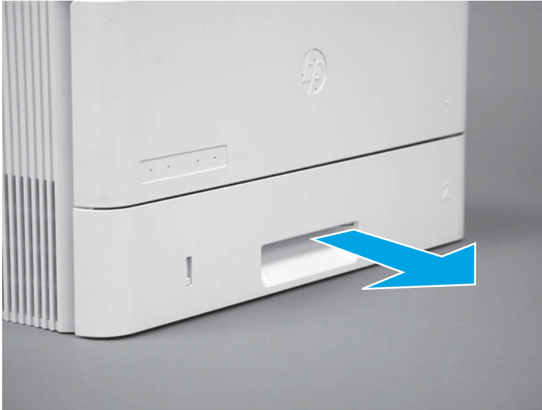
Figure 1-278 Remove the tray
