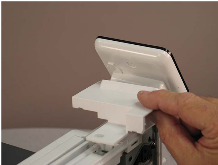
Figure 1-932 Remove the cover
