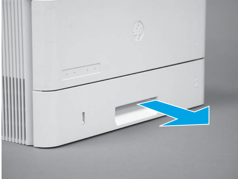
Figure 1-101 Remove the tray
