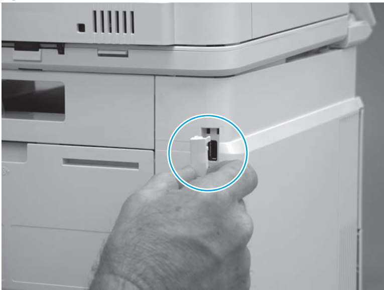
Figure 1-58 Remove the cover
