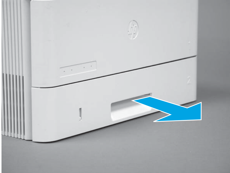
Figure 1-390 Remove the tray
