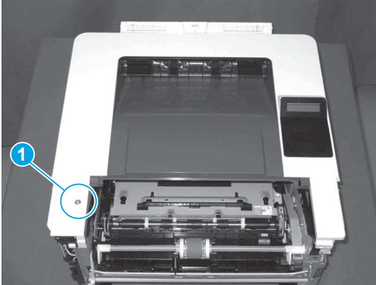
Figure 1-591 Remove one screw
