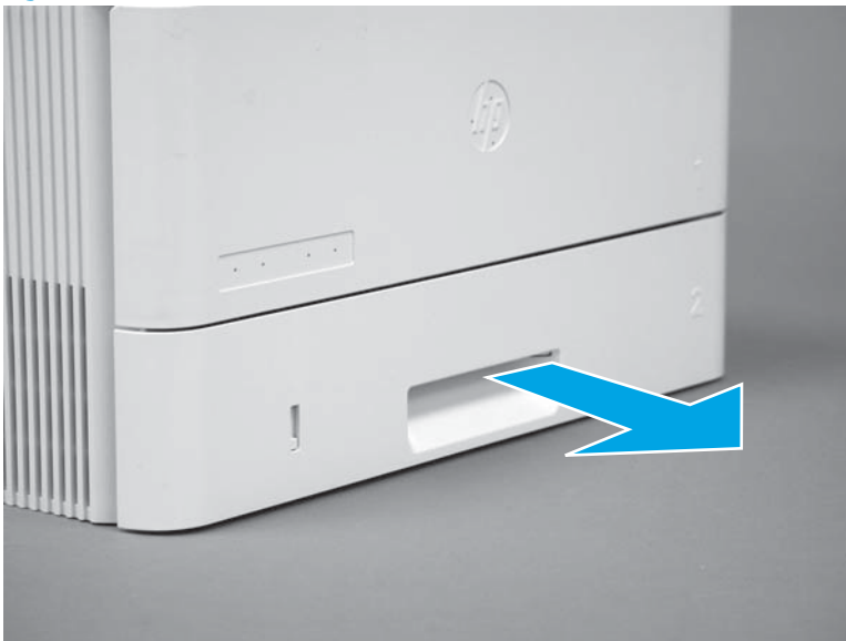
Figure 1-749 Remove the tray
