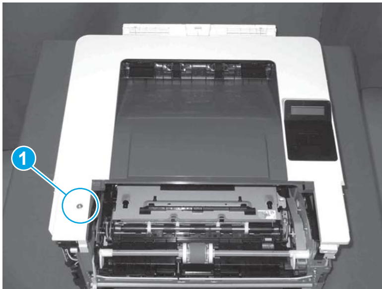
Figure 1-940 Remove one screw
