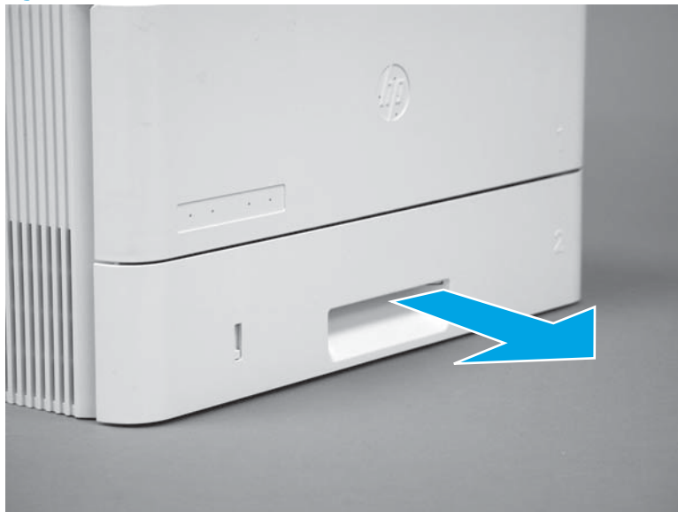
Figure 1-699 Remove the tray
