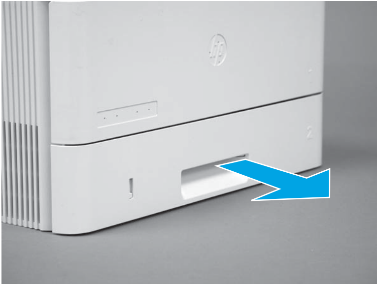
Figure 1-578 Remove the tray
