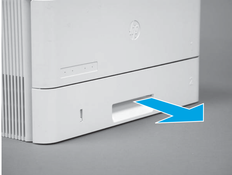
Figure 1-1025 Remove the tray
