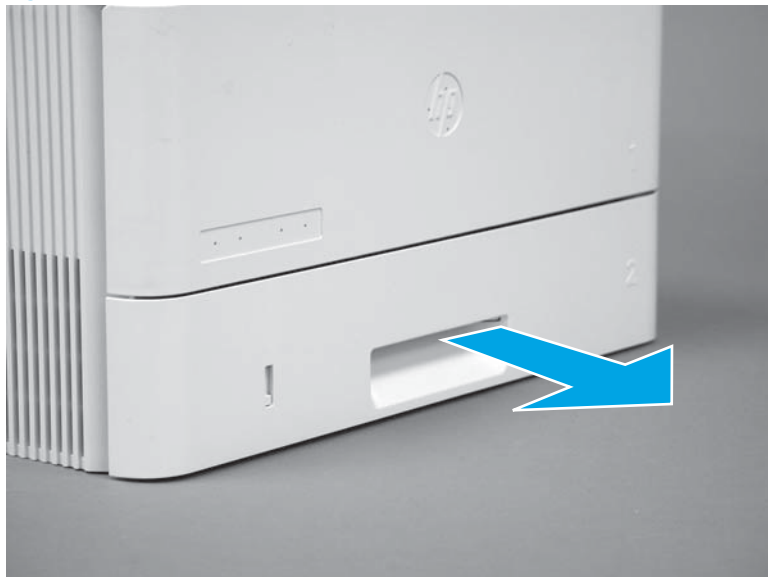
Figure 1-492 Remove the tray
