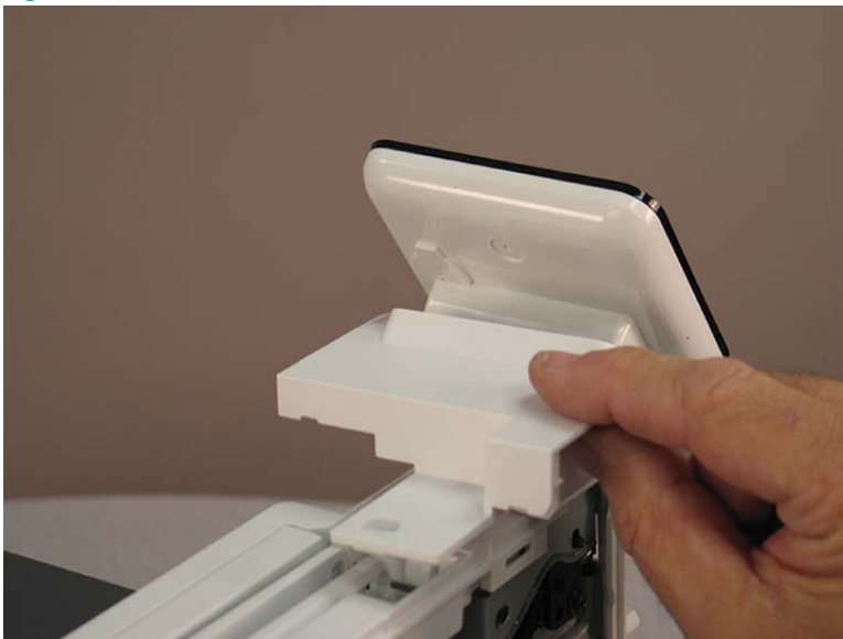
Figure 1-624 Remove the cover
