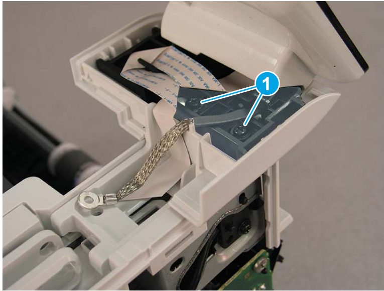
Figure 1-992 Remove two screws
