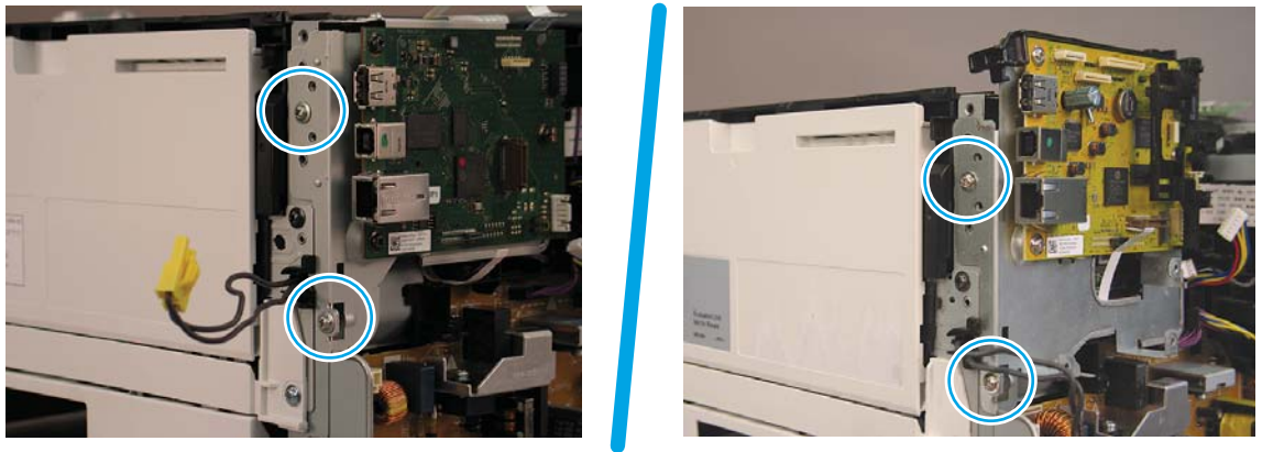
Figure 1-574 Remove two screws
