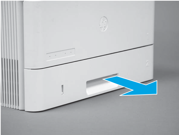
Figure 1-532 Remove the tray
