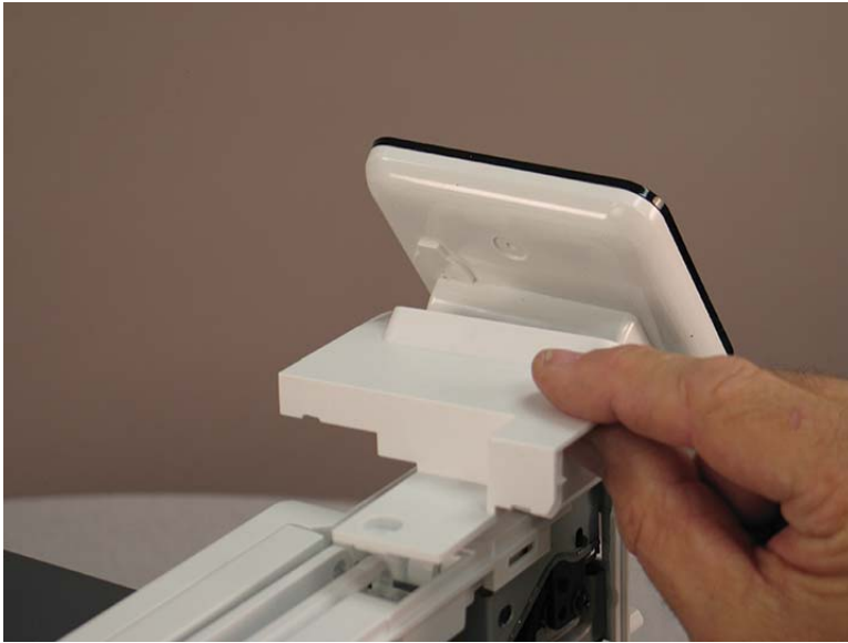
Figure 1-990 Remove the cover
