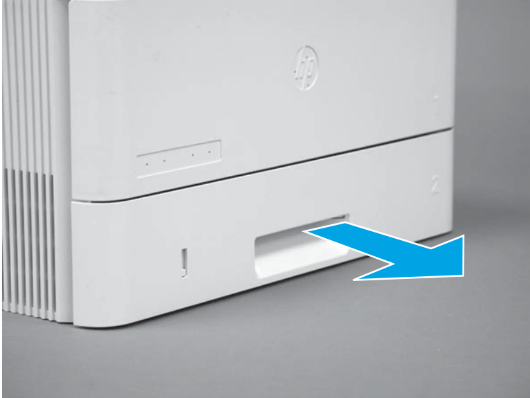
Figure 1-221 Remove the tray
