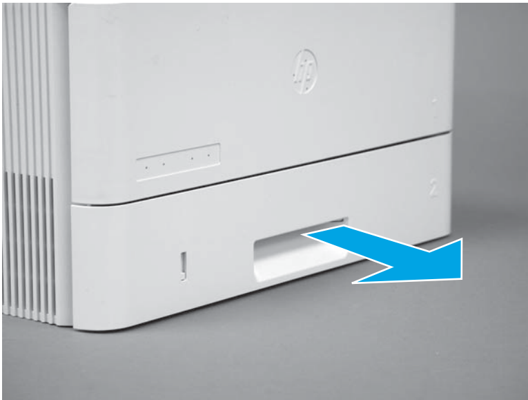
Figure 1-80 Remove the tray
