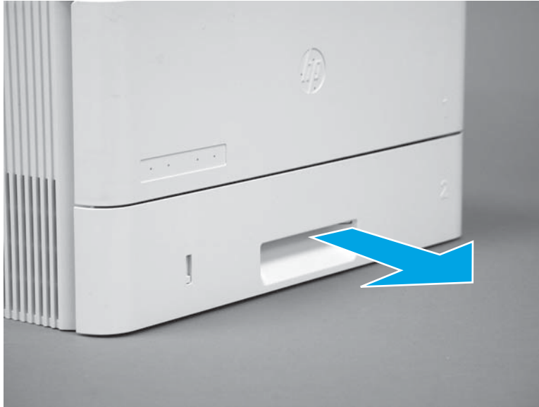
Figure 1-964 Remove the tray
