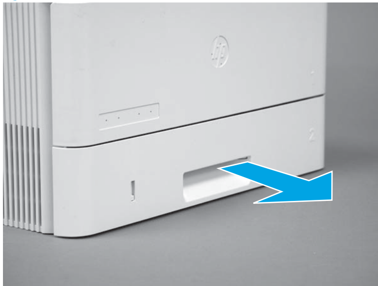
Figure 1-646 Remove the tray
