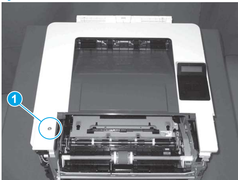
Figure 1-362 Remove one screw
