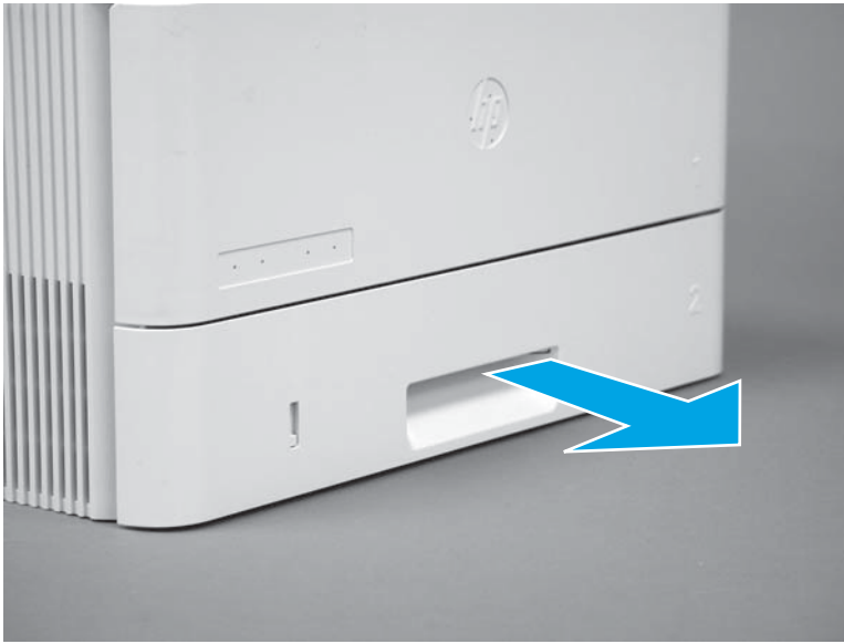
Figure 1-305 Remove the tray
