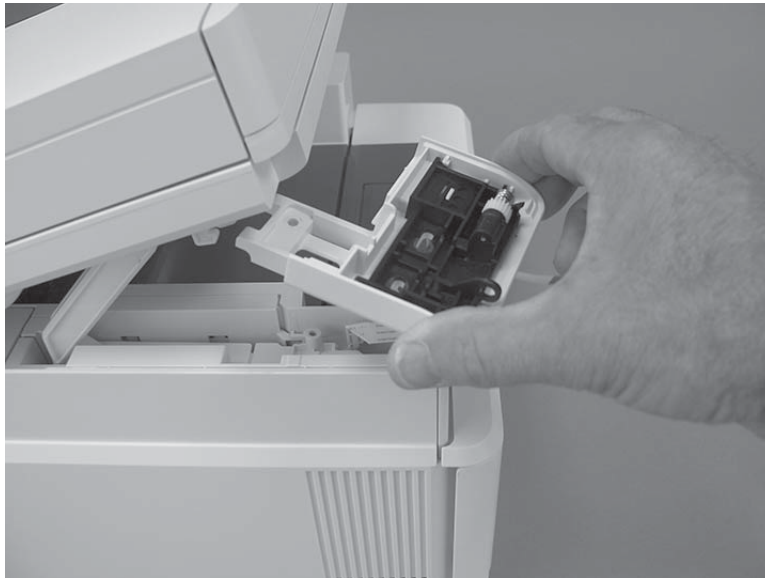
Figure 1-997 Release the control panel mount base
