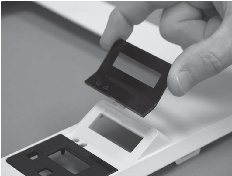
Figure 1-238 Remove the cover
