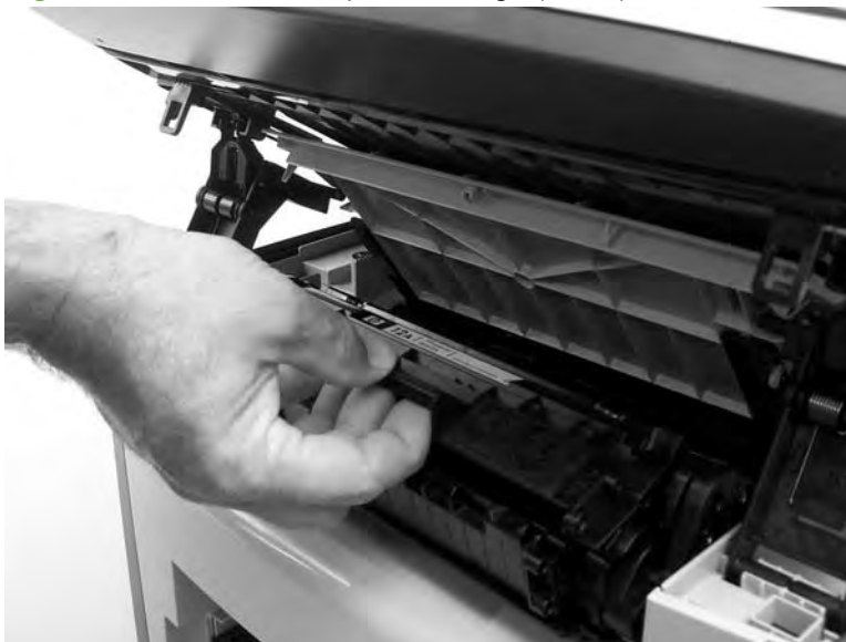
Figure 5-40 Remove the print cartridge (2 of 2)
