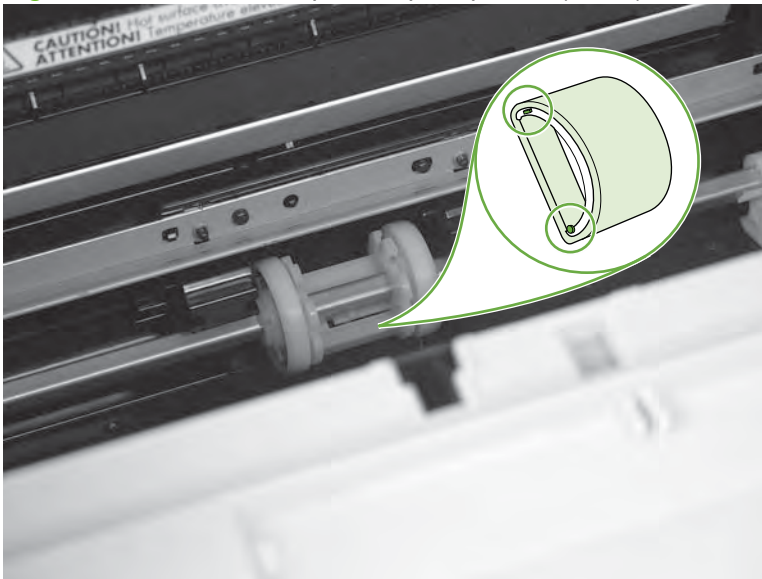
Figure 5-46 Remove the product pickup roller (4 of 5)
