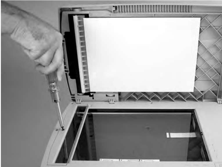
Figure 5-26 Remove the ADF scanner glass (1 of 3)
