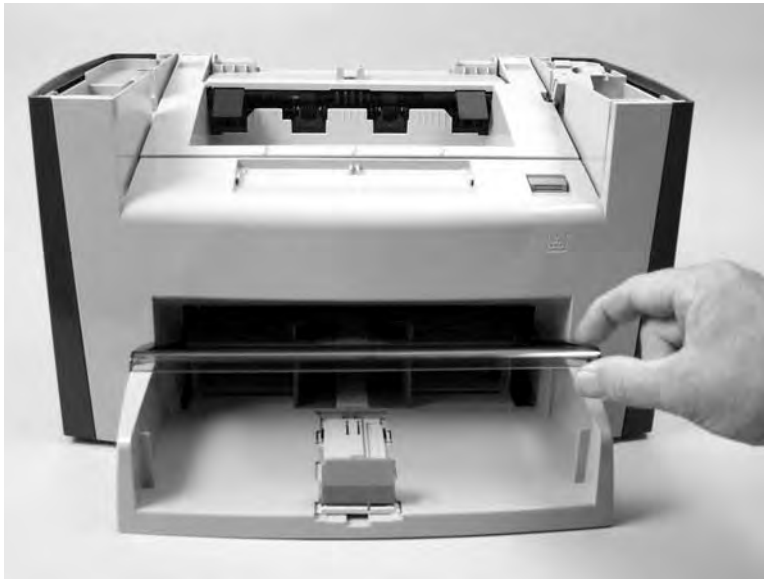
Figure 5-49 Remove the media input tray (1 of 3)
