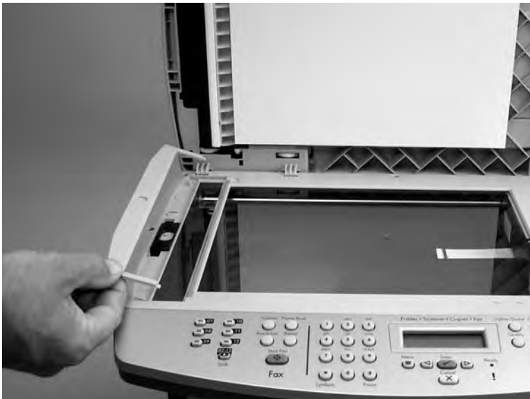
Figure 5-27 Remove the ADF scanner glass (2 of 3)
