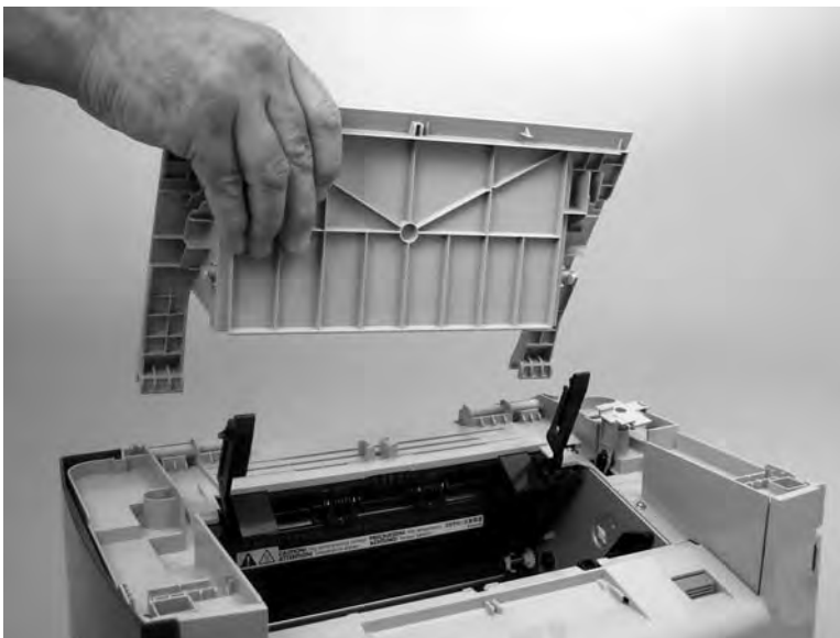
Figure 5-58 Remove the print-cartridge door (2 of 2)
