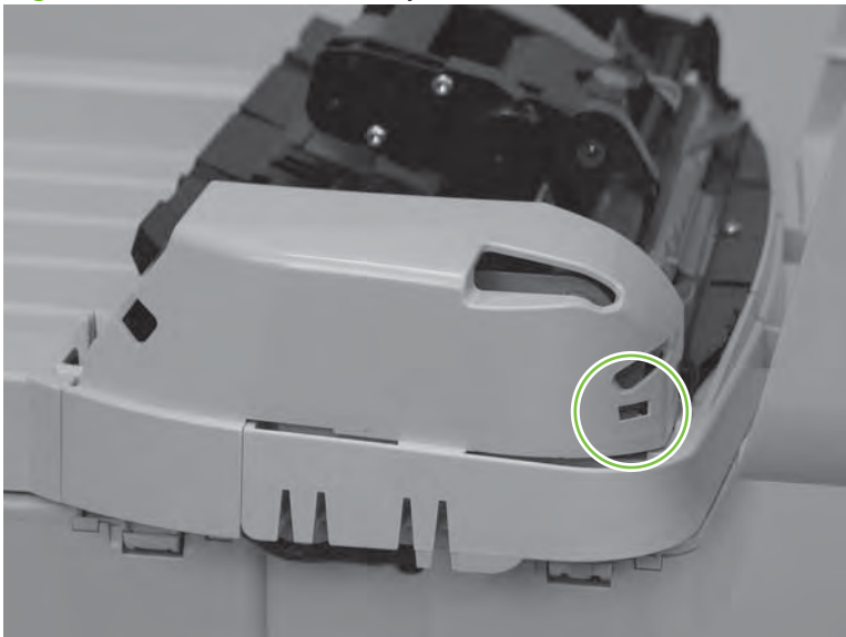
Figure 5-6 ADF cover correctly installed
