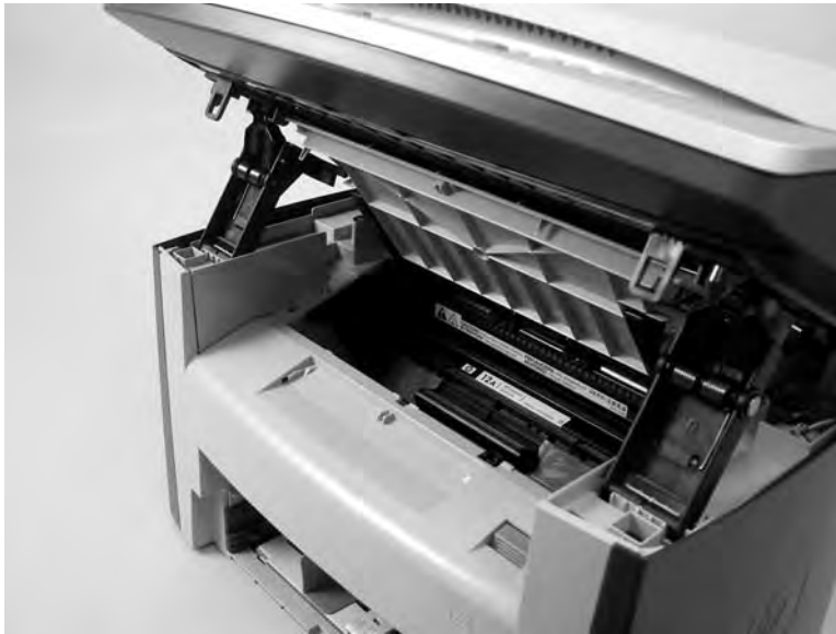
Figure 5-39 Remove the print cartridge (1 of 2)
