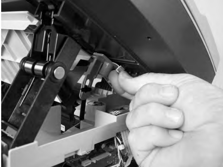
Figure 5-35 Remove the scanner assembly (7 of 10)
