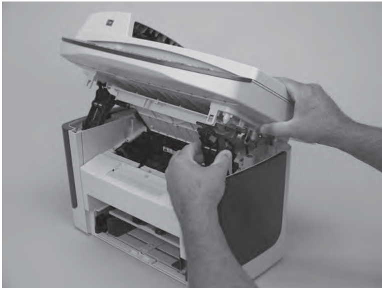
Figure 5-12 Remove the link assemblies and scanner support-frame springs (2 of 4)
