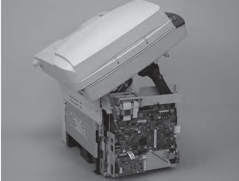
Figure 5-33 Remove the scanner assembly (5 of 10)
