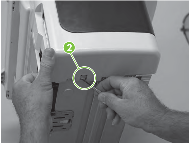
Figure 5-31 Remove the scanner assembly (3 of 10)
