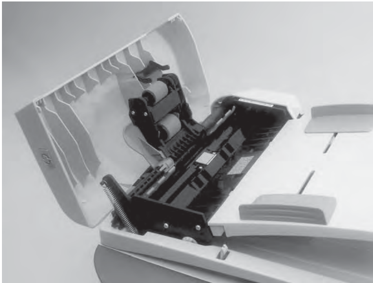
Figure 5-20 Replacing the ADF pickup roller assembly (1 of 6)
