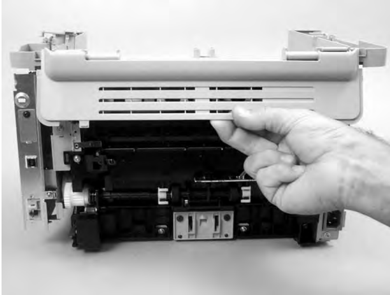
Figure 5-61 Remove the rear cover and fuser cover (3 of 3)
