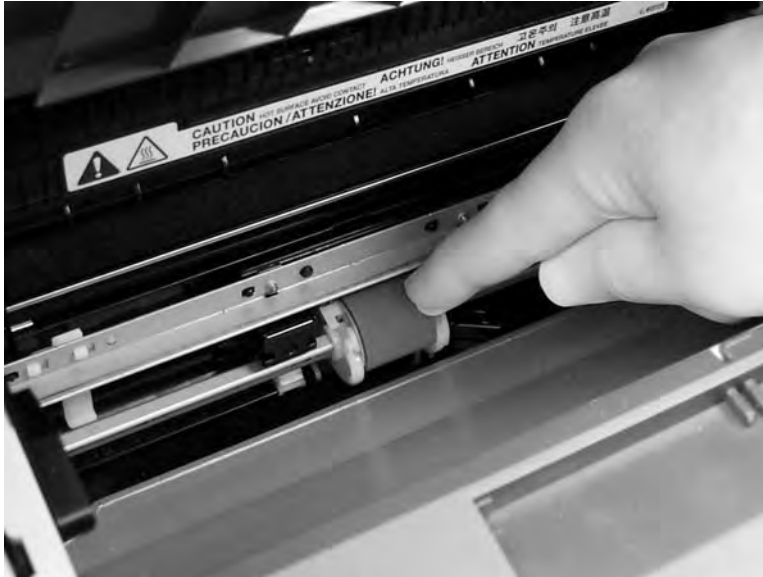
Figure 5-47 Remove the product pickup roller (5 of 5)
