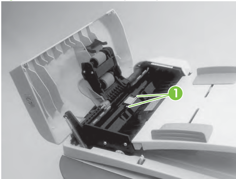
Figure 5-18 Remove the ADF separation pad
