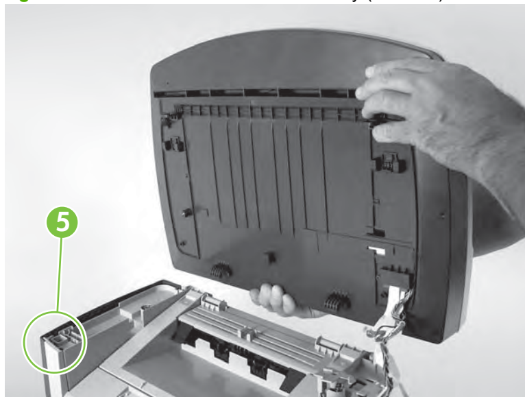
Figure 5-38 Remove the scanner assembly (10 of 10)
