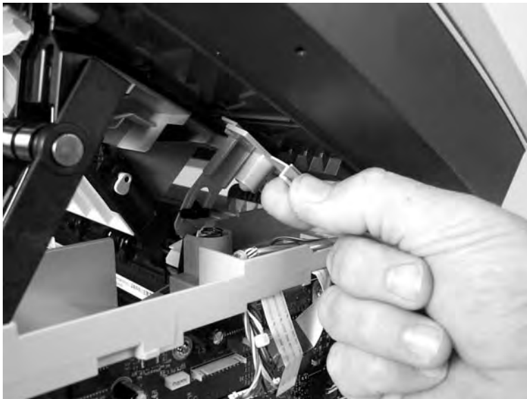
Figure 5-36 Remove the scanner assembly (8 of 10)
