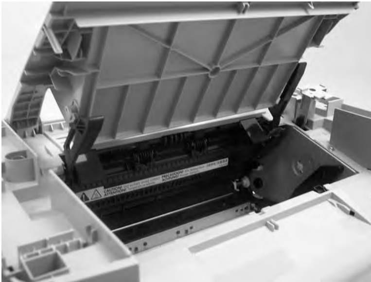
Figure 5-57 Remove the print-cartridge door (1 of 2)
