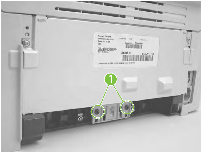
Figure 6-45 Removing the separation pad (1 of 2)
