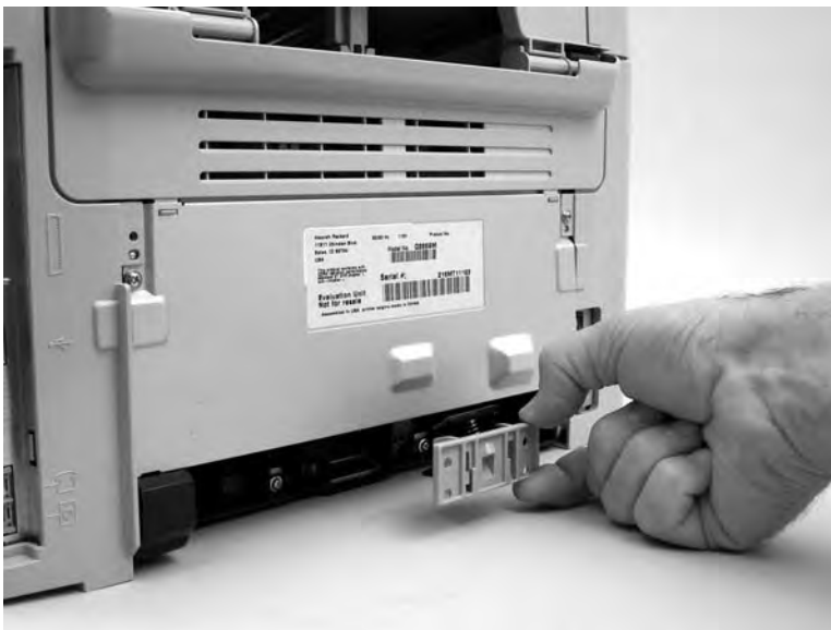
Figure 6-46 Removing the separation pad (2 of 2)
