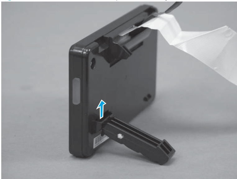
Figure 1-34 Remove the control-panel assembly (4 of 4)
