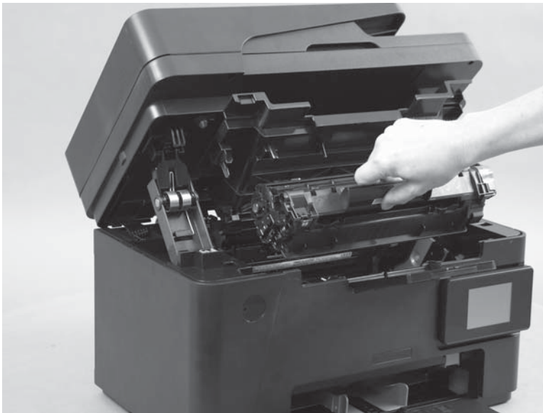
Figure 1-9 Remove the pickup roller (3 of 5)
