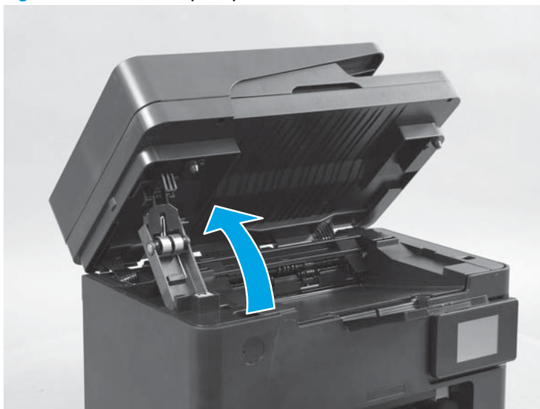
Figure 1-7 Remove the pickup roller (1 of 5)
