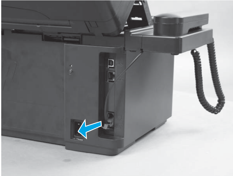
Figure 1-14 Remove the handset (1 of 2)
