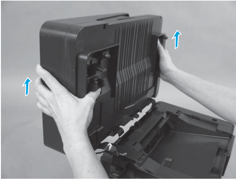
Figure 1-22 Remove the scanner assembly (4 of 4)
