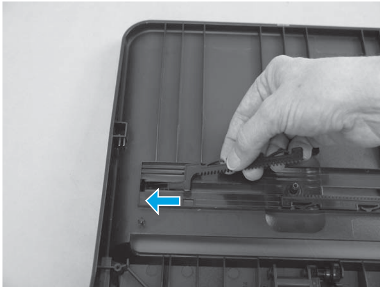
Figure 1-139 Remove the ADF input guides and gear (2 of 3)
